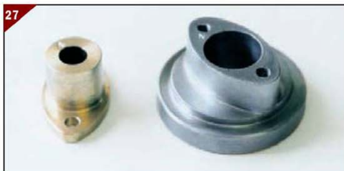
27. The completed bottom cover in cast iron and its brass gland.
