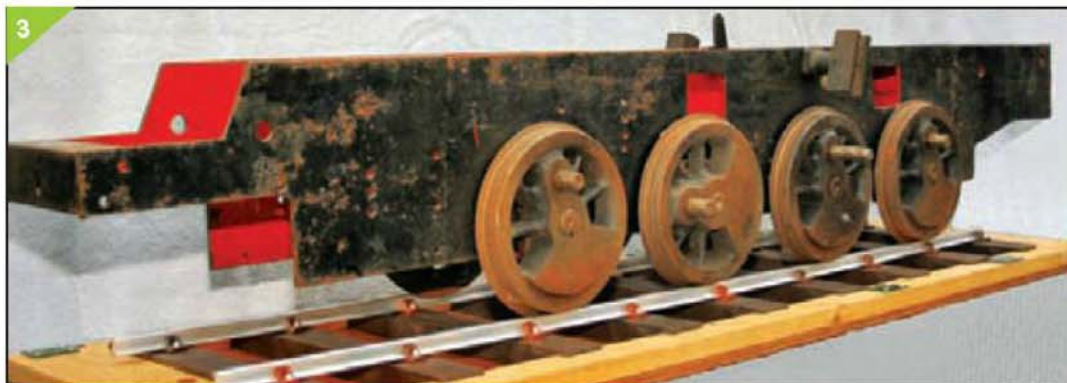
3. Malcolm Freestone's 2-8-0 locomotive chassis.
