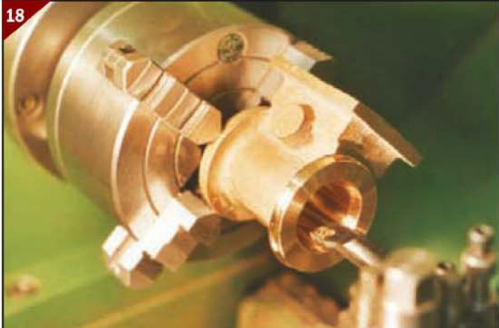
18. Boring out the cylinder. One jaw of the chuck is reversed so it can bear on the steam chest face. The other three locate on the periphery of the flange.
