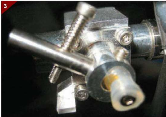
3. The carburettor of Ian's engine showing the modification to the slow running adjustment.
