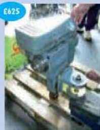
Beaver slotting head (will also fit Bridgeport)
