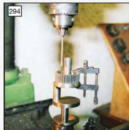
The four 5/32in. holes being reamed for the bolts, indexing on a rotary table (photo: Stan Nipper).
