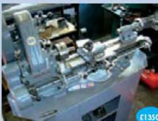
Myford ML7 lathe 3 1/2" x 19" lathe complete with clutch and stand
