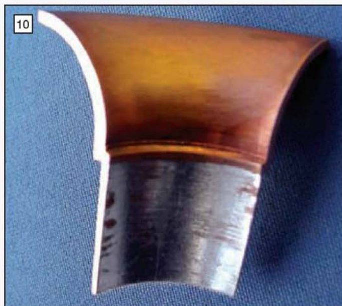
A close up view of one of the finished quadrants after tidying up with a file. The stepped in lower portion is clearly discernable.
