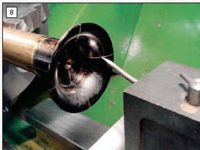
Marking the bell with quadrant lines. The surface gauge has been set to the centre height of the lathe.
