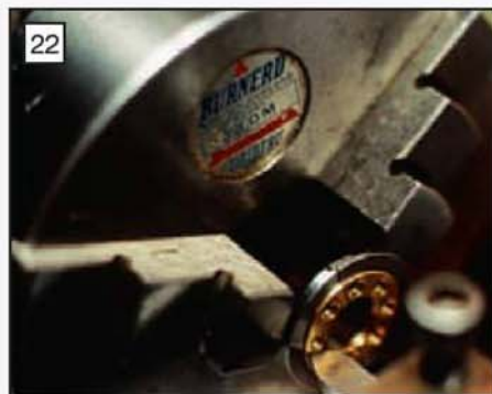
Facing the second surface of the ball retainer. Note the use of the split holding ring.
