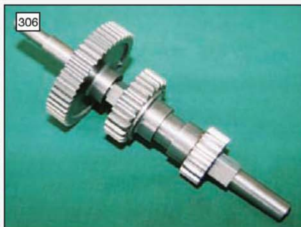
306 The completed second shaft is now ready to fit into the crankcase. Photo: Stan Nipper.
