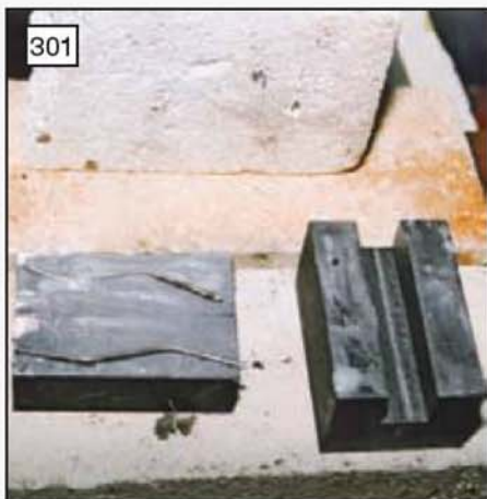
301 Silver solder and flux were added prior to heating (photo: Stan Nipper).
