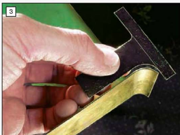
A template was made out of thin brass material carefully filed to the correct profile. It is seen here testing the radius in one of the panels.
