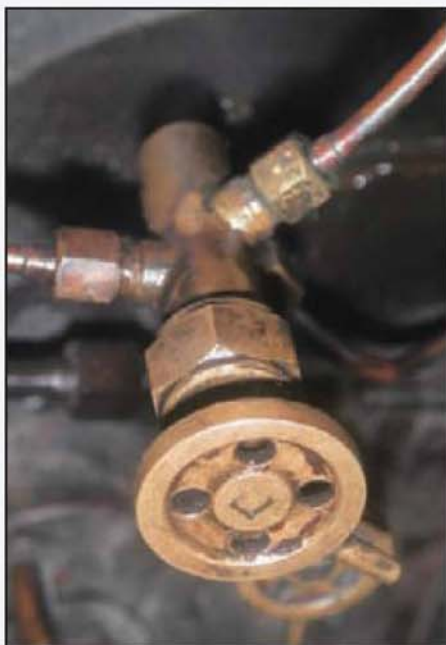
Undergoing tests for forty years, the backhead valve fitted with a dummy hand wheel.
