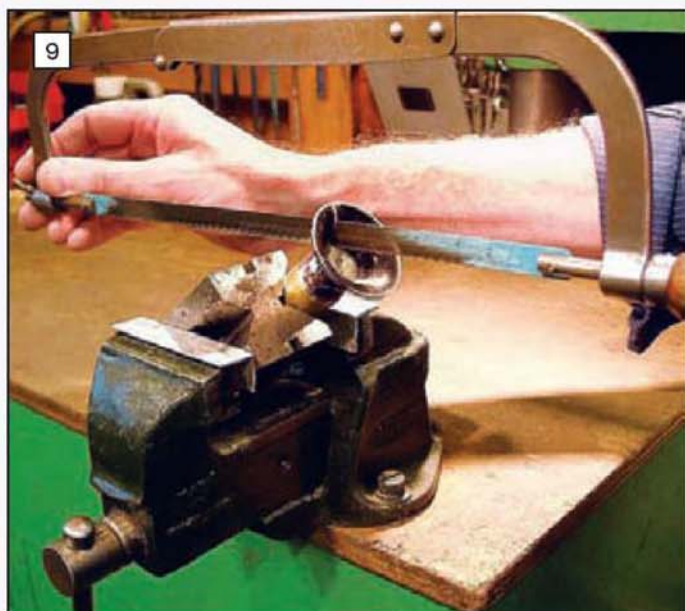
The bell provided two quadrants obtained by sawing outside the scribed lines of two opposing quadrants.
