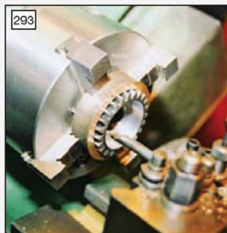
A bronze sleeve is bored to a push fit on the gear to ensure concentricity (photo: Stan Nipper).
