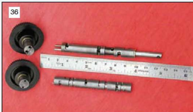
The two valve rotors of the V-6 engine shown with their drive shafts and timing belt pulleys.
