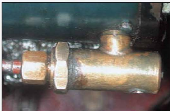
A close up view of one of the neat cylinder pressure relief valves. The author apologises for not cleaning the locomotive before taking the
