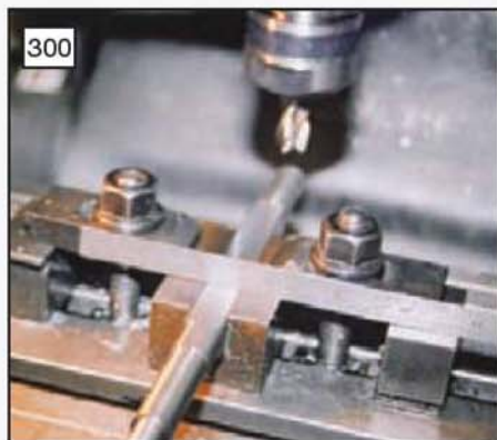
The slot in the bobbin being matched to the second shaft (photo: Stan Nipper).
