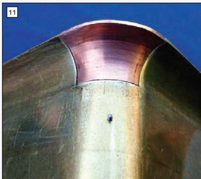
Here a quadrant has been fitted to the tender using a 12BA setscrew. Final fitting will be done using soft solder.
