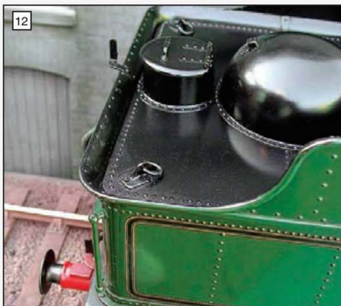
The finished tender after the rivet details and paint have been added. The tender lives with a 78xx (Manor) class locomotive.
