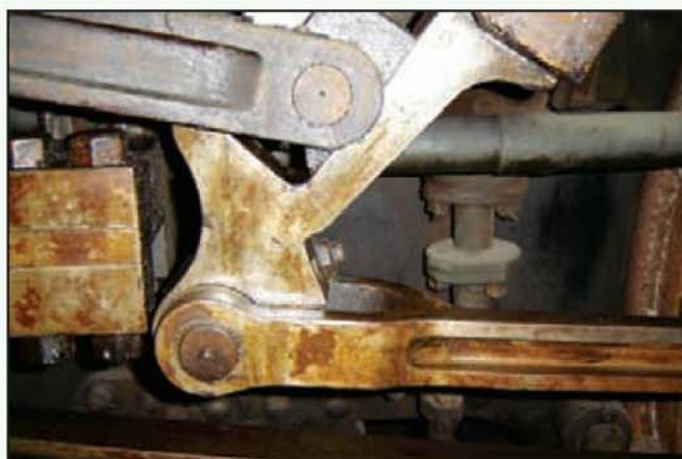
The left hand expansion link. Note the wrap around suspension bracket (photo: Derek Tulley).
