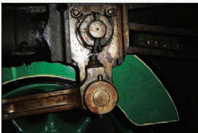
Stowe's crosshead and union link fastening. Note the use of the split pin (photo: Derek Tulley)
