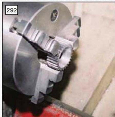
The 27 tooth wheel may be held in a 3-jaw chuck for roughing purposes (photo: J. Thomson).
