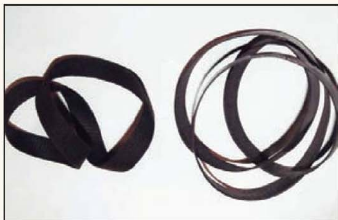
On the left can be seen an endless, woven cotton belt whilst that on the right is of plastic. Both are black in colour and 0.02in. thick x 5/8in. wide.
