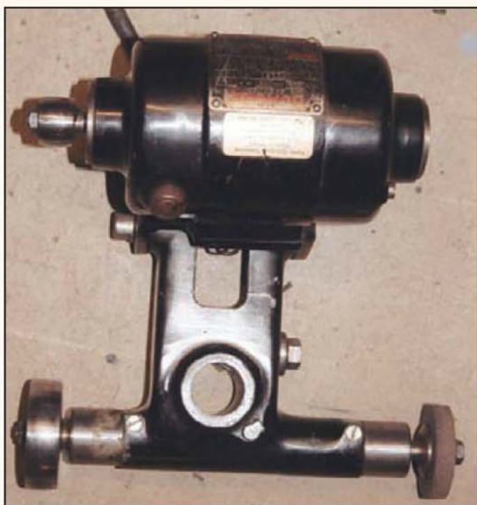
A Dumore toolpost grinder of a size suitable for 3 1/2 in. centre height lathes. The pulleys can be swapped for bore grinding operations.
