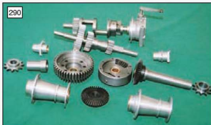
The Savage Universal Carrier gear train laid out neatly in 'exploded' form to show all the various components (photo: Stan Nipper).
