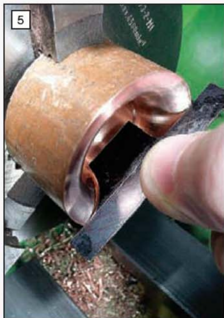
Using the template to check the radius formed in the bore of the 'bell mouth'.
