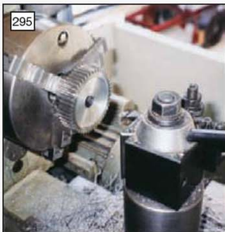
295 The 47 tooth gear is hollowed out to save weight and accept the bearing (photo: Stan Nipper).
