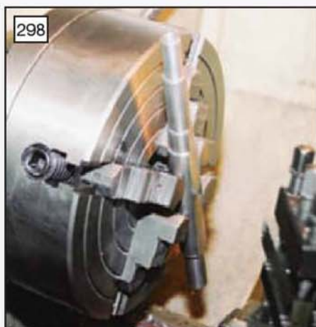
The lathe being employed to machine the square section on the second shaft (photo: Stan Nipper).
