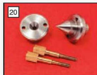
Above: The completed centres together with jacking screws.
