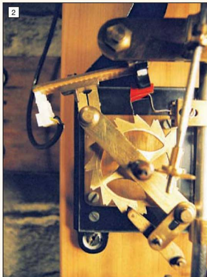
A close up view of the sensor components and the gathering pawl. Care is needed in setting up the parts to give good performance.
