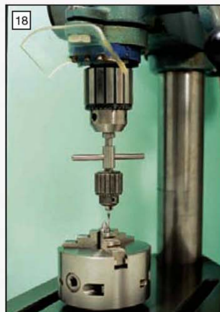
18 Tapping the 10BA jacking screw holes in one of the centres, using a guiding attachment set up in the drilling machine.
