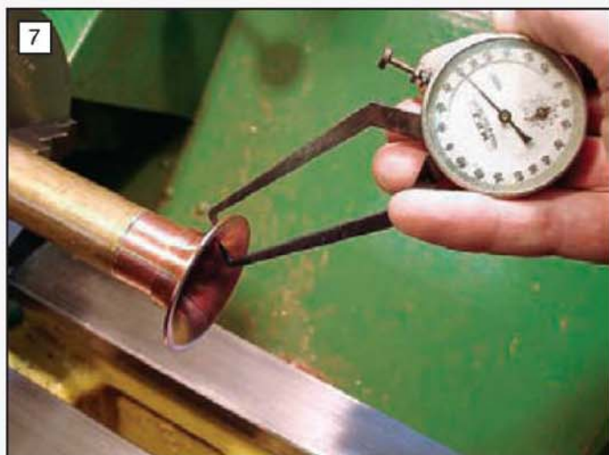
Checking the thickness of the 'bell mouth' with a suitable gauge. It was made slightly thicker than the side panels at this stage.
