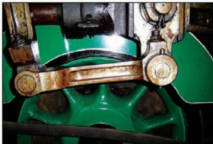
The union link fitted to the full size version of Stowe and photographed at the Bluebell Line (photo: Derek Tulley).
