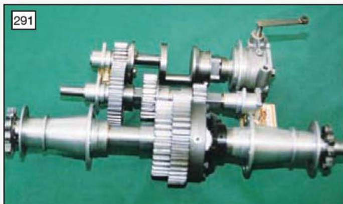
The vehicle's gear train fully assembled and all ready to be fitted into the crankcase (photo: Stan Nipper).
