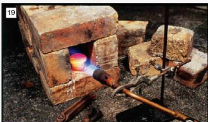
19 Improvised muffle furnace used for heat treating the centres.
