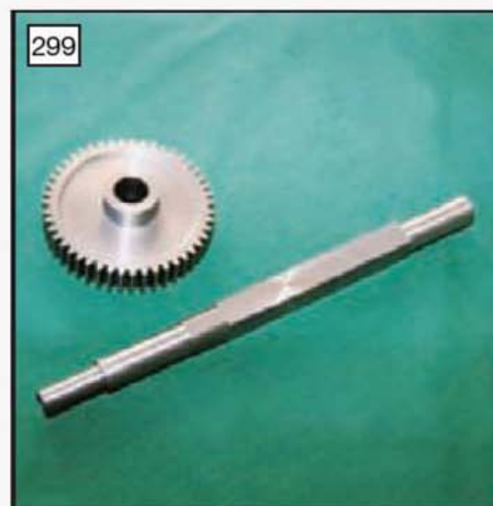
The completed second shaft and drive gear (photo: Stan Nipper).
