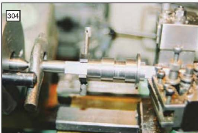
304 The gear registers were turned with the bobbin and shaft mounted between centres (photo: Stan Nipper).
