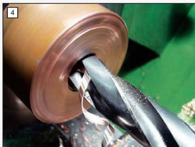
One of the first operations on the copper 'bell mouth' was to open up the bore with a suitable drill.
