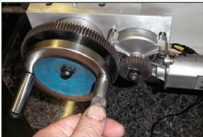
A view of the installation on the author's milling machine. The spring loaded drive plunger is being operated.
