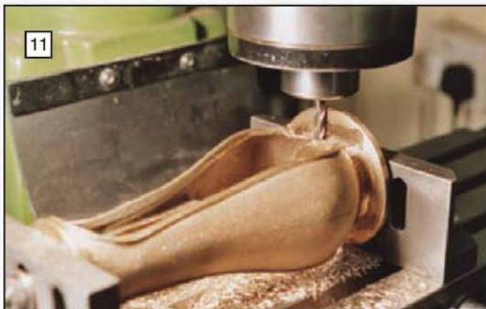
The pocket for the bearing pedestal being machined into the main frame with a 6mm end mill.
