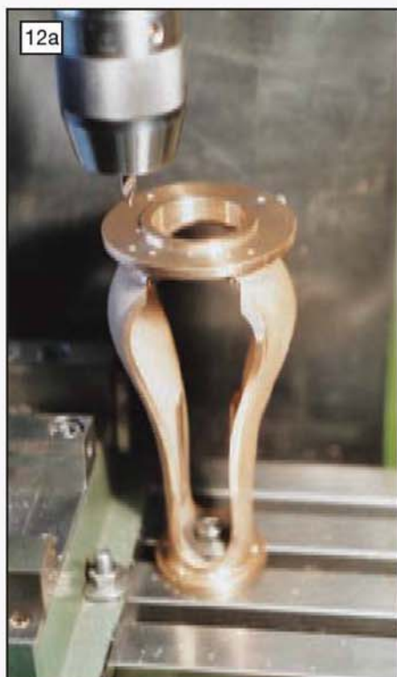
Above: Drilling the main frame base. Right top: Drilling the mounting holes for the slide bar oil cups. Right bottom: Boring the separate pedestal bearing in the lathe.
