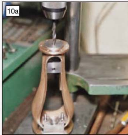
The cross head being spotted by a drill passing through the bottom cover.
