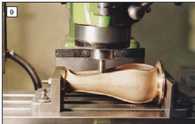
A photo showing the set up approach used when mounting the main frame on the milling machine.
