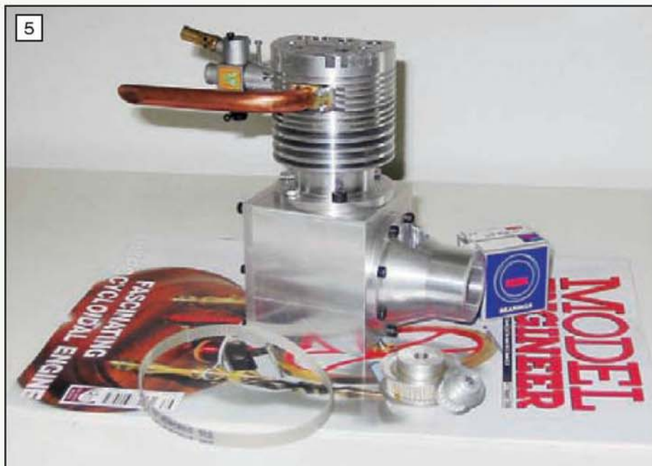
John Brown's NE15S displayed with the cam drive components.
