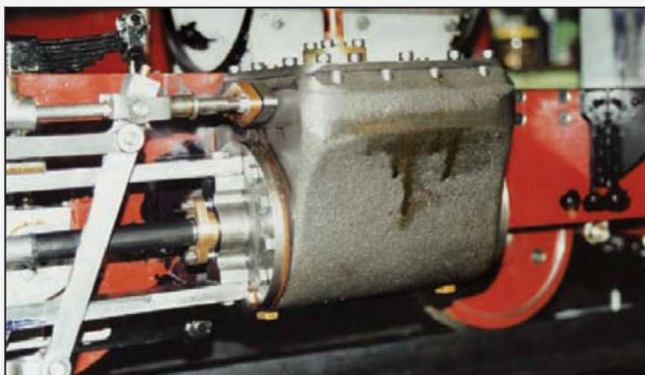
Close up of one of the large cylinders, cast by a local New Zealand foundry.
