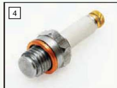
The finished spark plug showing the annular spark gap.
