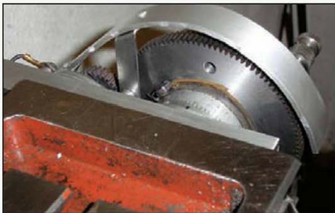
The large gear is fitted between the feed screw handle and the index dial and does not interfere with manual operation of the machine.
