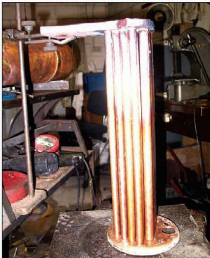
The set-up used to get the tubes into tube plate and silver-braze them without drama.
