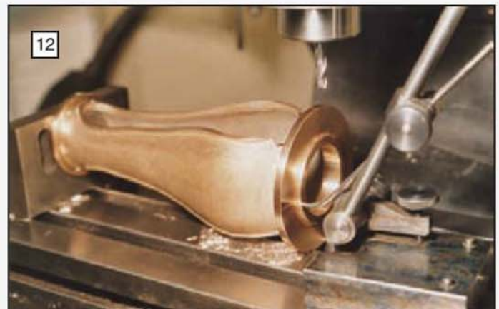
Scribing a line across the bottom of the main frame along the centre line using the surface gauge.
