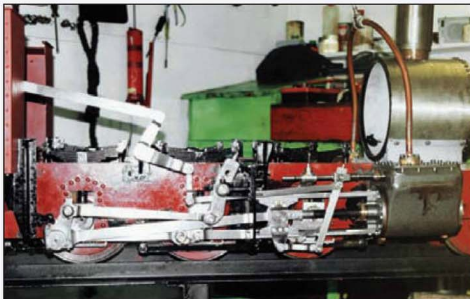
Walschaerts valve gear, just like the original.
