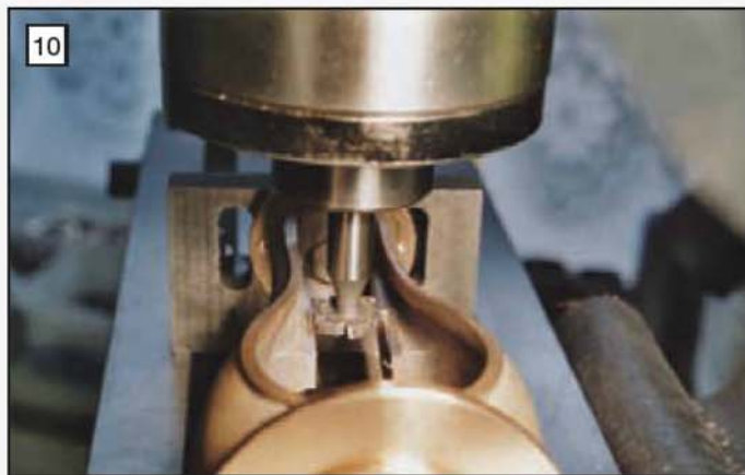
Machining the edges of the slide bars in the main frame on the milling machine using a Woodruff cutter.
