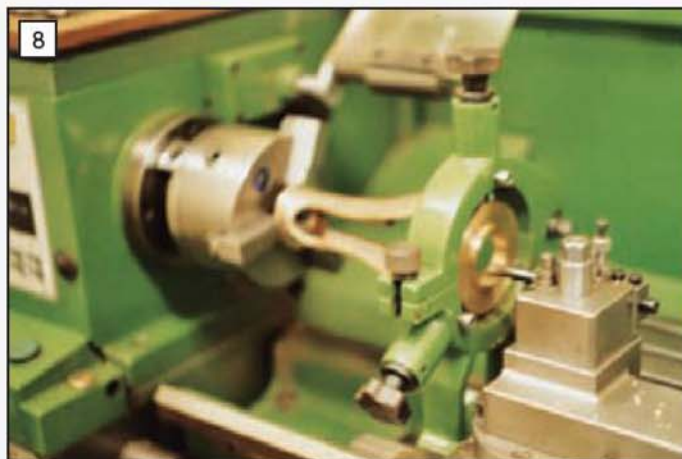
The fixed steady is brought into use again when boring the hole in the bottom flange.
