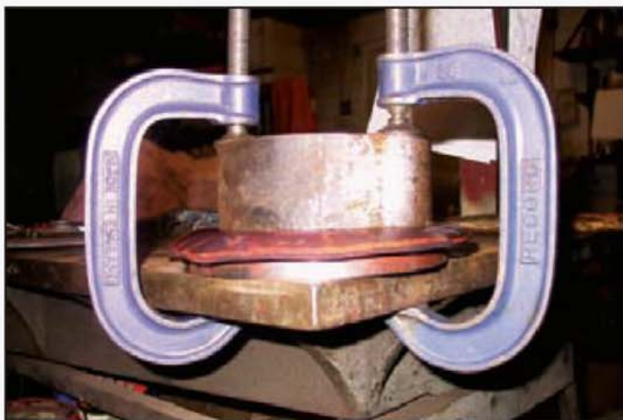
This photograph shows a plate-bashing operation under way and the set-up used to support the work.
