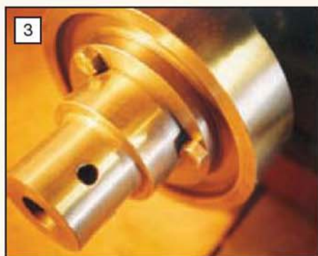
Cast iron shaft coupling and flywheel.
