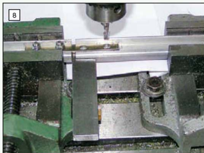
Set-up in the milling machine for cutting the fishbolt slotted holes. Note the gauge, with brass distancing pip at the right-hand side, for the outer hole.
