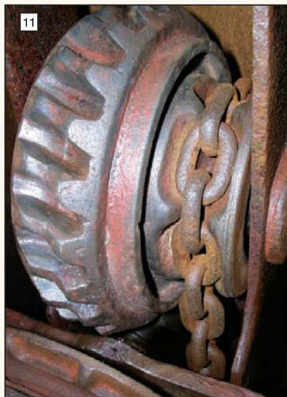
This chain is transmitting power from the worm wheel via the notched pulley.
