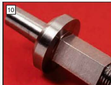
A close-up of the interface between the square part of the mainshaft and shoulder, showing the small witness left to the original round section.
