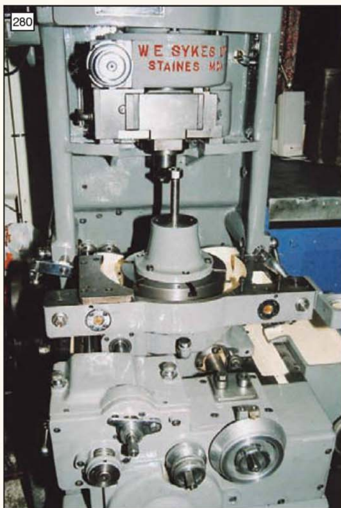
280 The Sykes V10A after major restoration. Behind the red lettering is a large worm and wheel to rotate the reciprocating cutter, a second worm and wheel beneath the table rotates the work (photo: M. Wallis).
