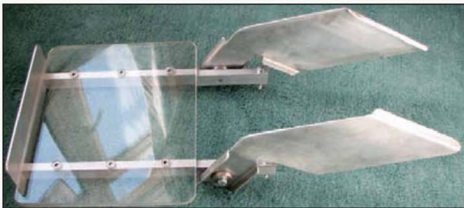
This shelf, to aid a Royal Mail sorter, was fabricated from aluminium and Perspex.
