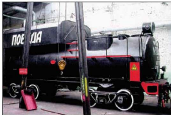
A fine job of restoration on the Vanderbilt type tender of the Russian 2-10-0.
