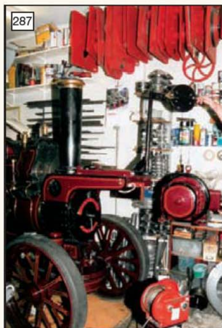
287 The dynamo is winched up into position with a special hoist.
