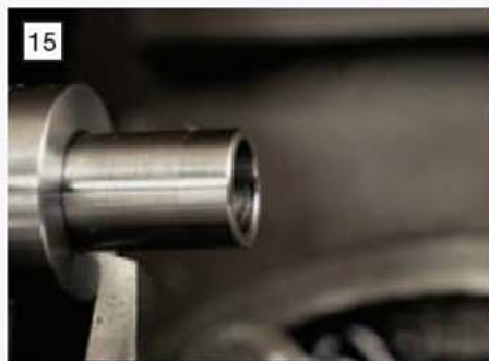
Producing the undercut on the thrust transfer sleeve, using the specially ground lathe tool.
