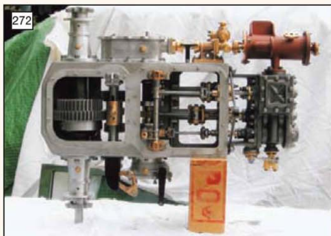
The completed engine unit less the inspection covers. The red drum (top left) is the feed water heater (photo: Roger Barnwell).
