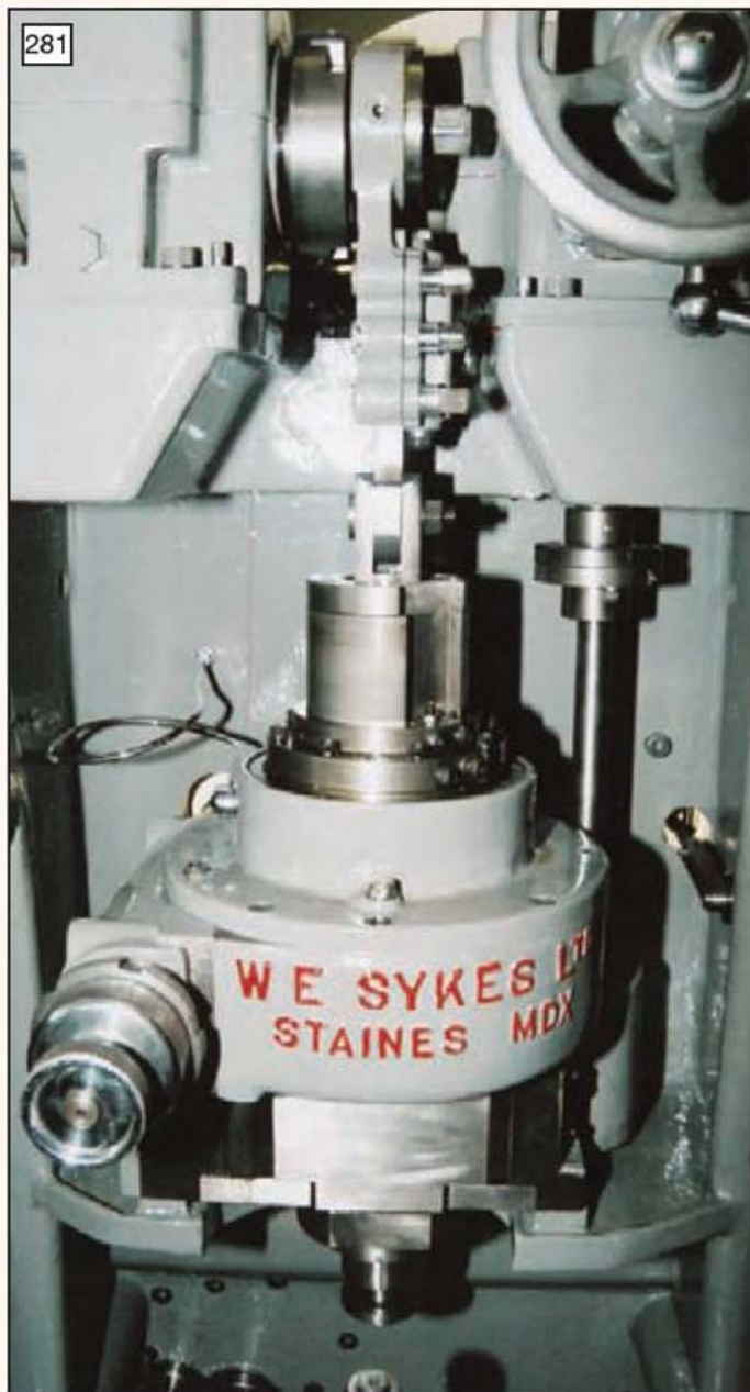
The crank and connecting rod on the rebuilt Sykes gear cutting machine (photo: M. Wallis).
