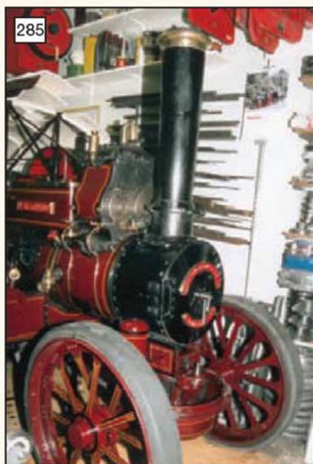
285 Road locomotive form, but five loose rivets in the smoke box have been removed.
