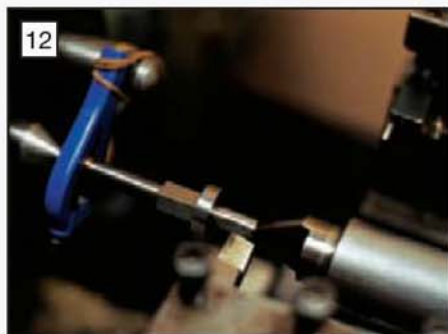
Producing the tapered portion on the mainshaft.
