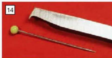
Undercutting tool, shown alongside a dressmaker's pin for size comparison.
