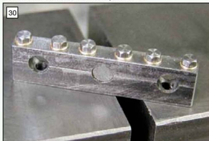
Three big ends ready and waiting for the last operation.
