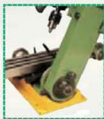
Unique spring loaded plunger to locate column in vertical position
