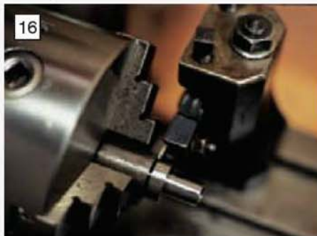
Severing the embryonic thrust transfer sleeve from the parent material. Note the use of a parting tool held in a rear tool post.
