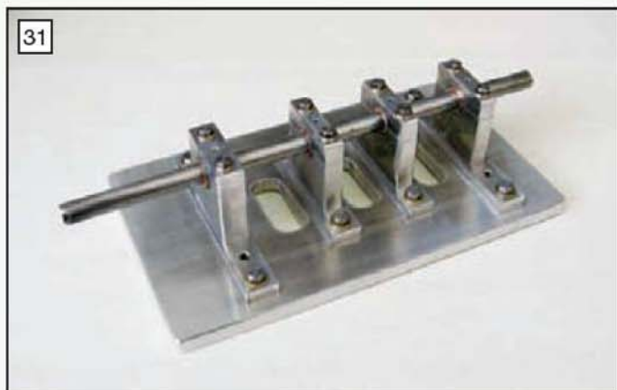
Aligning the crankshaft bearings.
