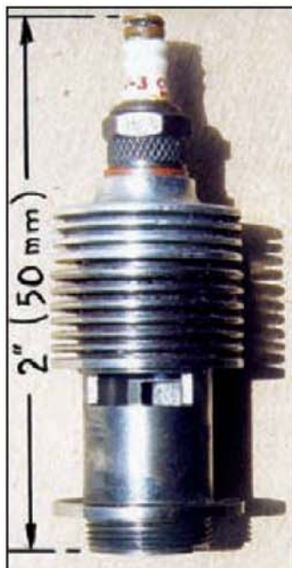
Peter Spenlove-Spenlove's 1cc 2-stroke engine cylinder and spark plug.
