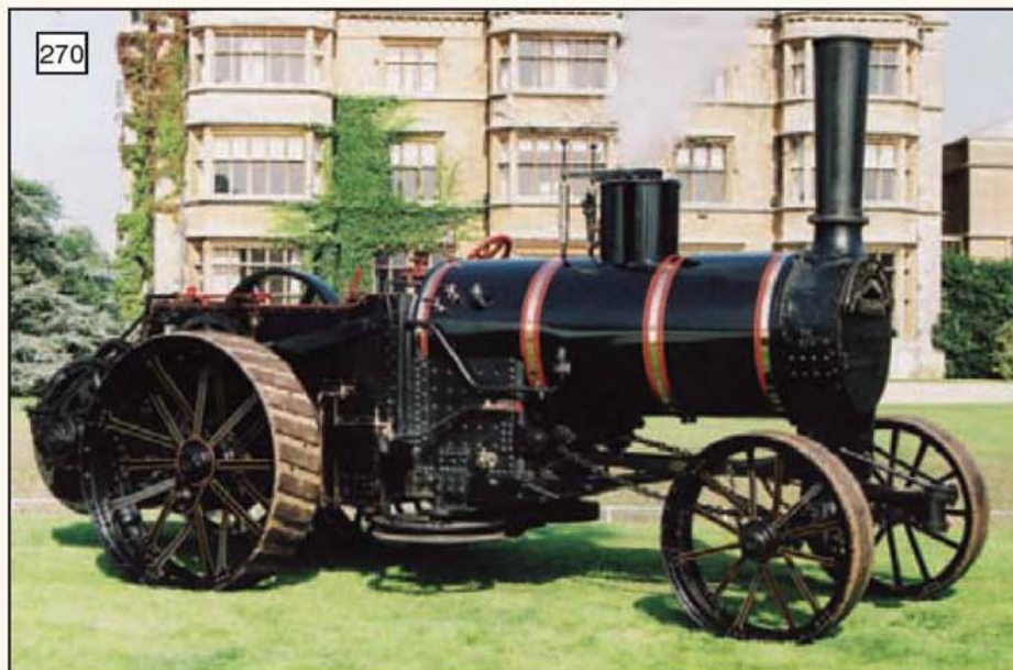
Howard Farmer's Engine No. 110 of 1876, rated at 8nhp, reg. AP 9197. Note the two pulleys under the ash pan so the cable could be payed out either to the left or the right (photo: M Wallis).
