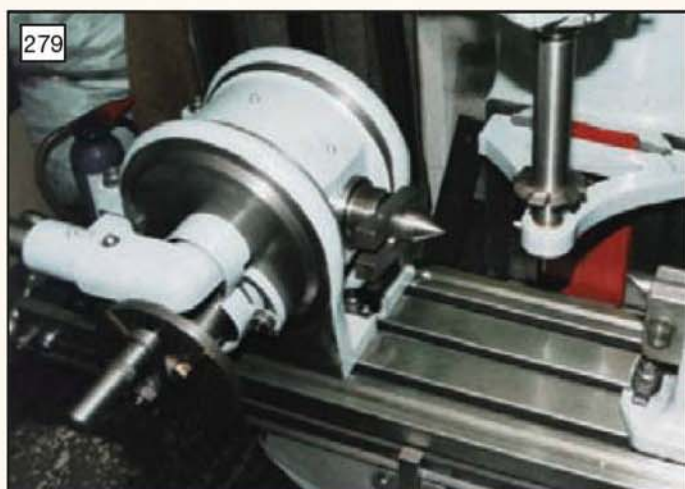
279 The gear cutting arrangements before the Sykes machine was purchased (photo: M. Wallis).
