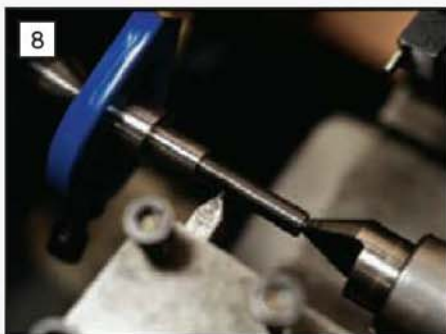
Cutting the screw thread on the mainshaft, held between centres.
