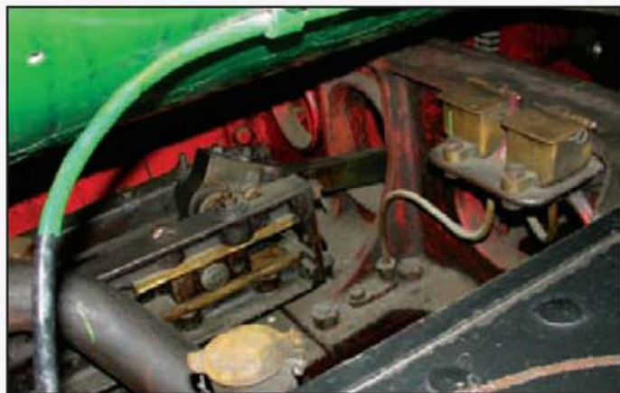
Inside valve spindle guide on a full size Schools class locomotive complete with full size oil and dirt.
