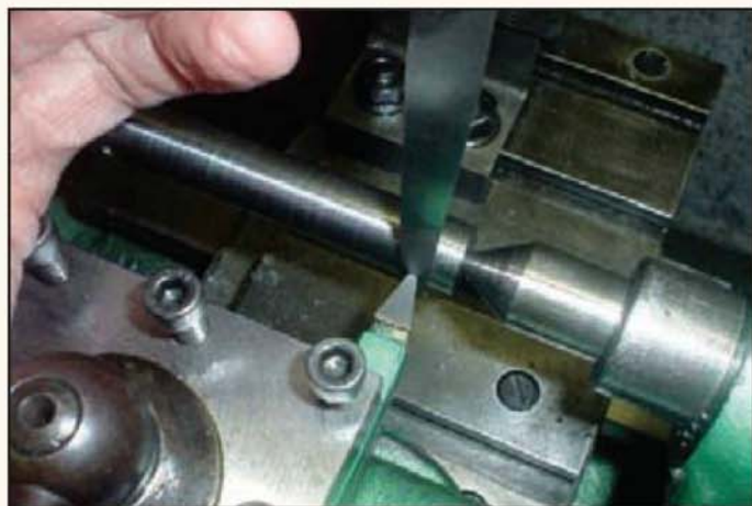
Using a feeler gauge to check the position of the test bar with reference to a round nose turning tool if no dial test gauge is available.
