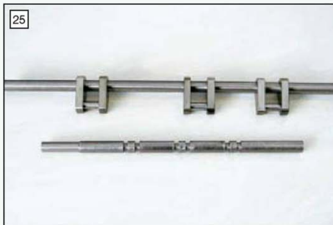
The three offset cranks have been assembled on a piece of 6mm rod.
