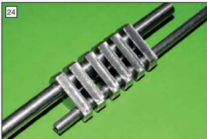
The six webs are all aligned and kept in this order until assembled
