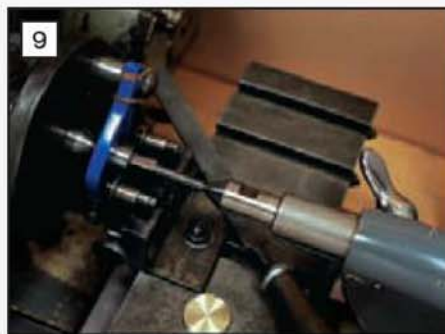
Using a file guide, set up in the lathe, as an aid to producing the square section on the mainshaft.
