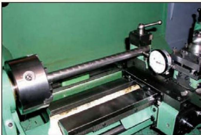
Setting up the test bar and dial test indicator to check the alignment of the tailstock with the headstock.
