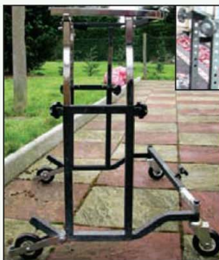
Above left: the original walking frame without any diagonal bracing. Inset pic shows the many holes that allowed the ingress of water when in the shower.
