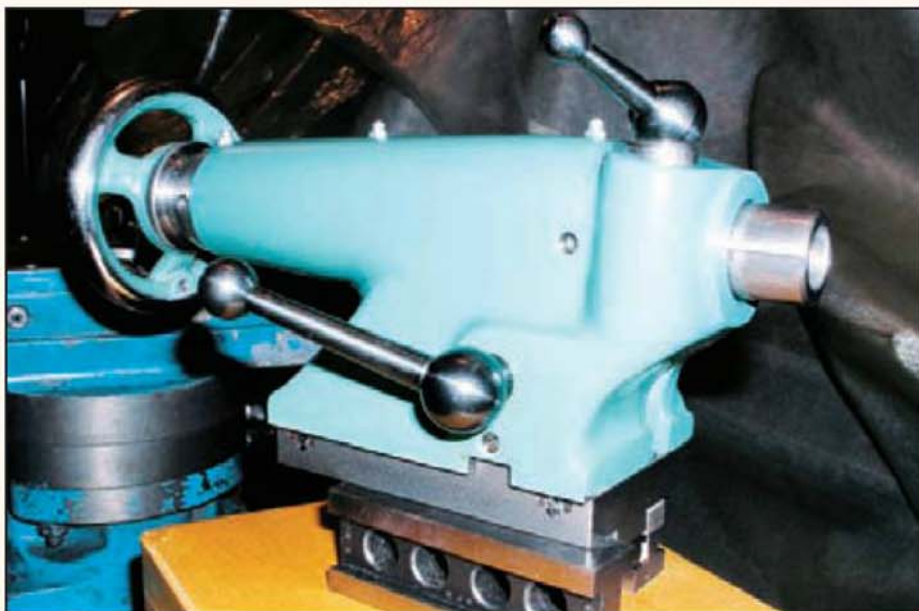
A Myford Series 7 tailstock. The gib strip adjusting screws are on the unpainted base and the rear alignment screw just below the locking lever.
