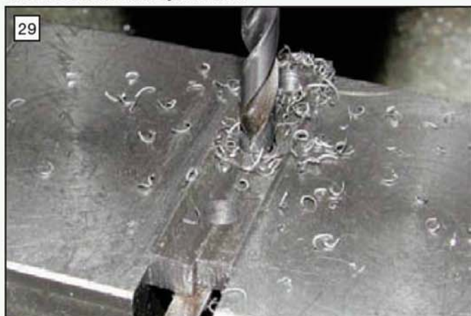
Drilling down on the joint line to make three big ends.
