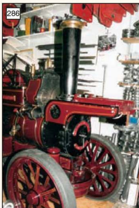
286 The dynamo bracket is fitted with five 10mm high tensile cap head Allen screws (head inside).
