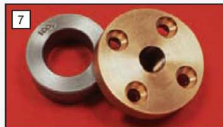
Completed feedstock nut together with the hole gauge used in its manufacture.
