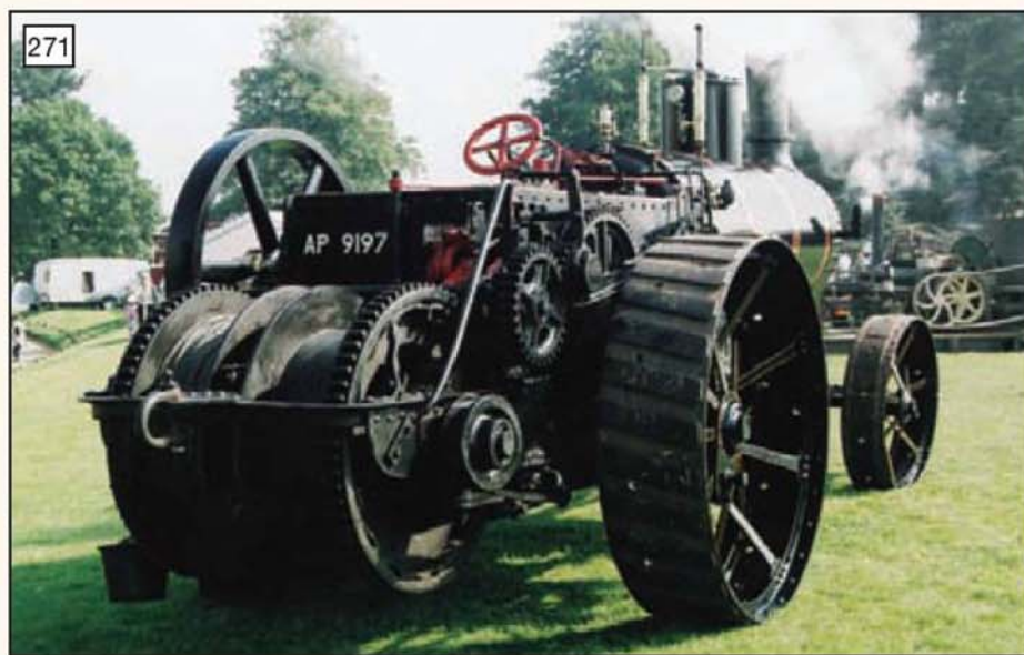
The two substantial cable drums fitted to the rear of the unusual Howard Farmer's Engine No. 110 of 1876 (photo: M Wallis).
