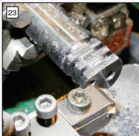
The fourth web being faced on one side prior to parting off.
