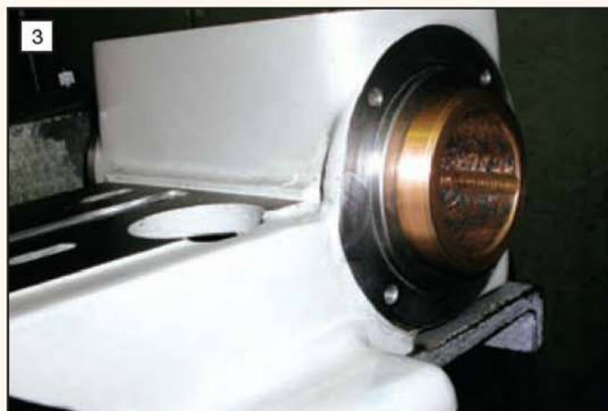
The front spindle bearing in the work head is also carefully scraped to a perfect fit on the spindle.
