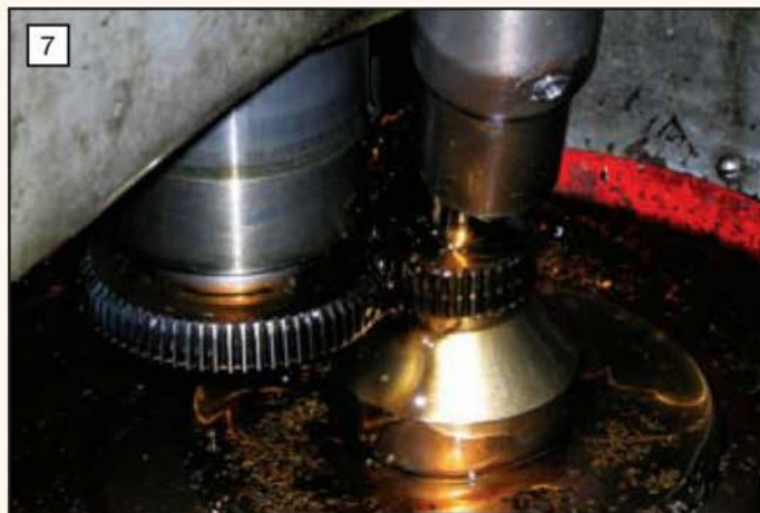
Shaping two gears simultaneously on a Drummond Maxicut machine. The 'gear' on the left is the cutting tool.
