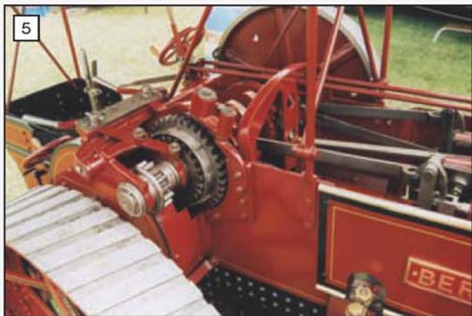
5 The Burrell three speed gearing. Note the middle speed gear slides inside the fast speed gear.
