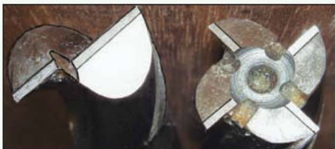
The initial slot for the T-slot is probably best made with a slot drill like that on the left. The cutter on the right is an end mill.
