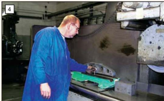
Setting up a lathe bed for grinding on the Snow grinding machine. The operator is turning the clamp screw to deflect the bed.
