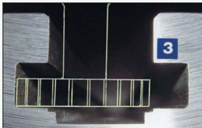
Stage three is machining the T-slot undercuts. This is shown being done with a Woodruff cutter using several passes.
