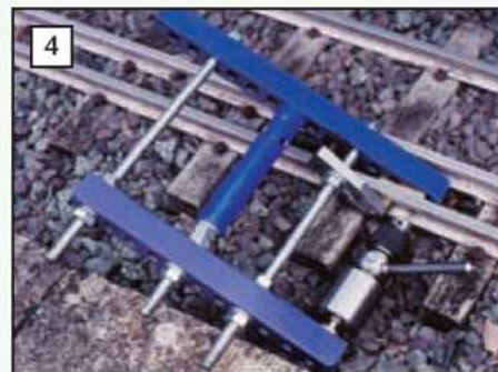
Using the brace to drill holes for track circuit connections in the author's ground level railway.
