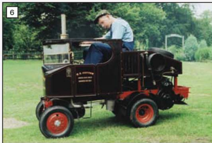
6 This 1:3 scale Sentinel seen at Bressingham is a very powerful and speedy engine. The full size was designed for timber cartage.
