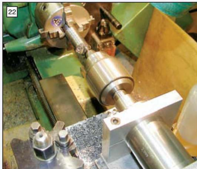
The shaft holes being drilled in the webs while they are still mounted on the bar of material.
