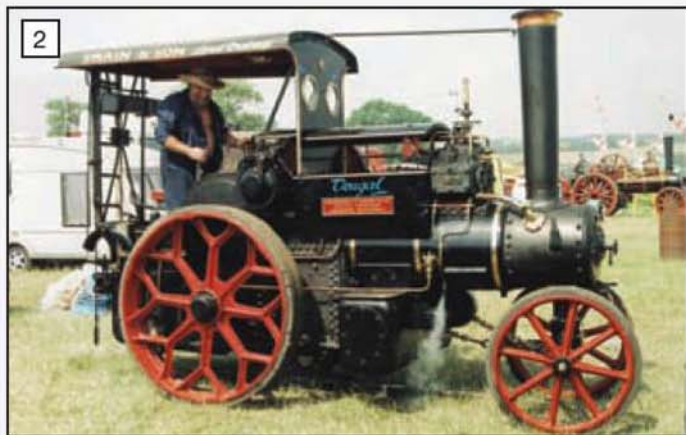
Aveling and Porter tractor No 6021 of 1906. The wheel design is that adopted by Maxitrack on their model Aveling.
