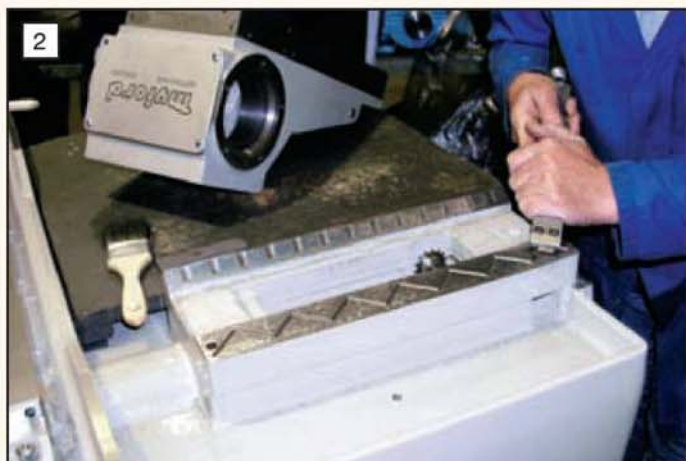
Scraping the feed-slide V-flat slide-ways on a Myford MG12 cylindrical grinding machine.
