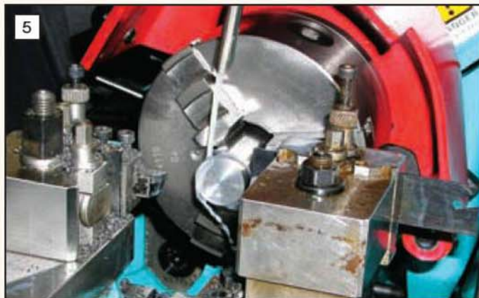
Parting off in style with a rear tool post and an Iscar tungsten carbide, throw away tip tool.
