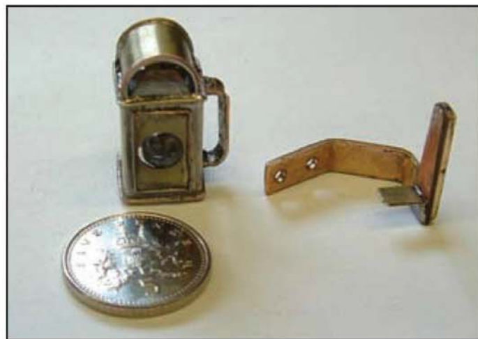
Above right: A close-up view of the working LED gauge glass lamp and bracket on Doug's locomotive.
