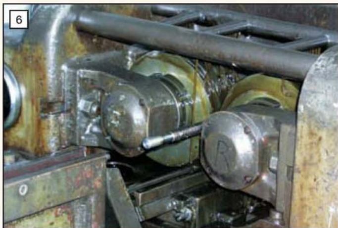
Rolling the thread on a leadscrew on a BSA thread rolling machine, a fast and accurate process.
