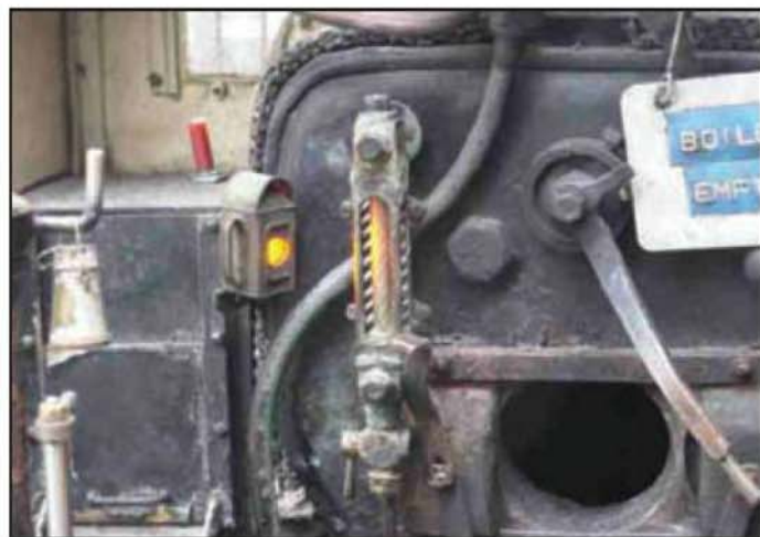
Above left: The very neat working gauge glass lamp fitted to Doug Hewson's locomotive for the recent night run by members of Lindsey Model Society.
