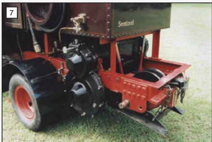
7 The powerful winch fitted to the rear of the Sentinel. It is sign written W.E. Cuttner, Union Saw Mills, Axminster on Sea.
