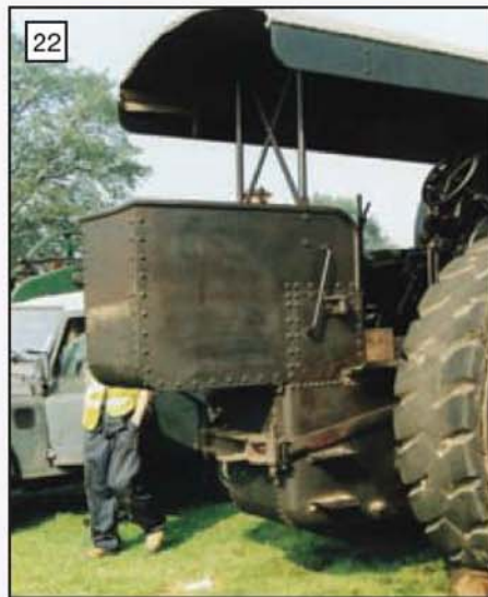
Fowler fitted an oversized bunker - routine on colonial engines.
