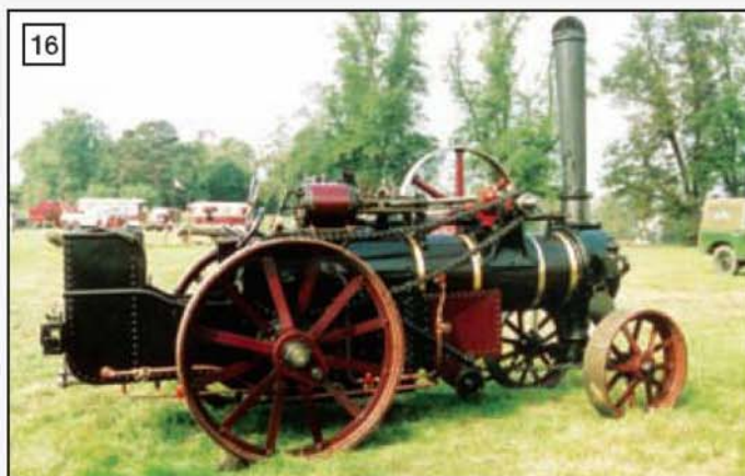
16 This 5in. to the foot scale chain drive Foster rope haulage engine was built by Brian Baker.
