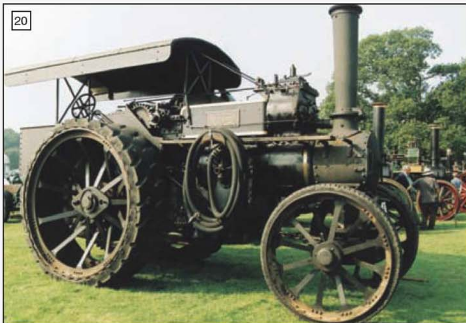
Fowler A8 No. 12754 built in 1928. Note the two brackets on the side of the smokebox, which may have carried the actuation mechanism for the elevation gear.
