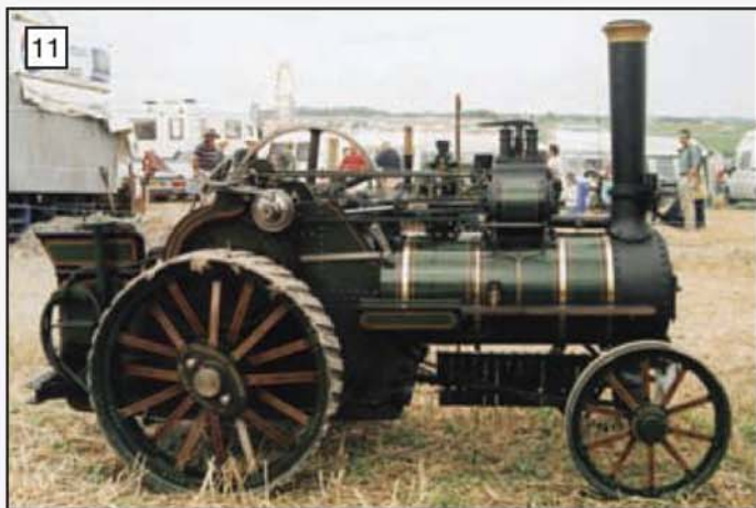
11 A fine 4in. to the foot scale Wallis and Stevens expansion engine built by Graham Hunt.
