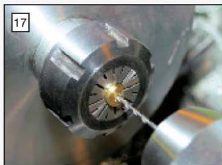
Drilling the spray bar hole in the barrel.
