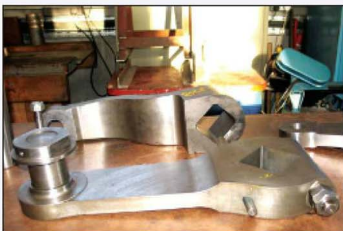
Two nicely machined and polished return cranks carefully laid out for inspection.
