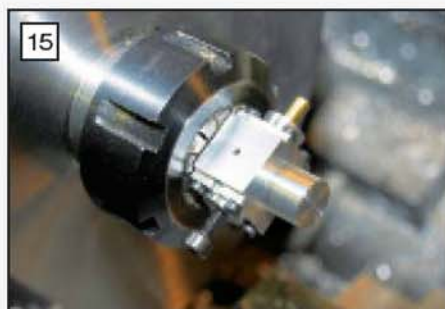
The barrel assembled and locked in the body ready for boring the carburettor air passage.
