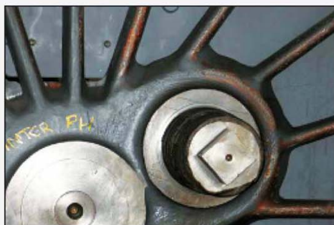
The crank pin on the drive centre shown together with some detail of the wheel casting.
