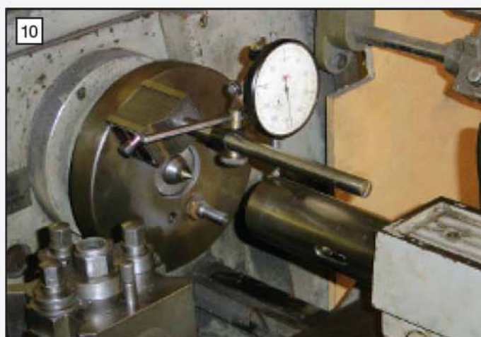
Using a dial indicator mounted on the catchplate to set the tailstock barrel in line with the mandrel.
