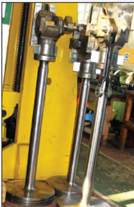
The pistons and rods for the Tornado Project. Looks as if they were turned from the solid.
