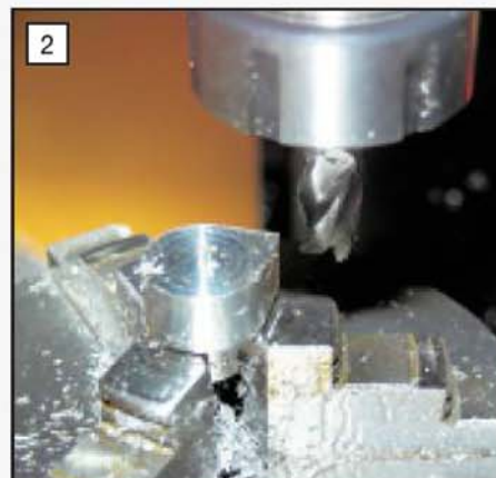
Milling the timing case outer profile.
