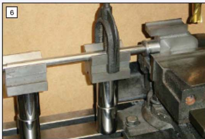
6 Machining the crosshead grooves, using the same parallels to help support the work.
