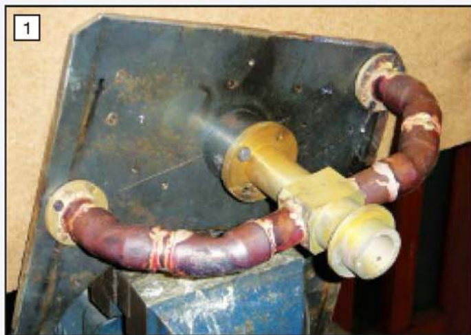
The improvised assembly fixture for the smokebox pipework made from a scrap of 6mm thick plate.
