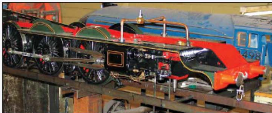
The chassis of the 7 1/2 in. gauge King stripped and undergoing overhaul after twenty-five years or so of hard work
