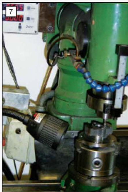
7 Rear cylinder cover set up for machining the rear surface area.
