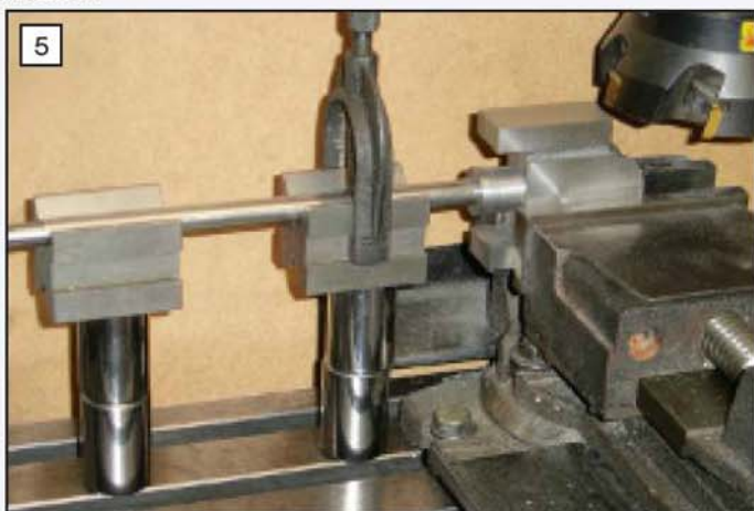
5 Machining the crosshead top and bottom surfaces. Note the parallels to fix the height.
