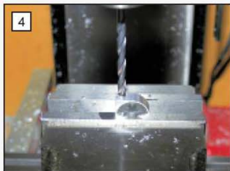
Drilling the transistor mount in the timing case.
