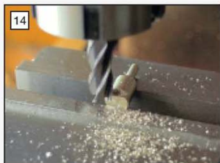
Milling the throttle stop cutaway on the barrel.
