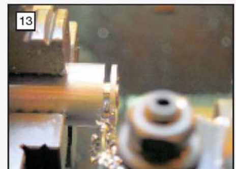
13 Turning outer spigot on end cap before parting off.
