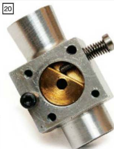
A view of the end of the barrel with the throttle turned fully clockwise against the stop in the closed position.
