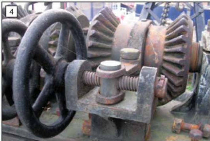
4 An example of a reversing bevel cone clutch assembly photographed on a steam jib crane.
