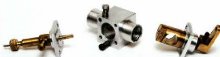
21 The carburettor broken down into the main units, left - the spray bar and end cap, centre - the body, right - the barrel and other end cap.
