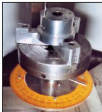
Above left: indexing device produced by Mr. Hammond. Above right: component parts of the indexing device.
