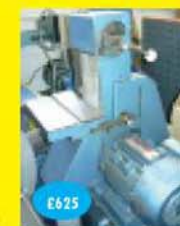
RJH 4" liner complete on dust extraction cabinet stand
