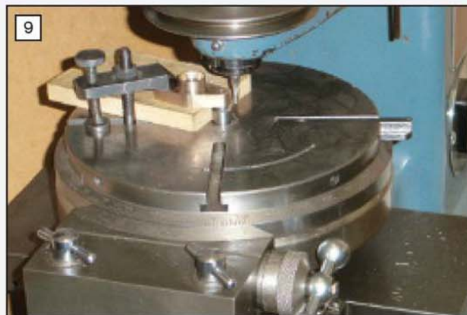
Finishing the end arcs of the piston rod glands on the BCA milling machine. Note the MDF packing under the work.
