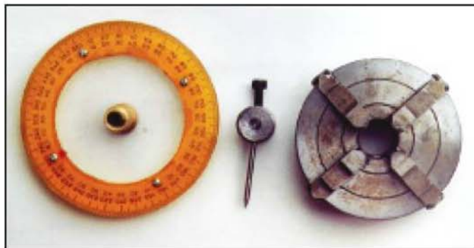
Above left: indexing device produced by Mr. Hammond. Above right: component parts of the indexing device.
