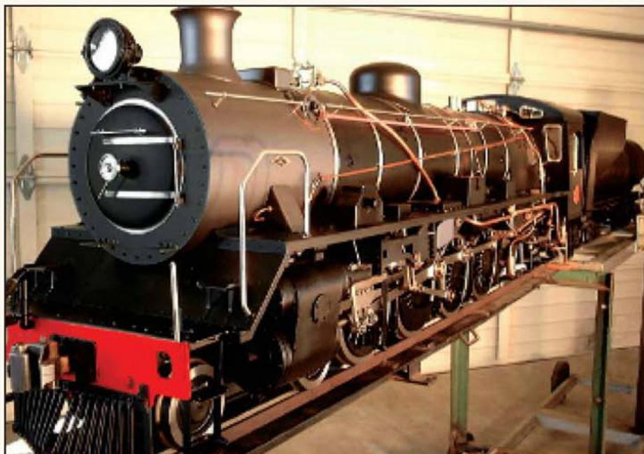
South African Class 19D 4-8-2s make an impressive and large model in 5in. gauge with a length in excess of 10ft, and taking around 4,000 hours to complete.
