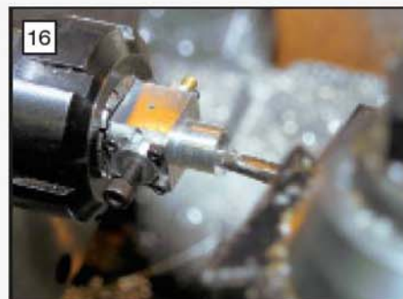
Turning the inner venturi shape.
