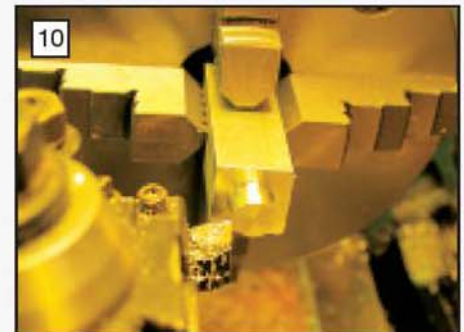
10 Turning the inlet portion of the carburettor body in the self-centring 4-jaw chuck.
