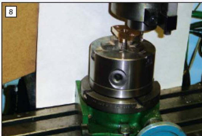
A similar set-up to that shown in photo 7 for machining the piston rod glands.
