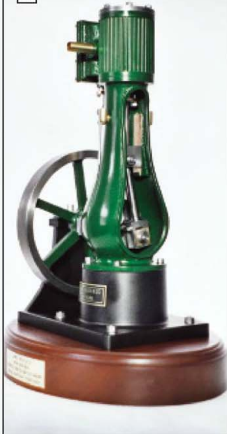
A model of the bottle frame engine with an overhung crank and the outside end of the crankshaft carried in a separate pedestal bearing.
