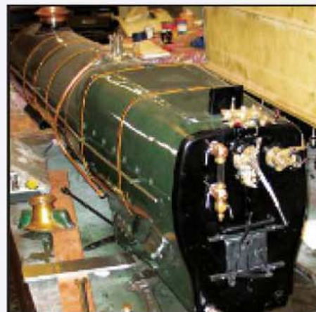
The other end of the boiler showing the neat backhead.
