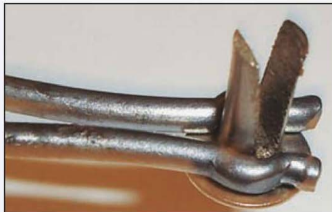
The loop of spring wire enables the rivets to be gripped firmly when it is necessary to drive them in with a hammer.
