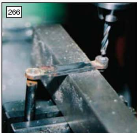
266 The reversing lever was drilled prior to reaming (photo: Stan Nipper).
