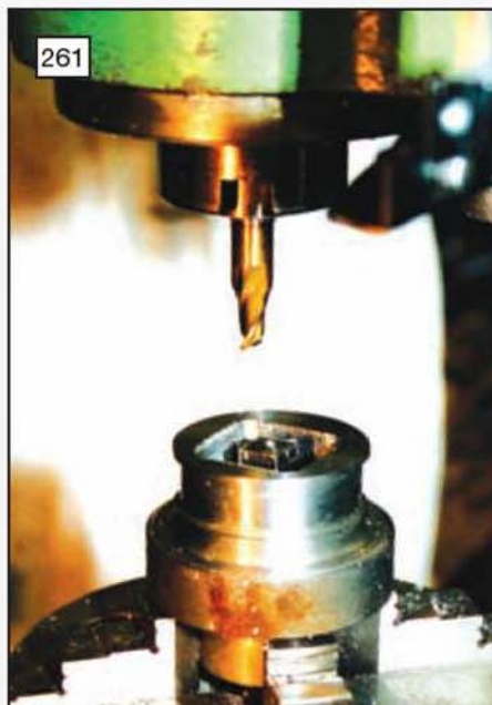
261 The square hole being milled in the eccentric (photo: Stan Nipper).
