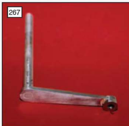
267 A completed and ready to fit reversing lever (photo: Stan Nipper).
