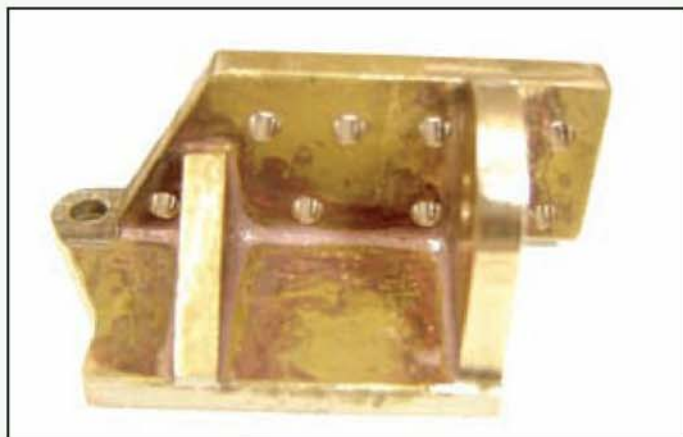
The bogie hornblock pattern.
