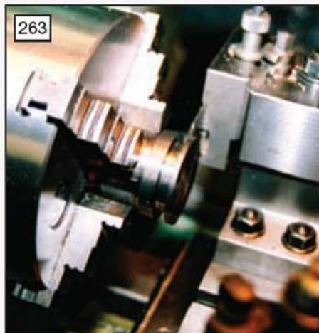
263 A rear parting off tool was used to put the groove in the reversing bobbin (photo: Stan Nipper).
