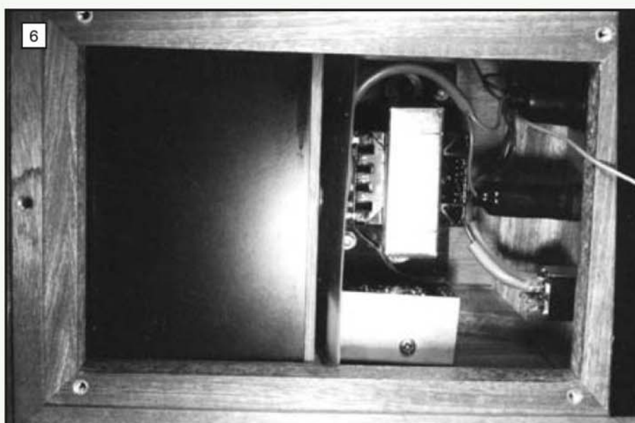
Underside of one of the clock's cabinet. The power unit is to the right whilst the spare drawer fits in the left hand side of the cavity.
