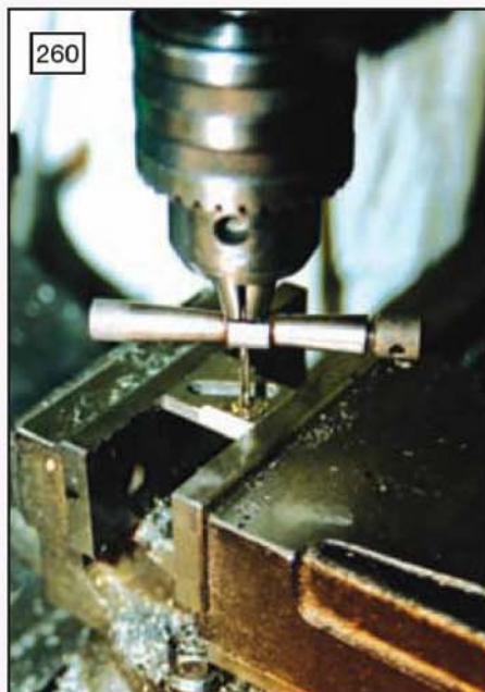
260 The retaining hole on the slipper being threaded (photo: Stan Nipper).
