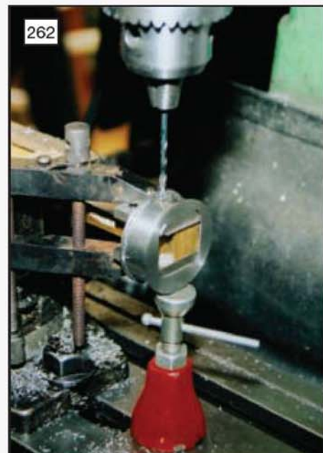
262 The fixing hole being drilled in the eccentric and through into the slipper (photo: Stan Nipper).
