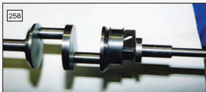
The pin, now hidden at the other end of the slot, has moved the eccentric from forward gear to full backwards (photo: Stan Nipper).
