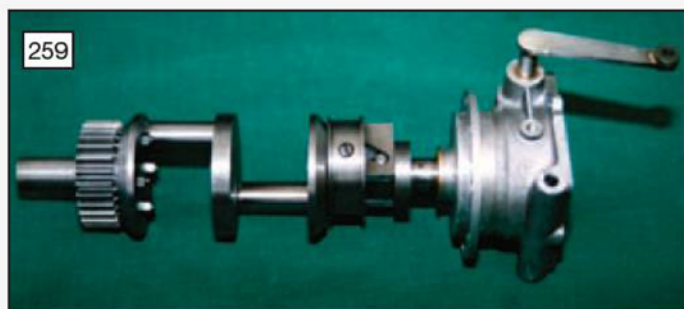
The right hand bearing housing with the sliding eccentric operating gear (see end view in photo 269) on the crankshaft (photo: Stan Nipper).
