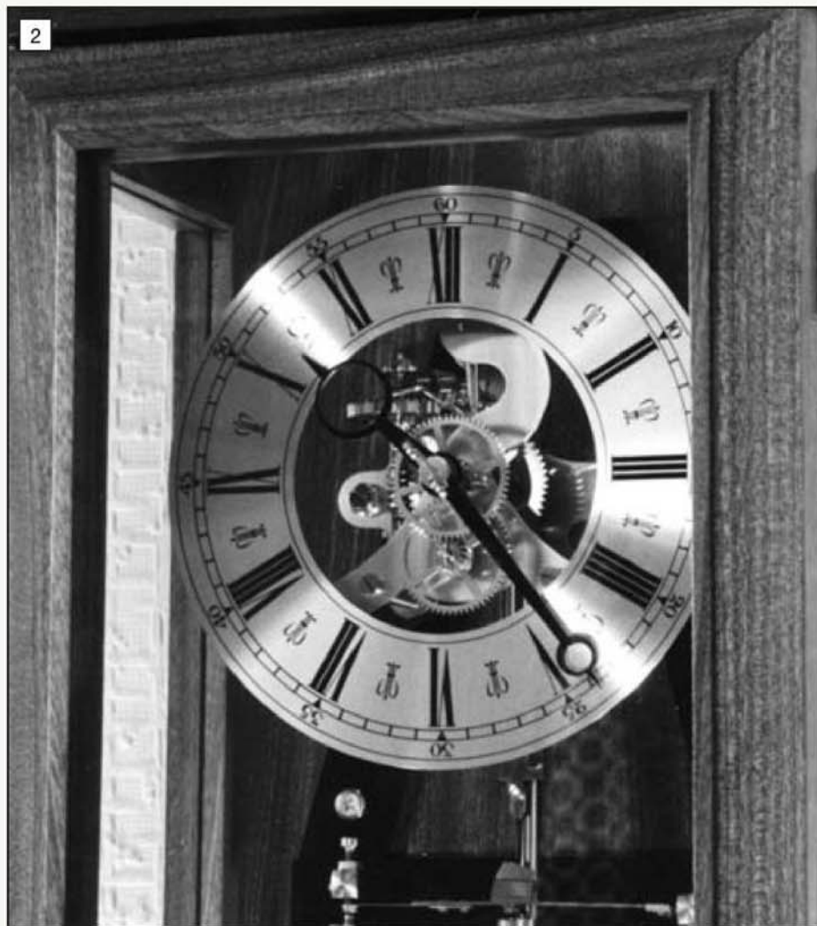
2 View of the face of one of the clocks and showing, in the lower part of the picture, the specially made trigger blade and contact strip.
