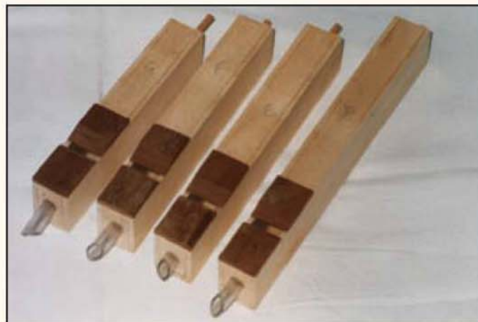
Selection of wooden pipes. the choice of material is not critical and hardwood, softwood or MDF can be used.
