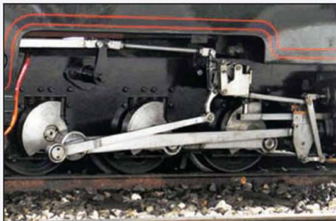
The Baker valve gear on one of the Evesham Vale Light Railway locomotives.
