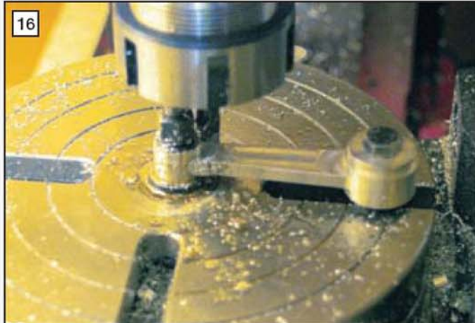
Finishing the small end of the connecting rod.
