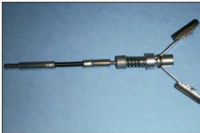
The inexpensive honing device used to finish the bore of the cylinder to a fine finish.
