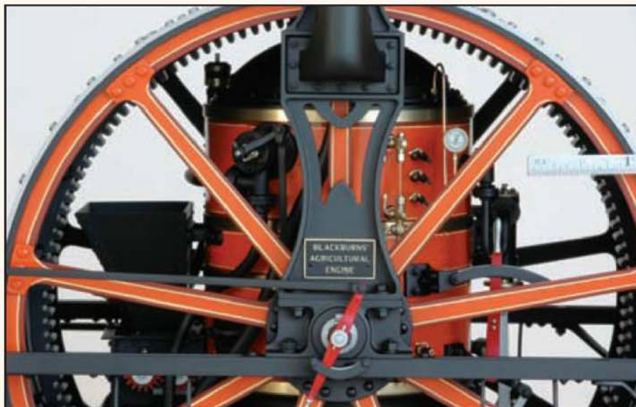
Large internal drum gear in place.
