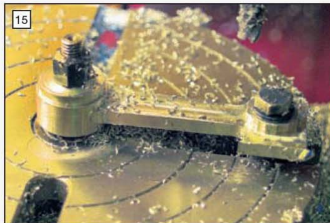
The front and rear faces of the connecting rod milled to size.
