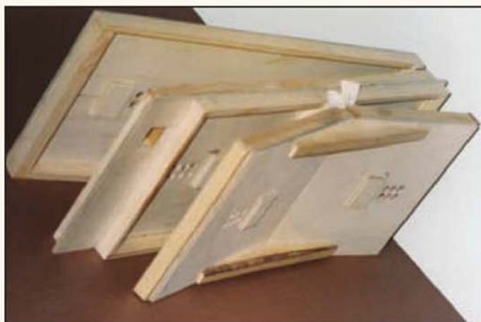
The bellows and reservoir frame before fitting with material. Black out material was used to cover the frame rather than traditional leather.
