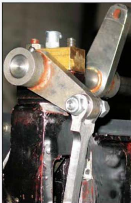
A view of the expansion link bracket complete with modifications.
