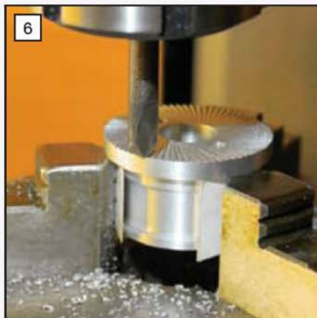
Cutting the propeller driver face grooves.
