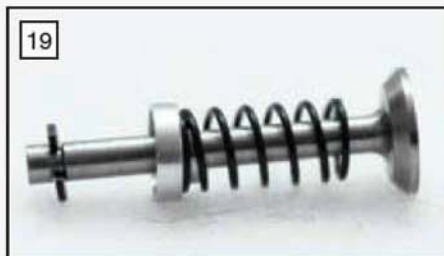
Valve, spring, cap and e-clip assembled.
