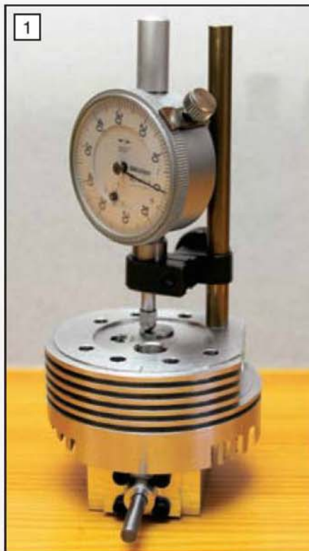
Using a dial gauge to measure the surplus valve stem length.
