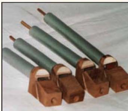
As an alternative metal pipes can be used. These were made from copper tube.
