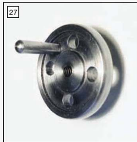
The hand wheel is turned from 7/8in. dia. mild steel bar.
