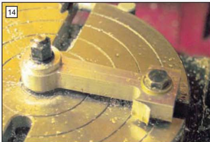
Milling the outside edges of the connecting rod.
