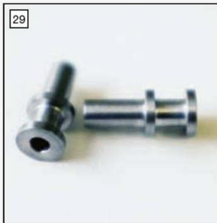
Jockey pulley spacers are a simple turning job in mild steel.
