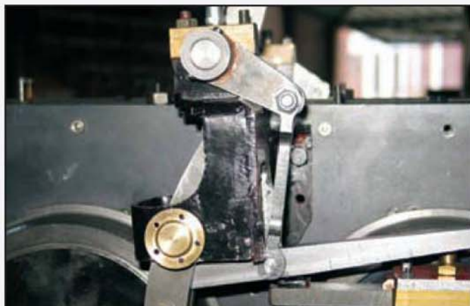
The modified expansion link bracket shown with the guide bar, cross-head and other parts.
