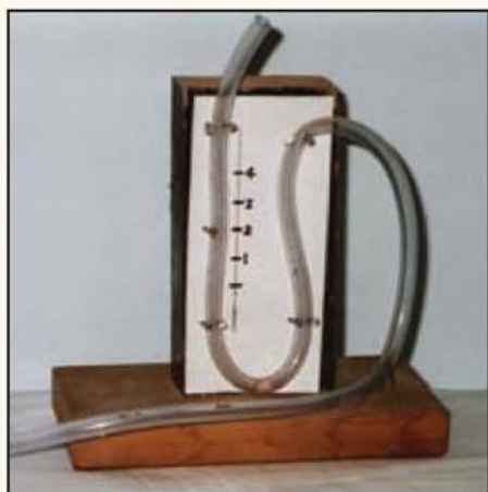
Gauge for the bellows test. Scale is marked at 1/2in. intervals for each inch of water pressure.
