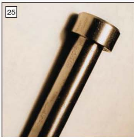
The pulley spigot needs to be machined to a good standard of finish.
