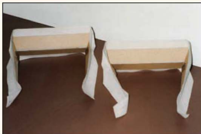
Bellows material shown with its cardboard reinforcement prior to being fitted to the wooden frame.
