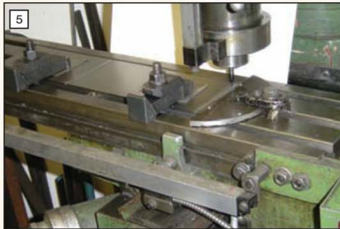
5 Cutting grooves in the sandbox using a ball nosed cutter. A scrap of steel plate keeps the job flat on the table.
