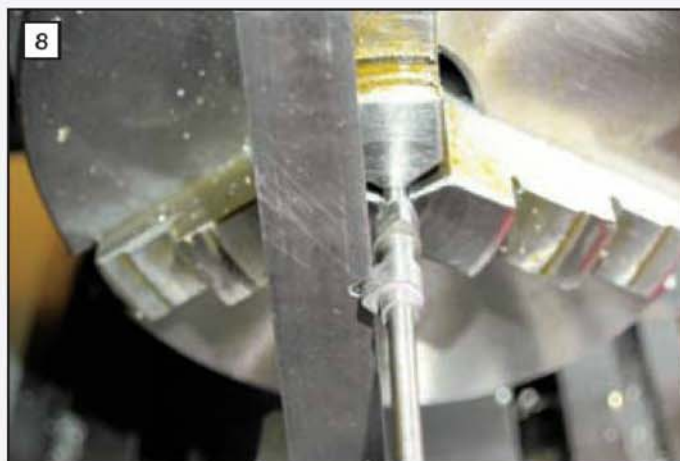
8 Setting the exhaust cam in position using the simple jig and rotary table.
