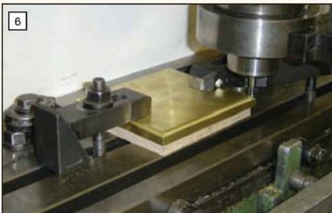
6 After 'running round' the job, the stops have been fitted to the table. Note the MDF pad for security and protection.
