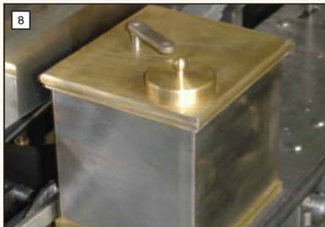
One of the sandboxes in position, shewing the brass beading sweated into place.
