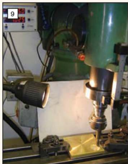
The hole for the filler cap is shown being bored in the top of the sander.
