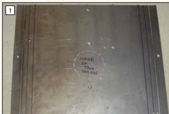
Laser cut tank sheet with 0.020in. deep grooves for bending and guide lines marked for rolling.
