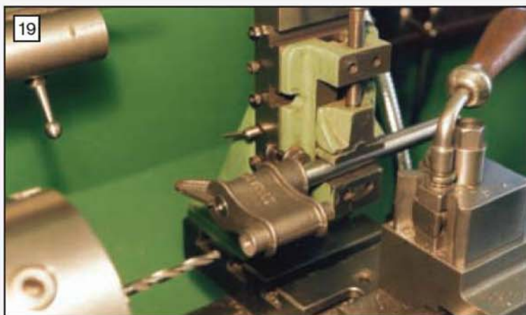
The set-up used for drilling the hole for the spindle in the drill head casting. The casting is located on an expanding mandrel held in a vice.
