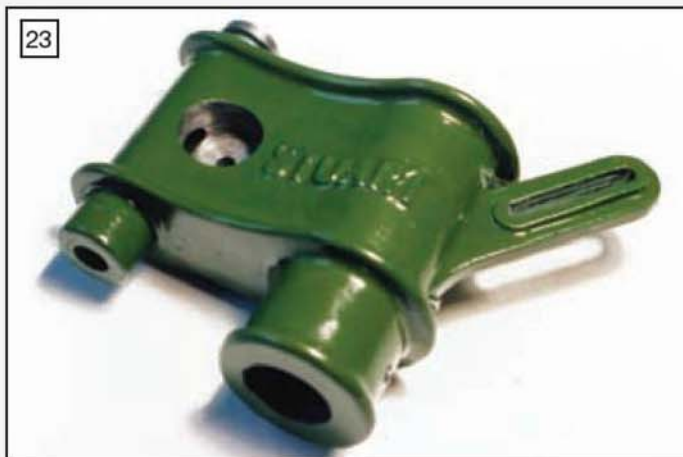
23 The finished drill head casting after painting. This is possibly the most demanding part required for the model.
