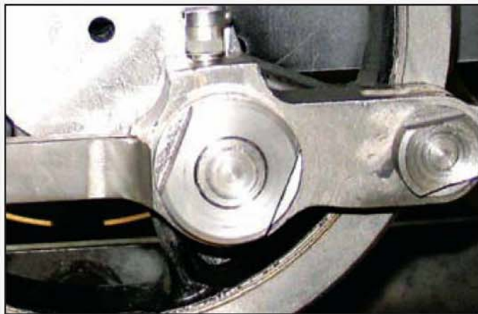
The fork-joint pivot and C-nut assembly on the centre wheels.
