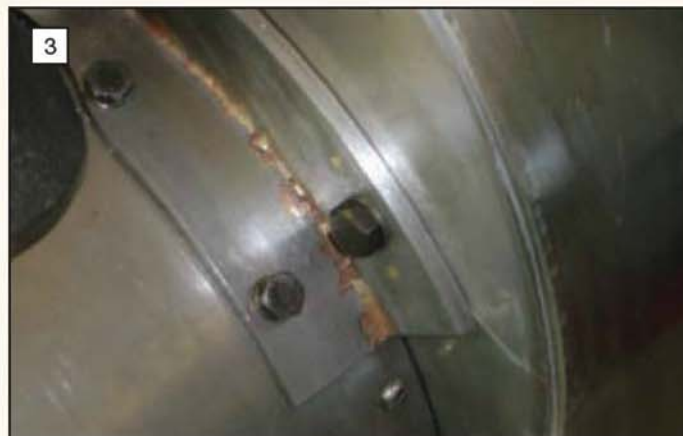
Close-up of 2mm thick end panel stuck onto the tank end. Note also the fabricated 'rolled angle iron' joining the tank to the smokebox. Screws inside the tank are capped with dome headed nuts and fibre washers.
