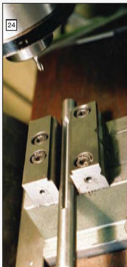
24 Machining the rack slot in the column using the vertical milling machine.
