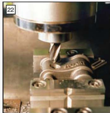
22 Machining the counter bore for the lever handle spindle with an end mill.
