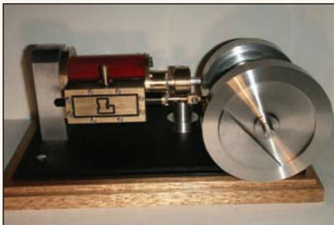
View of the engine from the flywheel side showing its embellished valve chest cover.
