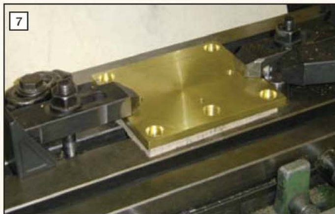
7 Drilling operations following milling the small locating grooves. All components register against the stops.
