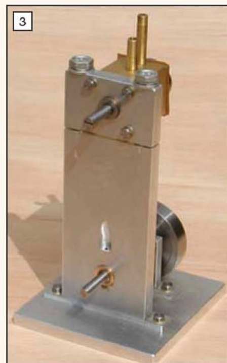
A variable height front frame was made by cutting the original one in two.
