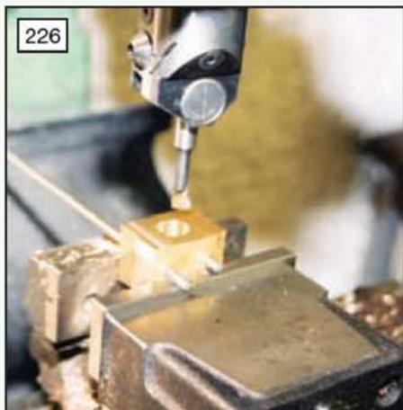
The bearing journal being bored. Note the silver steel location dowels (photo: Stan Nipper).
