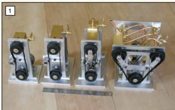
The family of overhead valve engines that form the subject matter of this series.
