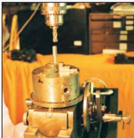
Cutting the flutes in the specially made, left hand thread tap.
