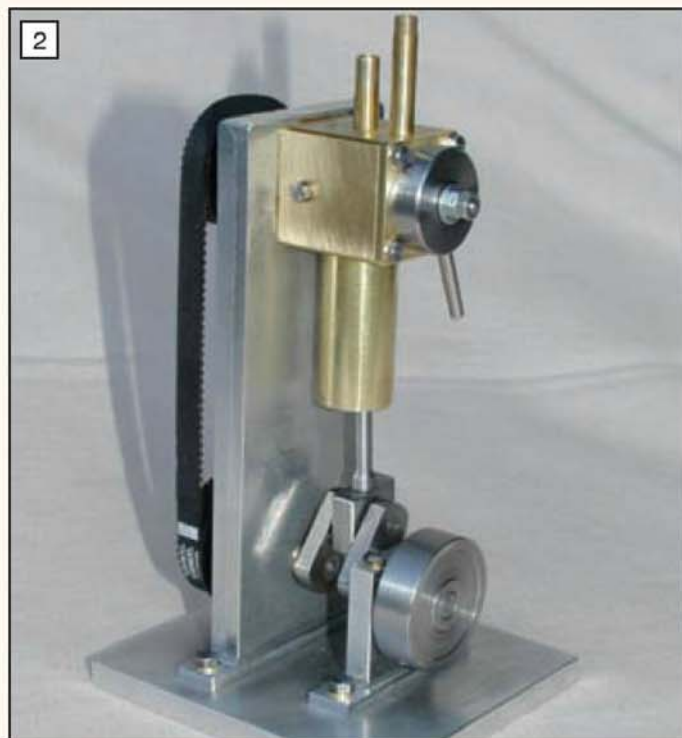
The neat little step 1 engine began the author's design quest. Note the toothed timing belt and pulleys.
