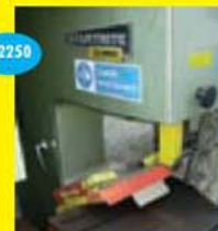
Startrite 20 RWH (hydraulic) vertical metal cutting bandsaw
