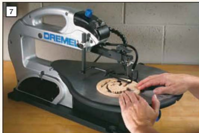
The saw in use with the work clamp holding the work down to the table.
