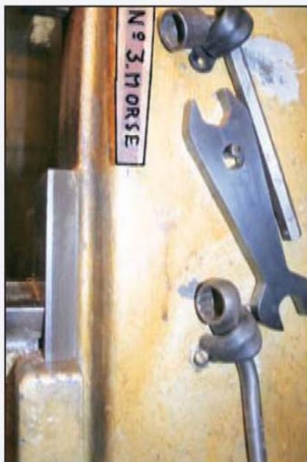
The spanner storage devices fitted to the author's vertical milling machine.
