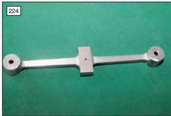
224 The completed pair of rods before being separated into two (photo: Stan Nipper).
