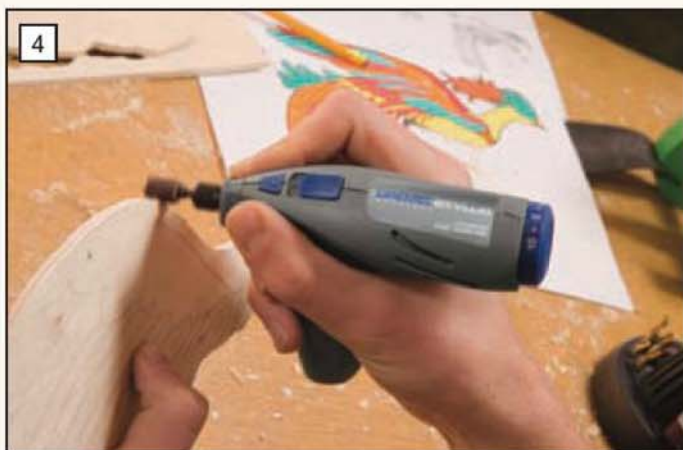
The Stylus in use with a sanding drum showing the good grip afforded by the design.
