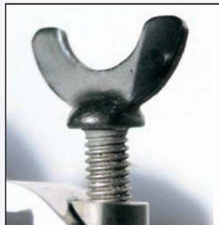
An improvised wing headed screw made by fabrication methods.
