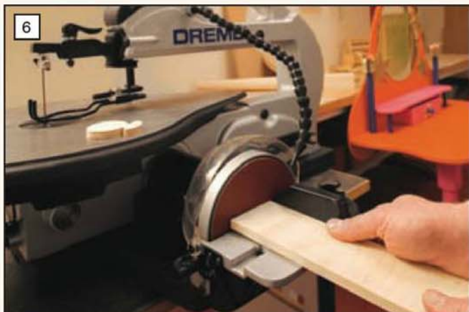
The disc sander in use showing the adjustable guide fence and table.
