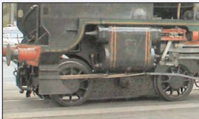
A close up view of the bogie assembly on Repton.
