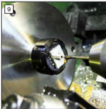
Reaming the 4mm camshaft hole in the housing.
