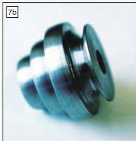
The finished pulley. Note the crowned peripheries of the pulley steps.
