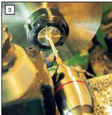
3 Turning the valve stem with the stem end supported with a live centre.
