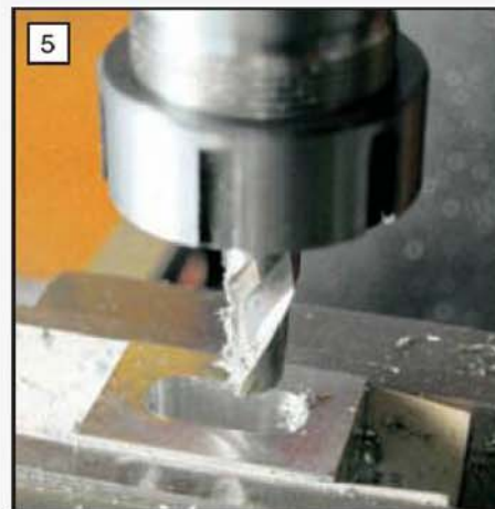
5 Using a 10mm slot drill to remove the waste metal when milling the cam box cavity.
