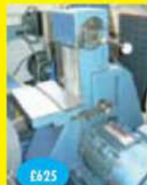
RJH 4" finisher complete on dust extraction cabinet stand
