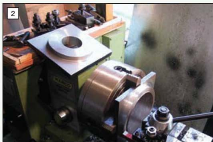
Machining the table. The finished base is resting on the headstock. The relatively high bottom speed of the lathe meant frequent tool sharpening.
