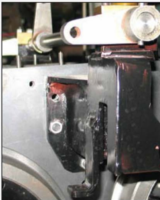
The lifting lever and weigh shaft. Note the L-shaped guide bar bracket at the bottom.
