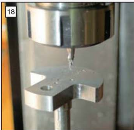
Drilling holes for the securing screws in crankshaft.
