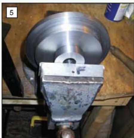
The method used to fit the pivot to the table. It was a nice press fit.
