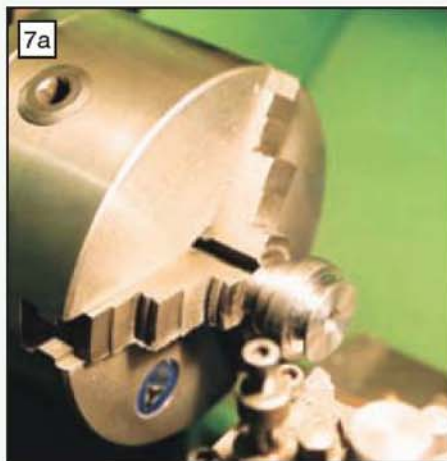
The second operation on the pulley involves the use of an expanding arbor.
