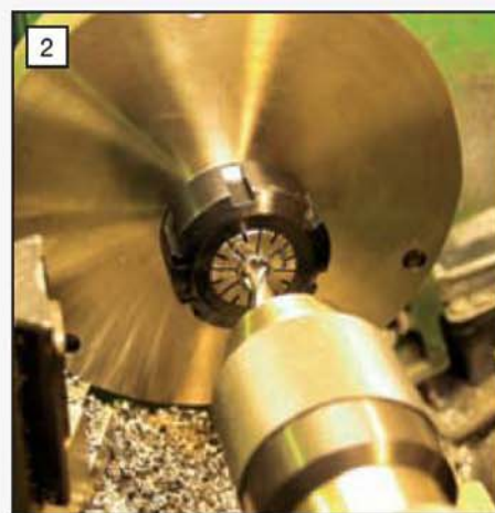
Boring the inside of the tappet using a slot drill.
