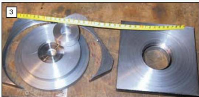
View of the under sides of the circular table and the square base. The 2in. dia. pivot pin is resting on the table.
