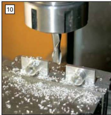
Milling the bearing housing flanges to size.
