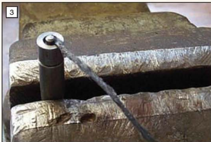
The gland packing tool, the making and use of which is described in detail in the text.
