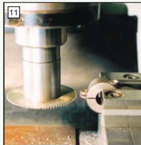
11 Slitting the table bracket main column hole using a slitting saw.
