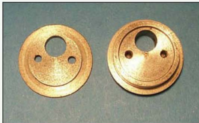
The two eccentric sides referred to in the text. This design facilitates easy fitting of the eccentric strap.
