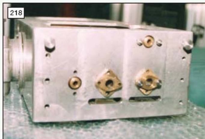
A photograph showing the valve guides fitted in to the crankcase (photo: Stan Nipper).
