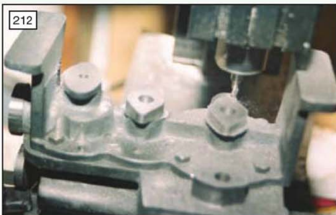
212 A CNC machine is shown being used to profile the gland bosses (photo: Stan Nipper).
