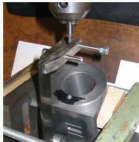
The set up used for drilling the steam passages from one of the end faces of a cylinder casting.
