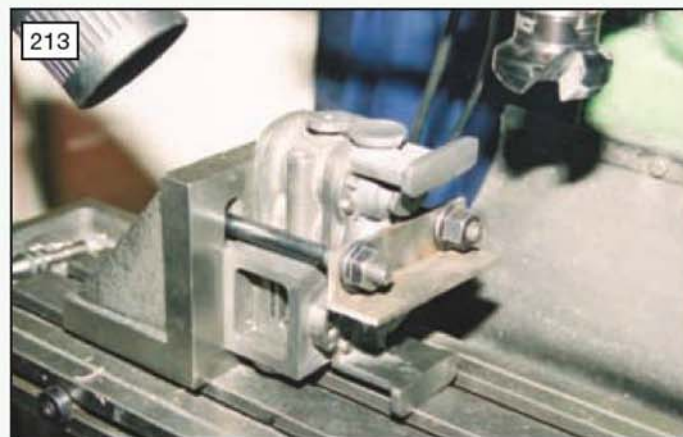
213 Larger flange on the back cover is the main steam inlet, smaller one on the cylinder is the steam inlet from the simpling valve (photo: Stan Nipper)
