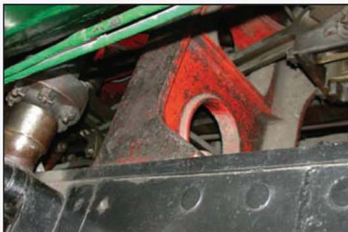
Full size slide bar stay. Note how the flush rivet heads are formed (photo: Dr. Peter Thomas).
