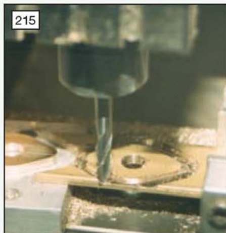
A CNC machine will make quick work of cutting out the valve rod guides (photo: Stan Nipper)
