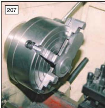
207 Facing across the front cover on the lathe (photo: Stan Nipper).
