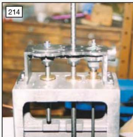
The back cover is fixed to the crankcase with six 2BA bolts (photo: Stan Nipper)
