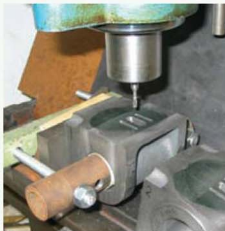
Milling the steam ports in the cylinder. Note the improvised clamping arrangements.
