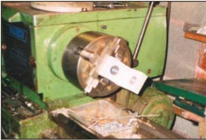
The main attachment body being bored in the 4-jaw chuck. The material chosen was Duralumin.
