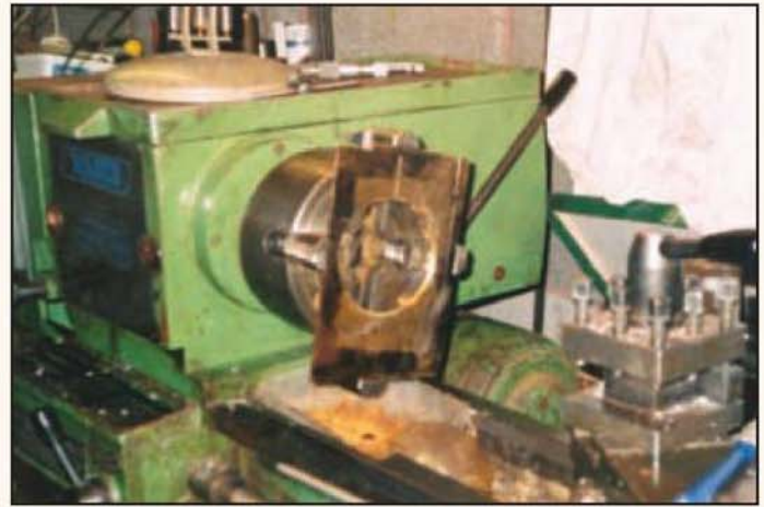
Trepanning the large hole in top plate in the lathe. It was subsequently bored to finished size.
