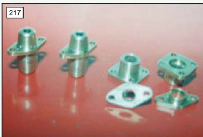
The fully machined set of valve and piston rod guides all ready to fit (photo: Stan Nipper).
