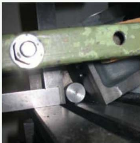
An engineer's square and a turned roller being used as an improvised sine bar.
