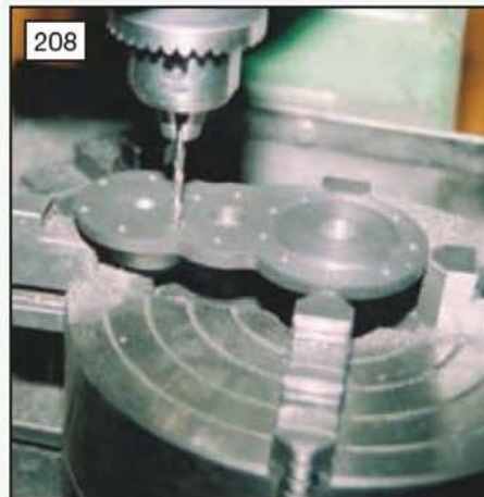
208 Co-ordinate drilling the holes for the front cover (photo: Stan Nipper).
