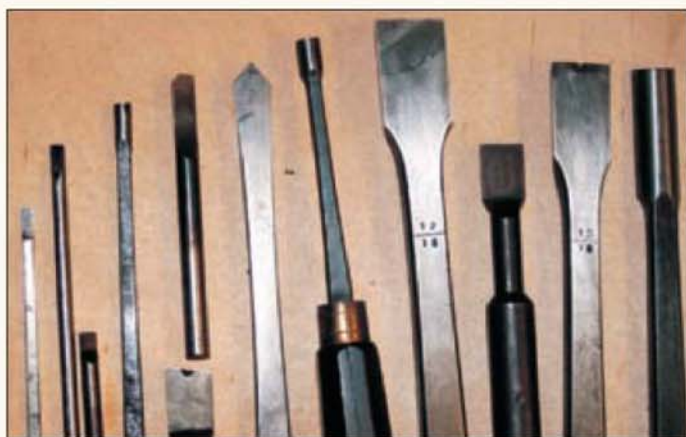
Selection of home made and commercial D-bits. Just left of centre is an early spear drill.
