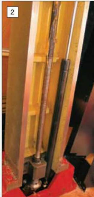
Above right: The compact X3 mill as delivered showing the Y and Z control handles at the front of the machine for easy use. Right: The top cover removed to show the toothed belt drive to the gearbox and the spur gear final drive. Above: The rear casing removed to show the gas strut and the head lead screw.
