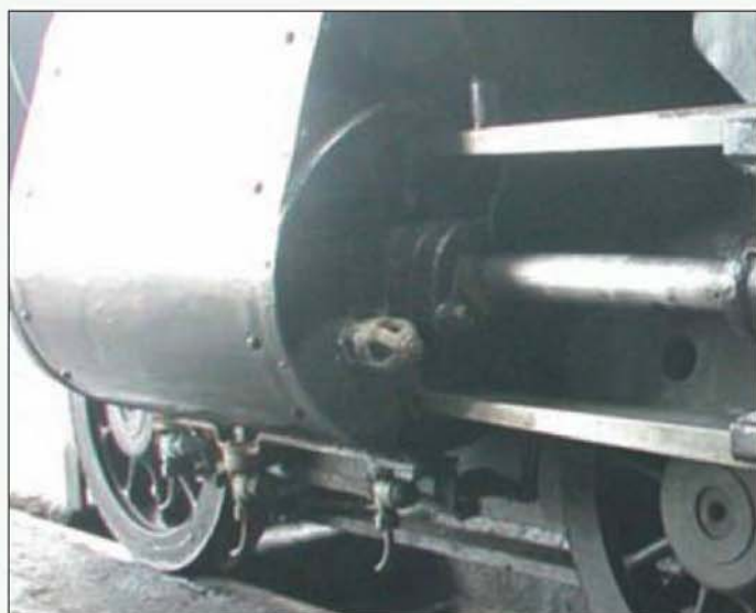
The draincocks from the opposite side. Actuation in full size is by link but a Bowden cable is used on the model.
