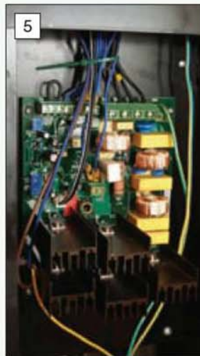
5 Electronic speed control is totally enclosed in the rear casing.
