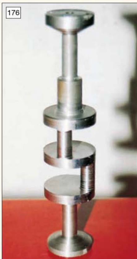
176 The roughing out is complete and the part is decidedly crankshaft looking (photo: Stan Nipper).
