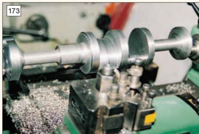
173 The crankshaft mounted between centres and driven by the catch plate. The second big end journal is being machined (photo: Stan Nipper).
