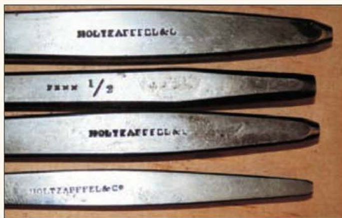
Shanks of the early D-bits. These are designed to be guided by a tailstock centre and locked by the grip of the hand or a spanner.
