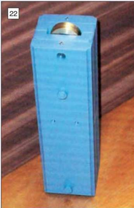
The author's driving weight prepared from pieces of steel plate.
