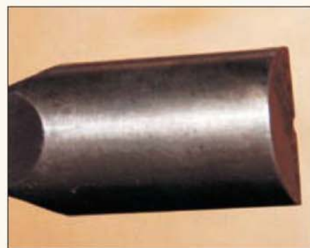
Underside of the same D-bit. Note the front clearance angle.
