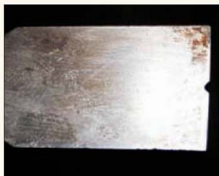
Carefully honed top of one of the author's Holtzapffel D-bits
