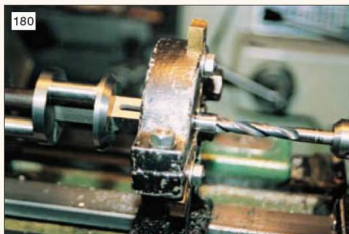
180 A fixed steady is used to support the crankshaft when drilling the hole for the valve gear operating rod in the lathe.
