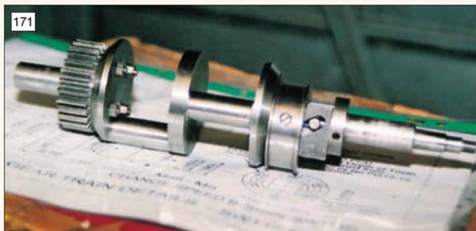
John Thompson's crankshaft with the drive gear and valve gear eccentric assembled (photo: John Thompson).
