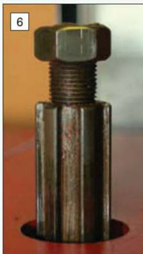
6 The captive draw bar thread on top of the quill.
