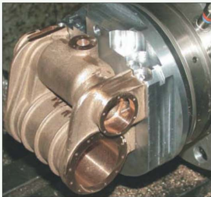
A Penrhos Grange cylinder undergoing machining at Polly Model Engineering Ltd. Note the fixture plate holding the casting.
