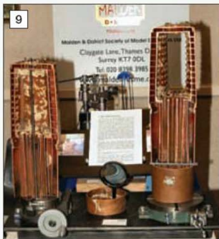
Malden DSME showed a sectioned boiler as an illustration of what happens when things go wrong.
