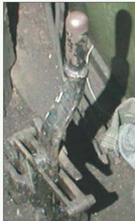
Full size draincock lever shown mounted on the cab floor.
