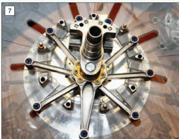
The radial engine crankshaft assembly for the engine under construction by Mike Tull of the I/C Engine Builders Group.
