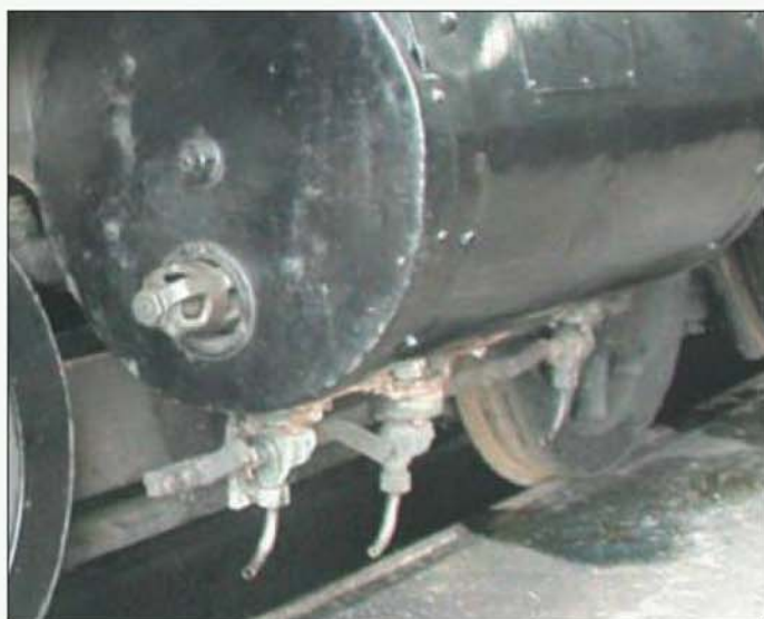
A view of the full size draincocks fitted to Manor and Grange cylinders by the GWR.
