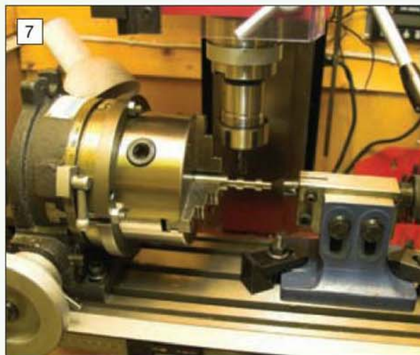
7 A 6in. rotary table on the machine with plenty of vertical clearance still available.
