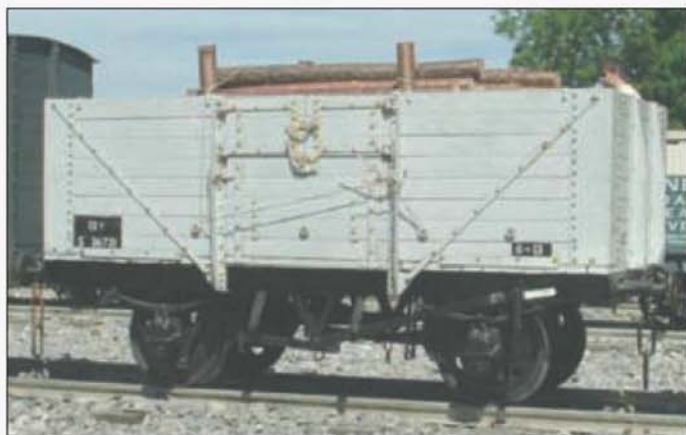
This is one of the many wagons brought to the GL5 Rally by Martin Rant from Didcot. It is a Southern 8 Plank, what the Southern term a 'High Sided Goods'.
