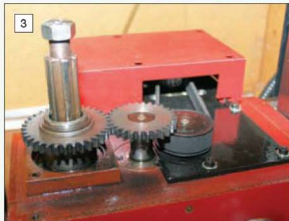
Above right: The compact X3 mill as delivered showing the Y and Z control handles at the front of the machine for easy use. Right: The top cover removed to show the toothed belt drive to the gearbox and the spur gear final drive. Above: The rear casing removed to show the gas strut and the head lead screw.
