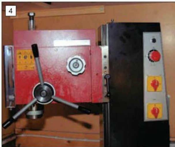
4 The quill lever and the high/low speed change knob are on the left side of the head.
