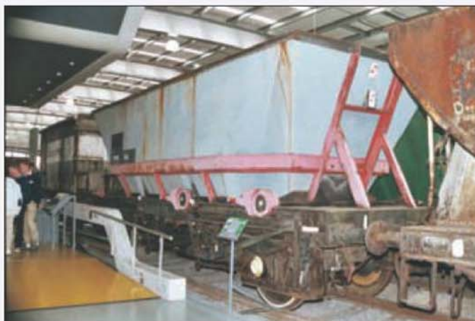
HAA coal wagon for 'merry-go-round' trains; 10,000 were built at Shildon.
