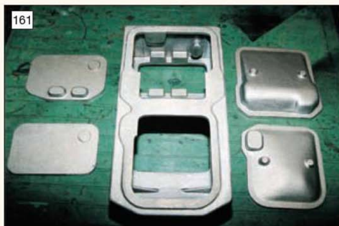
161 Inside view of the complex crankcase casting and the four covers (photo: M. Wallis).
