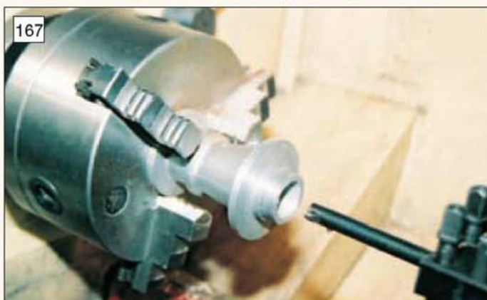
Lightly grip the casting in the chuck to avoid marking it and remember to take light cuts.
