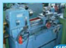
Raglan 5"x24" lathe complete with gearbox, variable speed & power cross feed
