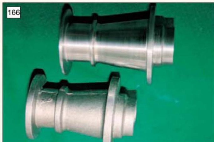
The final drive bearing housings are machined from high tensile aluminium alloy castings.
