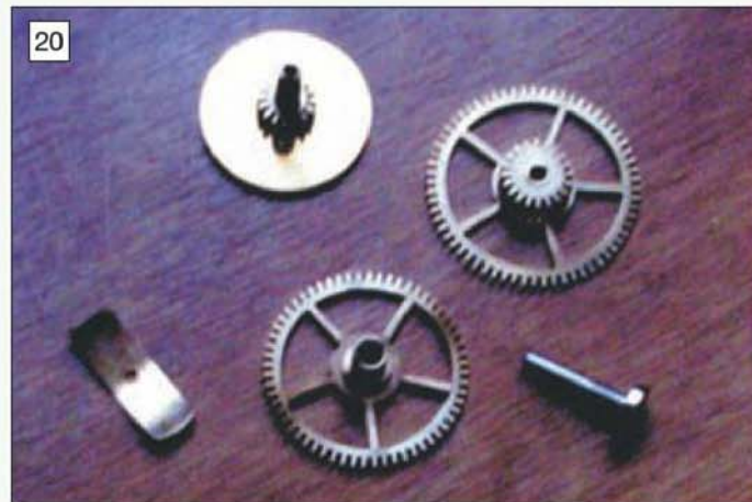
Motion work components laid out for inspection. Note the neat crossing out and, on the left, the hammered brass clutch spring.
