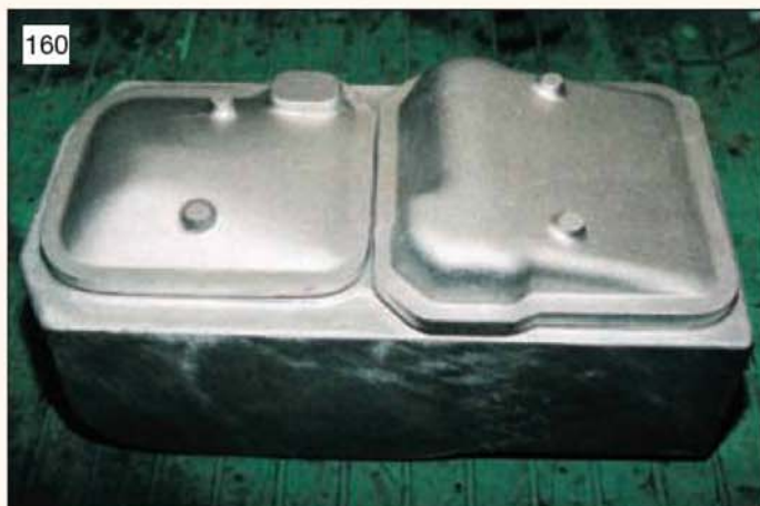
160 A view of the high tensile, aluminium alloy crankcase and top cover castings (photo: M. Wallis).
