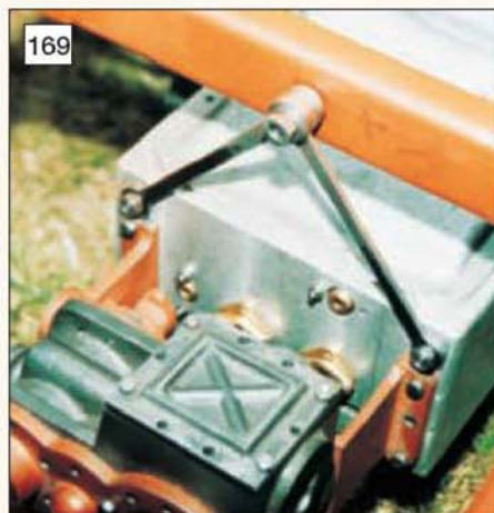
The single point chassis mounting for the front of the engine.
