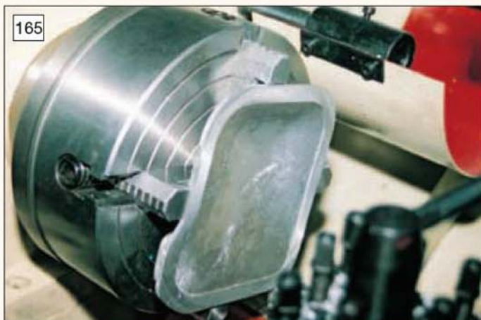
Alternatively the covers can be machined on the lathe. Do not over tighten the chuck as this may distort the relatively light casting.
