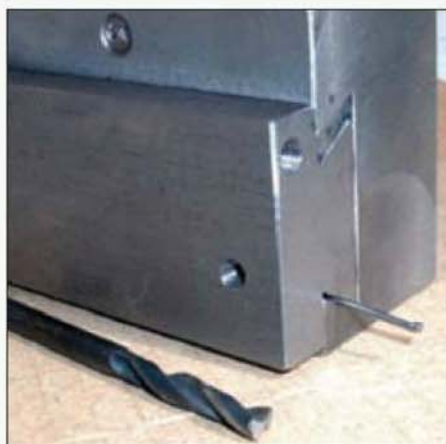
The method used by the author to locate the gib strip for drilling the clamp screw seats.
