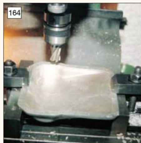
164 The mating surfaces of the covers may be machined on a milling machine.
