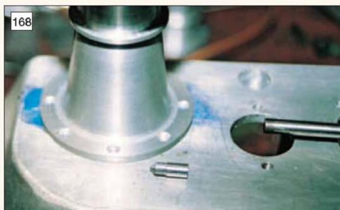
A small round dot punch may be prepared to transfer the centres of the stud holes in the bearing housing to the crankcase.
