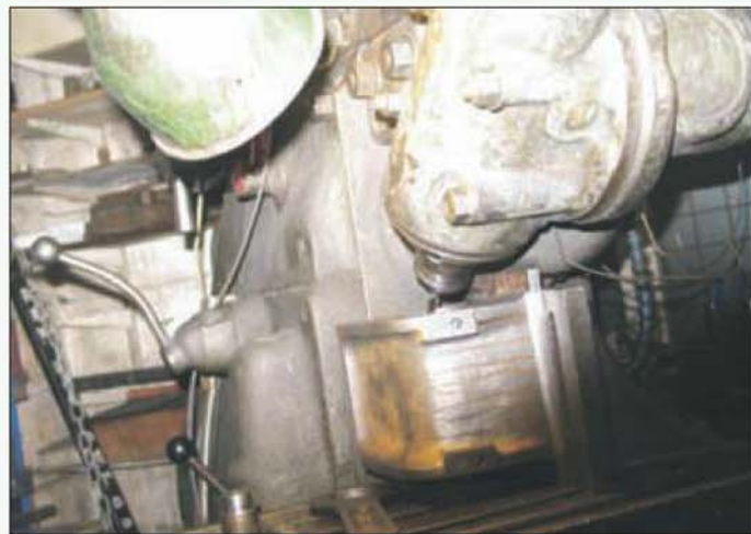
Milling the steam access ports at one end of the cylinder. A universal vertical head is a valuable accessory.
