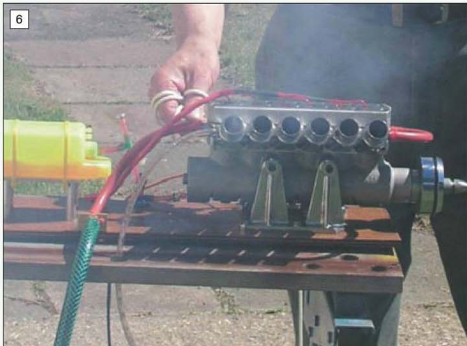
Eldon engine being run on the bench with a total loss water-cooling set-up.
