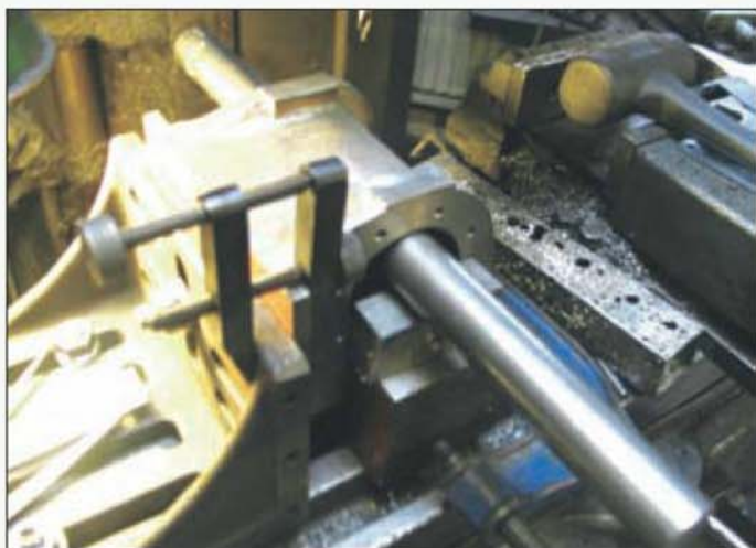
Using a piece of bar to help ensure the cylinder bore is parallel to the top surface of the milling machine table.
