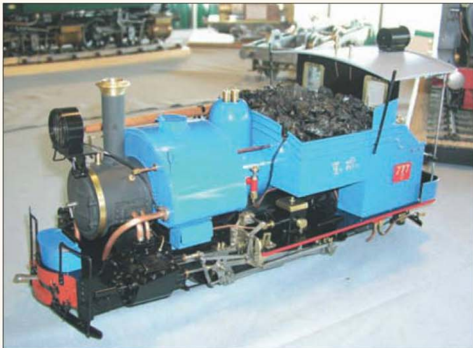
This 2 1/2in. gauge model of the very pretty B series Darjeeling 0-4-0 saddle tank locomotive No.777 was built by Jack Evans and was awarded a VHC Certificate and the Bill Deane Memorial Trophy.
