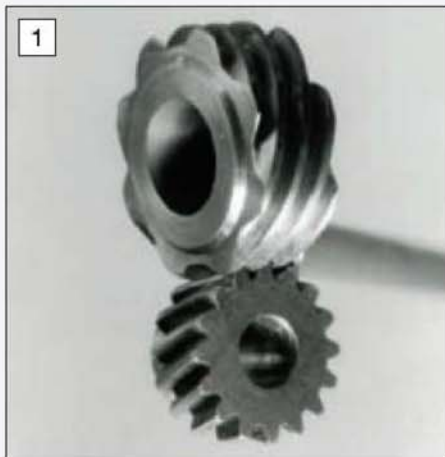
The finished gears made by the methods outlined in this article.
