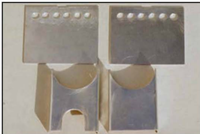
The components for the firebox were made from aluminium alloy and have been cut, drilled and bent prior to rivetting together.
