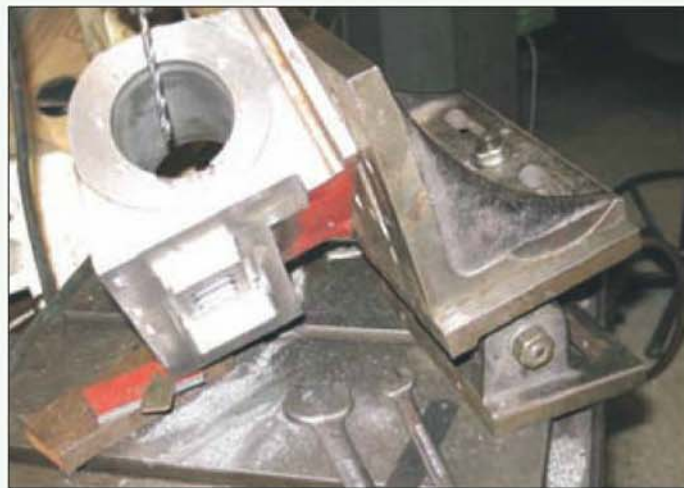
Drilling the steam ports on the drilling machine using an adjustable angle plate in conjunction with a fixed angle plate.
