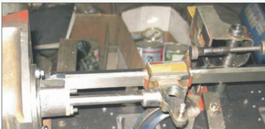
Left to right: The cylinder block including the floating gland cover, dummy piston rod and guide bar. A G-clamp holds the motion bracket in place and the cross-head on the dummy rod. A 3/4 in. dia. pin is placed through the motion bracket to locate it on the frame. An O-ring on the end prevents the pin dropping through.
