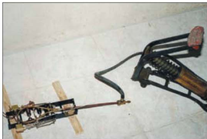
Initial tests on the chassis were made with a foot pump. The foot pump used originated from a 1930s Sunbeam car.
