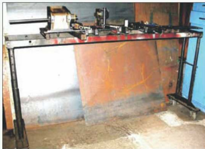
The portable erection stand. On the top is the left-hand frame member with its cylinder and other parts.
