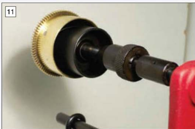
11 Once the spring is safely contained by the retaining ring the clock barrel can be refitted.
