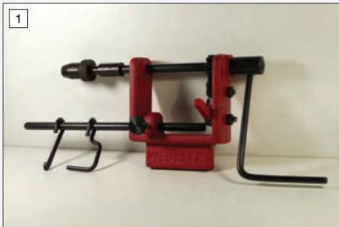
The Meadows & Passmore mainspring winder is based around a robust cast iron frame.
