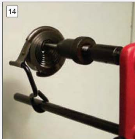
14 This form of mainspring winder is well equipped to deal with clamped loop-ended springs.
