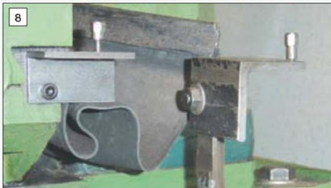
Photographs 6 to 11. The digital readout scales fitted to the author's milling machine showing details of the fixing brackets.
