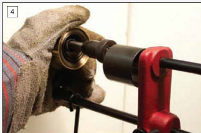
The first stage in removing a spring from its barrel is to offer the eye in the centre of the spring up to the hook on the arbor.
