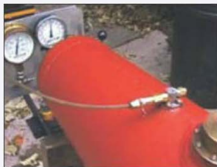
The proof of the pudding, the pressure at 160psi, not a weep.
