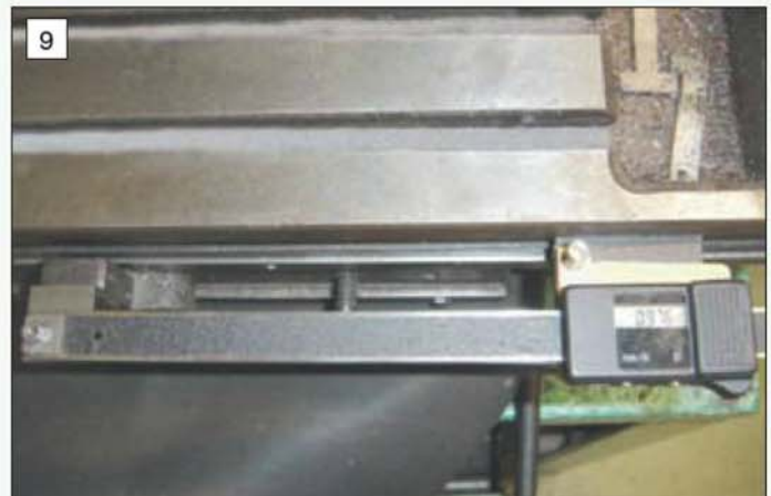
Photographs 6 to 11. The digital readout scales fitted to the author's milling machine showing details of the fixing brackets.
