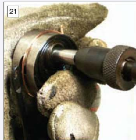
21 Gripping the spring tightly fit the hook attachment as shown.
