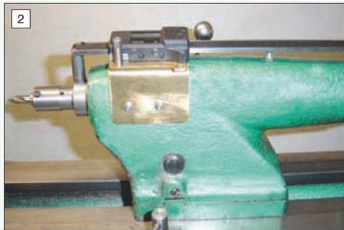
This photo shows how the digital readout slide bar is mounted on the front of the tailstock barrel.
