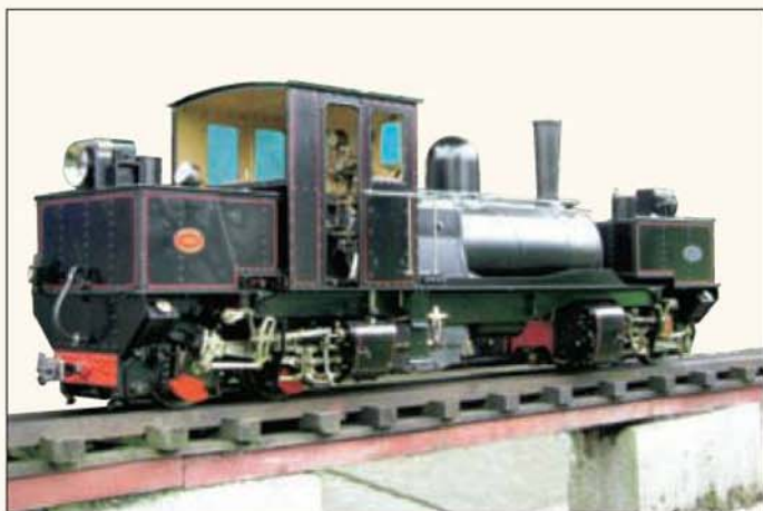
John Hartup's superb 3 1/2in. gauge K Class 0-4-4-0 Garratt. The first two Garratts were supplied by Beyer Peacock to the 2ft. gauge North East Dundas Tramway, Tasmania. The engines differed from subsequent Garratts in being compounds and the cylinders were at the inner ends of the bogies.
