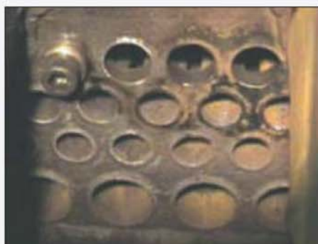
The collet fitted in the firebox.
