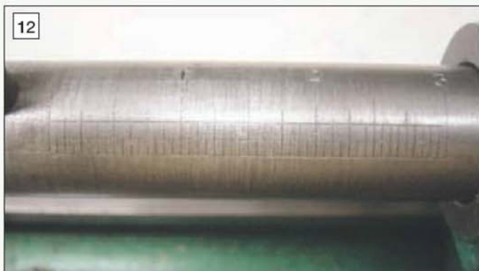
Above: The rule markings on the lathe tailstock. Right: Setting the top-slide round to 5deg. to provide a fine feed facility.
