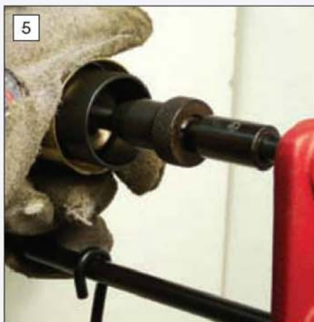
5 Wind up the spring and insert the retaining ring. 1in. of the spring should protrude from the slot.
