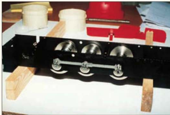
The wheels fitted to the frame and coupling rods in place. The frame has been painted as have the buffer beams which are in the background.
