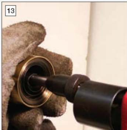
13 The spring can then be unwound into its barrel. Note the gloved hand.
