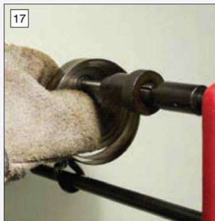
17 Rewinding is best carried out using a gloved hand to control the spring.
