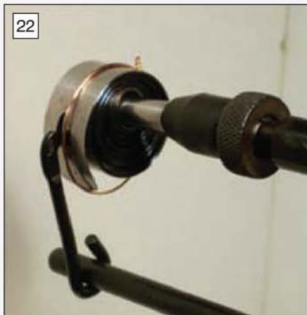
Now wind the spring up until the tension on the retaining wire is released.
