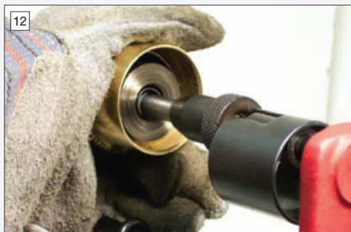
12 Engage the barrel hook on the hole in the tail of the spring, wind the spring up slightly to release the retaining ring and pull it clear.
