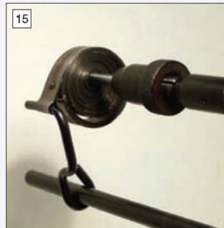
15 By winding the spring up slightly the clamp can be released.
