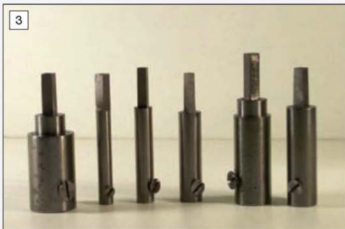
The set of winding arbors made by the author to suit this particular type of mainspring winder.
