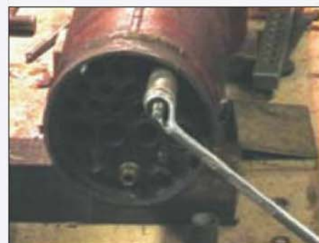
Suitable spacers used to fully extract the tubes.
