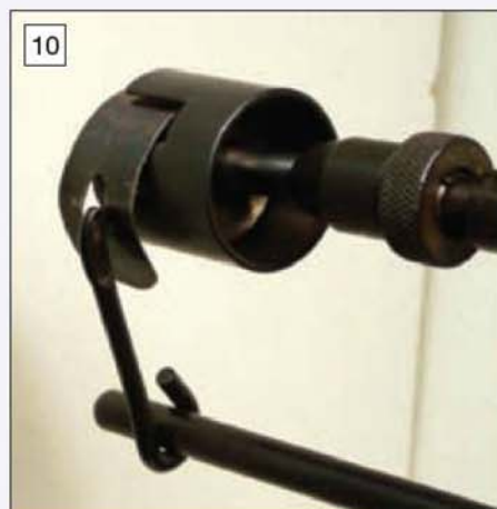
10 When rewinding a spring, first wind it up using the hook then fit the retaining ring.
