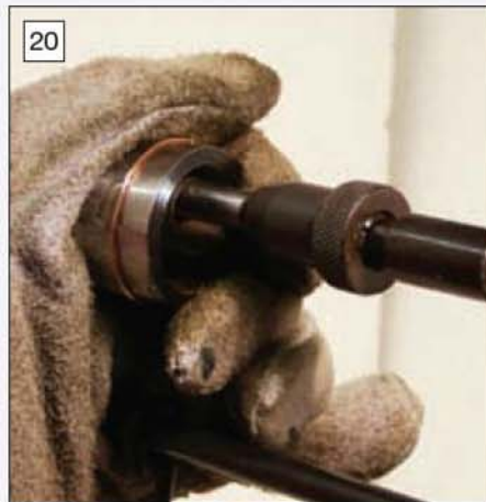
20 For new barrel springs retained by wire first fit the spring to the arbor and wind up slightly.
