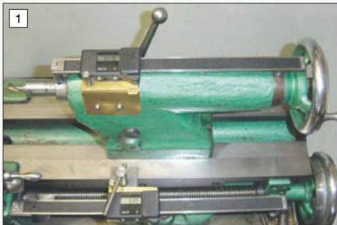
A view of the digital readout scale fitted to the tailstock of the author's lathe to give a direct indication of barrel position.
