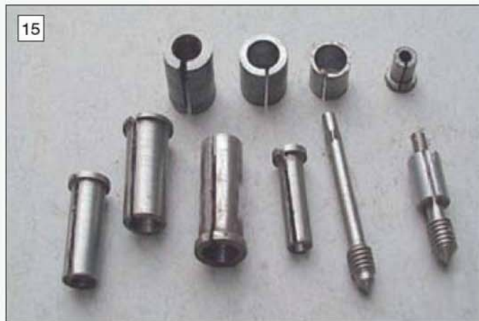
A selection of special collets made from bright mild steel for different jobs and carefully stored for future use.
