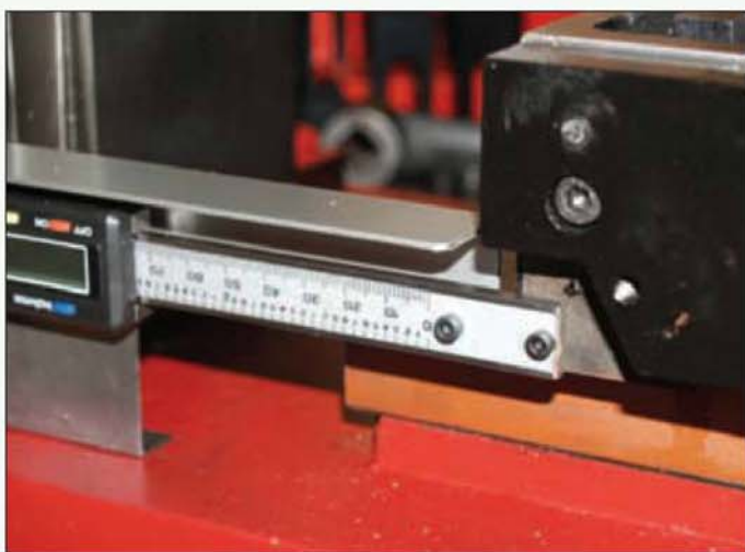
5. Y axis decoder mounting on the machine base.
