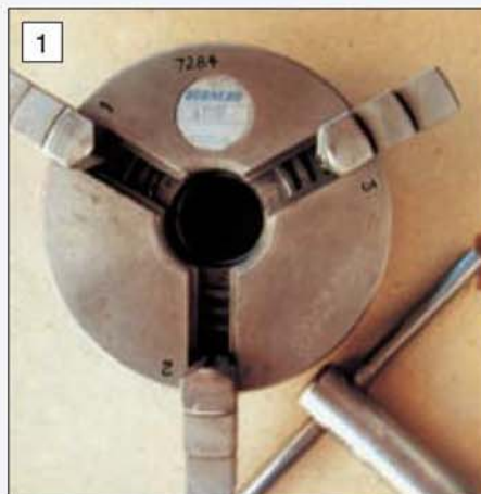
Typical 3-jaw chuck for an amateur's lathe fitted with its jaws for small diameter bar work.
