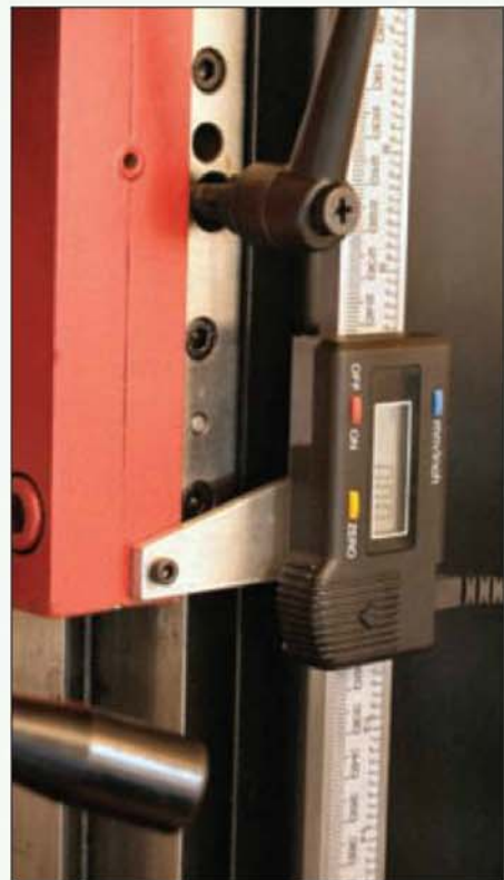
2. Z axis decoder showing the bracket fixing.
