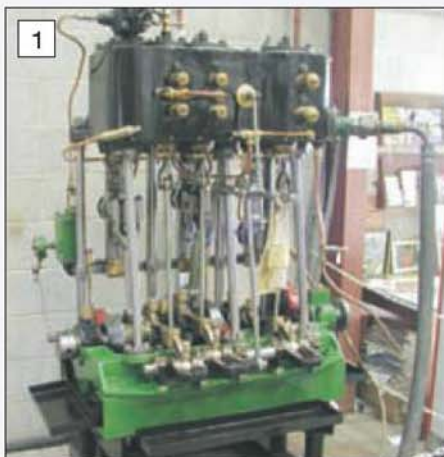
1 The Sisson triple expansion steam marine engine that inspired the project.
