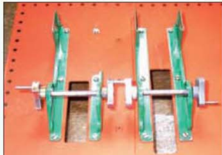
Crankshaft and frames only for alignment adjustment.
