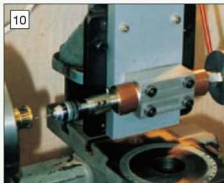
10 The set-up used for drilling lantern pinions. This spindle has been turned through 90 degrees.
