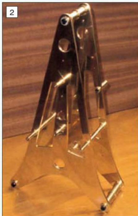
A trial assembly of the frames and pillars. The clock is already beginning to take shape.
