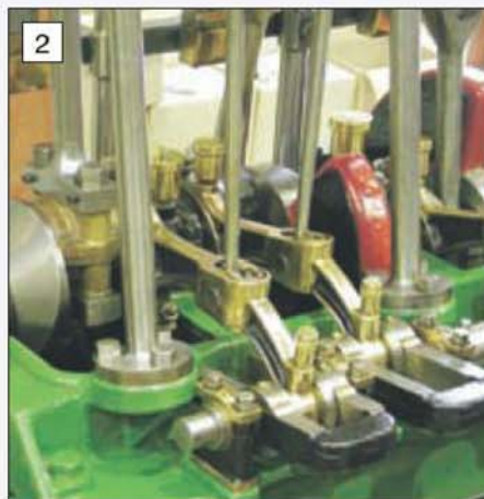
2 A close up view of two of the three sets of valve drive and reversing gear.
