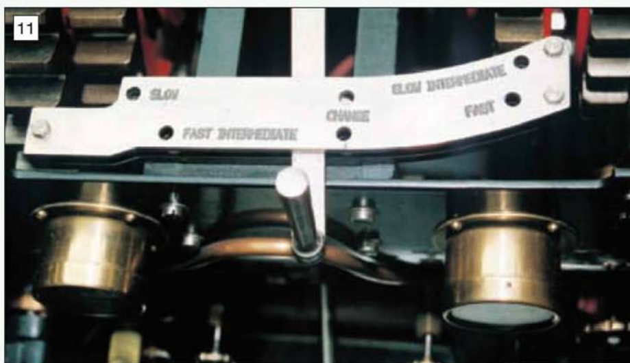
11 The gear selector neatly engraved with the gear positions. The vehicle was unusual in having four speeds instantly available with an additional four provided by a change of gear if required.
