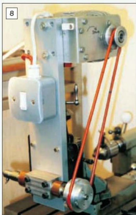
8 The author's home made wheel cutting spindle and drive arrangement.
