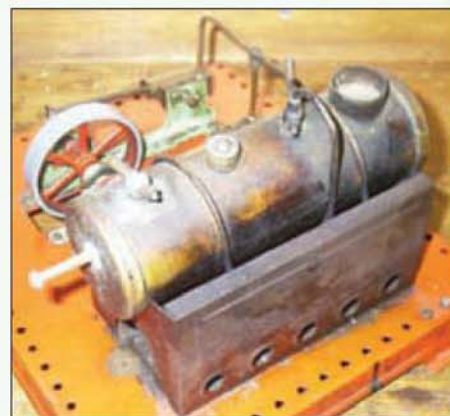
Close-up view of engine 'B' showing the poor condition of the boiler.
