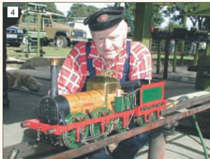
Geoff Cocking's Thunderbolt was the only 3 1/2 in. gauge model in the competition. The name explains the unusual colour scheme and reminds us that Curly Lawrence originally published the design as Titfield Thunderbolt.
