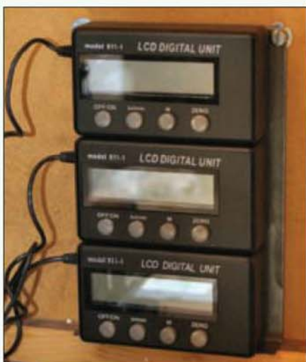
7. Z axis decoder showing the bracket fixing.
