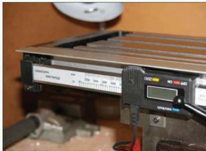
4. X axis decoder showing the bottom of the mounting bracket.
