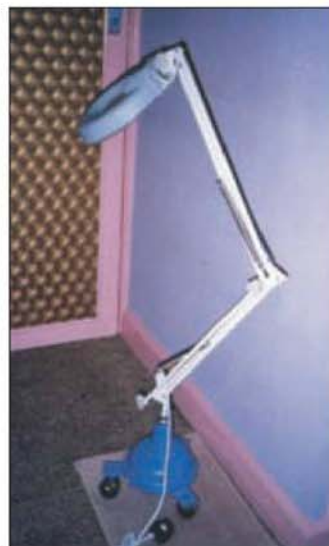
A Mercedes truck wheel hub from a vehicle scrapyard was the solution to James Wells' lighting problem!
