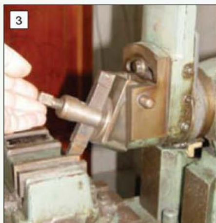
The clapper box prevents the tool dragging during the return stroke.
