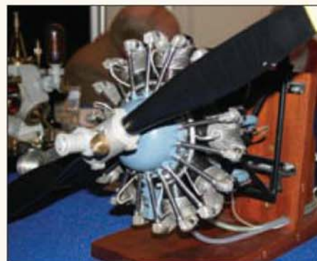
7. Another engine by Ron Harris, this time the 9 cylinder Pratt and Whitney Wasp radial engine.
