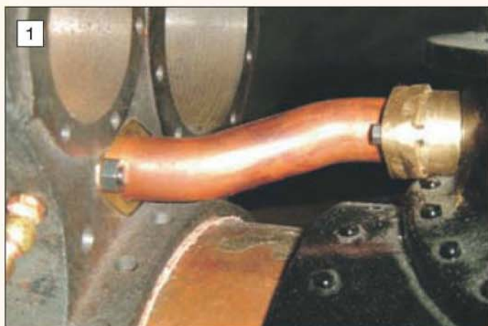
1 A tight bend accomplished in copper tube to form the exhaust pipe on the author's traction engine.
