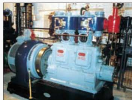
Totally enclosed Reader Compound Engine coupled to a dynamo generating 440v D.C.
