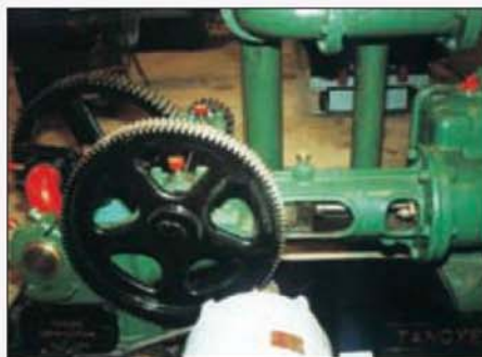
A 1931 Tangye Sludge Pump used at Lewes Treatment Works until 1998.
