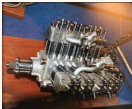
6. Another V8, this time Ron Harris's 98cc engine based on the 1924 Airdisco engine.
