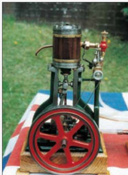
Well-restored early 20th century vertical engine. The oil box fitted to the top of the connecting rod is noteworthy.
