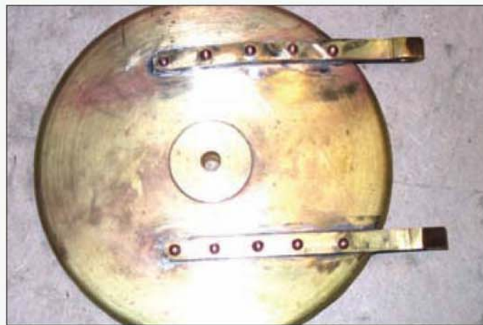
The finished smokebox door fitted with its hinges is a heavy item. Castings for the door and smokebox ring should be available in due course.
