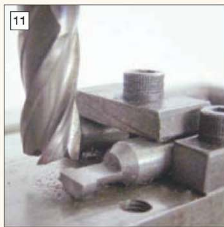
11 The fixture is used to put the flat on D-bits and ensure only the correct amount is removed.
