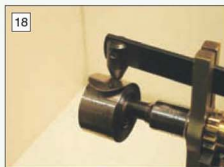
18 With the wire removed the spring is still fully under control.
