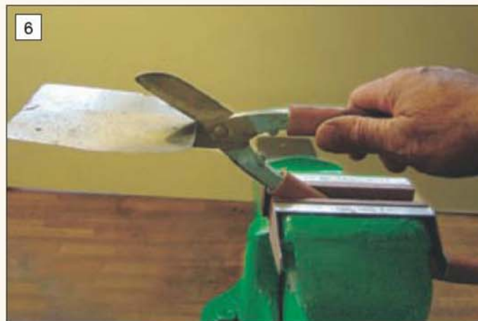
It is sometimes useful to grip one handle of tin snips in the vice to help give better control of the cut.
