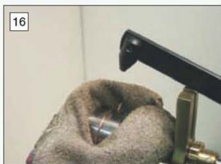
16 Fitting a new spring to the winder arbor for unwinding, cleaning and inspection.
