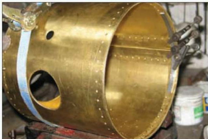
The smokebox barrel can be rolled from 3mm thick brass. Here the butt strip is about to be fitted.
