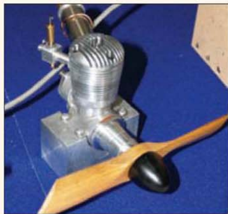
2. John Scott-Scott's 6.5cc sleeve valve aero engine
