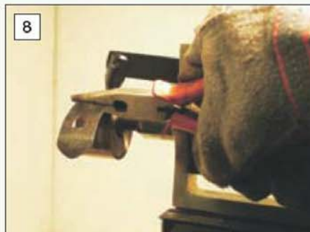
8 With the tail of the spring gripped by pliers the barrel can be removed and laid aside.
