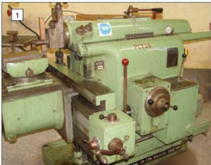
The 18in. stroke Butler Super Shaper, a machine that the author found pleasant to use during his time in industry.
