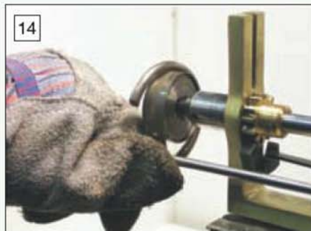
14 When the C-clamp is to be refitted, wind up the spring, refit the clamp and reverse the ratchet.
