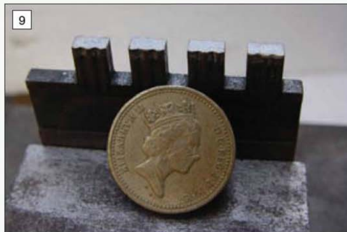
Punch used to form the pockets or windows in the upper plate of the Braille slate.
