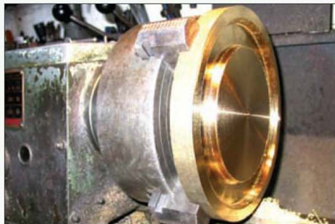
Turning the smokebox door ring from solid bar. The centre was salvaged to form the top of the steam dome.
