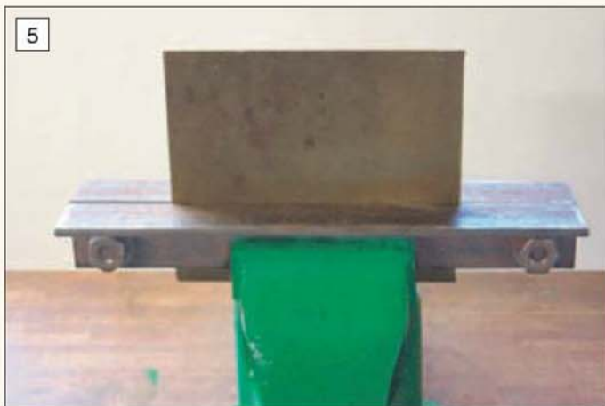
Angle iron can also be used to make useful support bars for bending sheet material. Use different pieces to those for the sawing guide.
