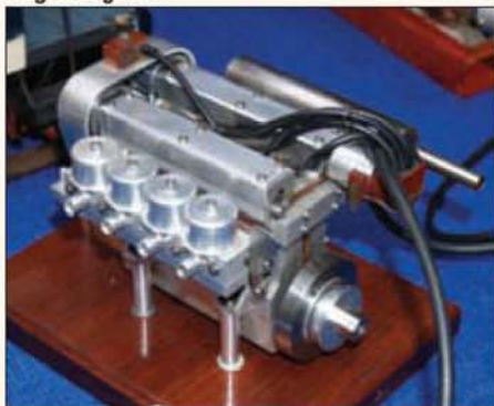
11. Another fine engine on the Birmingham stand, this time a DOHC four cylinder spark ignition petrol engine.
