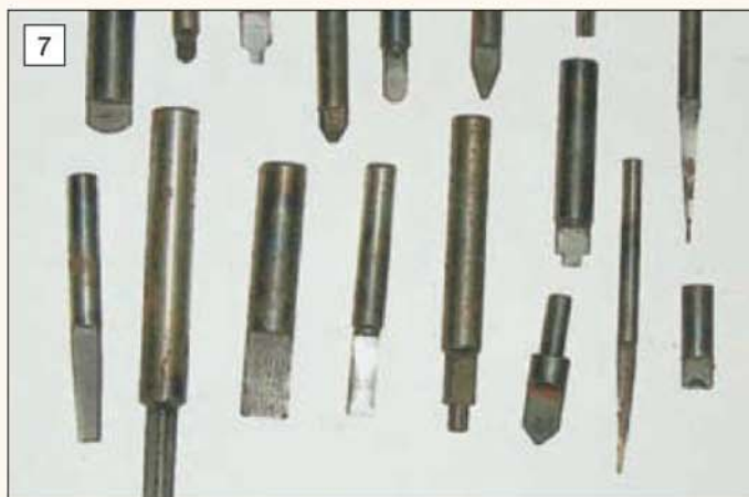
Selection of D-bits made by the author. These are kept and carefully stored for future use.
