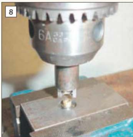
8 An unusual D-bit devised to remove a broken 1/16in. drill from a work piece.
