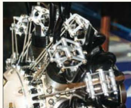
13. Cylinder head detail on the Gerald Smith 18 cylinder radial engine, built between 1924 and 1930.
