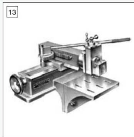
Perfecto Model No. 1 hand operated shaper was based on earlier designs.
