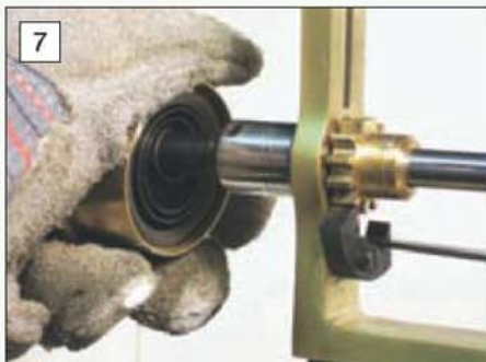
7 Winding up the spring in the barrel prior to its removal.
