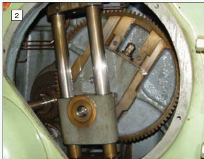
Ram actuation mechanism in the Butler shaping machine permits the stroke length to be rapidly changed.
