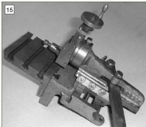
Left: Although small the Adept 1A shaping machine was capable of useful work in the hands of model engineers.
