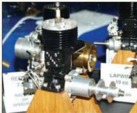
12. The Gerald Smith Wizard 10cc single cylinder two stroke engine.
