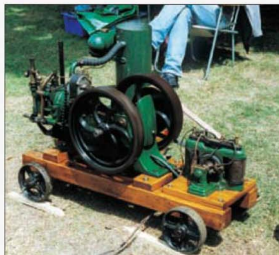
Right: Hartop 'S' Type engine of circa 1923 driving a Dynamo from around 1890-95. This develops 12-18 volts D.C. and was made by the Dymo-Crypto Works Co. Ltd. of London.
