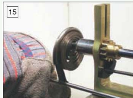
15 Unwind the spring in a controlled way until constrained by the C-clamp.
