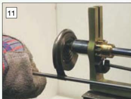
11 Loop ended springs can be dealt with by inserting a rod in the spring loop.
