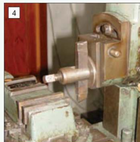
The clapper box drops down into cutting position under its own weight.
