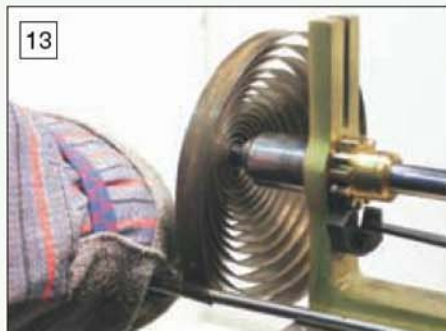
13 The spring can then be unwound in a controlled and safe manner.
