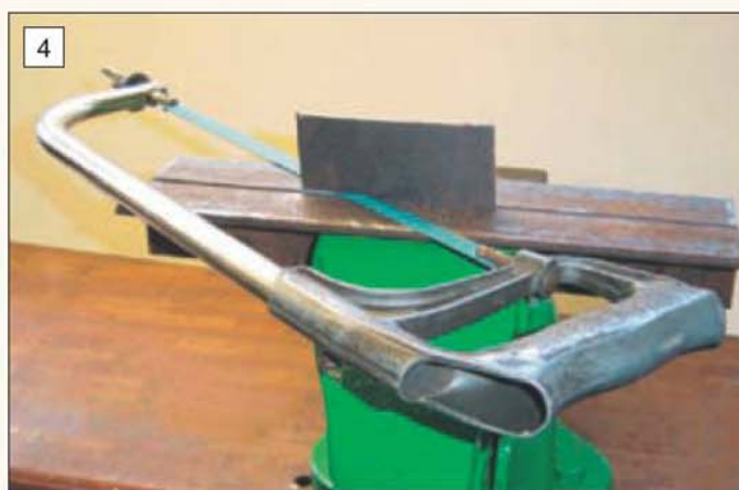
4 Sawing thin material can sometimes be more readily accomplished by using angle iron as guides and using the saw on its side.
