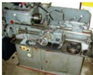
Harrison L5 9" Swing Gap Bed Lathe, Chucks, Steadies, Toolpost, Bed Stop, 3ph, £975.00 plus vat
