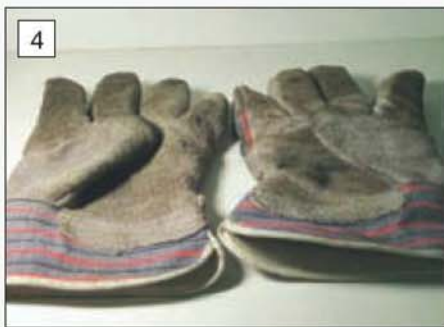
4 Stout gloves should always be used when winding or unwinding clock springs
