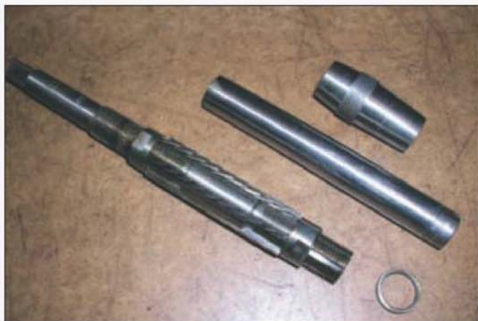
Component parts that go to make a standard adjustable reamer into a pilot reamer.
