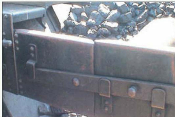
Coal door detail showing the latch and rivet layout. This photo was also taken at Toddington.
