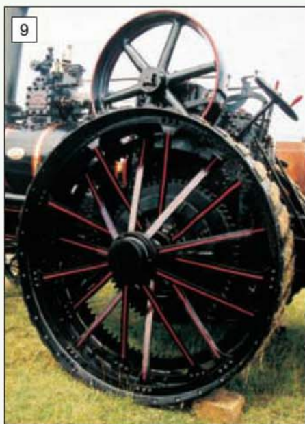
One of the rear wheels of the Fowler type BAA traction engine.
