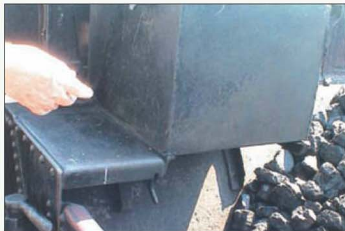
Lower part of the toolbox showing the support bracket and plates used on these tenders
