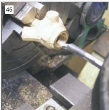
45 Machining the thread in the top of the fuel mixer body for the cap.
