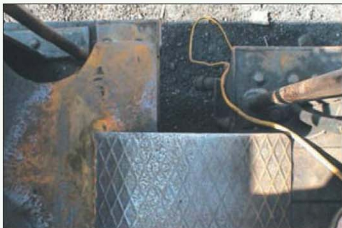
Aerial view of the shovelling plate. That for the model would be best made from steel like the prototype.
