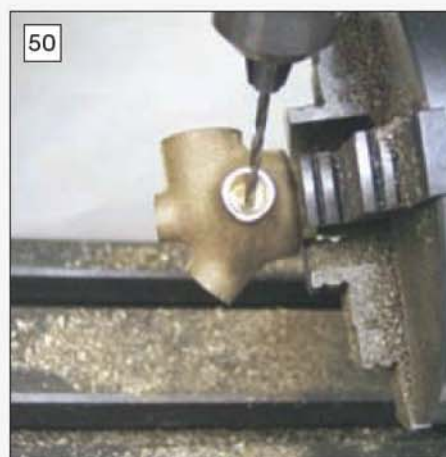
50 Drilling the transfer port hole in the fuel mixer body casting.
