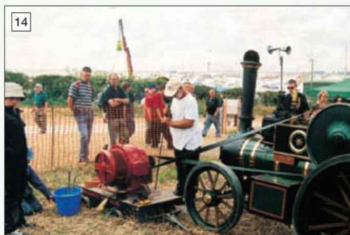
Fun with the dynamometer at the Great Dorset Steam Fair. The McLaren produced 13bhp.
