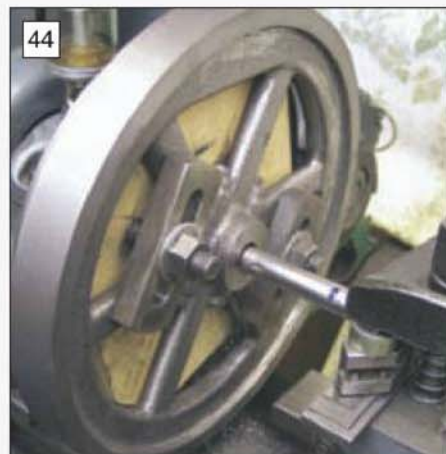
Cutting the key way in the bore of one of the flywheels with a special slotting tool.
