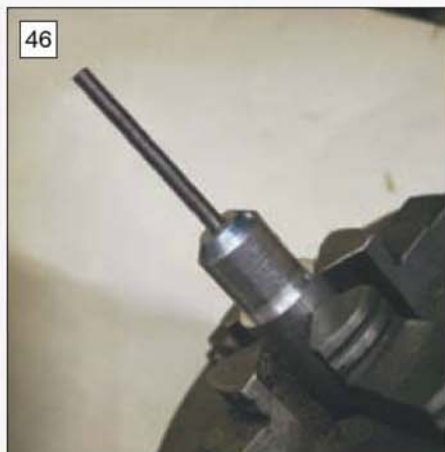
46 The mandrel devised for drilling the jet hole so that it comes out correctly in the valve seat face.
