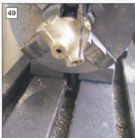
49 The method used to line up the drill prior to drilling the transfer port hole.
