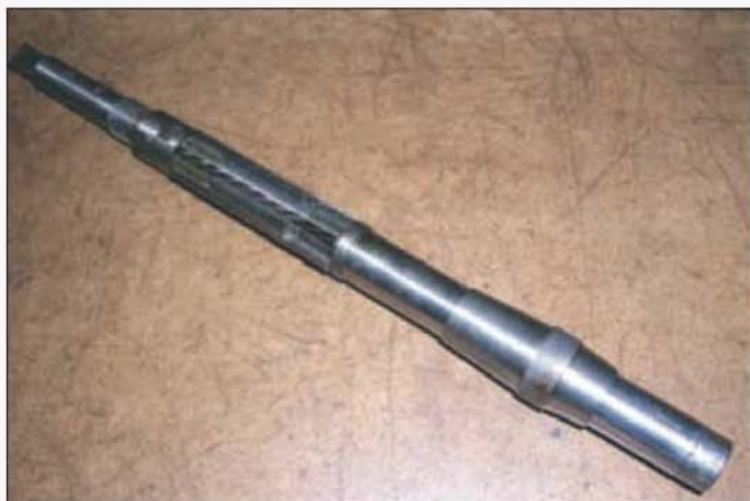
Typical adjustable reamer assembled with its extension pilot and tapered pilot sleeve.
