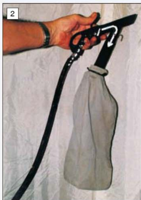
Marked up photograph showing the path of the compressed air in the device.
