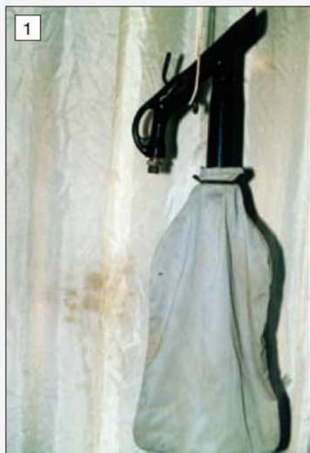
The compressed air vacuum cleaner used by the author for sucking up sawdust.
