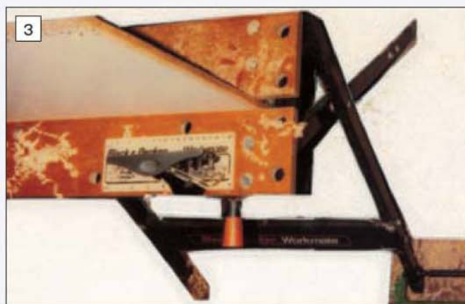
Steadying a Black and Decker Workmate with an old G-cramp. A foot is placed on the clamp.
