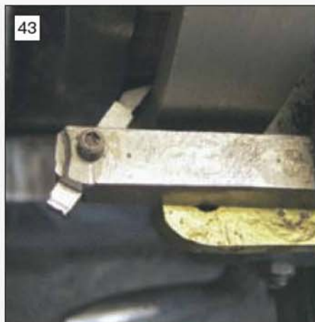
Machining the flywheel face nearest the faceplate with a hooked tool.
