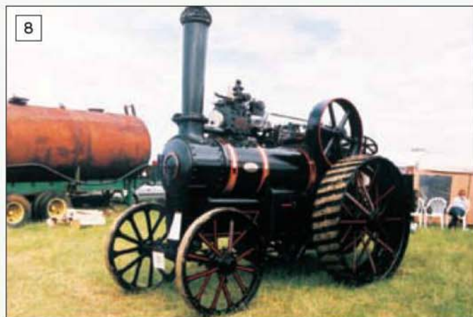
Richard Vernon's 1909 BAA Fowler No.11717, an unusual engine designed for colonial use.
