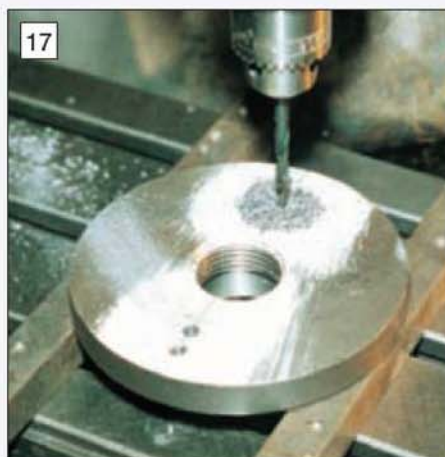
Drilling the back plate for the driving slot in the mill/drill machine.
