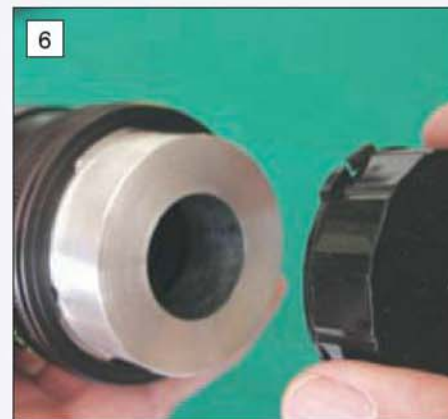
The plastic lens cover being used to check the dimension of a click in adaptor.
