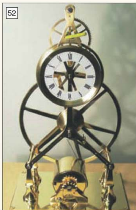
52 Escape wheel restrained, and the fusee line fed on to the fusee.
