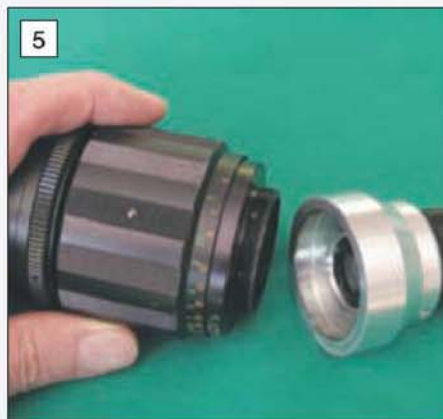
Some lenses have a 'T-adaptor thread' which is 42mm dia. and 32tpi.
