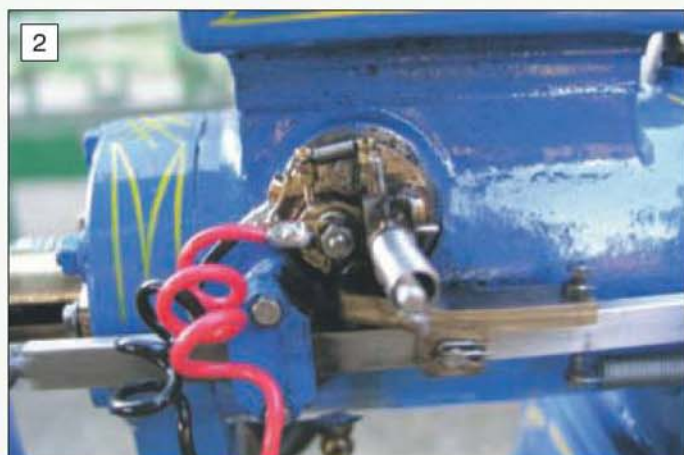
Contact point operating mechanism on the Galloway engine.
