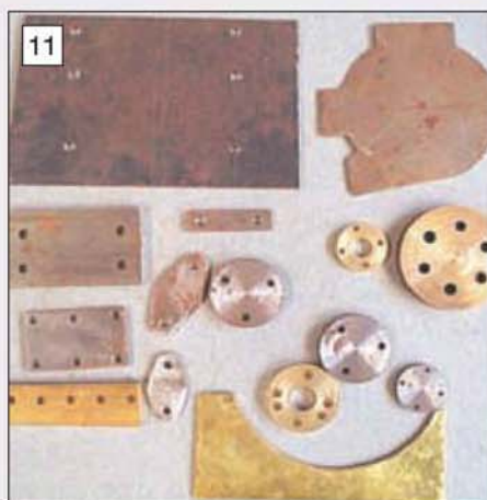
Selection of jigs made by the author as an aid to accuracy and ease of manufacture.
