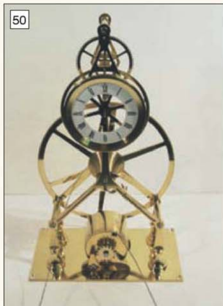
50 Ready for setting the mainspring. It should be clamped down for this operation.
