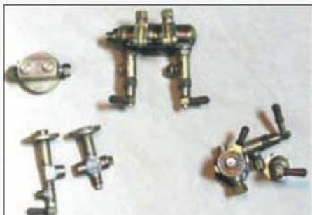
A selection of backhead fittings. Bottom right is the brake control valve with its distinctive rows of holes.
