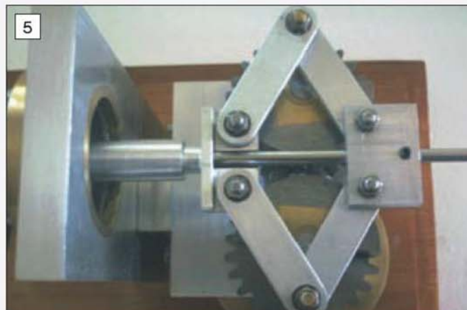
Close up view of the rhombic drive arrangements. The gears linking the two crankshafts can be seen below.
