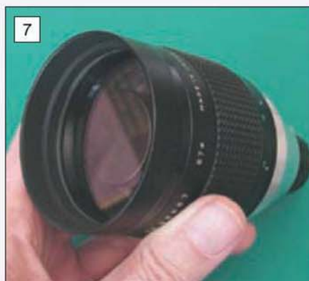
A 300mm mirror lens makes a compact unit but the x40 magnification needs a steady hand.
