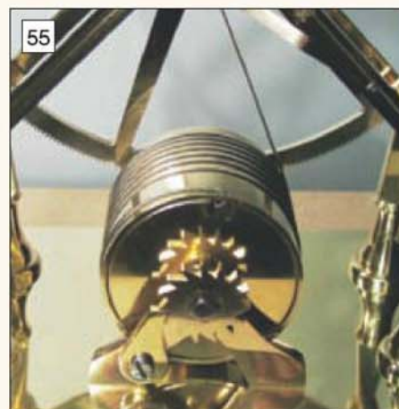
55 After winding all the line is on the mainspring case and the ratchet click secured.
