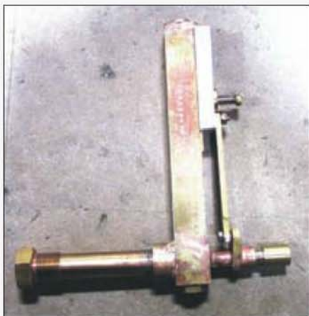
The recommended form of regulator for Lillian offers proportional opening.
