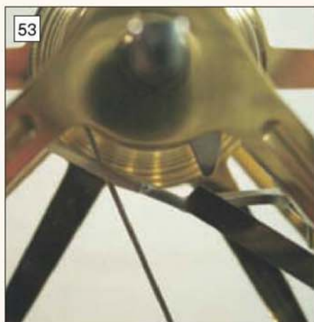
53 Beak of the fusee stop just approaching the notch in the stop lever.
