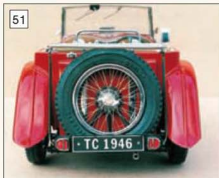
Petrol tank and spare wheel from rear of car.
