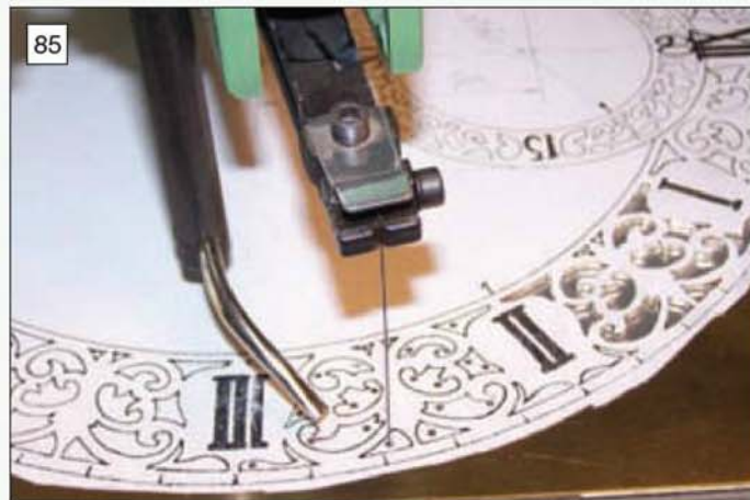
Fretting out the dial ring on the author's Rexon powered fretsaw. Note the drawing is glued to the brass with Spraymount.
