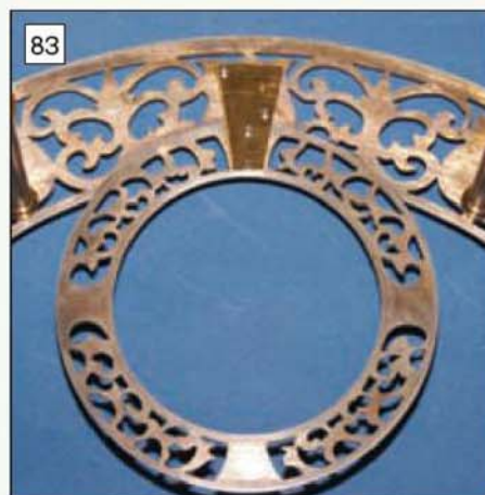
Reverse view shows how the seconds ring is secured into position.
