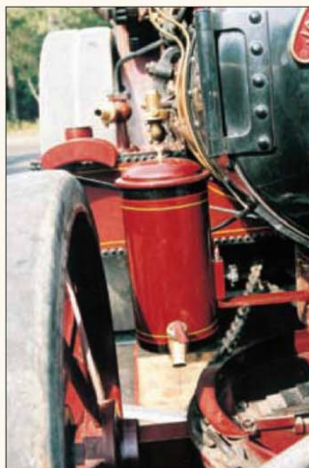
The neat steam kettle fitted to the author's Fowler road locomotive.
