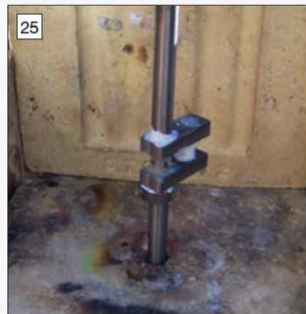
Silver soldering the parts of the crankshaft together on the brazing hearth.
