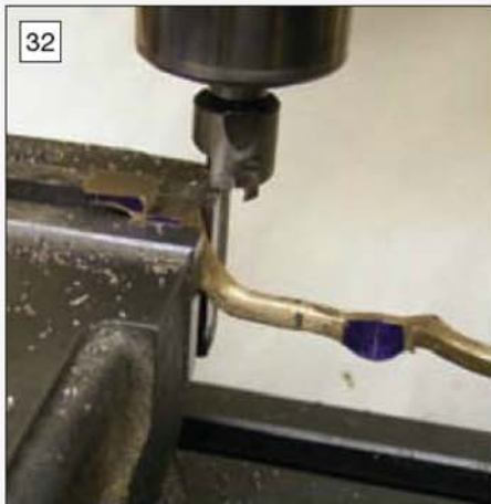
After marking out a step was milled on the latch-out bar as shown.
