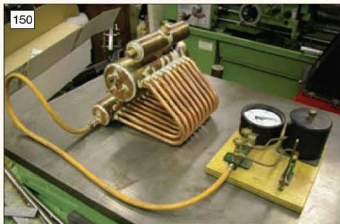
The completed, unusual water tube boiler undergoing its pressure test on the bench.
