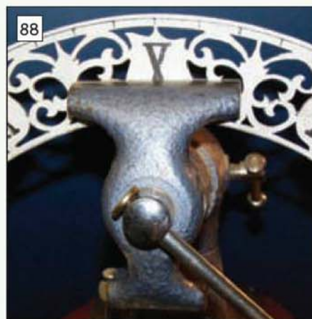
88 The dial held in the instrument vice, a useful aid for delicate work.
