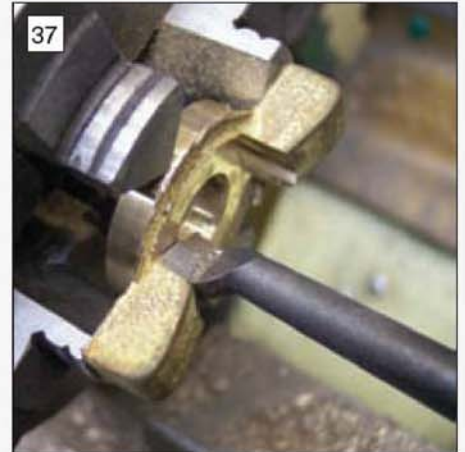
Machining the recessed face on the governor weight bracket.
