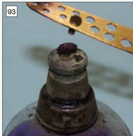
93 Method used to blue small screws. The screw should be a loose fit in the hole.
