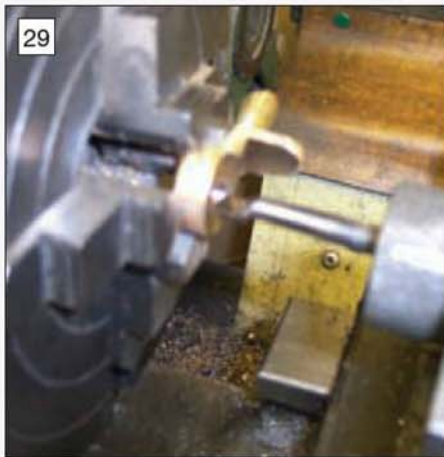
Boring the hole in the timing gear lever with the work in the 4-jaw chuck.
