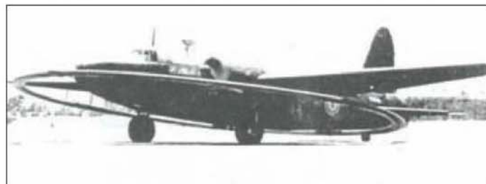
Wellington Mk. IA bomber equipped with a 48ft. mine hoop.
