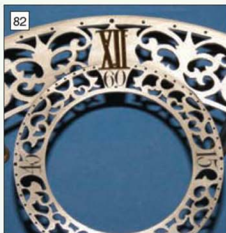
View showing how the seconds ring is let into the main ring.
