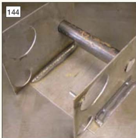
John's fixture designed to keep the boiler components together during silver soldering.
