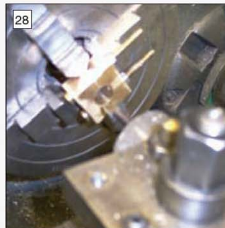
Boring the big end bearing in the lathe. The outer dimension were subsequently machined to size.
