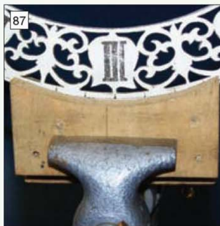
87 Curved vice chops were used to support the ring during filing.
