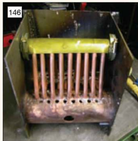
The boiler in position in the fixture during silver soldering.
