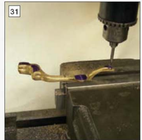
Further operations on the latch-out bar were facilitated by marking out on the milling machine.
