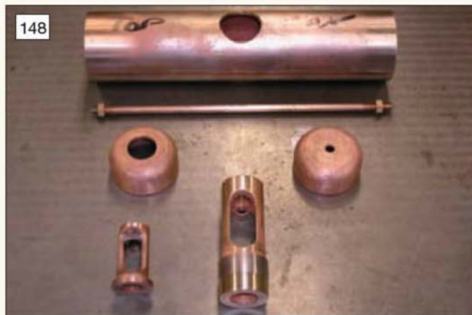
The various components of the steam drum shown prior to silver soldering them together.
