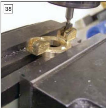
Machining the slots in the governor weight bracket on the milling machine.
