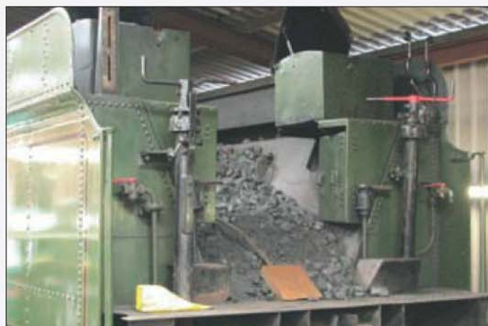
The new Grange cab photographed under construction at Llangollen. The other photos show a 4,000gal. tender (photos: Pete Thomas).
