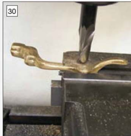
First operation on the latch-out bar is machining the flat on the central lug.
