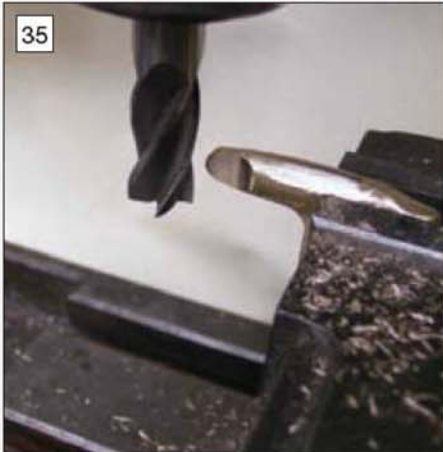
The method used to produce the beaks on the governor weights.
