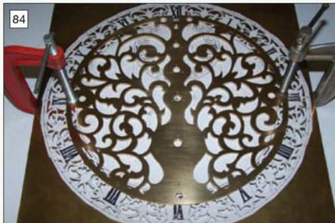
Method of clamping the back plate and the dial together while drilling the dial pillar holes.
