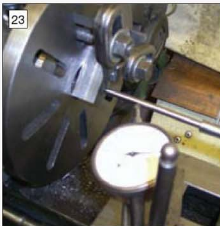
Picking up a centre on the two crank webs prior to boring on the faceplate.
