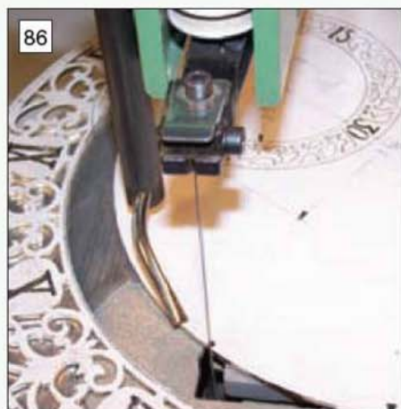
86 The dial centre was also removed using the powered fretsaw.
