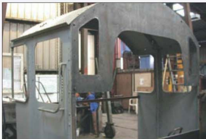
The new Grange cab photographed under construction at Llangollen. The other photos show a 4,000gal. tender (photos: Pete Thomas).
