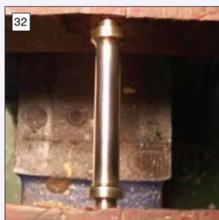
A pillar being gripped ready for polishing in the bench vice.
