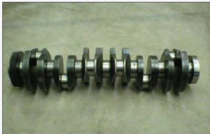
The finished crankshaft for the model's engine. The prototype engine is the Caterpillar 3406E.
