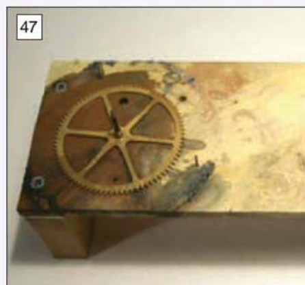
47 Polishing the escape wheel assembly on a special, raised board.
