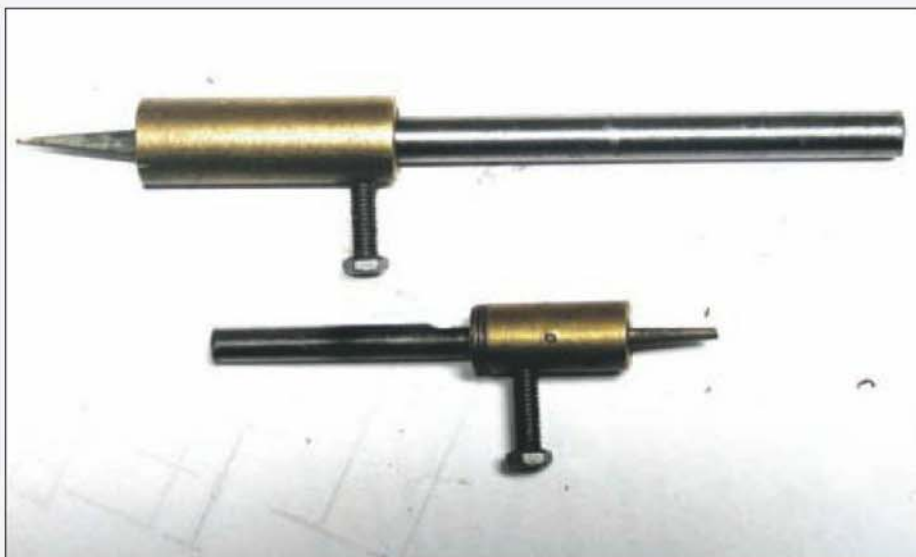
Two injector reamers fitted with collars to maintain the correct depth of penetration in the cone.
