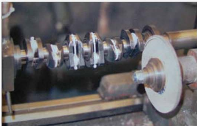
The bearing surfaces of the crankshaft were finished ground using a tool post grinder on the lathe.
