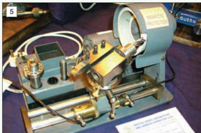
5 The neat Colyer/Caseley tool and cutter grinder attracted the attention of many visitors.
