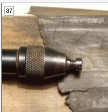
Here the screw is held in a pin chuck so the head can be polished.
