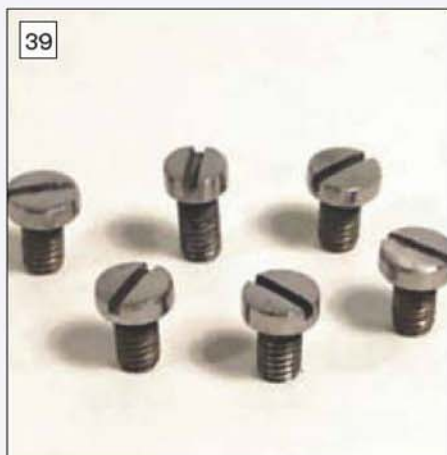
A selection of screws with their heads polished and ready for assembly.
