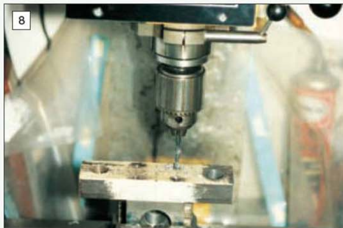
Spotting the ram mounting bar holes into the ram mounting block using the mounting bar itself as a drill jig.
