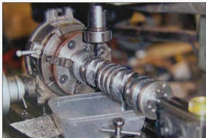
The crankshaft was made from EN24B steel using a combination of turning and milling techniques.
