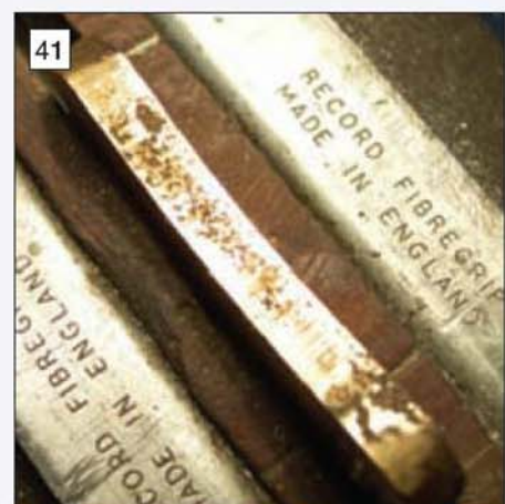
Polishing the mainspring arbor supports. Some filing was necessary to remove the cast surface.
