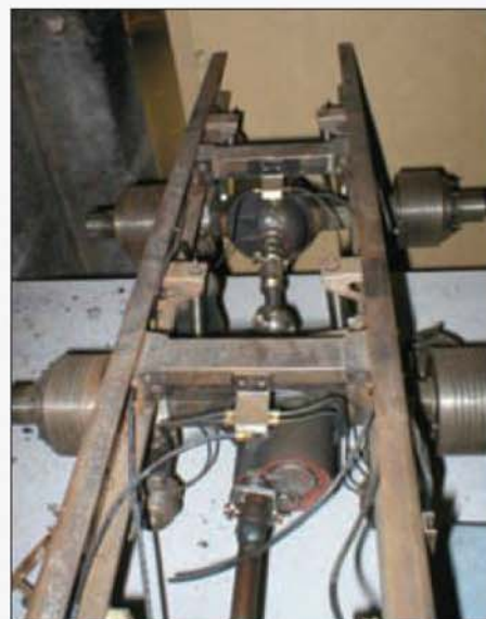
A view of the vehicle's chassis showing the rear axle and drive arrangements.
