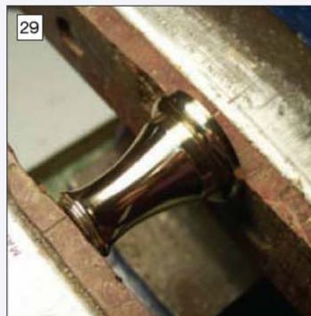
A foot after being polished. Progressively finer grades of emery cloth are used then metal polish.
