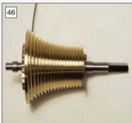
46 The fusee was well machined but the grooves were polished.
