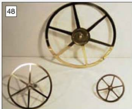
48 The great wheel, centre wheel and escape wheel after polishing.
