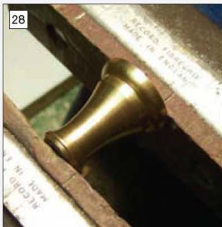
The feet were held between soft jaws in the bench vice for polishing.
