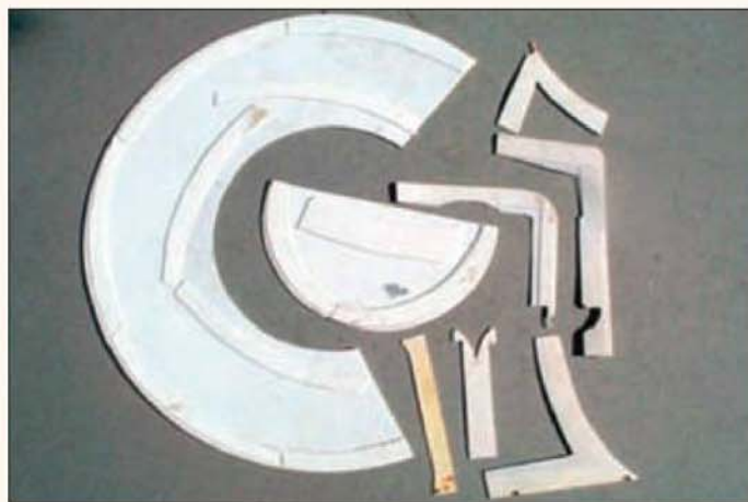
Further examples of lining templates. It is recommended that these templates are cut from Plasticard.
