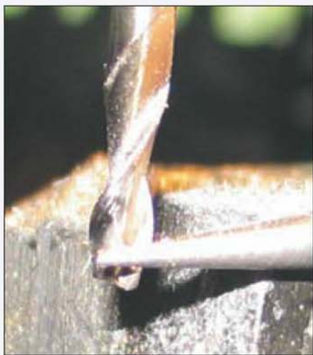
Milling the side of the tapered reamer to achieve the D-section. Care is needed to avoid damaging the work.
