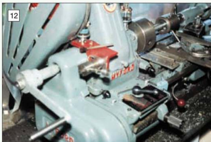
Cutting the threads on the pillars using the tailstock die holder and lathe mandrel handle.
