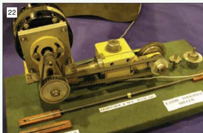
22 Maurice Turnbull's tool post milling device with examples of threads milled in the foreground.
