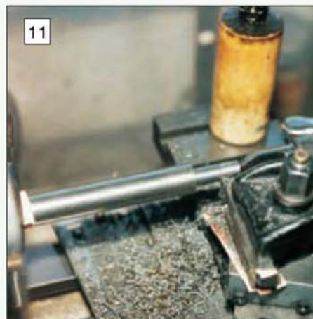
The pillars were turned between centre to give good concentricity and parallelism.
