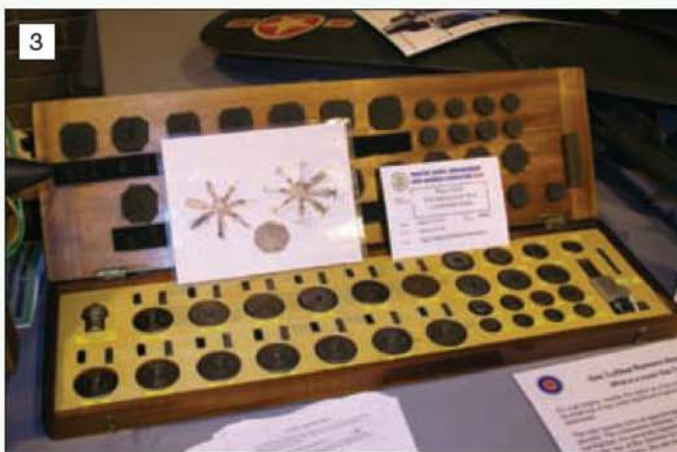
3 Some press tooling used by James Hill of the Gas Turbine Builders Association to make axial flow compressor blades.
