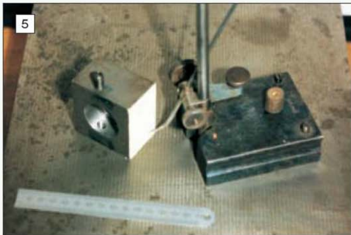
Marking out the ram mounting bracket on the surface plate using a surface gauge. Note the cork to protect the scriber points and prevent injury.
