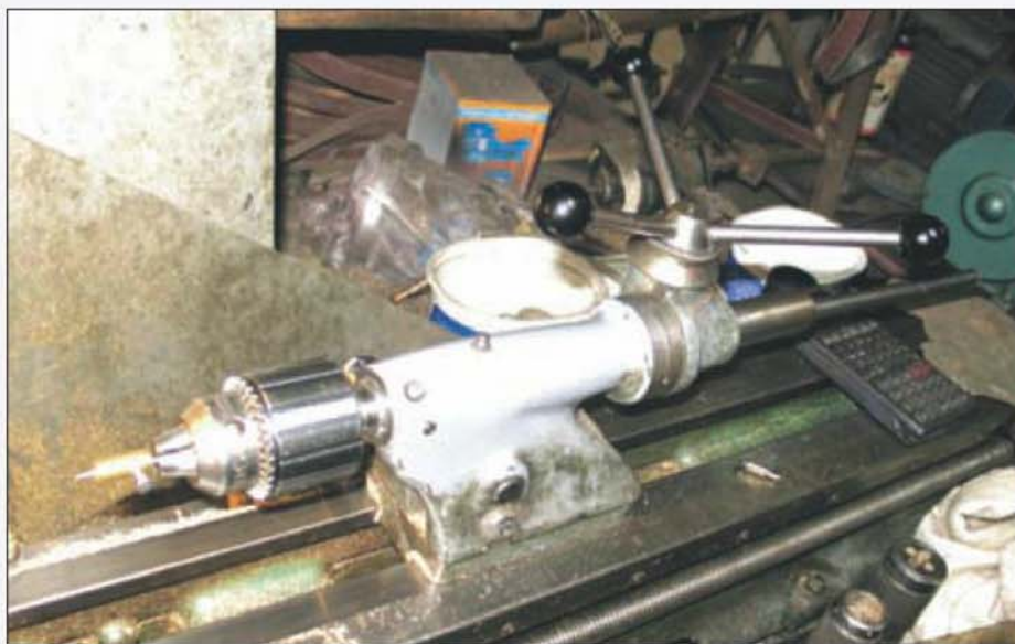
Drilling and reaming are speeded up if your tailstock is fitted with a capstan feed device.
