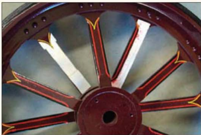
An example of the lining applied to one of the author's model traction engine wheels. Note how the templates described in the text are used.
