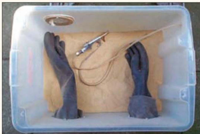
A view inside the grit blasting unit showing the rubber gloves used to hold the work, the grit and nozzle.
