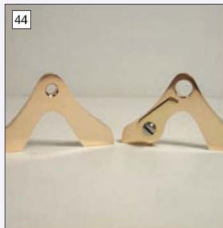
44 The finished arbor supports. The front one shows the polished click and screw.
