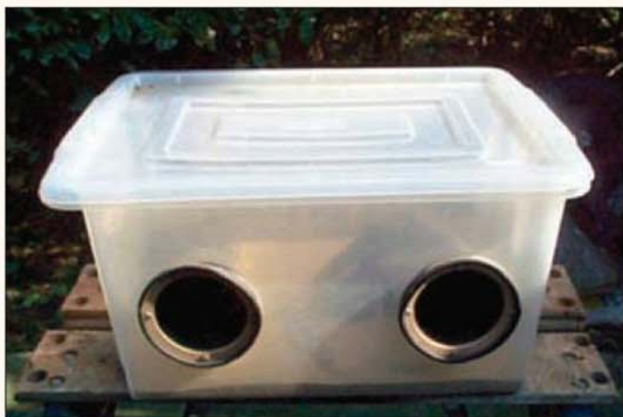
A small grit blasting unit made to the design of a friend of the author and utilising a plastic storage container.
