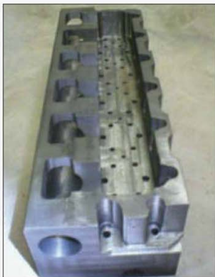
The complex cylinder head was machined from solid, continuously cast iron.
