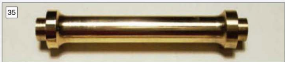
A finished pillar. It important to be patient when polishing and not try to rush the process.
