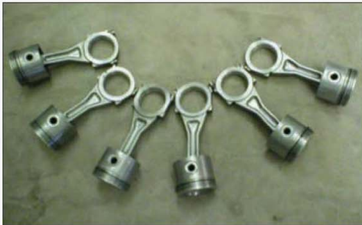
The set of pistons and connecting rods prepared for the engine. The model's pistons were machined from material cut from full size pistons.
