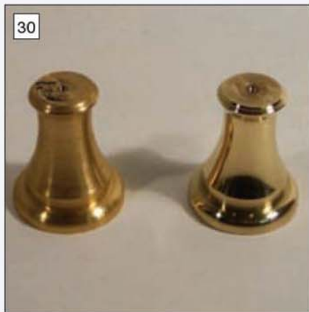
Spot the difference? The machined finish on the foot is good but is improved by polishing.
