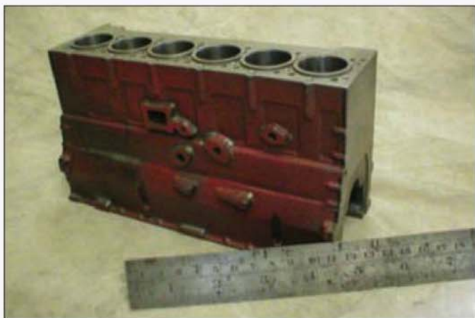
The engine cylinder block was cast from home made patterns. It is of the wet liner type.
