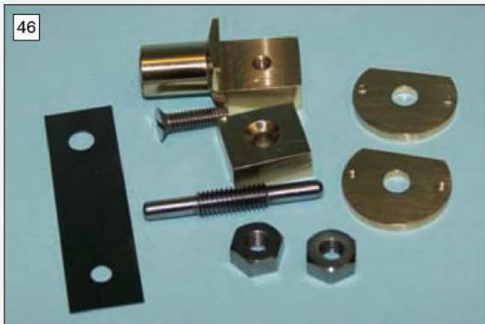
The pendulum suspension parts dismantled. The suspension spring is the object on the left.
