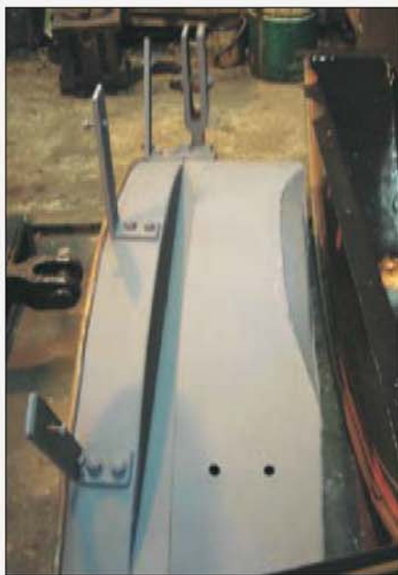
Another view of the 'Castle' splasher. Note the reach rod steady and indentation.
