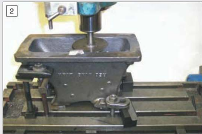
2 Using a slitting saw to remove the risers from the underside of the main engine base.
