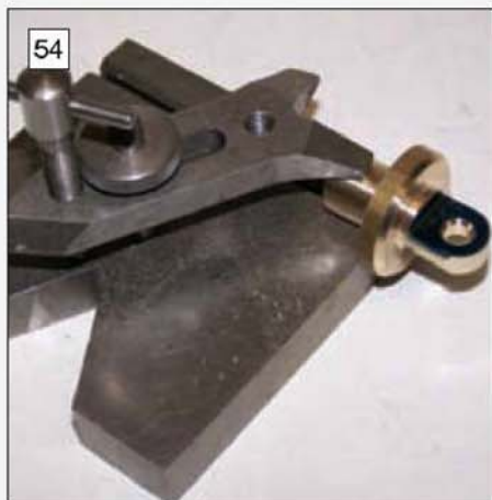
54 The holes for the weight hook should be well chamfered both sides.
