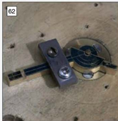
62 Method of clamping the pallet arms to a wooden faceplate.
