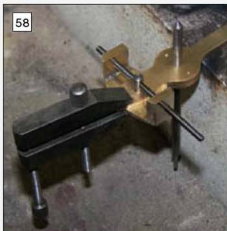
58 The set-up for soldering the extensions to the yoke piece.
