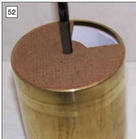
52 The set-up used for pouring the lead. A piece of hardboard with a window cut in it was used.
