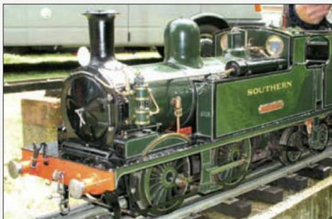
Superbly finished Southern Railway O2 class, 0-4-4T by John Gates from Sutton MEC.
