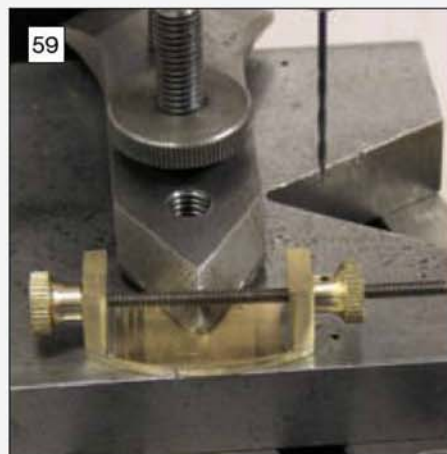
59 Set-up for drilling the pin hole through the knurled screw and threaded rod.
