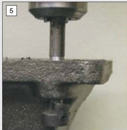
Spot-facing the holes for bolting the engine down on its mounting surface.
