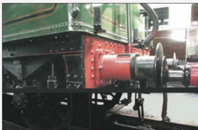
A close up view of the Collett buffers and rear steps fitted on a 3,500gal. tender.
