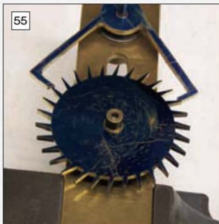
55 A pair of trial pallets should be made from soft material in order to test the action.
