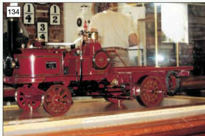
The other side of the model which is based on a 1904 prototype so the engine and change speed gearing are two separate units.
