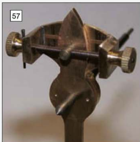
57 The ingenious beat setting arrangement uses a leadscrew with both 10 and 14BA threads.
