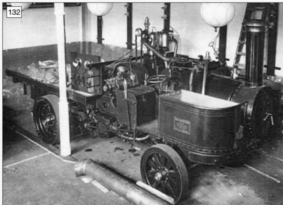
An early OA, A or A1 class Savage wagon fitted with a locomotive boiler and complete with a generator set for showman's use. It has been suggested elsewhere that the engine for the 110V generator is a duplicate of the one already fitted. We suspect this is true for the most part, but doubt if there is any need for it to be reversible. Note the Little Samson chimney cap and curved spoke steering wheel.
