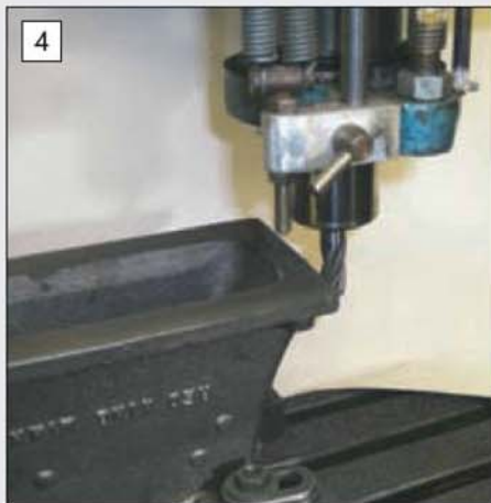
Using an end mill to clean up the edges of the flange on the main engine base.
