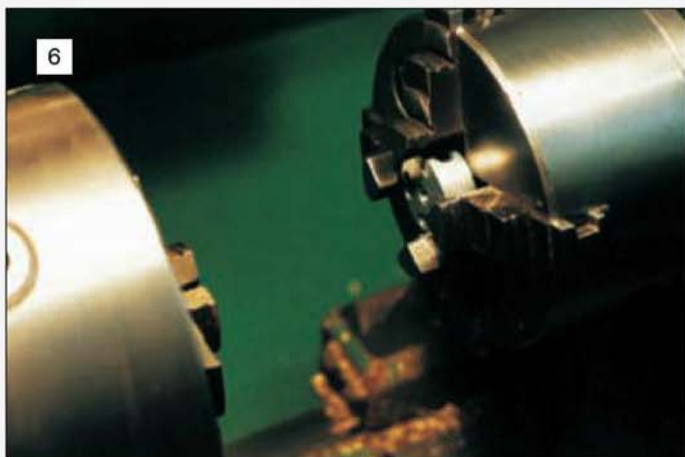
Setting up the flywheel in a dividing head facilitates machining the crank pin hole and those for the propeller shaft drive.
