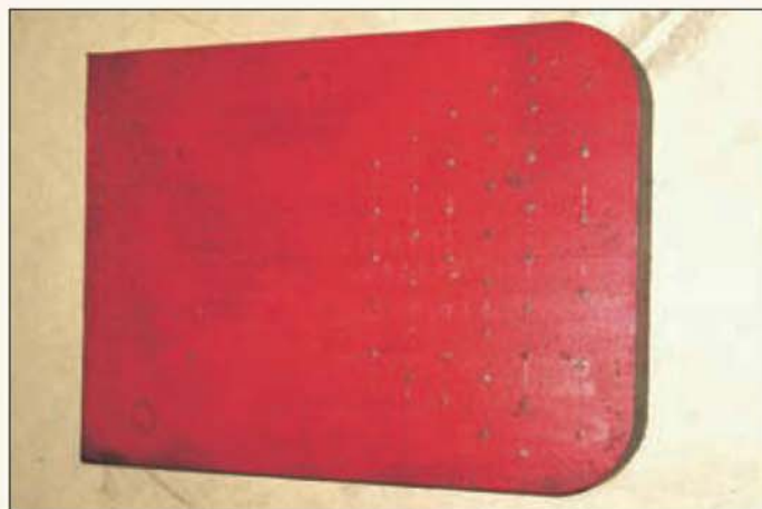
One of the substantial steel formers for flanging the various boiler parts. Heavy hammer work is required to make this boiler.
