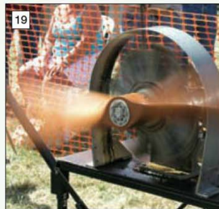
19 The fearsome 830cc nine cylinder rotary engine by Bill Connors seen cooling the crowd outside.
