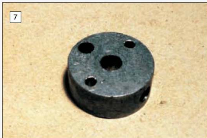
A close up view of the finished flywheel. The smaller, diametrically opposite holes are those for the propeller shaft drive.
