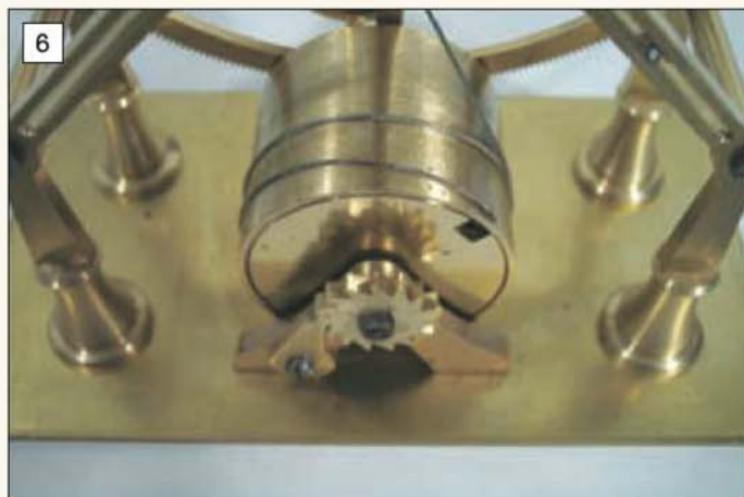
The design of this clock is such that the winding square does not protrude far through the frame and ratchet wheel.
