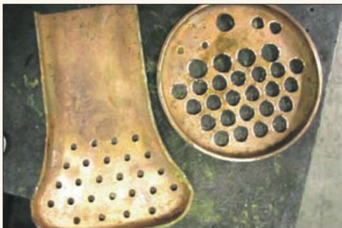
The drilling of the tube holes in boiler plates is best done in stages. Those on the right are now to size.
