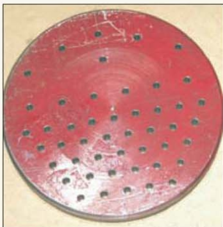
The boiler barrel front tube plate former is approximately 8 3 / 4 in. diameter.
