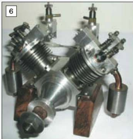
6 The V-twin design Vega four stroke glow plug engine.
