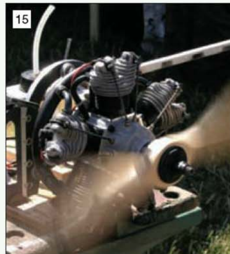
15 Another engine shown by Mike Tull, this time the very attractive five cylinder radial engine by Seidel.
