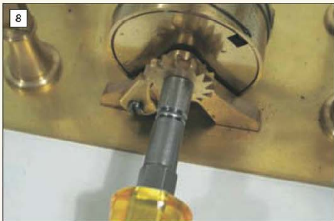
Here the letting down tool is in use. The ratchet click can be eased out of engagement and the arbor allowed to turn a few teeth at a time.
