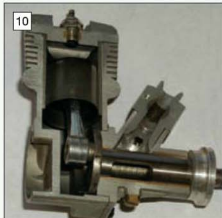
Sectioned two stroke engine displayed by Mike Tull.
