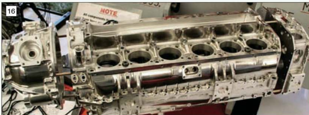
16 Superb part finished crankcase from the Napier Dagger engine being built by Norman Lawrence.
