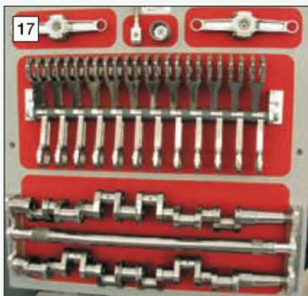
17 Crankshafts and connecting rods from Norman Lawrence's 24 cylinder Napier.
