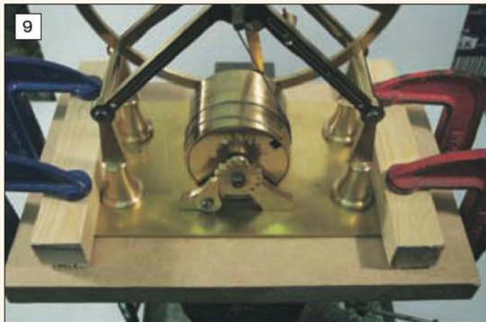
It is important that the clock is firmly clamped down for the letting down process or the movement may try to rotate around the mainspring arbor.
