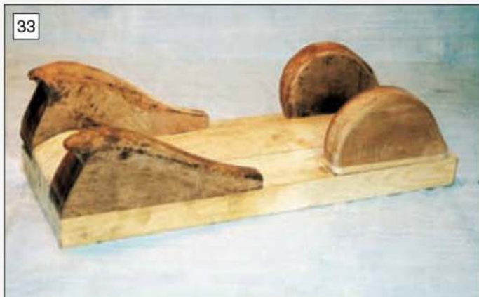
33 Wooden formers on a baseboard for working mudguards.
