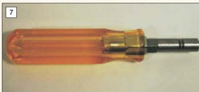
The tool used by clockmakers to safely let down powerful clock springs. Different sized arbors can be fitted to suit different winding squares.
