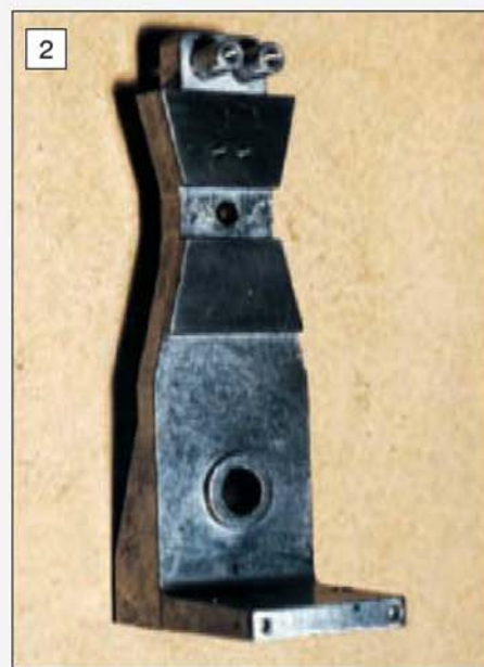
The main frame is a die casting and requires a minimum of machining.
