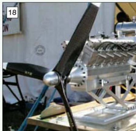
18 New engine from Ron Hankins, his own design V12 four stroke glow engine.
