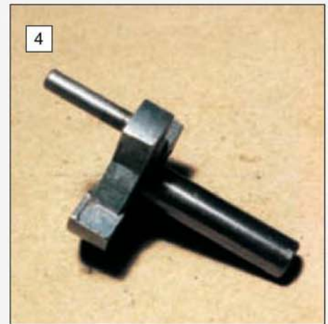
The crank comprises of an alloy casting with steel crankshaft and crank pin.
