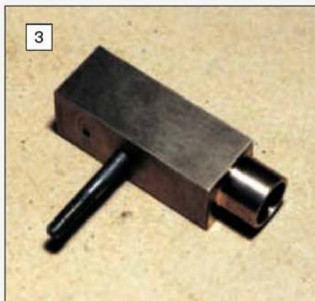
The completed cylinder and pivot sub-assembly. The bore needs to be finished with care.
