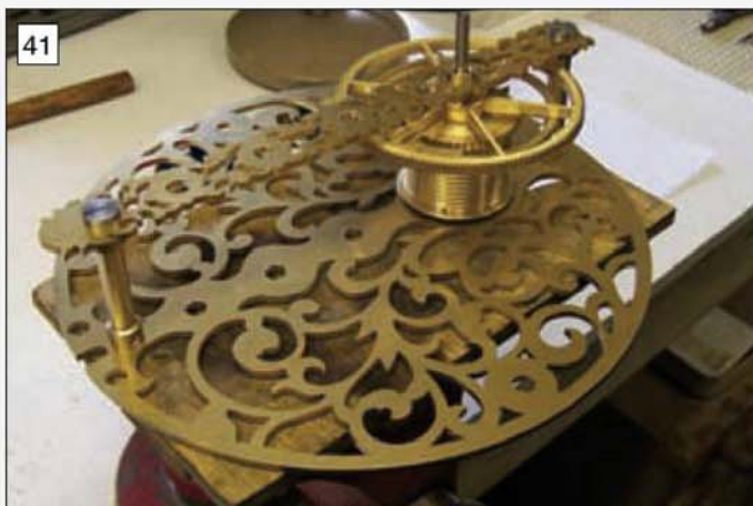
The main wheel assembly in position in the frames of the clock. The delicate ornamental piercing can be seen to good advantage.
