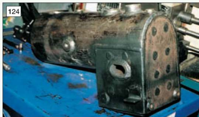
Another view of the finished locomotive boiler photographed on Stan Nippers work bench (photo: Stan Nipper).
