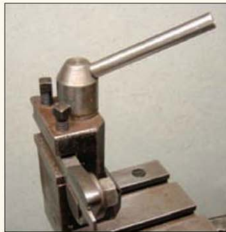
A great time saver - the special nut made for the Myford rear tool post.
