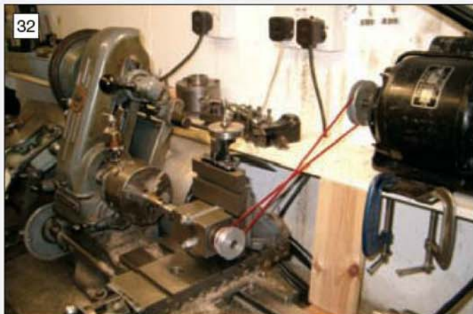
The arrangement used by the author in his workshop for drilling the lantern pinion bobbins.
