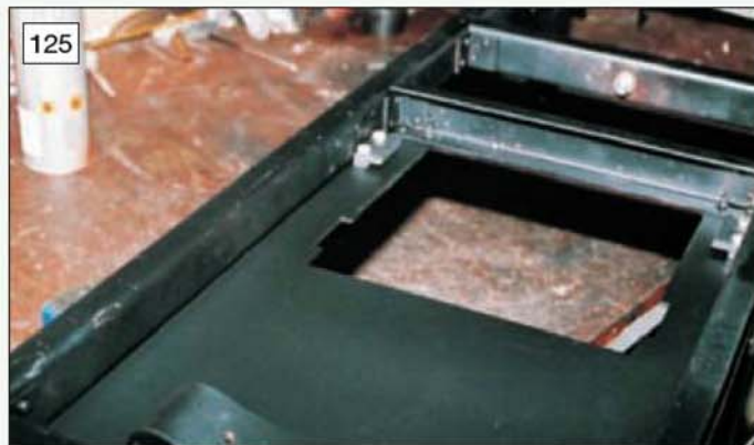
The boiler mounting plate is rivetted underneath the chassis frames. Note the rear boiler retaining keeps (photo: Stan Nipper).
