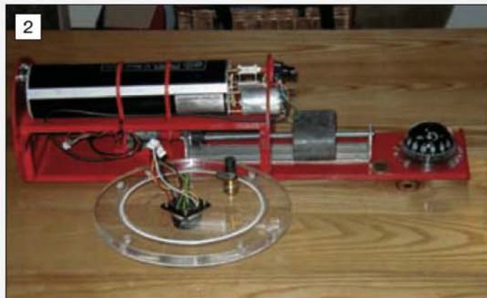
2 A side view of the chassis. The sliding lead weight that is used instead of hydroplanes can be seen right of centre.
