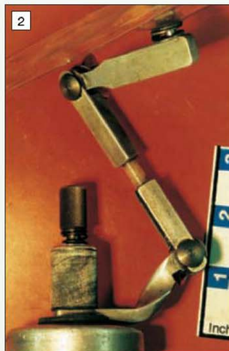
The neat stand devised to hold a plastic guard and place it close to the cutting area.
