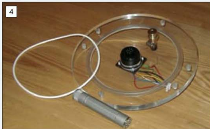
4 The control plug in the end bulkhead with its O-ring and the all important light (bottom left).
