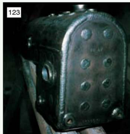
The backhead. The number BB87 is Bell Boilers reference number. The number at foundation ring level is again plate stamping (photo: Bell Boilers).
