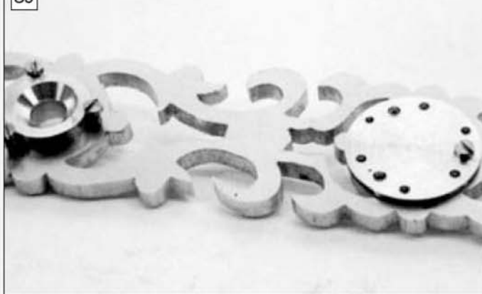
A simple jig was used to position the 10BA holes used to secure the bearing bushes in the front motion plate.
