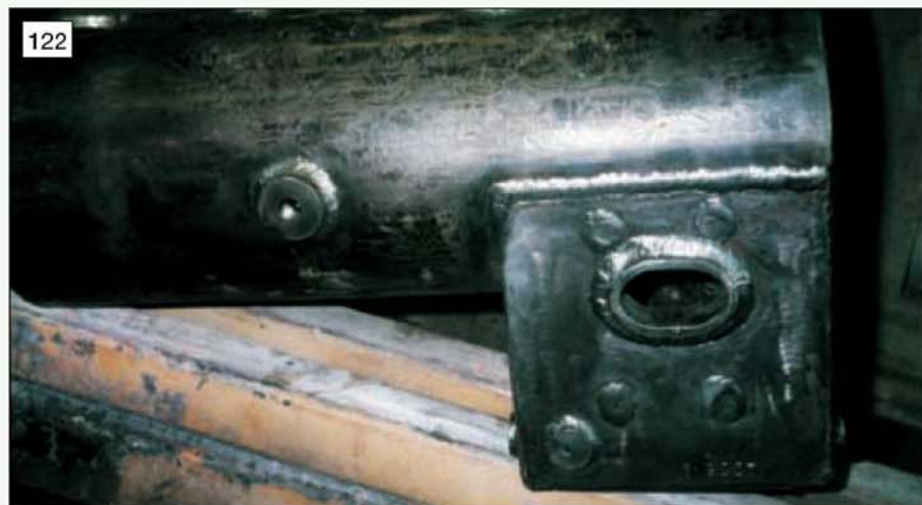
A model boiler. Note the vertical firing chute and the plate stamped at foundation ring level (photo: Bell Boilers).
