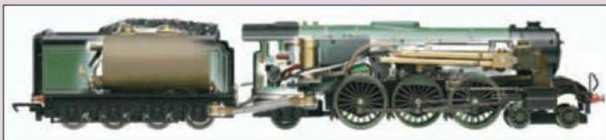
Live steam in 00 gauge: how it is organised in Flying Scotsman .
