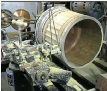
Here a bamboo pattern is being cut vertically on the main component of a Wassail Bowl; the wide flutes were also cut vertically.
