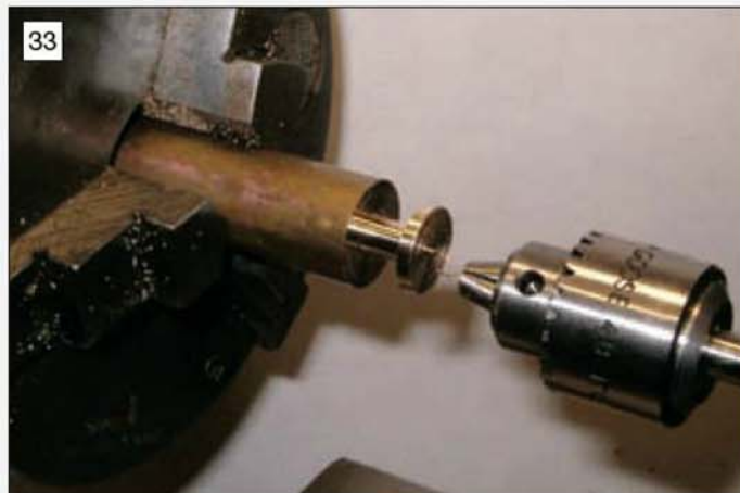
The drill has been retracted into the chuck here and is being used to drill the face nearest the drill chuck.
