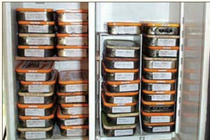
Tins used for the storage of nuts, bolts and other small parts should be clearly labelled as an aid to rapid identification of the contents.
