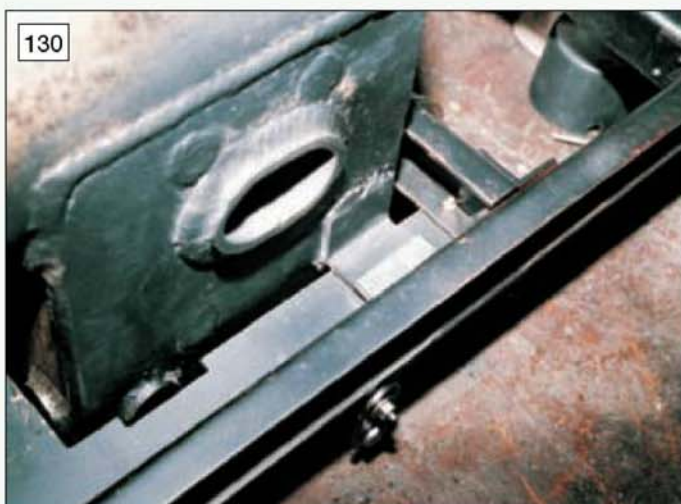
130 A rear boiler mounting. The bracket can slide under the retaining keeps (photo: Stan Nipper).
