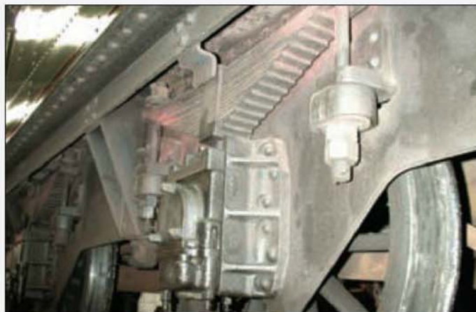
An example of a late type spring and axlebox assembly showing the flat fronted shock absorber.
