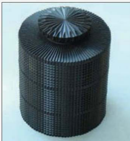
The patterns on these boxes were cut with the Horizontal Cutting Frame; one using a round-nosed cutter and the other a point tool.
