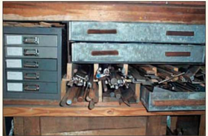
The method used to store steel stock and similar larger items. Being systematic and tidy in the workshop saves time.
