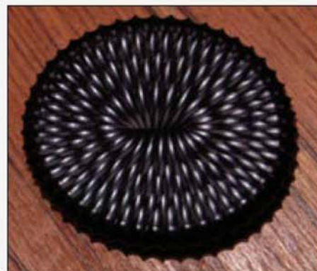
The patterns on these boxes were cut with the Horizontal Cutting Frame; one using a round-nosed cutter and the other a point tool.
