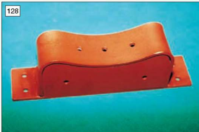
128 The assembled front boiler mount after a coat of undercoat (photo: Stan Nipper)
