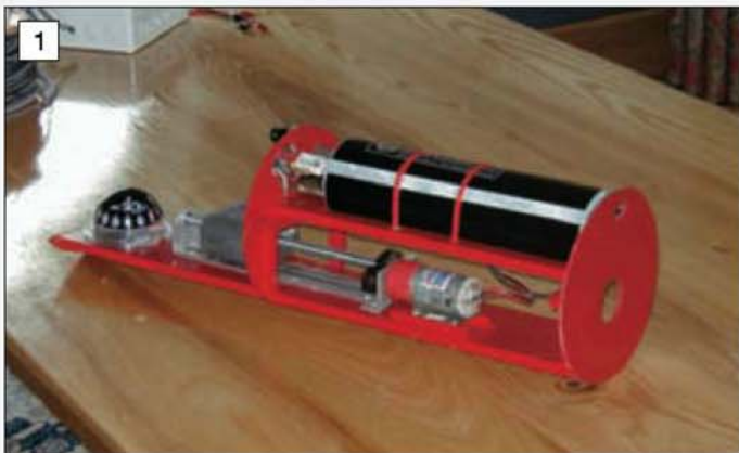
1 A view of the submarine chassis before enclosure in the Perspex tube hull. The ballast tank can be seen at the top of the structure.
