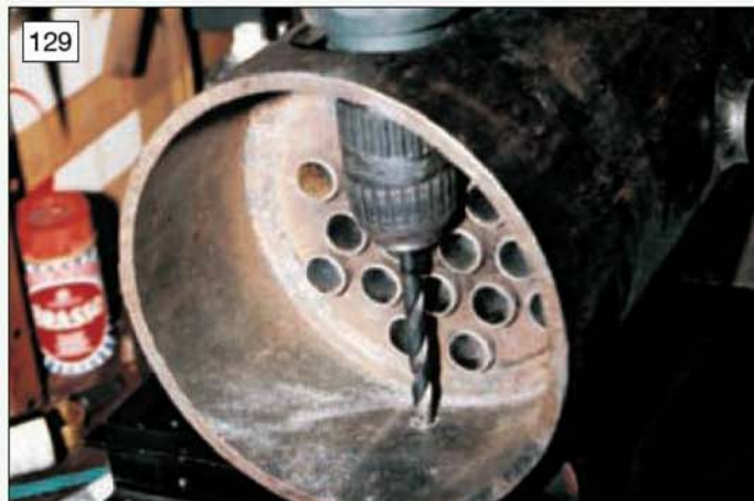
129 Spotting the front boiler fixing bolt holes through to the mounting bracket (photo: Stan Nipper).
