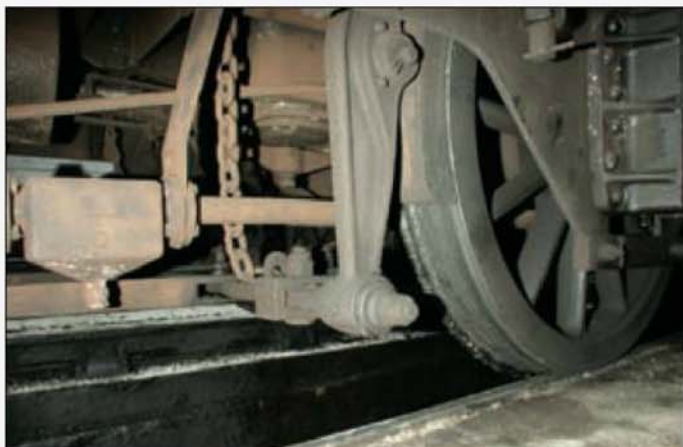
This photo shows details of the brake hanger. Note that all the nuts and retaining pins are split pinned.
