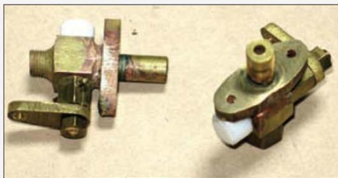
A pair of draincocks with PTFE valve members. Stainless steel would be a suitable alternative.
