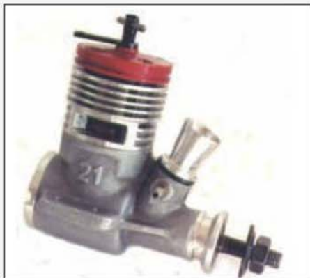
The earlier Dynamic 21D produced using a crankcase casting.
