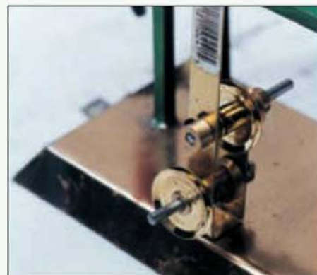
Pulley frame with the pulleys temporarily assembled to find the best alignment for the belts. This is best done by trial and error.
