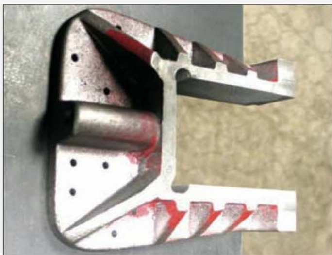
A view of a hornblock laid in position in the frame. Some notes on machining these appear in M.E. 4249, 10 June 2005.
