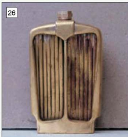
Completed radiator front with bars.
