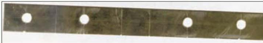
The pulley frame marked and drilled before bending.
