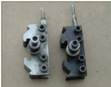
Two lathe tools for working in holes as small as \frac{3}{16} in. diameter. Screw cutting tool is on right.
