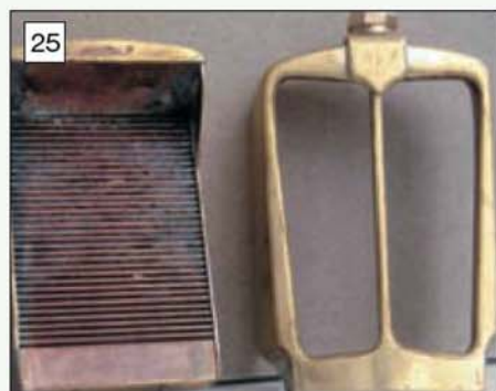
Inside of radiator and completed front.
