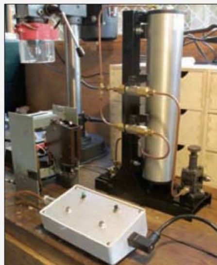
The test rig includes a regulating valve, reservoir, distribution manifold, and electrical console.
