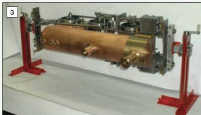
Once locked into position the locomotive can be orientated to give access to which ever feature is required.
