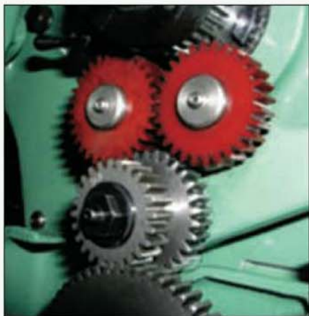
Tufnol tumbler reverse gears in use on a Myford Super 7 lathe.
