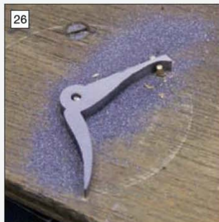
26 Using the sawing board and clock pins to locate the barrel ratchet for filing to width.
