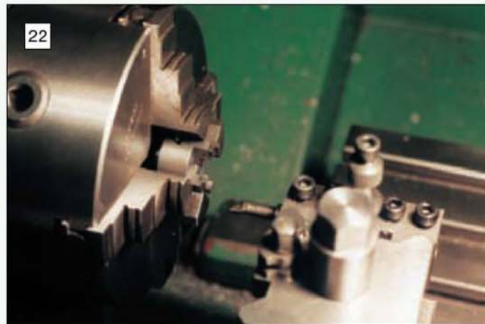
Turning the steps in the jaws of the miniature chuck using a small boring tool. The work is held in a self-centring 4-jaw chuck.
