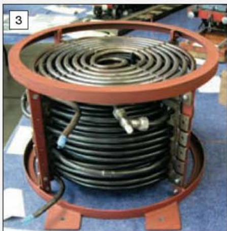
3 D. Beale's monotube boiler intended for a steam car and seen on the Leeds SMEE stand.
