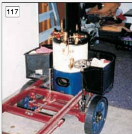
117 View of the nearly finished boiler in the chassis (photo: John Thompson).
