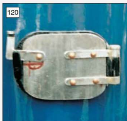
120 View of the hinged fire hole door (photo: Martin Wallis).
