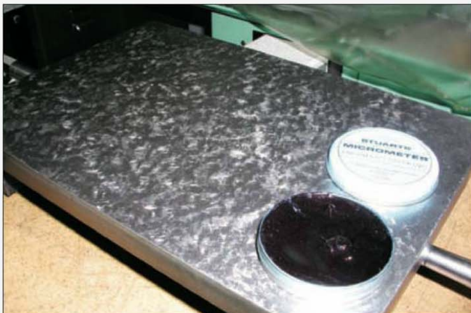
A scraped surface plate is valuable in precision engineering. A piece of plate glass is a good substitute for the amateur.
