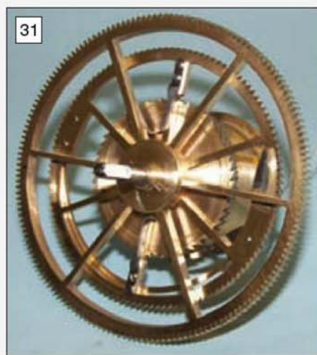
31 The completed barrel assembly viewed from the front.
