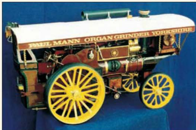
The author's 1\frac{1}{2} in. to the foot Fowler 'Big Lion' showman's engine built from Bill Hughes' drawings.
