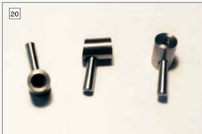
Three locking levers are used on the machine, one on the saddle, one on the tailstock barrel and one on the tool post.
