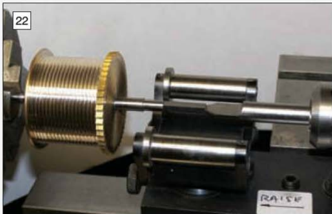
Forming the barrel square using the lathe filing rest. Note the slight taper produced on the square section.
