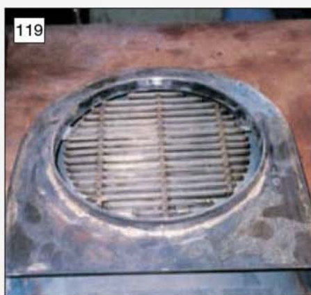
119 Stainless steel circular grate (photo: John Thompson).
