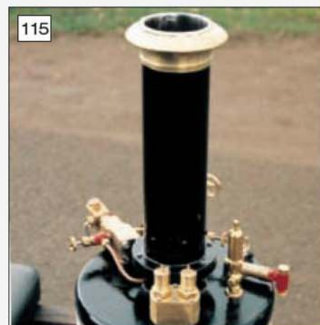
Finished, painted cap in position on the lagged boiler (photo: Martin Wallis).
