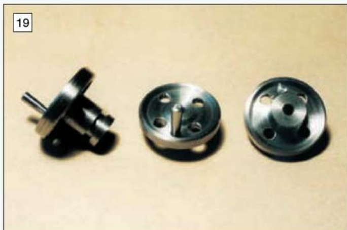
The tailstock spindle handwheel and the handwheels for the saddle and cross-slide actuation.
