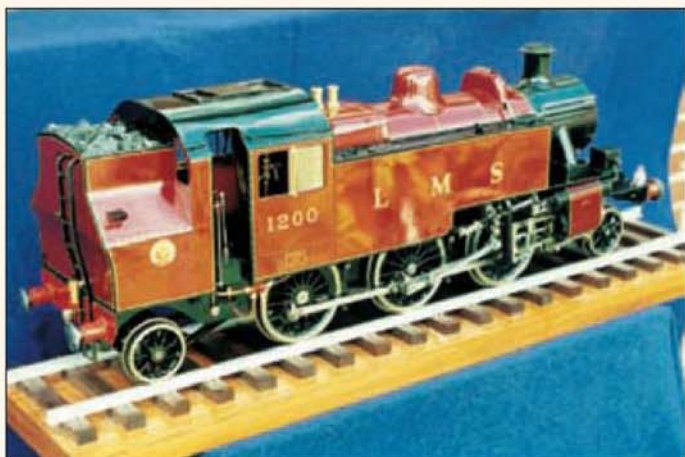
The author's 5in. gauge LMS Class 1200 'Ivatt' tank engine. It was built to Don Young's and the LMS works drawings and was completed in 1995.
