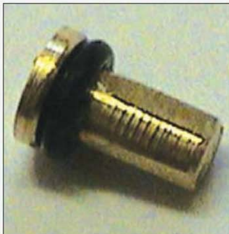
The clack valve shuttle fitted with its O-ring. Note the flats on the minor diameter.
