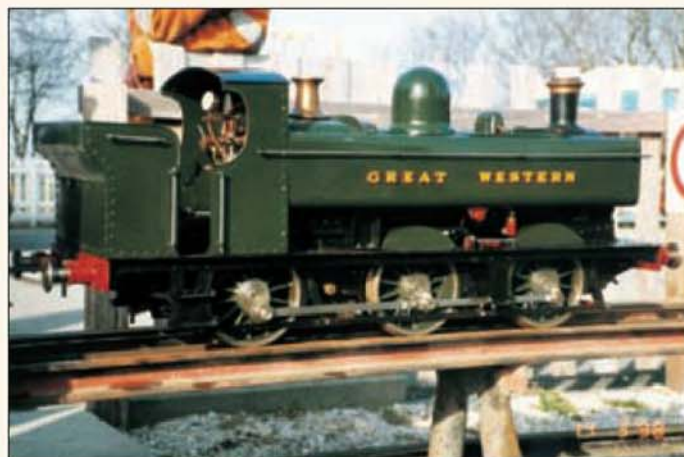
Friend John's 5in. gauge Pansy built to the design of LBSC. It was this locomotive which suffered from injector problems.
