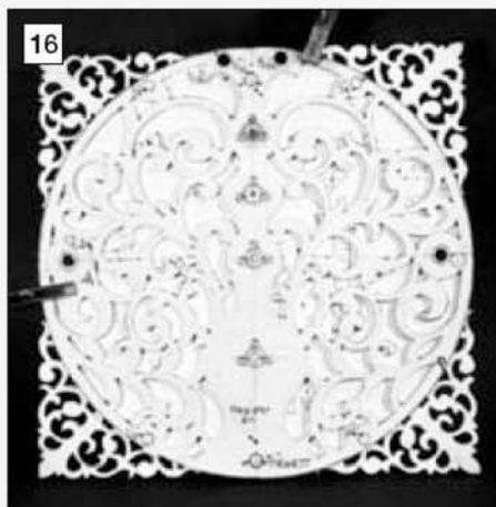
Both back plates are clamped together for drilling the four pillar holes common to both.
