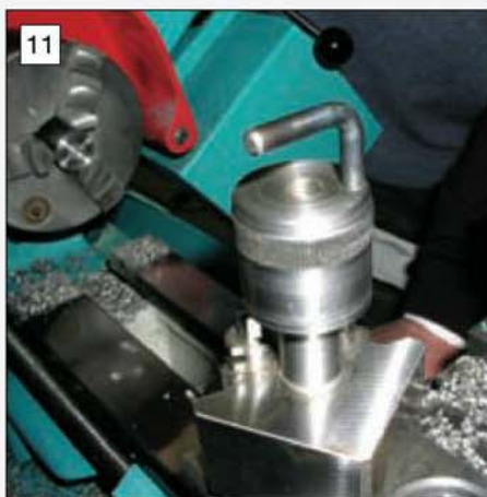
Tony Phillips' (SMEE) neat hydraulically locked nut seen in use on a Myford lathe.
