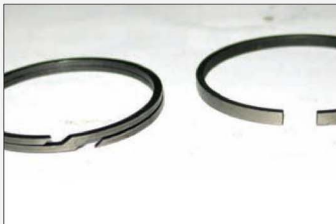
A Clupet ring (left) compared to a standard ring. Clupet rings are available directly from the makers.
