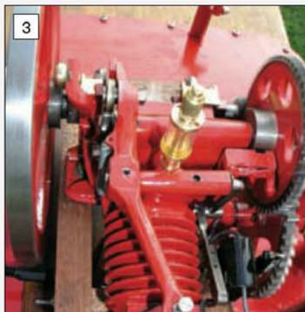
3 A top view showing the exhaust valve operating lever and cylinder lubricator.
