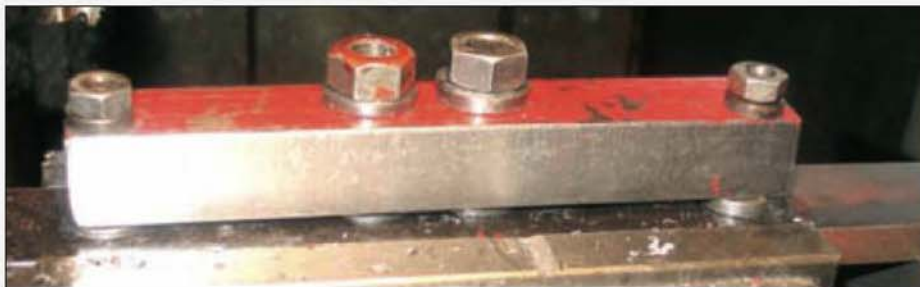
The method used to support the material for the front spring hooks to facilitate machining on the milling machine.
