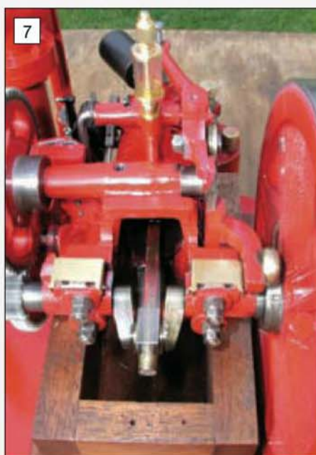
7 The big-end and crankshaft bearings. Just inside of the flywheel is the 'hit and miss' drive.
