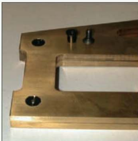
Two clock plates fastened together with the alignment bushes.
