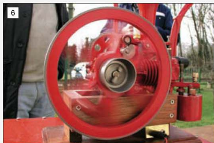
6 A view of the engine running seen from the flywheel side. A heavy flywheel is necessary to accommodate the eight-stroke cycle.
