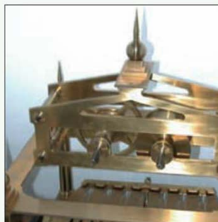
The cover washers on the pillars of this Congreve clock cover the bush countersinks.
