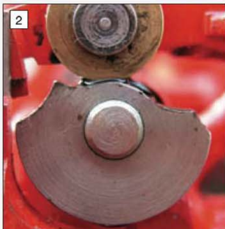
2 The unusual cam and roller follower used to give eight-stroke operation.
