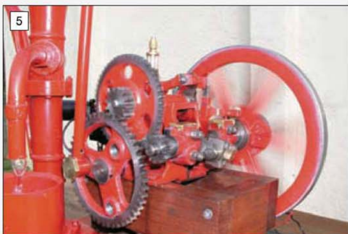
5 A view of the engine running showing the 4:1 timing gears and the pump drive arrangements.
