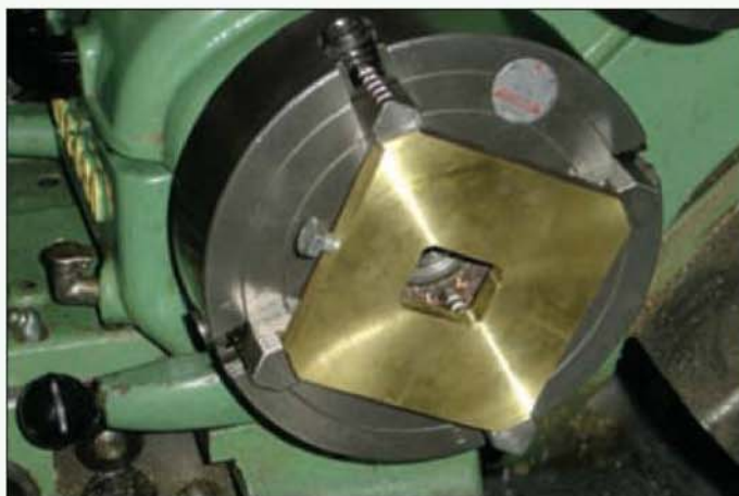
The method finally used by our contributor to correctly position the holes in the split rod brasses.
