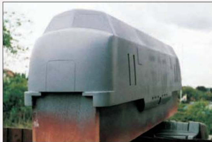
A nearly finished wooden pattern for the body work of a German V200. The bodies will be moulded in fibreglass.
