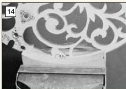
14 Curved wooden vice chops were used to hold the circular weight pulley disc for filing.
