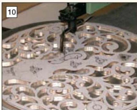
10 Cutting the intricate back plate on the Rexon fretsaw machine.
