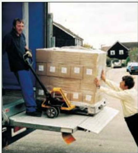
The first pallet is carefully unloaded using a pallet truck and the truck's hydraulic tailgate.
