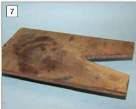
This normal size sawing board (9in. x 6in.) is really too small for the plates of this clock.
