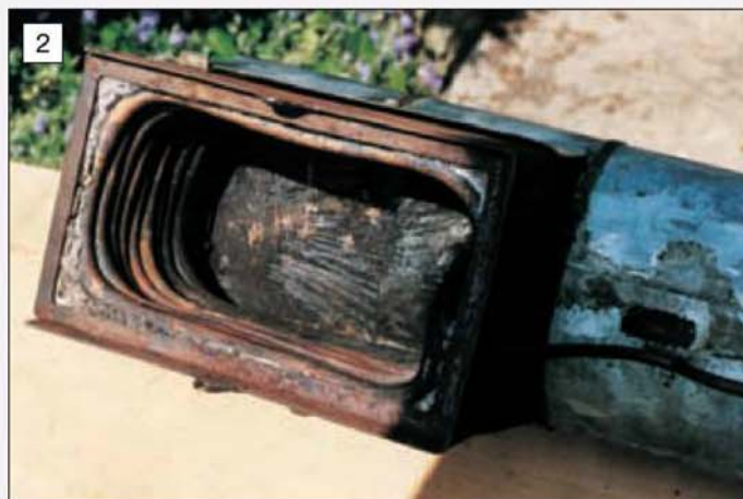
...a firebox comprising water tubes
