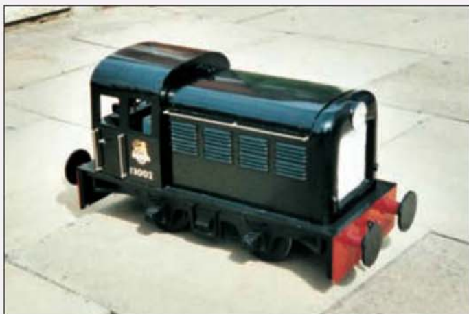
A small 0-4-0 shunter built for approximately £200. Power is provided by a 12 Volt battery housed in the nose.
