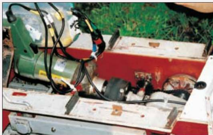
A budget traction unit built up around a 12 Volt cordless electric drill and a German chassis.
