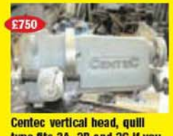
Centec vertical head, quill type fits 2A, 2B and 2C if you have the adapter
