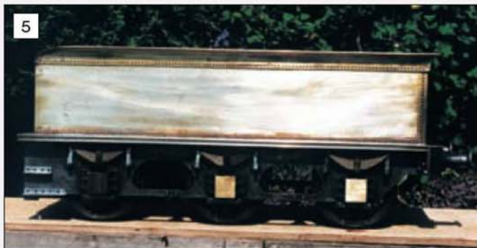
Flared top edges were made from brass tube
