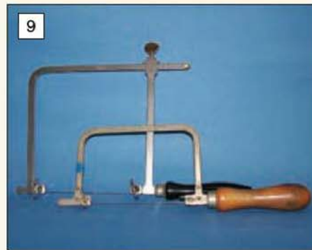
Two piercing saw frames. The larger has a 6in. throat clearance.
