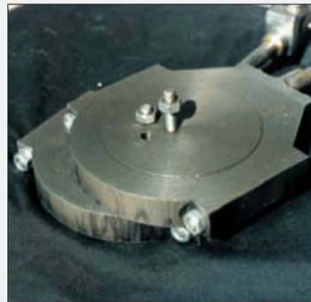
The finished eccentric straps machined from cast iron bar.
