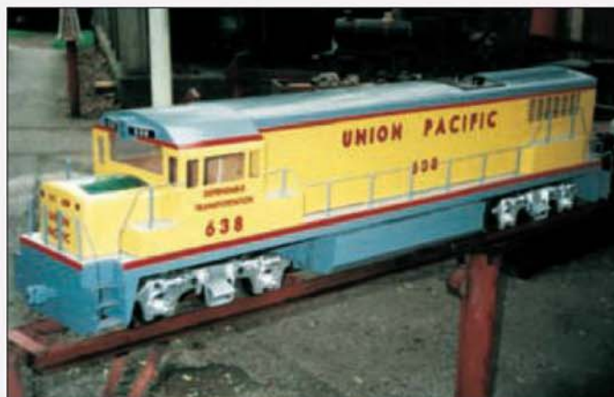
A scratchbuilt U25B made by J. Campbell. Power is via 2 off 200 Watt, 12 Volt motors.
