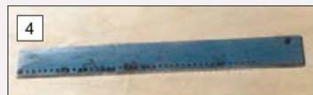
Drill jig for accurate rivet holes
