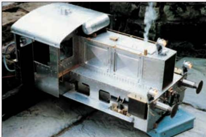
Kit built K6f II locomotive with lights, smoke and sound. It is built from CNC machined aluminium alloy.
