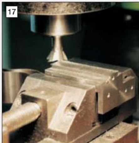
Machining the cross-slide dovetail on the saddle with a suitable milling cutter.
