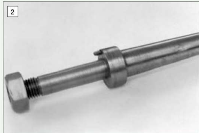
The Morse taper mandrel on which the finished hob is mounted and fitted into the spindle of the Dore Westbury milling machine.
