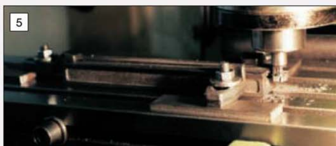
5 The Woodruff cutter just emerging from the end of the lathe bed after cutting the T-slot.
