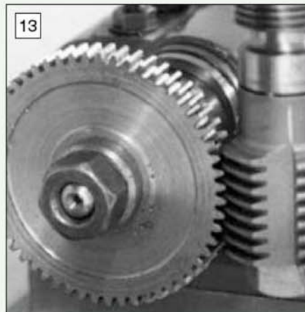
A gear being cut in the Dore Westbury. Indexing is via the G. Thomas dividing head.
