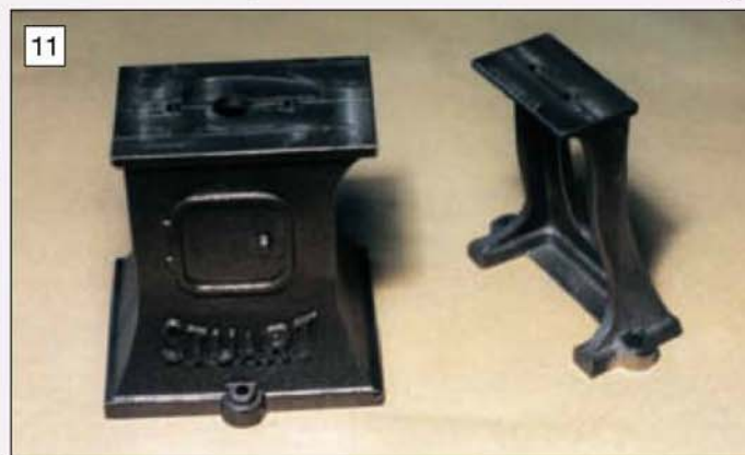
11 The headstock base and tailstock foot after the machining operations but before painting.
