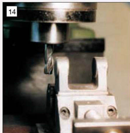
14 Cleaning up the faces of the headstock casting with an end mill.
