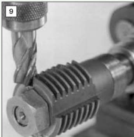
Close-up of the grooving operation. This aspect of making the hob is here seen nearing completion.
