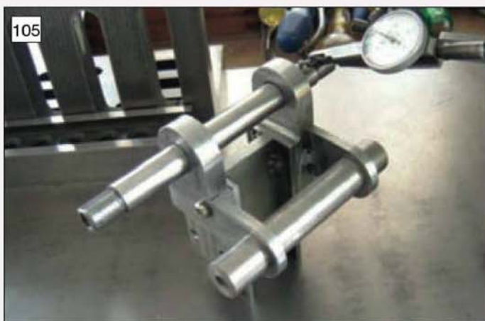
105 The mechanical aspects of the wagon have not been neglected. This picture shows the king pin bracket during assembly.
