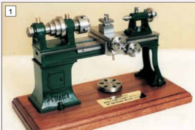
The finished lathe mounted on a neat wooden base. The chuck is fitted to the mandrel and the faceplate lays beneath the machine.
