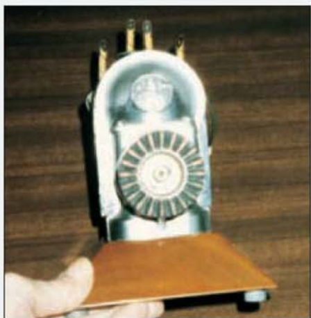
The author's BTH magneto, showing the toothed flange for the Vernier coupling on its spindle.
