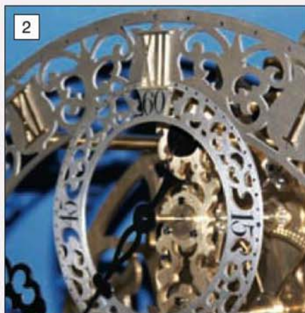
2 In this design the seconds ring is let into the main dial ring.
