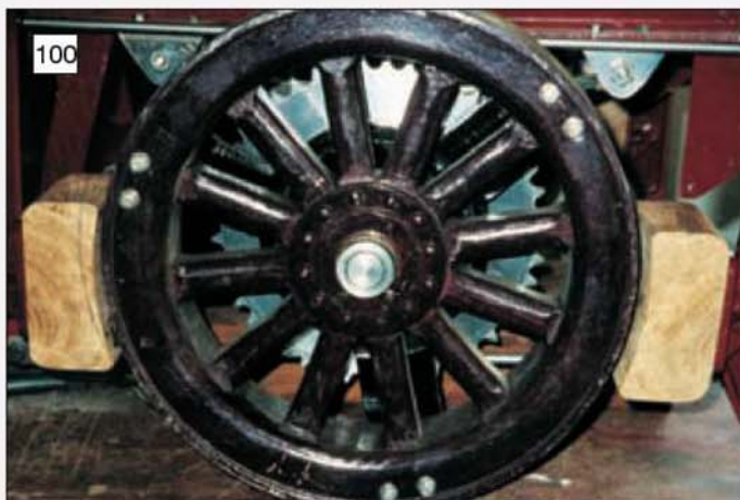
A set of completed brake blocks acting on an artillery style wheel. (Photo: John Thompson)
