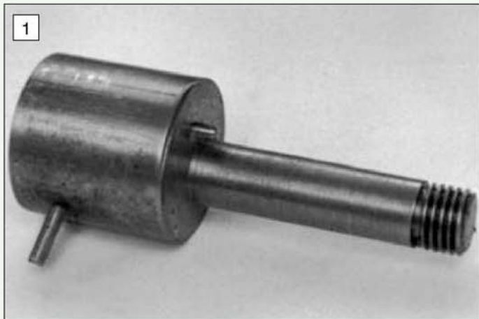
The eccentric mandrel used to form the four lobes in which the teeth were cut. Note the two pins for location purposes.
