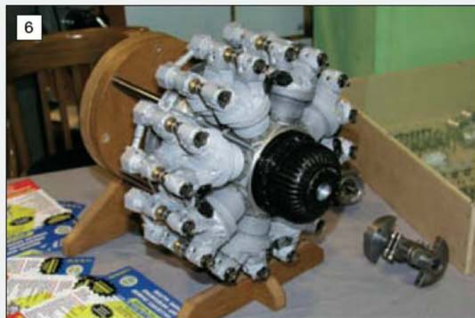
The remarkable Bristol Hydra double row radial engine by Brian Perkins enthralled many visitors.
