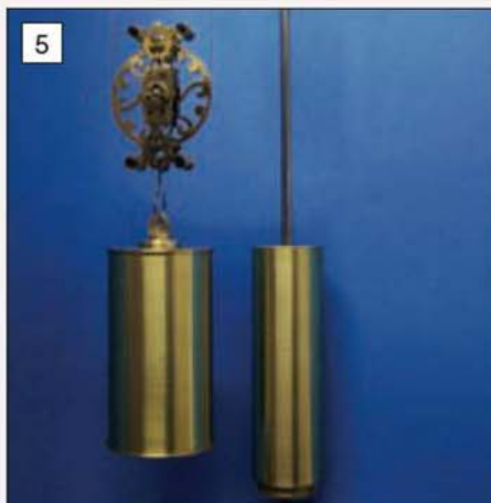
5 On the left can be seen the driving weight whilst on the right is the pendulum bob.
