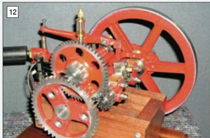
12 Also by Alan Thatcher was this unusual Aeromotor 8-stroke engine. The prototype was designed for driving water pumps.
