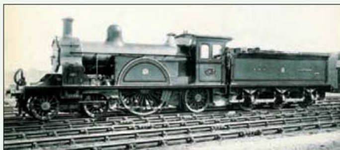
The older Worsdell preferred compounding and Joy valve gear for many classes.
