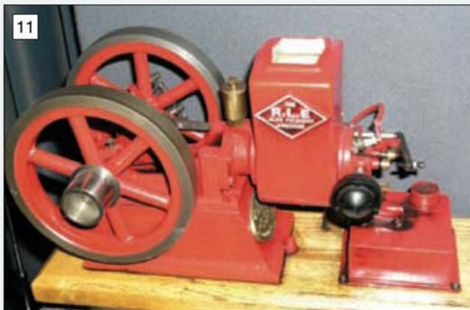
11 Alan Thatcher's handsome example of the well-known RLE engine had the correct three step timing cam.
