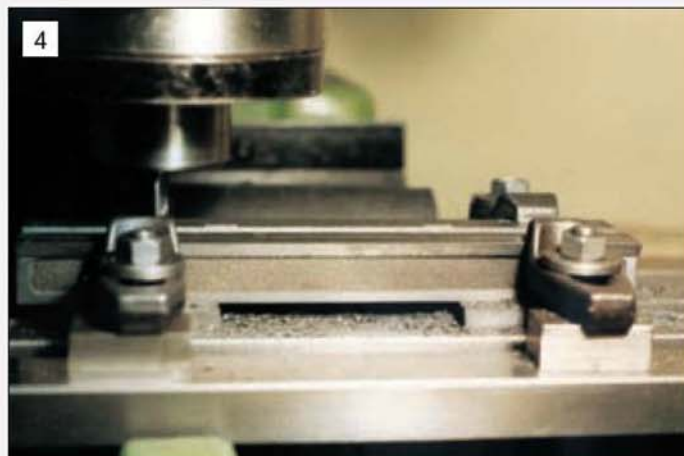
4 Machining the central slot down the middle of the lathe bed. Note the swan necked clamps to provide cutter clearance.
