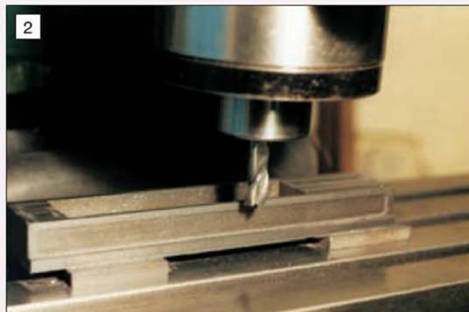
Milling the underside of the lathe bed on a vertical milling machine. Note that the method of clamping allows the whole bottom face to be machined.
