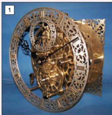
1 A general view of the movement. Note the piercing on the dial and motion plates.
