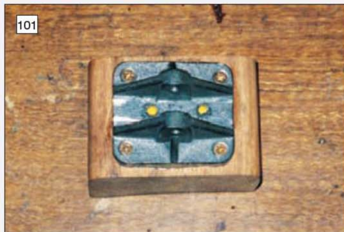
A brake shoe fitted to a brake block. Note the yellow screws referred to in the text. (Photo: John Thompson)
