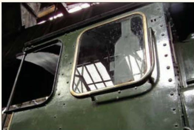
The cab side of the full size Cookham Manor showing the window and window frame arrangement.
