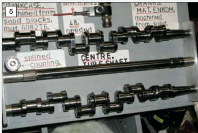
Some of the components machined for the Napier 'Dagger VIII' H24 engine under construction by Norman Lawrence.
