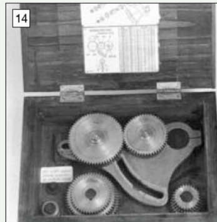
The finished metric gear cutting conversion set for the Myford Super 7B in its box.
