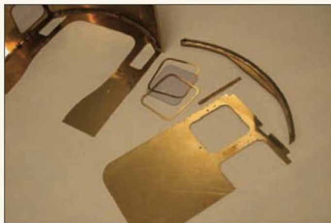
A view of some of the parts that go to make up the cab of the model prior to assembly.
