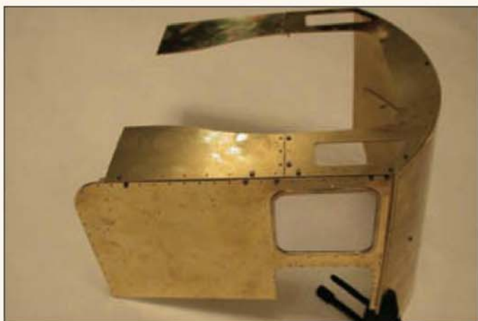
A trial assembly of the precision, cut parts for the Grange or Manor cab produced by Peter Thomas.
