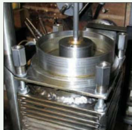
The cool end of the displacer cylinder showing the cooling fins.
