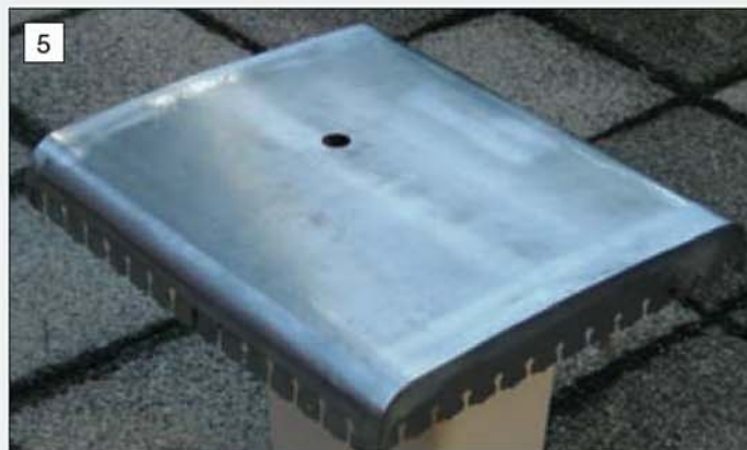
The finished canopy after welding and dressing.
