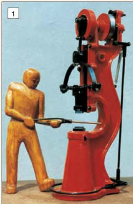
The completed spring hammer complete with miniature operator.
