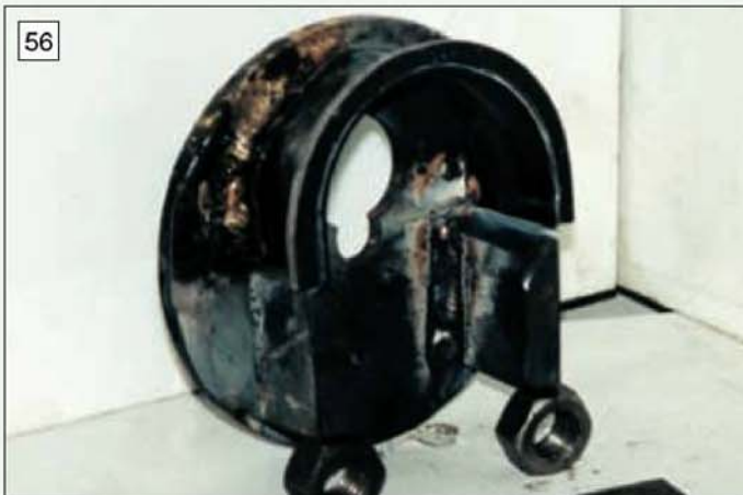
56 The housing for the rocking arm drive mechanism under construction using welding and brazing fabrication techniques.
