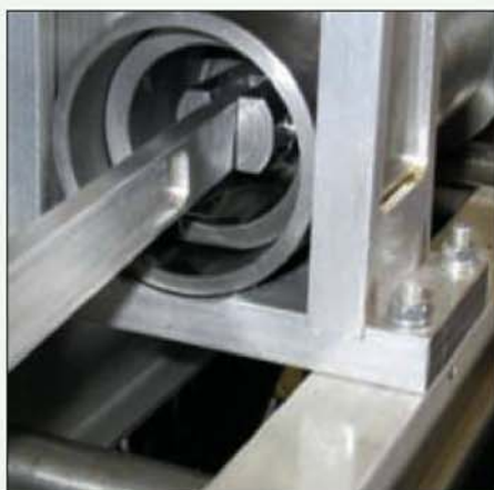
The power cylinder, piston and connecting rod. Note the A-frame construction.
