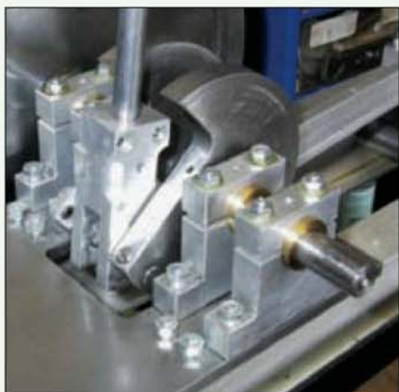
Detail view of the crankshaft and main bearings of the engine
