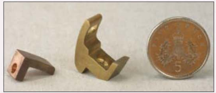
More details of the contact tip and lower arc horn showing the piercing of the latter to improve cooling.
