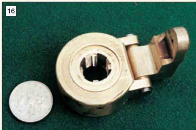
The breech ring with carrier frame and hinges shown with a 5 pence piece to give an idea of size.
