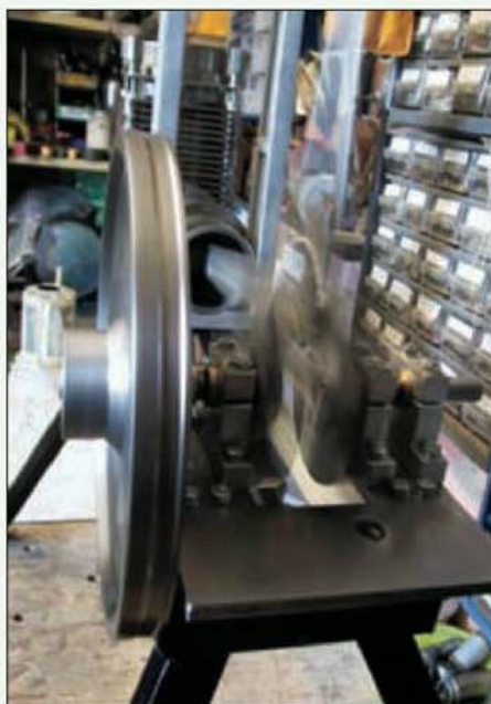
The flywheel is at present an old pulley and could be heavier.
