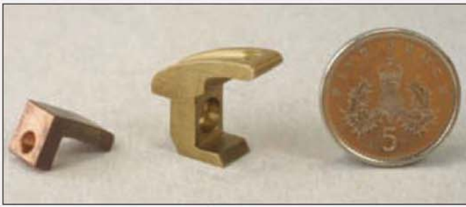
The main contact tip shown left alongside the lower arc horn. The lower arc horn is not fabricated but machined and filed out of brass section.
