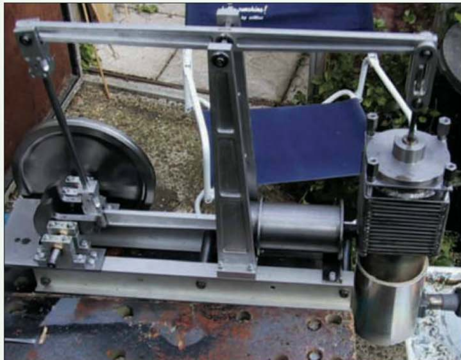
A view looking down on the engine showing some of the constructional details of the base. Firing is presently by gas torch.
