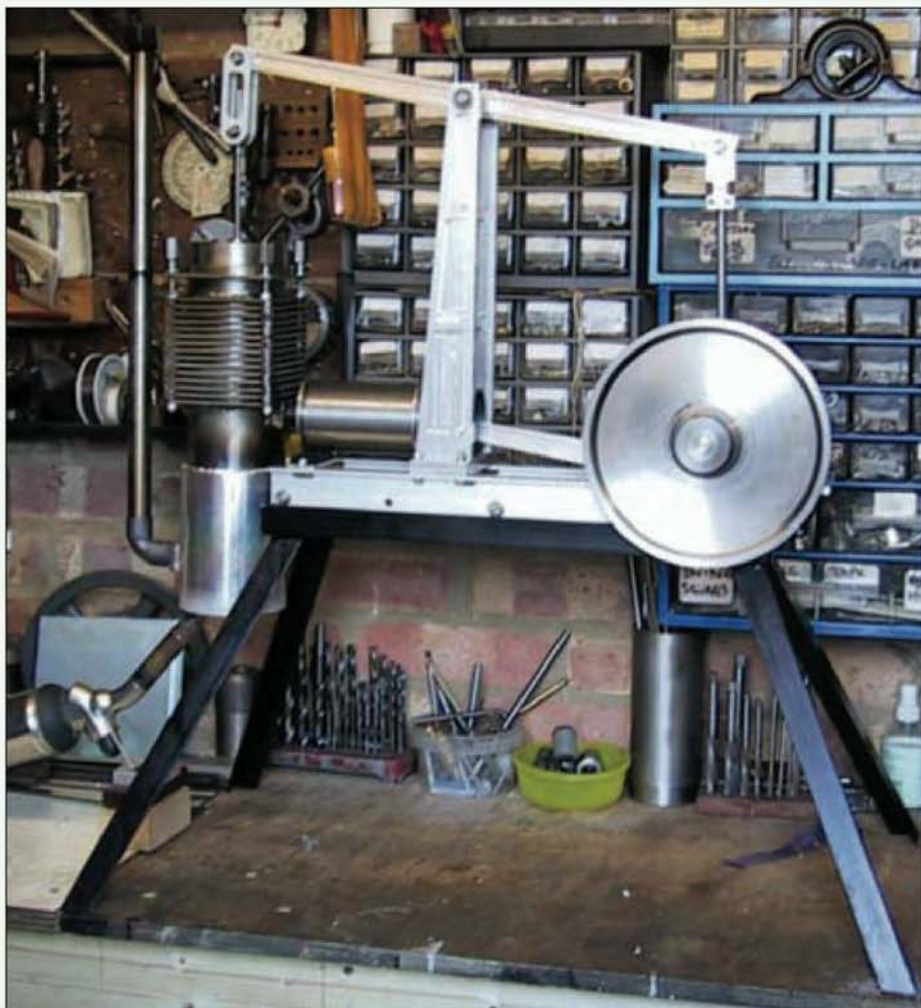
The impressive hot air engine designed and built by the author
