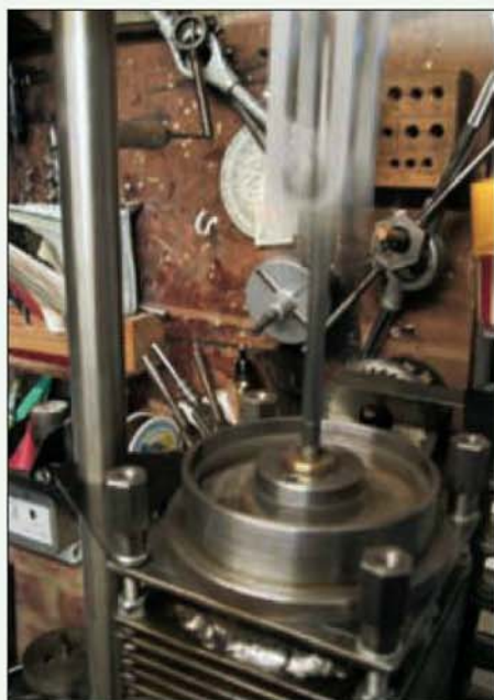
A view of the displacer cylinder with the engine running.
