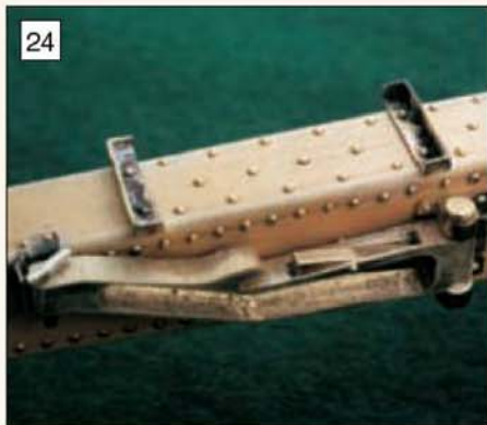
The cradle clamp on the left-hand leg. The model portrays the rivetted type of carriage and some of the simulated rivets can be seen.
