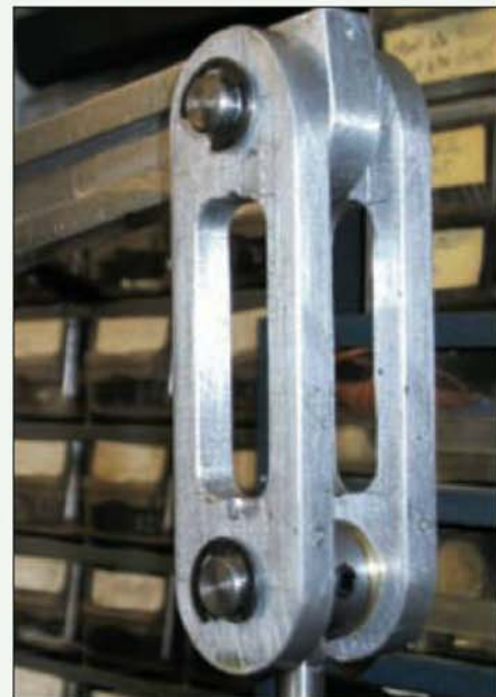
The robust beam to displacer rod link made from aluminium alloy.
