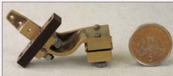
The terminal mounting insulator fits on to the fixed contact clamps and can be seen in this view of the terminal assembly. Note blow out coil connection.
