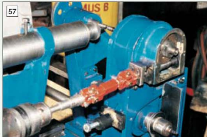
57 The rocking arm drive system currently in use. Drive is by an electric pistol drill via a cardan shaft and thence to a worm and worm wheel assembly.
