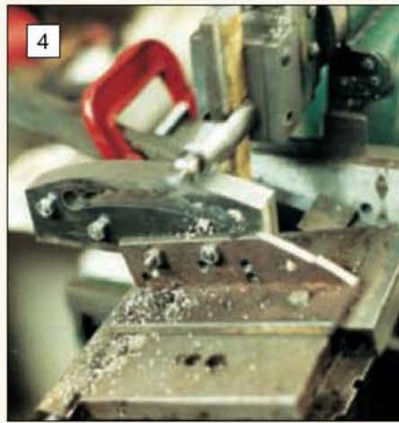
Cutting the inside convex curve on the expansion link. Note the different mounting arrangement.
