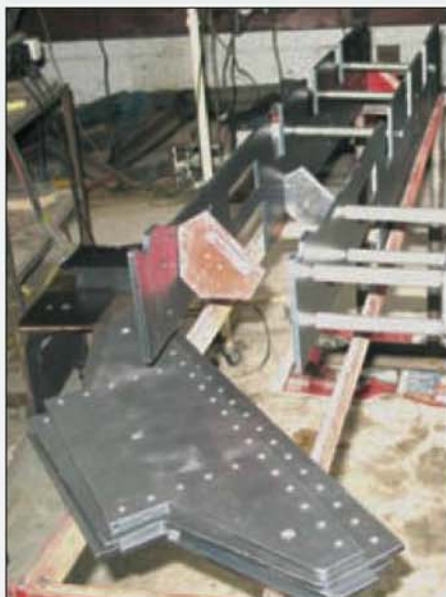
The substantial, laser cut frames and buffer beams for Lillian.
