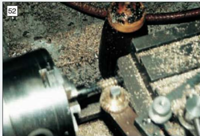
The set up used to cut the worm wheel for the fine feed gearbox assembly. The fourth attempt brought the required result.
