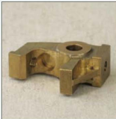
The contact rocker from below showing the pocket for the knuckling spring.
