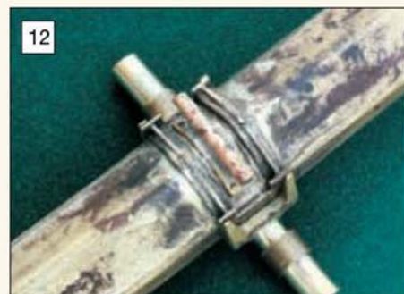
Underside view of the trough showing the trunnion band and cross shaft for the quick loading gear.
