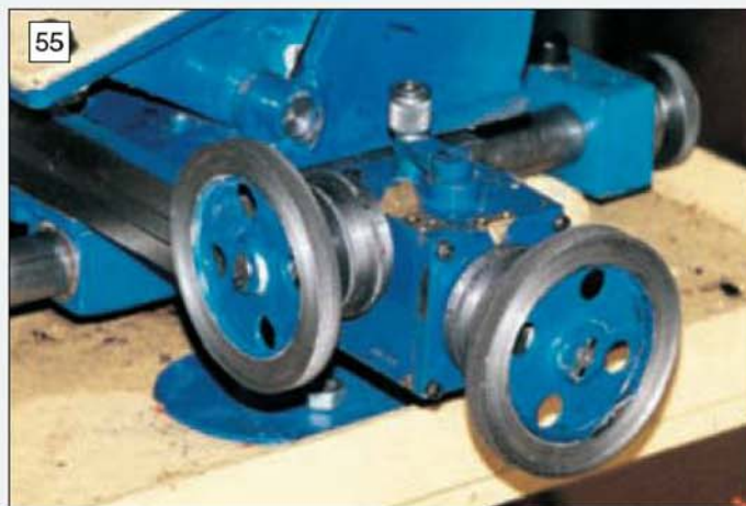
The fine feed gearbox assembled on the machine. The items that look like paint damage are brass index pointers.
