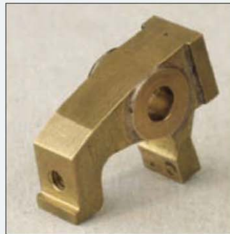
A front view of the contact rocker showing the shouldered tip seating register.
