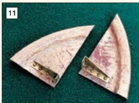
The protective wing plates. These were shaped from copper sheet beaten over a hardwood former.
