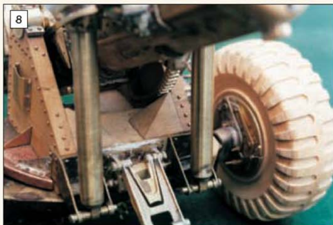
Front view of the saddle showing the balancing gear hinge brackets, front cradle clamp, protecting wing plates and simulated rivetted construction.
