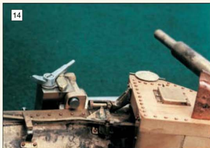
The quick loading gear lever pivot and right hand plunger assembly mounted on the gun.
