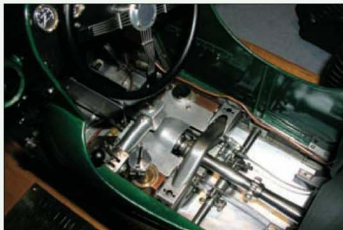
A close-up view of the cockpit of the model Austin with the seat removed to show the working gearbox and drive arrangements.
