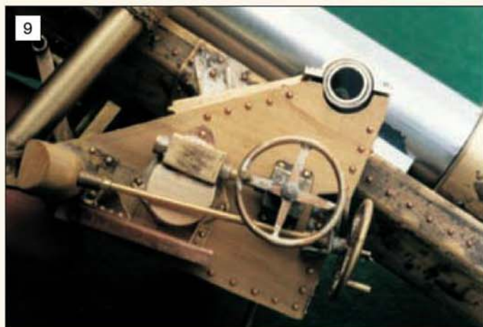
The left-hand side of the saddle showing elevation and the bearing hand wheels and gearboxes.
