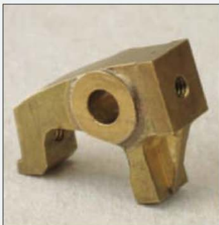
The contact rocker rear. The threaded face accepts the connection braid.
