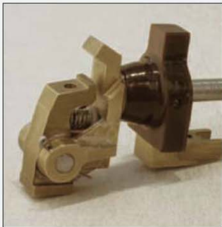
The contact rocker split pinned into the holder and insulator assembly. Note the knuckling spring.
