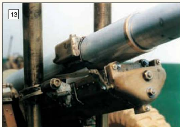
This shows the balancing gear brackets attached to the trough and also the cut-off gear and front cap of the cradle.
