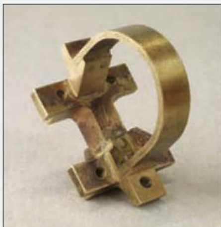
The fixed contact holder showing the loop of material that forms the arc horn and runner.
