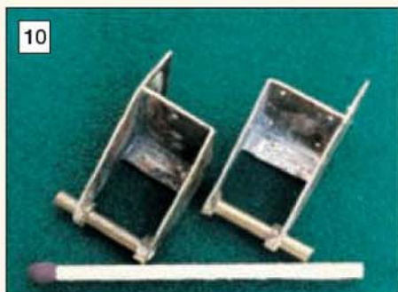
The balancing gear hinge brackets fabricated from brass sheet. Their size can be gauged from the match in the foreground.
