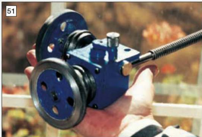
The compact fine feed gearbox assembly. Although designed specifically for Camcutter this item may have uses on other types of machine tool.
