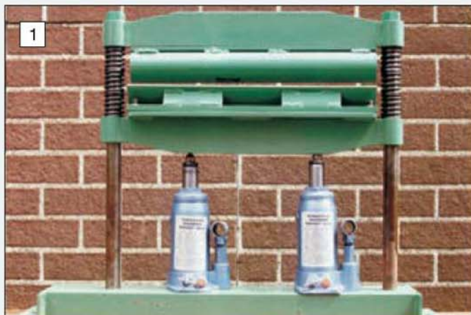
The hydraulic press devised to create the bends in the the copper for the authors boiler. It is based on that designed by Alec Farmer.
