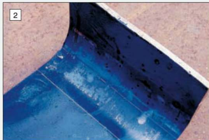
A sample bend in the copper made in the press shown in photo 1. Note the marking out lines to aid positioning.
