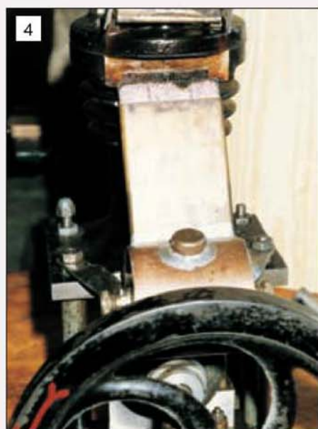
Details of the methylated spirit burner used on the home-made version of the engine.
