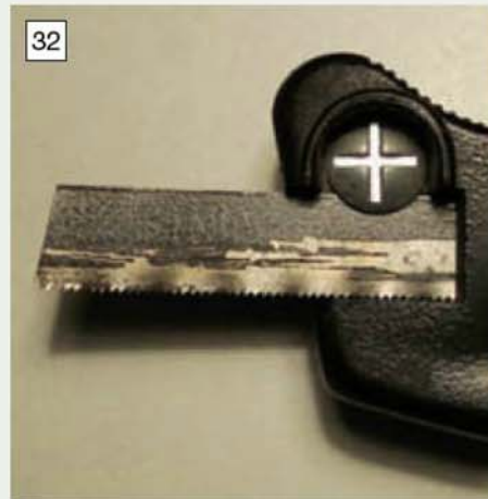
The tool used to make the second cut was a piece of broken hacksaw blade in a handle.
