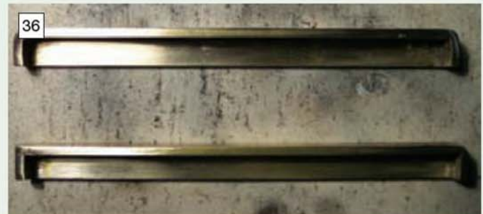
Here the saw cut grooves have been filled with soft solder so that each column is as rigid as possible.
