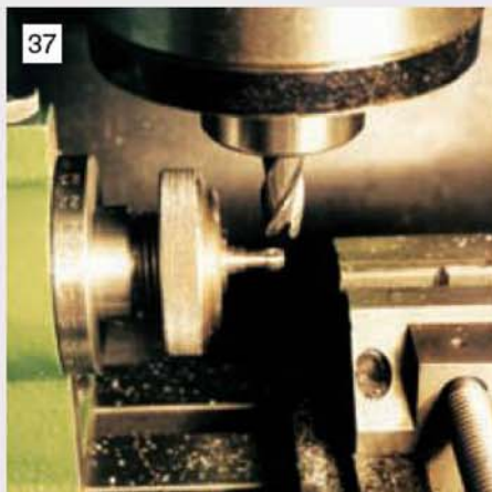
Milling the flats on the piston rod cross head using the vertical milling machine.
