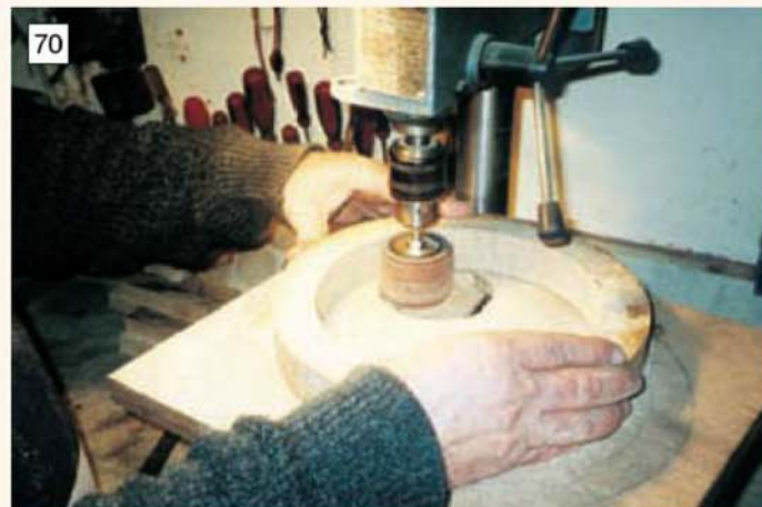
An alternative approach is to make the centre part of the rim in one piece. Here the drilling machine is being used as a sander (Photo: John Thompson)
