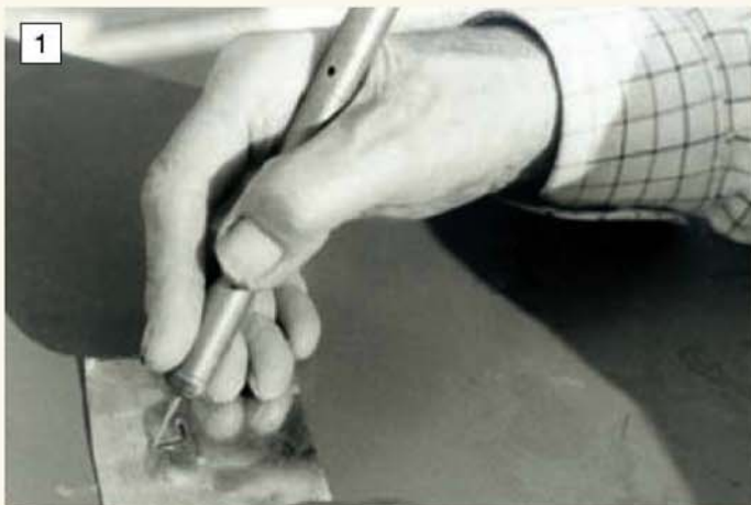
Using a lightweight hand-piece in the writing position described by the author in the text.
