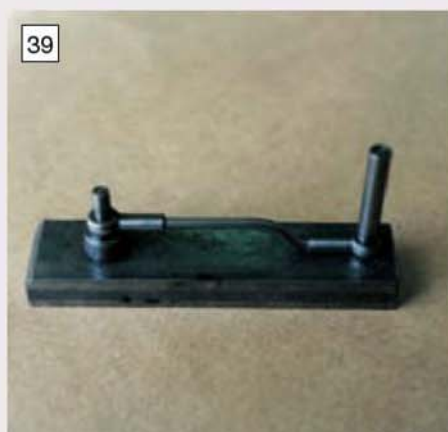
The small assembly jig devised for the parallel motion inner levers.
