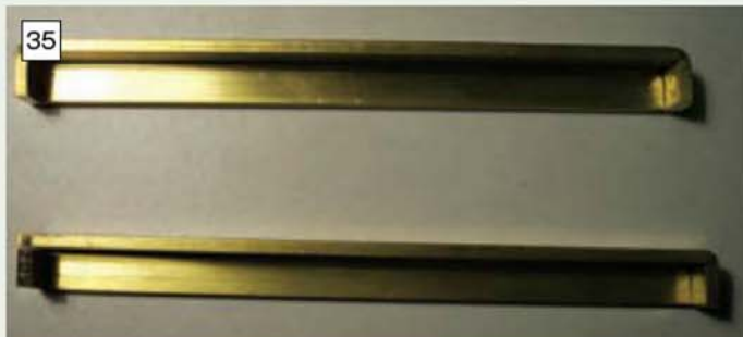
This is how the columns should look after both ends have been bent to the required 90deg. angle.
