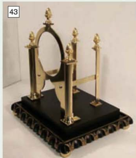
The polished main plate and columns assembled onto the base.
