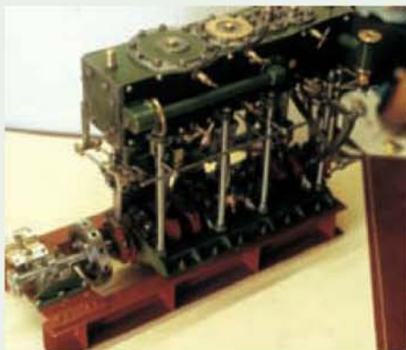
The top view showing the cylinder covers and the long, intermediate cylinder to low pressure cylinder steam transfer pipe.
