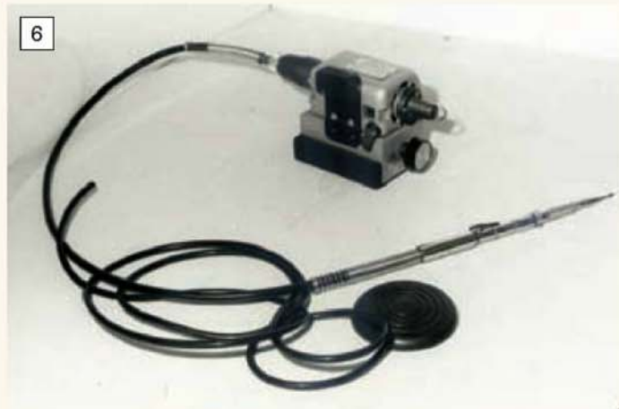
A small, commercial flexible drive system with its drive motor, flexible shaft, hand-piece and foot operated control switch.
