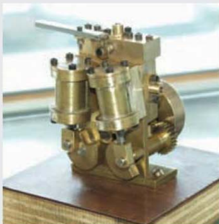
A neat two-cylinder, double acting, oscillating cylinder Uniflow engine by Ian Cornish.
