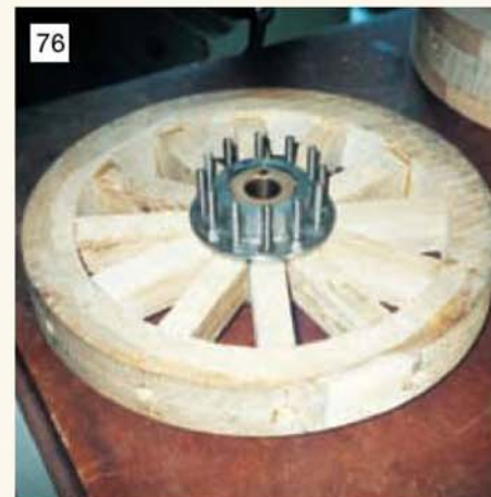
A part built rear wheel. The inner spoke ends are clamped by the hub. (Photo: John Thompson).
