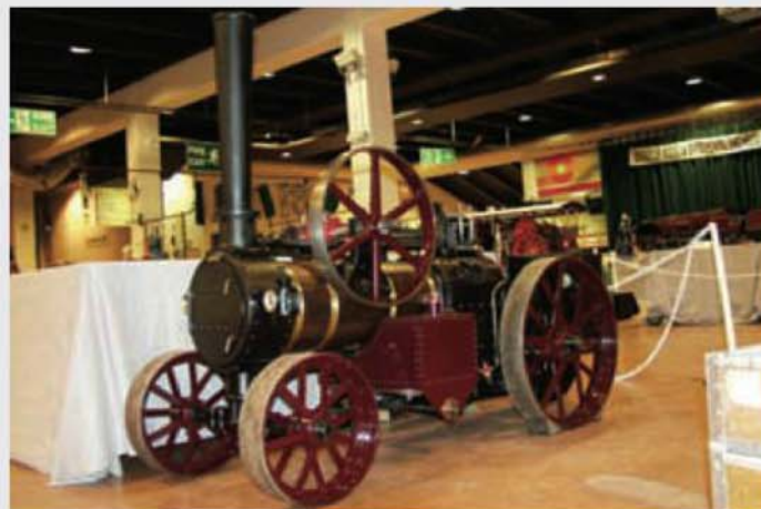
Based on an unusual prototype, Mr. Brian Baker's 5in. to the foot Foster single-cylinder, rope hauling engine was an impressive exhibit.
