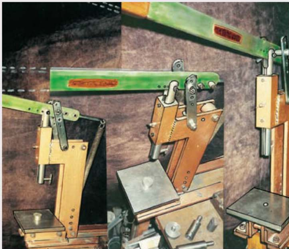
Some views of the fabricated lever press. This was an apprentice's design and build exercise carried out under the supervision of the author. It was fabricated from stock materials and is therefore well adapted for construction by amateurs for use in their own workshops.
