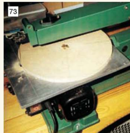
Rims can be cut on the jig saw by rotating the board around a fixed spigot (Photo: Cyril Hayler).
