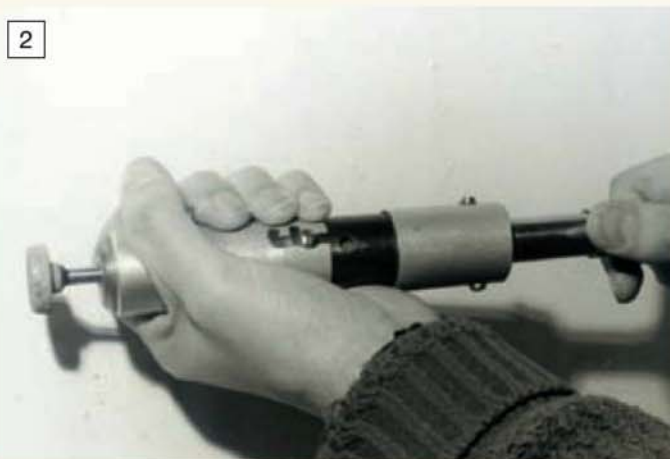
Heavier hand pieces are better gripped in the manner shown for work such as grinding or wire brushing.
