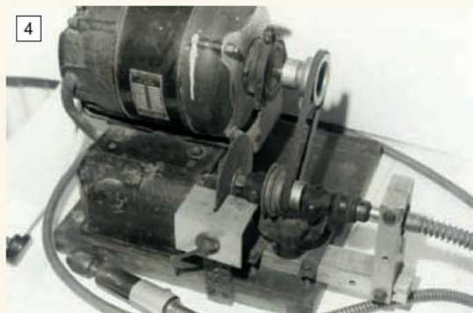
A typical flexible drive installation using a board mounted motor driving a countershaft which, in turn, drives the shaft and also carries a cut-off wheel.
