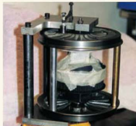
Driving wheels as set up for quartering on a plain axle. The masking tape prevents excess Loctite running down into the axlebox. Elastic bands hold the crankpins against the reference face of the jig.
