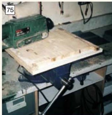
Spokes can be sanded 'en masse' using a hand held belt sander. (Photo: John Thompson).
