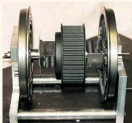
Driving wheels set up conventionally in the quartering jig. Note the oil hole in the axle to the left of the axlebox. The belt wheel takes drive from the rigidly-mounted layshaft, all 7bhp of it.
