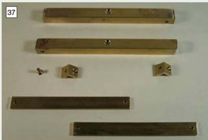
The columns and other parts can now be marked out and the necessary holes drilled and, where appropriate, tapped.
