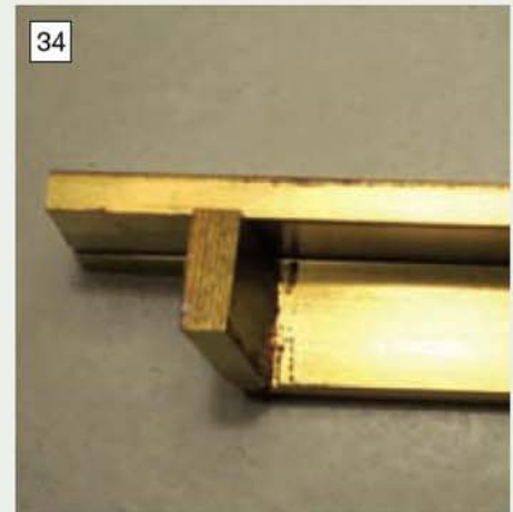
Further work with the hacksaw blade allows the bend to be completed as shown.
