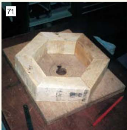
Ash sections are then glued to the rim to give the traditional appearance. (Photo: John Thompson).
