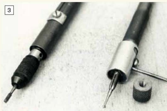
Two light hand-pieces with limited range chucks and of the type whose construction is described in the text.
