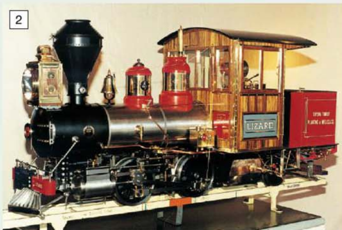
The author's 0-4-2 narrow gauge Baldwin locomotive seen here fitted with the spark arrester chimney.
