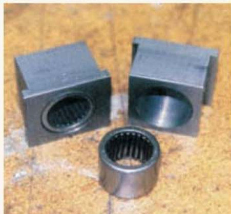
Mild steel axleboxes with 3/4in. bore needle roller bearings, to Neville Evans' design. Note the substantial single flange. (see Tim Coles' letter above)
