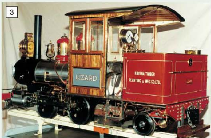
Another view of the author's Baldwin this time fitted with the alternative stovepipe chimney.
