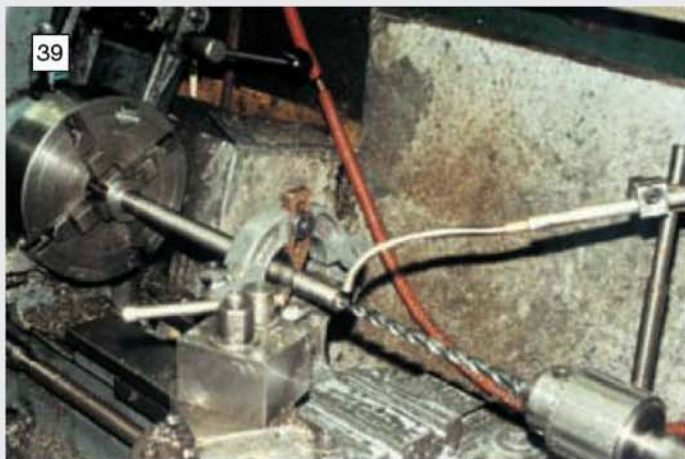
Drilling the 200mm long, 8mm dia. hole through the spindle using a long series drill, plenty of coolant and patience.
