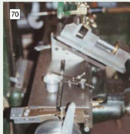
Dividing the linear vernier scale on the temperature compensating arm.
