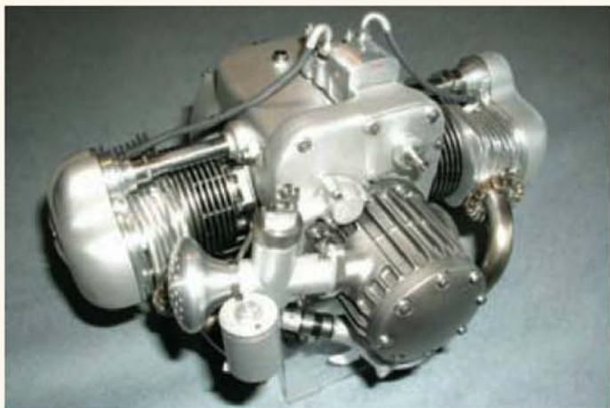
The well-detailed model of the 1938 twin-cylinder, supercharged BMW RS 500 engine by Rolf Depping.
