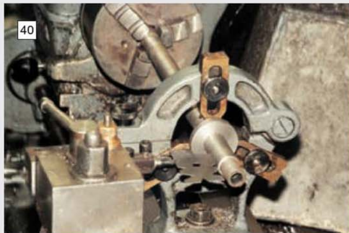
Setting up to screw cut the 16mm x 24tpi thread specified for the spindle nose. Note the use of the fixed steady.
