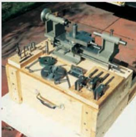
The lathe shown removed from its treadle base and displayed on its packing case, which is used for safe storage and transportation purposes.
