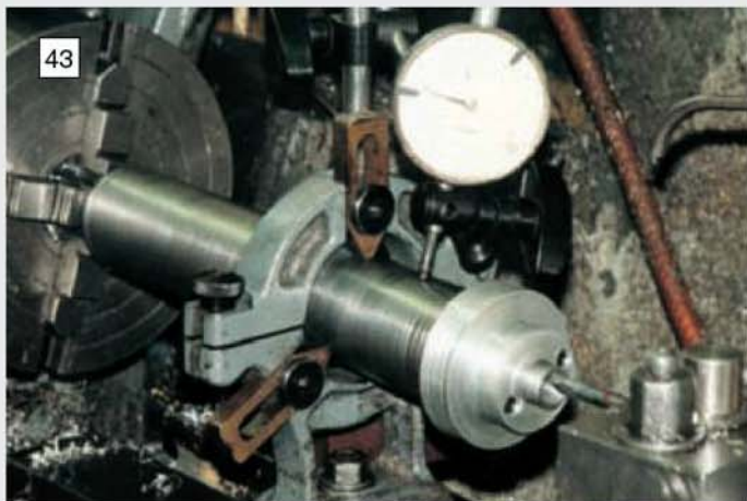
Another view of the tooling taper boring procedure. The method used was that described by Prof. Chaddock in his series on the Quorn.
