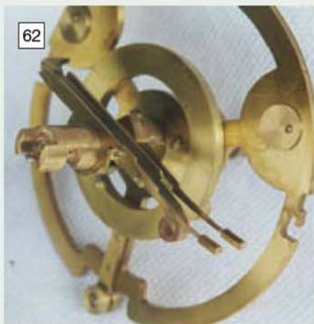
62 The lower balance arbor with the pallet adjustable for angle only plus the saddle cam.
