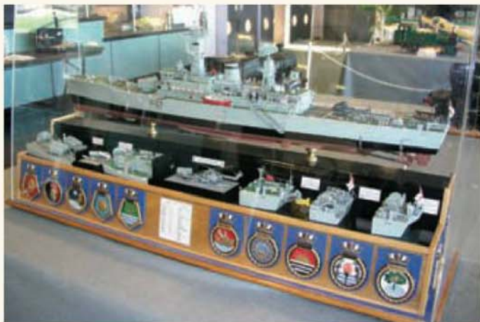
David Brown's Leander Class frigate HMS Danae was displayed with several alternative modules illustrating variations in ships within the class.
