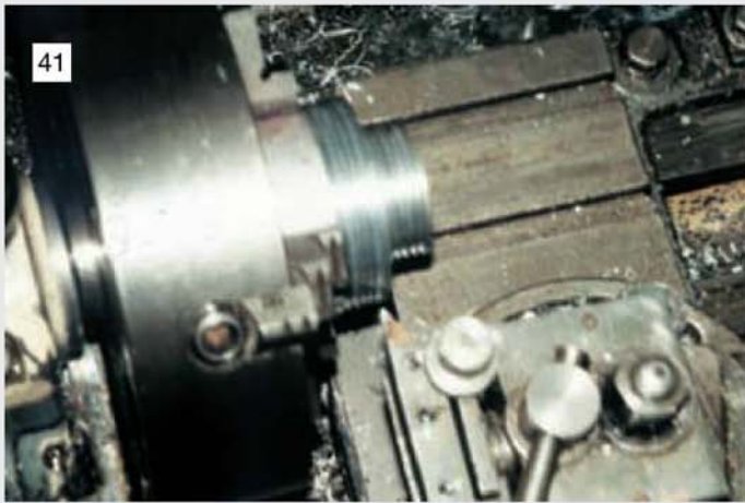
41 Machining the poly-V groove pulley from a billet of aluminium alloy using a special tool ground to the correct geometry.
