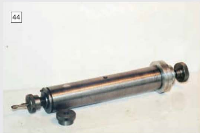
The finished spindle assembly. A 6mm dia. milling cutter is shown mounted in the milling end of the spindle.
