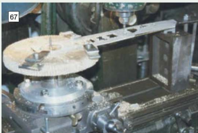
Milling the openings in the isochronism correcting adjusting lever on the milling machine.
