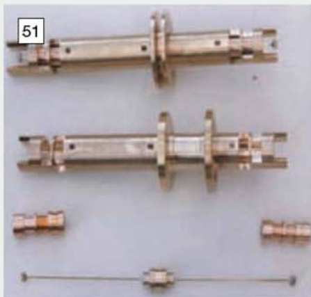
The upper and lower balance arbors, inserted bearing bushes and centralising wire.
