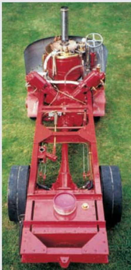
The virtually completed chassis showing the engine, drive arrangements, water tank and driving controls.
