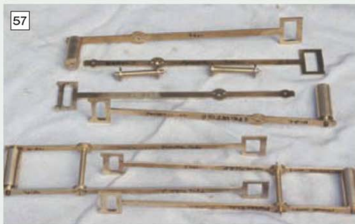
The balance arbor anti-friction arcs shown both in component form and assembled. The annotation is an aid to assembly!
