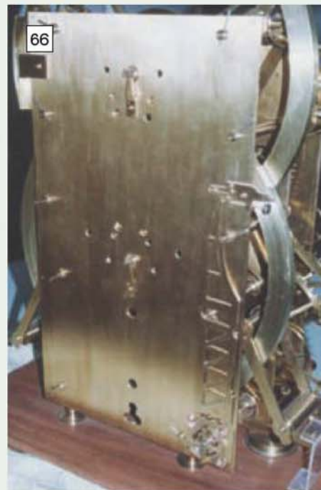
A three-quarter back view showing the isochronism correcting adjusting lever.
