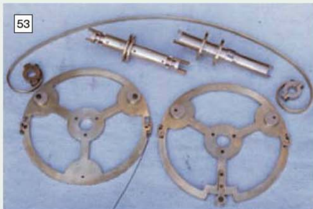
The pulleys, poising weights, upper and lower balance arbors and balance arc spring.
