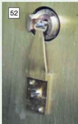
The balance arbor wire, sprung anchor on the back plate
