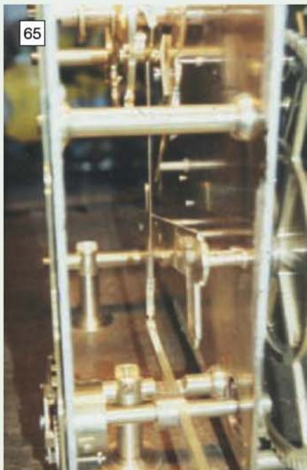
The isochronism correcting mechanism assembled in position on the clock.
