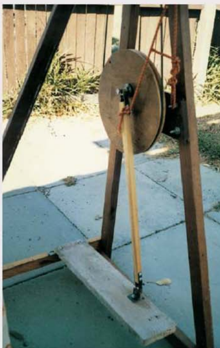
The lower portion of the treadle drive unit. All materials used are simple and inexpensive.
