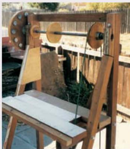
The upper portion of the treadle drive unit. The lead loaded flywheel can be seen to the left.
