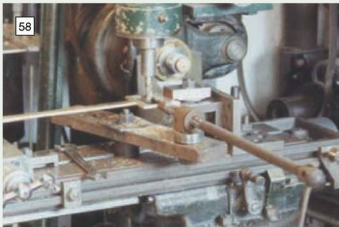
58 Machining the radial curve on the lower balance arbor anti-friction arc on the milling machine.
