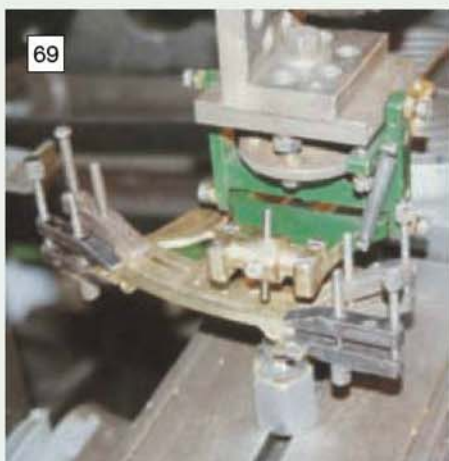
Dividing the curved vernier scale on the temperature compensating arm.
