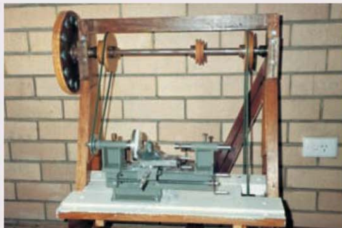
A front elevation of the completed machine shown with a work piece held to the faceplate by a draw bar.
