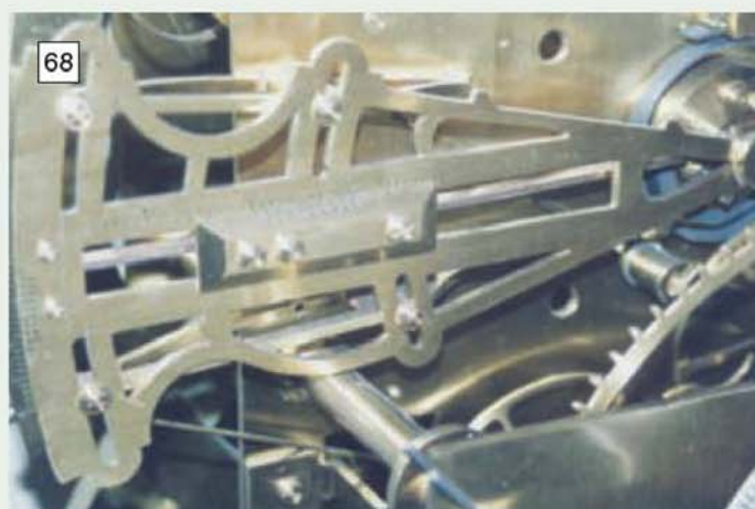
The temperature compensating arm. All the engraving was carried out in the author's home workshop.
