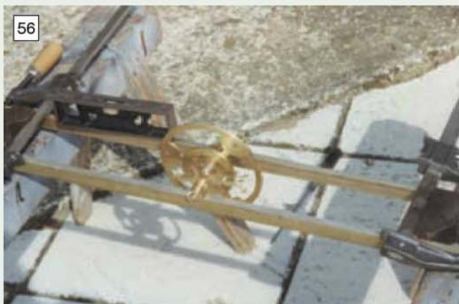
Setting the poise weights of the lower pulley and arbor using the level bars. The latter are supported on trestles.
