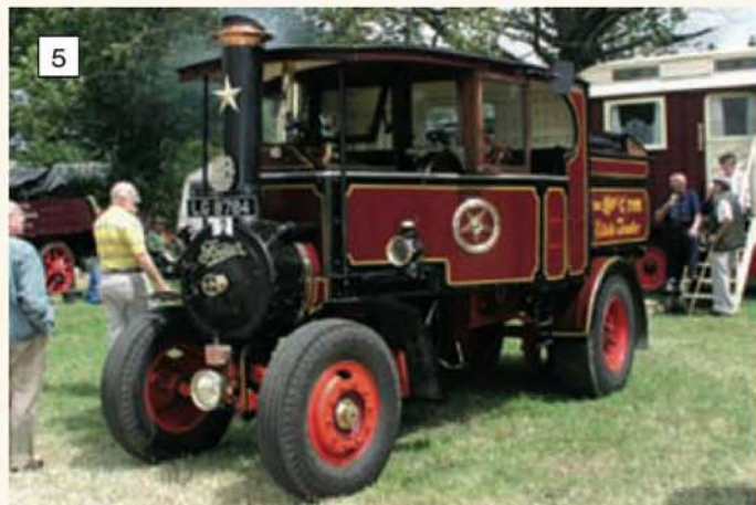
5 A 1925 Foden C Type tractor built for estate work. Note the period lighting and Royal Warrant on the chimney.
