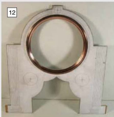
Here the plate has been cleaned up and the dial bezel being checked for fit.
