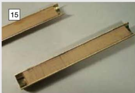
15: To give something for the fixing screws to bite into wooden dowel sections were cut and glued into the backs of the fluted tube halves using epoxy resin adhesive.
