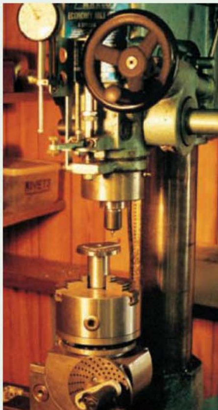
Drilling the indexing holes in the base of the South Bend pillar using the dividing head fitted to a versatile milling/drilling machine.
