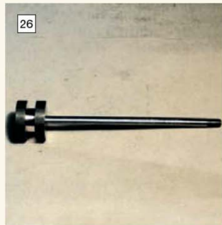
26 The finished piston and piston rod. The rod is of stainless steel and the piston brass.
