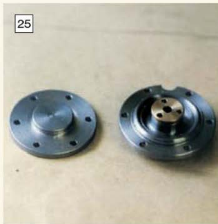
25 The completed top (right) and bottom (left) cylinder covers.
