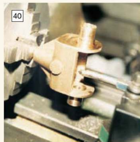
The steering box is fixed on a stub mandrel for machining the inside face. (Photo: Stan Nipper)
