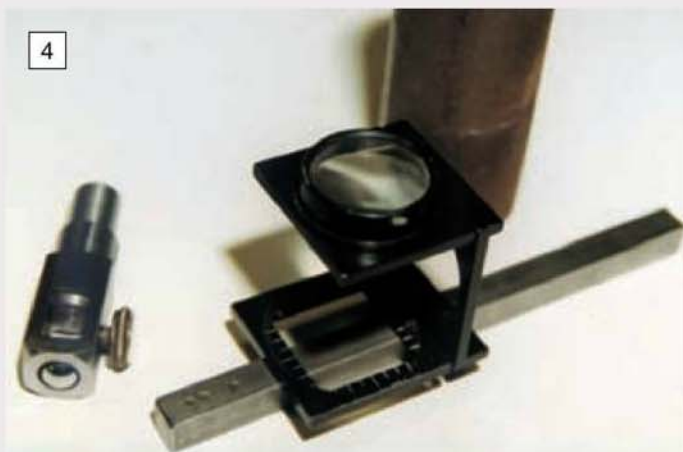
The diameter of the indentations made by the 10mm ball and a smart blow from a 1 1/2 lb. hammer can be assessed using a linen tester, as here.
