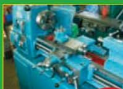
Raglan 5" x 24" variable speed, gearbox and chucks
