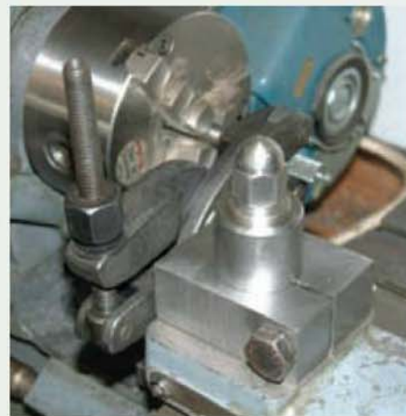
A commercial knurling tool modified to fit the pillar tool post system and in use on the Myford.
