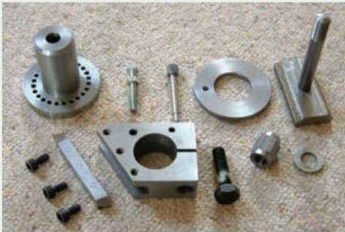
'Kit of parts' for the South Bend lathe showing the special indexing pillar, spacer washer, T-bolt, one tool holder and associated components.
