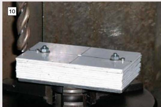
Setting up to machine the blanks. The layers for both of the two gears can be machined together.
