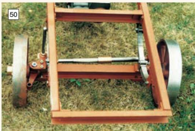
The drag link assembled on the model. The working parts are totally enclosed. (Photo: Stan Nipper)
