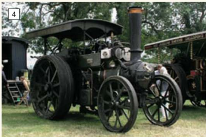
4 A 1914 Aveling & Porter 6nhp heavy road locomotive. A stately engine built for heavy haulage on the road.
