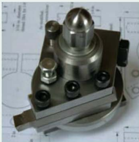
One of the 30deg. tool holders assembled with the South Bend pillar.
