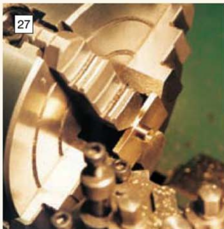
Machining the steam chest cover from a piece of solid brass bar.
