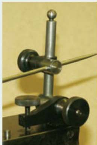
Mr. Gascoyne tells us that the finial at the top of this surface gauge column is not only decorative but facilitates assembly of the monkey.
