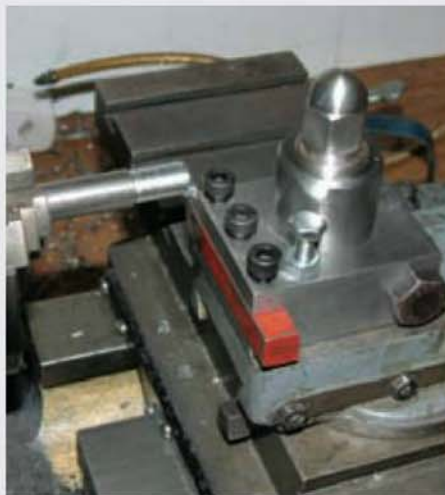
One of the straight tool holders in use on the Author's Myford lathe. The height adjustment screw and M10 locking screw can be clearly seen.
