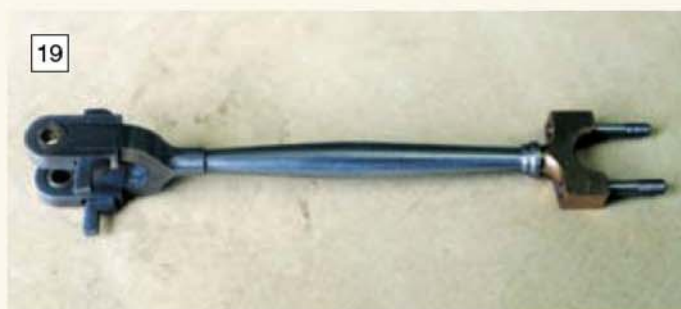
The alternative style of connecting rod for the two-web crankshaft shown here without its big end bearing cap.
