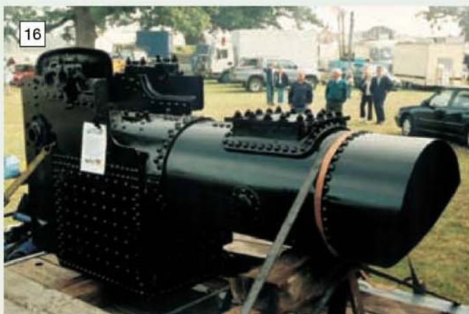
A bare boiler for an Aveling and Porter steam roller, which has been the subject of extensive restoration.
