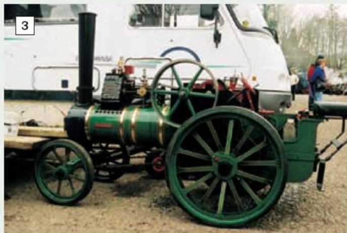
The 1:3 scale Dodman makes a handsome and unusual model. Note the sloping valve cover referred to in the text.
