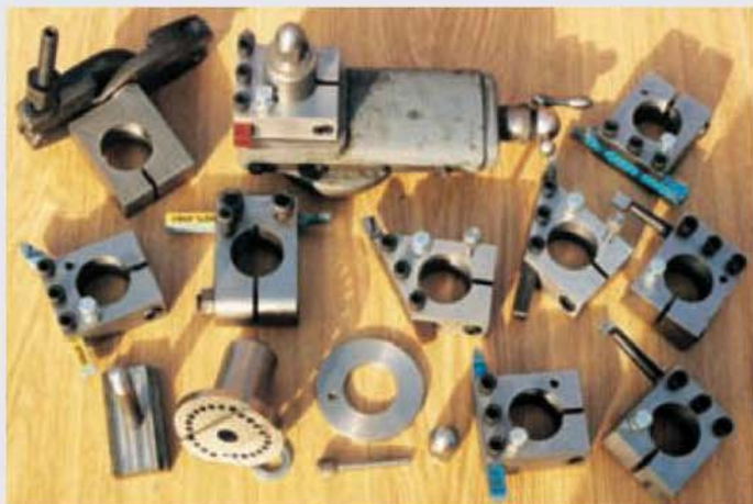
Some of the parts in the outfit. Shown is the Myford top slide, parts for the South Bend lathe, some tool holders and a modified knurling tool.
