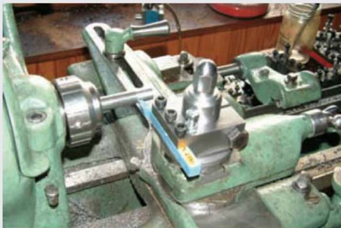
A straight tool holder in use on the South Bend lathe. The main pillar is attached to the top slide via the T-slot machined by the manufacturers.
