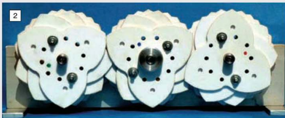
The three gears shown in this photograph mesh as follows: the centre and right hand gears mesh conventionally but the centre and left hand gears mesh paradoxically. Can you explain why?
