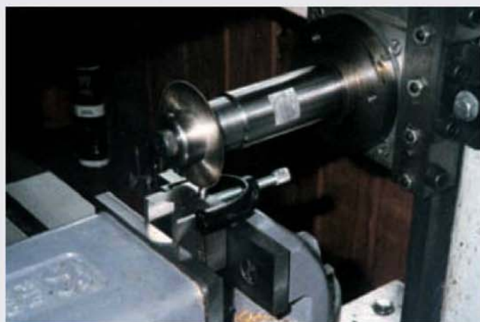
Cutting the screw driver slot in one of the dowels using the horizontal milling machine. Carefully used, a hacksaw would do nearly as well!
