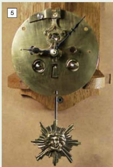
Having been fitted with a 'sunburst' pendulum, the movement undergoes test.
