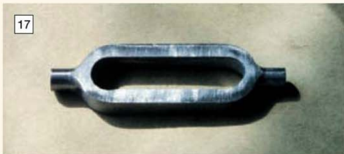
Although only one forked end is required for the connecting rod a pair were machined to simplify work holding.
