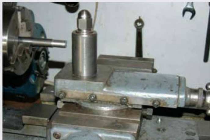
The main pillar fitted to the Myford Series 7 top slide showing the acorn nut which cleans up the appearance and helps prevent cut hands.
