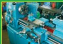
Raglan 5" x 24" variable speed, gearbox and chucks
