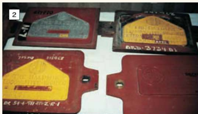
Some of the patterns used to cast Baldwin builder's plates after 1944. Not all are for steam engines.
