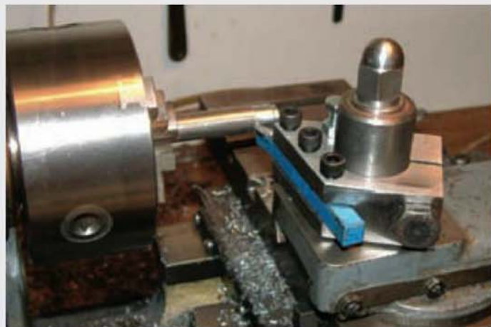
A 30deg. tool holder in use on the Author's Myford Series 7 lathe. This type of tool holder gives improved access on certain classes of work.
