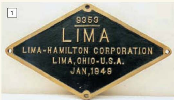
The diamond-shaped Lima-Hamilton plate fitted to steam engines built after the amalgamation of 1947.
