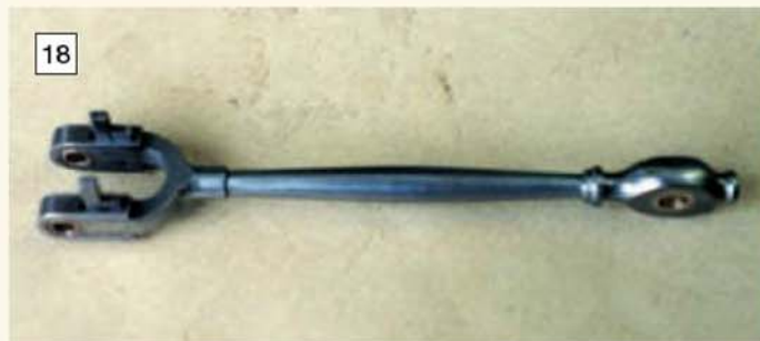
A finished connecting rod fitted with its bushes, straps and brasses for the overhung crank engine.
