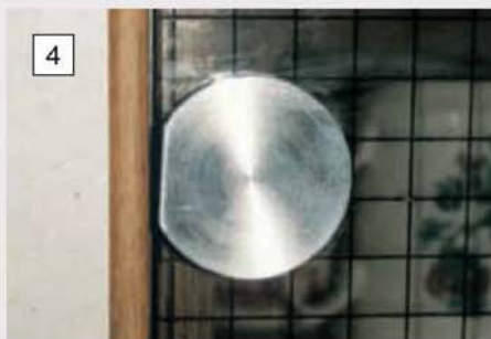
The neat appearance of the adaptor front pieces which are machined in stainless steel.
