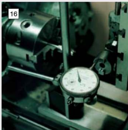
Using a DTI to check that both bedding faces share a common datum.
