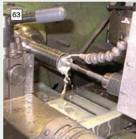
63 Honing under way on the lathe. The hone is powered by a home made drive unit.
