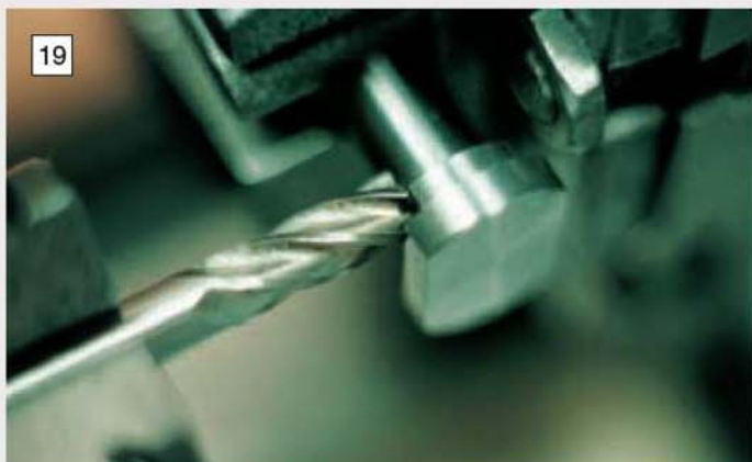
Milling the end of the T-bolt to give necessary form to engage in the T-slots of the cross-slide.
