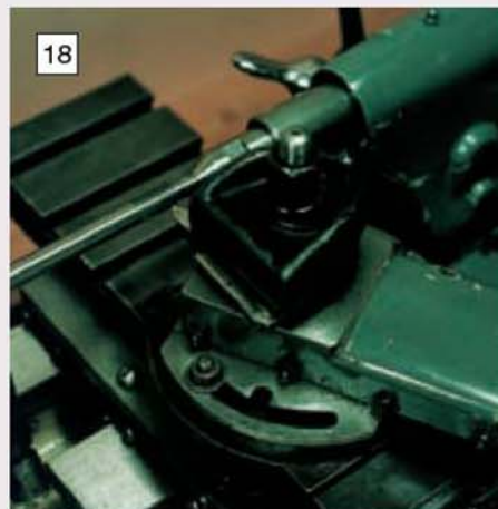
Screw cutting the T-bolt. Note the adaptor under the top-slide to facilitate the angle setting.
