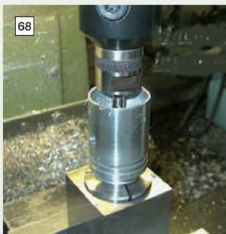
68 Milling out the internal features of the piston; note the collet block held in the machine vice.
