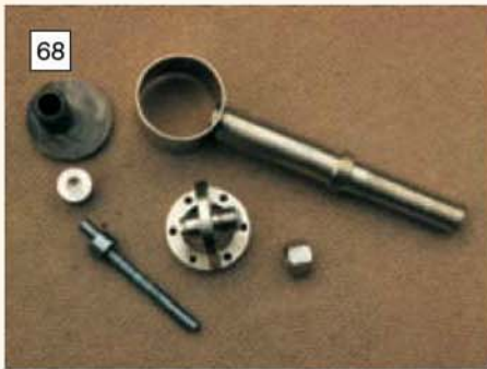
The components of the regulator; thin wall 1 1/4 in. OD brass tube should not be used here.
