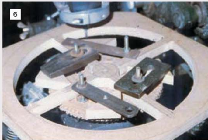
6 Machining the MDF board pattern for the balance wheel castings using the milling machine.
