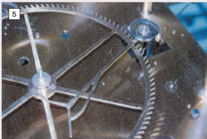
5 The escape wheel with 'lantern pinion', detent arm, loose claw and spring referred to in the text.
