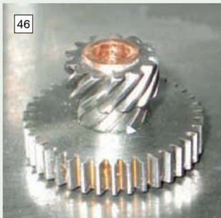
The spiral gear is attached to the large pinion by means of a through bush.
