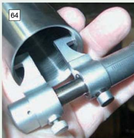
64 Checking the cylinder bore for size using an internal micrometer.
