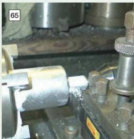
65 The first operation on the piston was to machine the chucking spigot.
