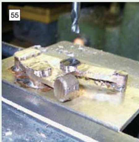
55 The brass backing plate gave unimpeded access to the workpiece.
