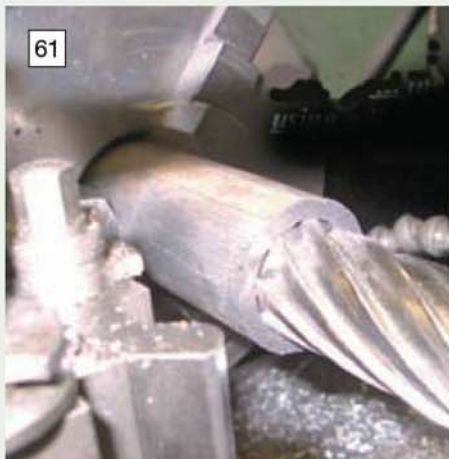
61 Machining the cylinder liner using the Author's favourite tool, a Rotabroach cutter.
