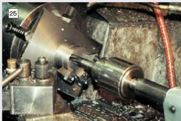
Reaming the hole that receives the spindle in the tailstock top member. The component has been attached to a plate for machining.
