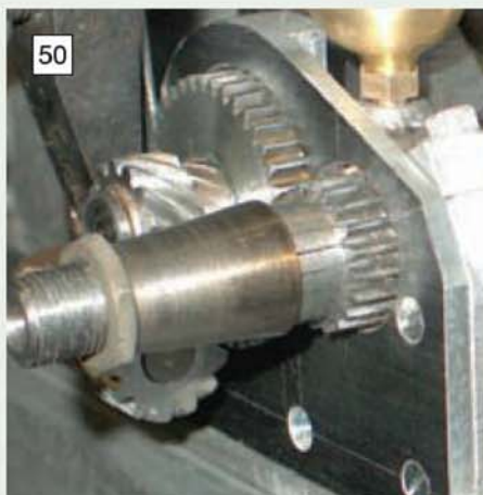
The camshaft drive in place on the engine: 1:1 spiral gears are used with 1:2 pinion gears.
