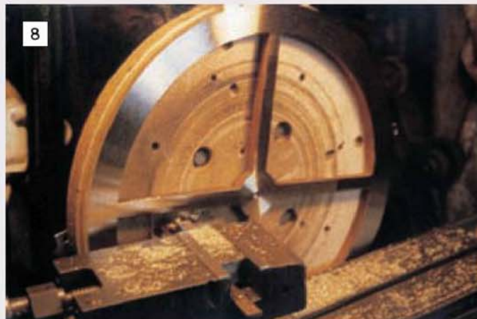
8 Preliminary machining of the face of one of the balance wheels. They were too large for the lathe and the operation was done on the milling machine.
