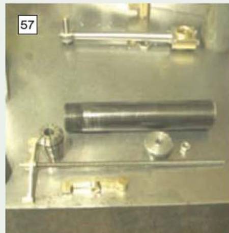
57 A selection of the tooling used to machine the rockers, shown in the foreground.
