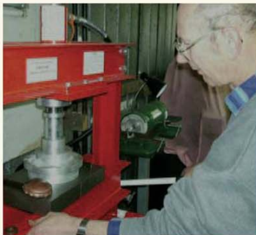
News from the Steam Locomotive Society of Victoria. Left: Bill Steward uses a hydraulic press to form a dished boiler end plate and right: progress is being made with work on the cutting wall.
