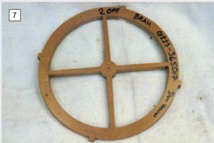
7 The finished pattern ready to go off to the foundry. MDF is a convenient material as it has no grain and simplifies the pattern making process.
