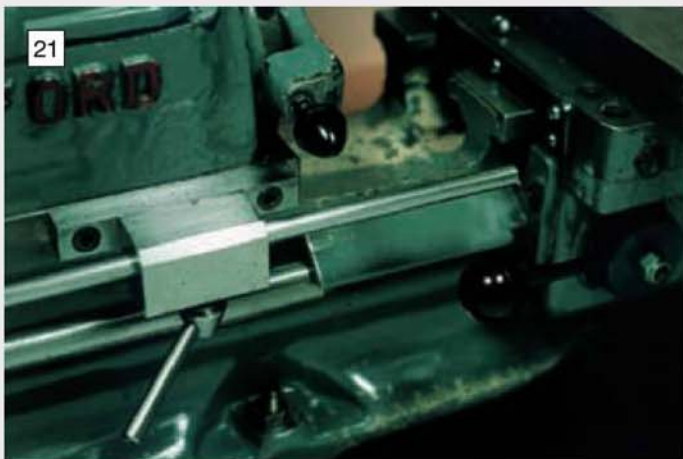
The parting off stop is often used in conjunction with a saddle stop, the drawing of which is given below.
