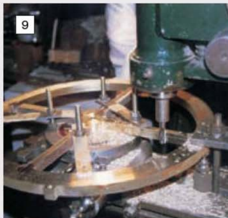
Preliminary machining of the balance wheel spokes using the rotary table mounted on the milling machine.
