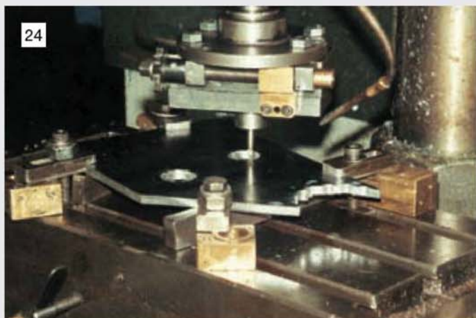
Boring the circular ends of the elongated sloping hole used for the tailstock stand plate on the milling machine.
