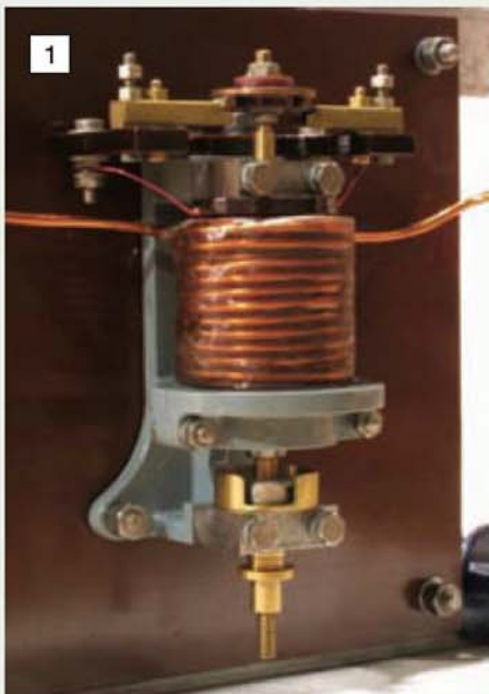
An accelerating relay. The coil carrying the motor current lifts the contact disc seen at the top of the relay. The calibration is adjusted by adding weight to the container in the coil.
