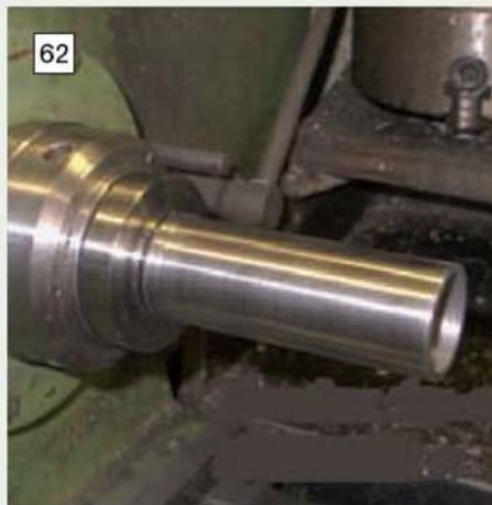
62 The finish turned cylinder liner ready for the final honing process.
