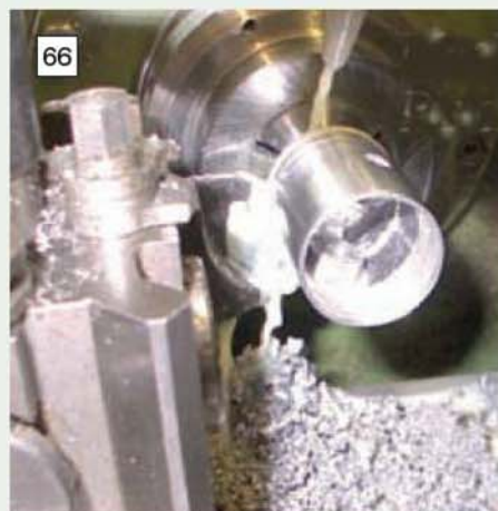
66 Machining the piston; internal milling has already been completed and finish turning is being done.
