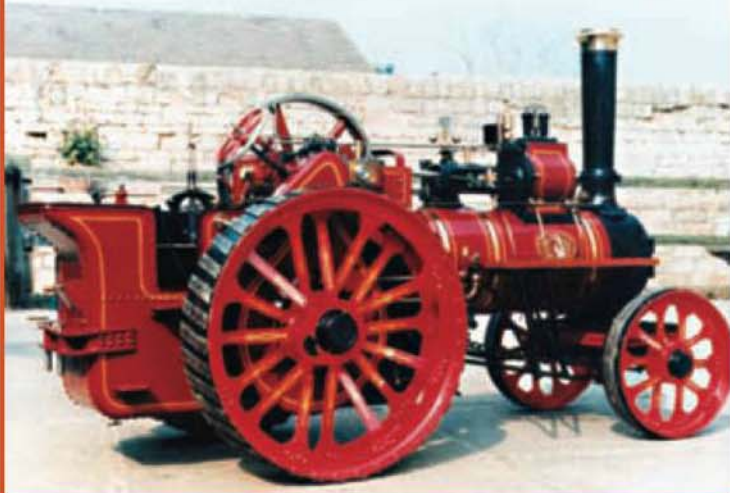
Shown here is the 3" scale MARSHALL 7 NHP single cylinder general purpose Traction Engine of 1910 'PRIDE OF THE ROAD' measured up from the full size Marshall number 54587/10. For Model Engineers who wish to build a relatively straightforward model, which is a true replica of an actual engine, at the same time powerful and robust enough to use on a rally field.
