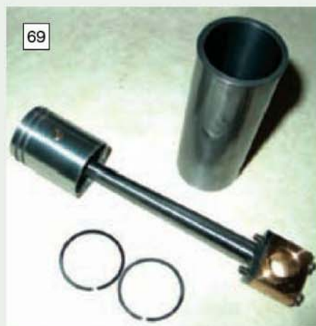
69 The piston and connecting rod assembly shown with the cylinder liner and piston rings.
