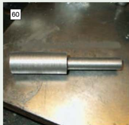
60 Careful machining resulted in a core of cast iron retrieved from the bar supplied.
