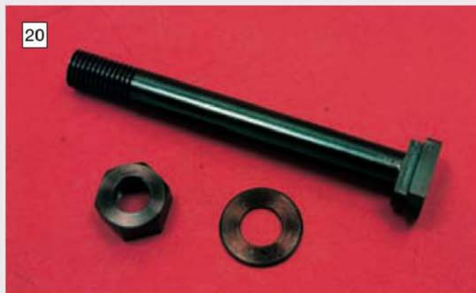
The T-bolt with its nut and washer. All were carefully blued using the sand bath method described in the text.
