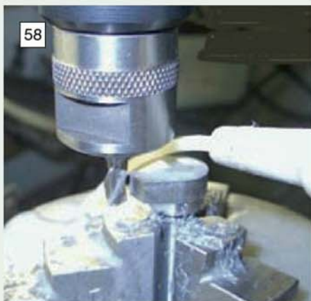
58 Milling a cam; final shaping of the profile was completed by hand.
