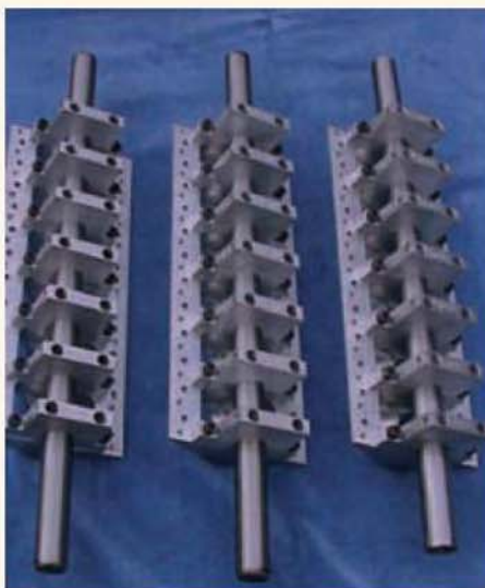
The three main bearing frames photographed during manufacture.
