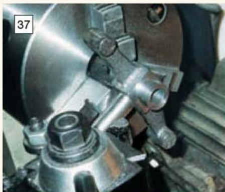
Shown here, the king pin hole has been bored and the boss machined.
