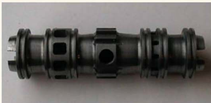
One of the cylinder liners. These were machined from cast iron. The position of the ports is crucial to engine performance.
