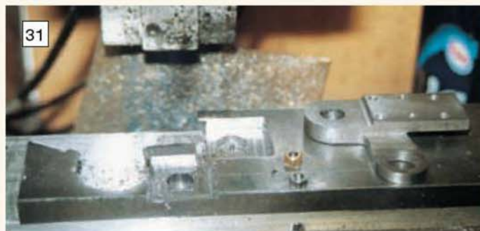
31 The completed right hand bracket and the remains of the stock from which it was cut.
