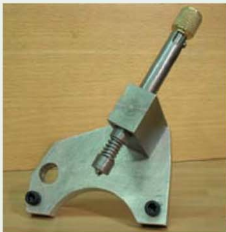
The assembled detent assembly. The design is such that an 80-tooth gear can be used.
