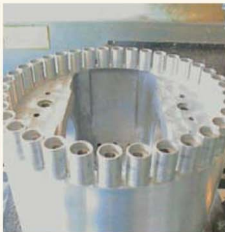
Machining the 'ringless' pistons for the assembly trials on the CNC milling machine.
