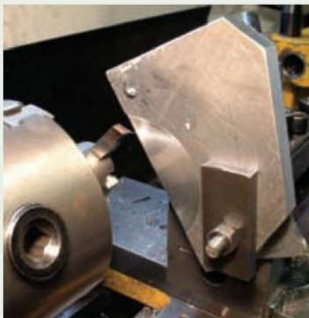
Machining the semi-circle in the Dural mounting plate with the work mounted in the top slide.
