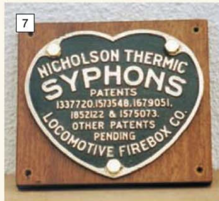
A typical equipment plate advising customers of the type and make of thermic-syphon fitted.
