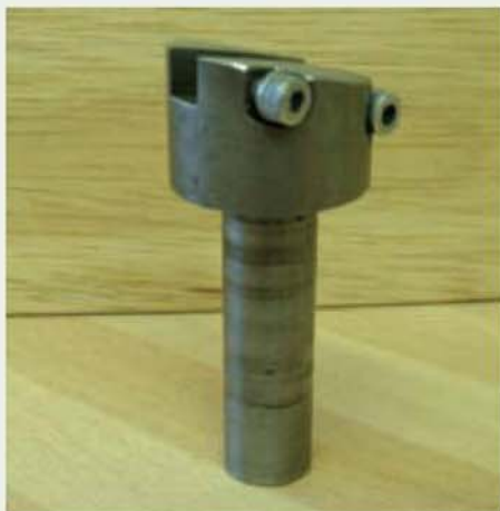
The fly-cutter used to machine the semi-circle in the mounting plate.
