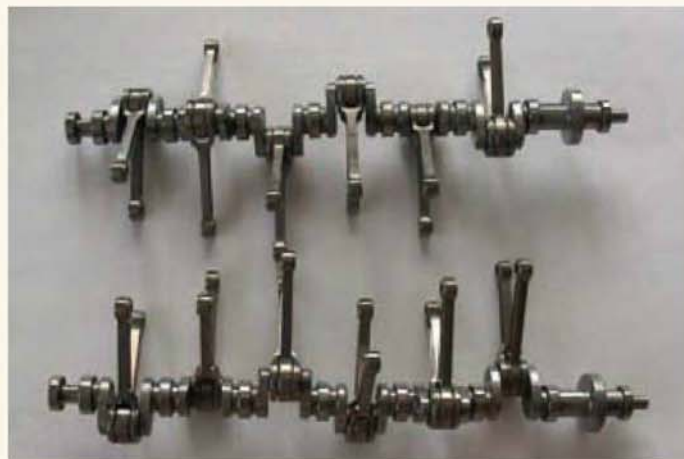
Two of the three crankshafts. Note the arrangement of the con-rods with one forked and one plain rod per big end journal.
