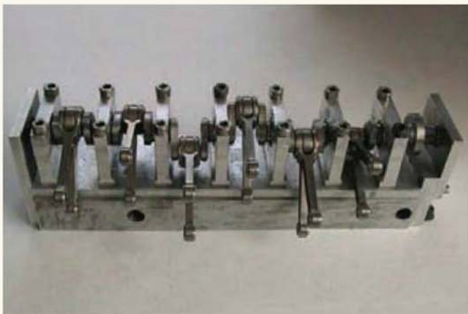
Crankshaft assembly. The crankshafts are built up using engineering adhesives for assembly.
