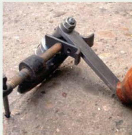
The set-up used to silver braze the handle to the handle sleeve or spacer
