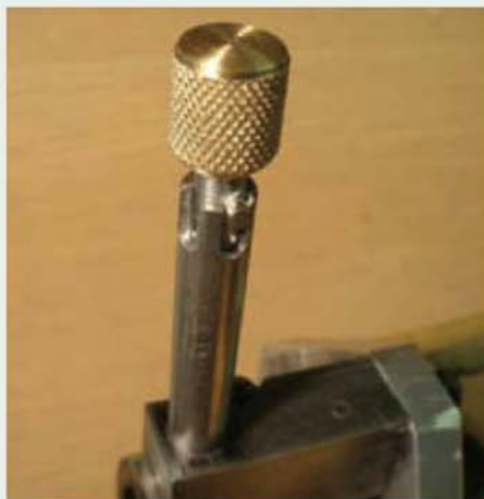
The detent barrel carries two slots to allow the detent to index through 90 degrees.
