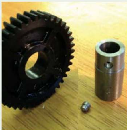
The modified handle spacer shown with its locating key and a change wheel.
