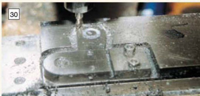
30 The right hand kingpin brackets have lugs to receive the steering gearbox.
