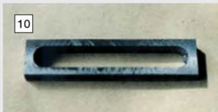
The partially finished rocker strap. It was decided to machine rather than bend this component.
