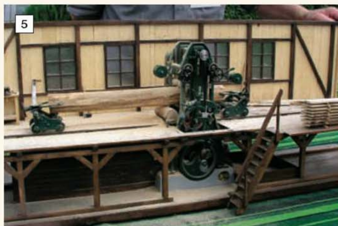
5 Heinz Muller's multi-bladed tree saw produced eight planks in a single pass.
