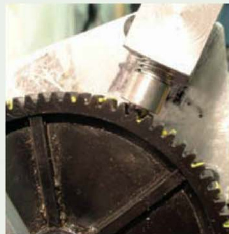
The detent in use. This type of detent can be used to index half a tooth.
