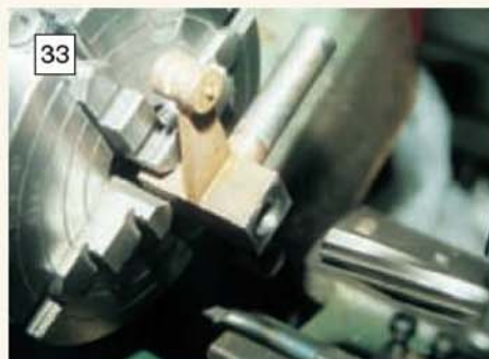
33 Reaming the kingpin hole in the stub axles after silver-soldering.
