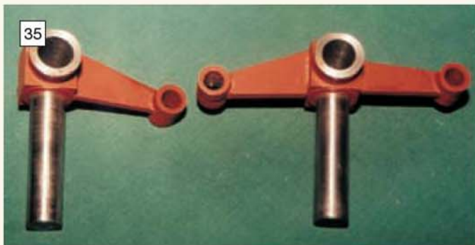
The pair of fabricated stub axles for Stan Nipper's wagon. Parts were located with 3mm dia. pins prior to silver-soldering. (Photo: Stan Nipper)
