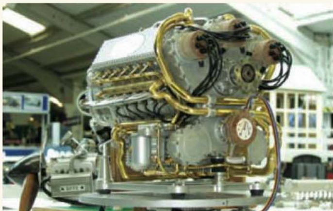
The model Deltic engine on display at the Harrogate 2004 exhibition. The ignition arrangements can be seen in this photograph.
