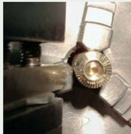
Using the dividing attachment to graduate an index dial for a boring head.
