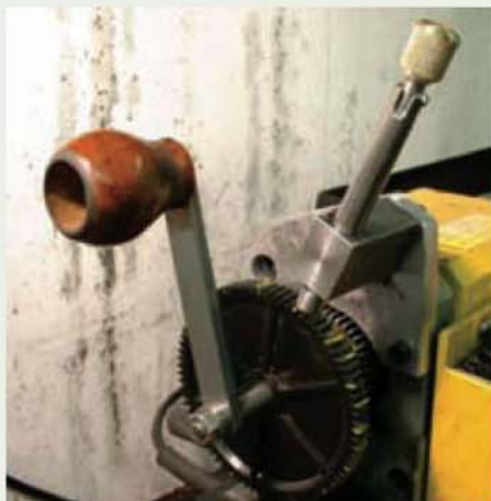
The dividing attachment in use on the lathe. It utilises the mandrel handle previously described.
