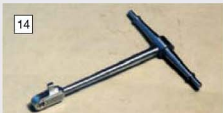
Rocker shaft and arm. The finished sub-assembly repays the care taken in its machining.
