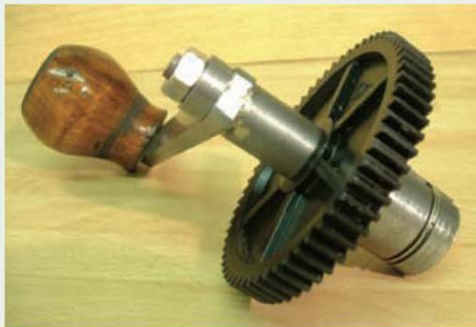
The addition of a suitable change wheel to the mandrel handle turns it into a simple dividing attachment.
