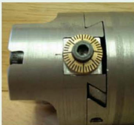
The finished index dial fitted to the home made boring head.
