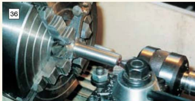
John used the spheroidal graphite iron castings available, using a tipped tool to get under the skin. (Photos 36-38: John Thompson)
