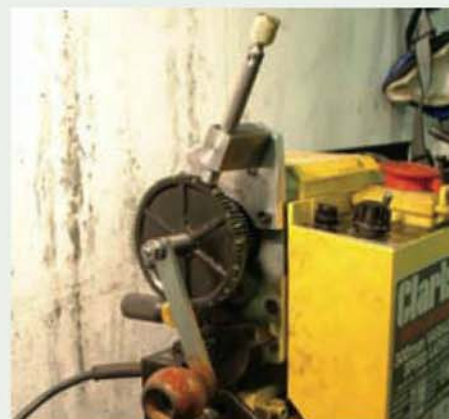
The machine must be isolated and the change wheel guard removed to use this device.
