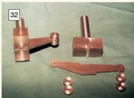
32 Stub axles being fabricated in steel. The colour is from the pickle bath.
