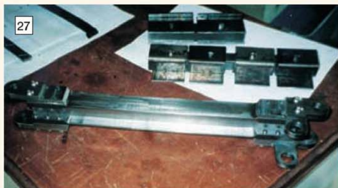
A front axle, the beam being machined from the solid. Note the pads left at the ends to receive the king pin brackets.
