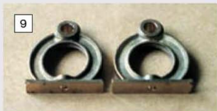
The pair of rocker brackets after separation and machining. They are supplied as one casting.
