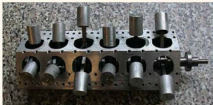
Only two more to do! One of the crankshaft assemblies complete in its crank chamber with con-rods and pistons.
