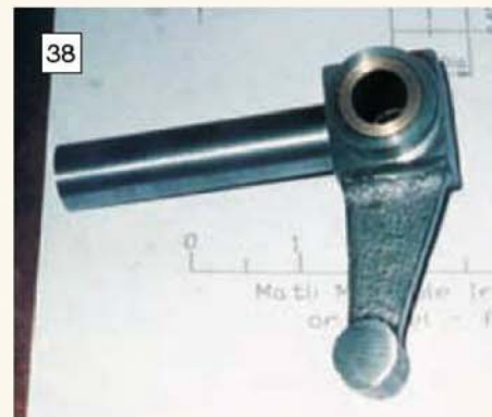
This right-hand cast stub axle now only needs the track rod hole to be drilled and reamed.
