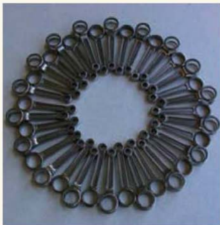
The connecting rods for the model engine. Thirty-six are required.
