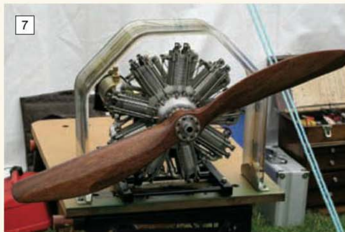
7 Ron Hankins' Bentley BR2 rotary engine impressed all who saw it run.
