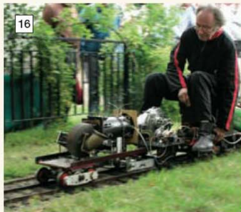
Pierre Bender's 7 1/4in. gauge experimental gas turbine locomotive utilises parts from lorry turbochargers.
