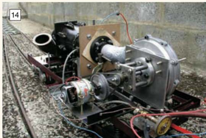
Pierre Bender's experimental 7 1/4in. gauge gas turbine locomotive.
