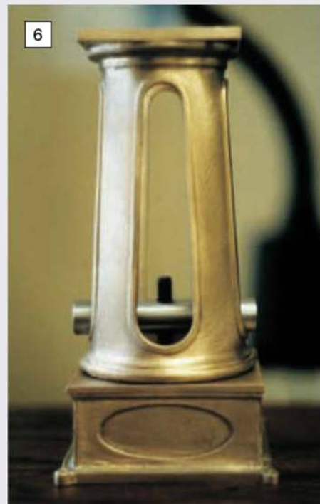
6 Once machined, the base can be clamped to the column for spotting through the fixing holes.
