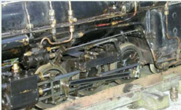
Annabel's four sets of cylinders are \frac{7}{8} in. bore x 1\frac{1}{4} in. stroke controlled by Baker valve gear operated by a steam reverser.
