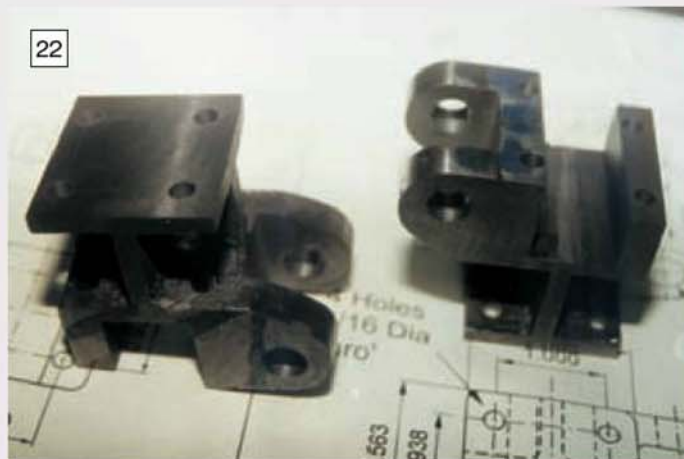
22 A pair of the spring pads shown finished machined. These components are for Stan Nipper's wagon.
