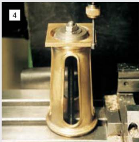
4 Using a wobbler to pick up the edges of the casting so that the hole coordinates can be set.
