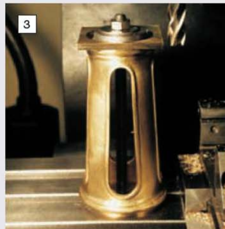
Milling the four edges of the square at the top of the column on the vertical milling machine.
