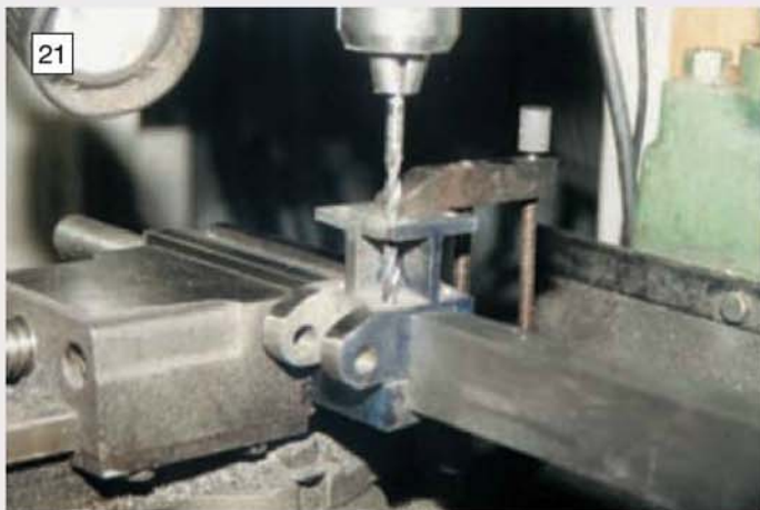
21 The back axle spring pads are assembled on the back axle and the pad and clamp drilled through together. (Photos 21-24: Stan Nipper)
