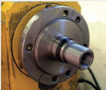
The arbor fitted to the lathe mandrel and shown after screw cutting the nose thread.
