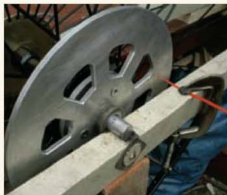
Cut from 6mm aluminium alloy plate, the brake discs were set to run true against a reference.
