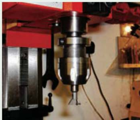
In addition to its use on the lathe, the chuck is a handy accessory for the Author's milling machine.
