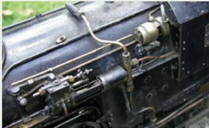
Power for the headlamp is provided by a miniature working turbo-generator given to Curly by Bobby Thompson of the Southeastern Live Steamers.
