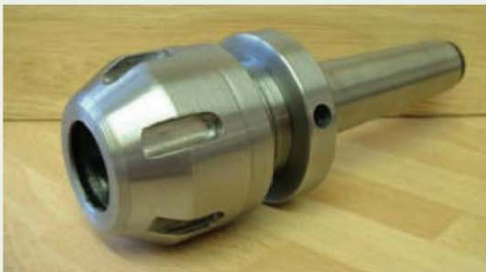
The finished collet chuck. The No. 3 Morse taper shank enables it to be used on both the Author's lathe and milling machine.
