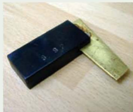
A small angle 'square' made to enable the top-slide to be set for repeatable tapers.
