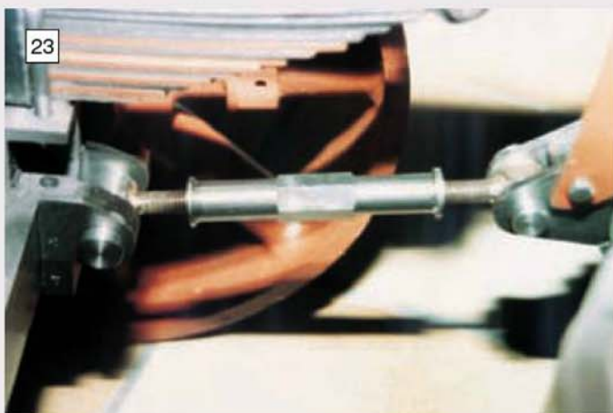
23 The back axle radial rods fit between the rear engine supports and the rear spring pads. Here the lock nuts are yet to be fitted.
