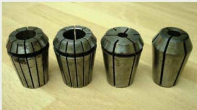
A selection of ER25 collets. The number of slots does not necessarily relate to the capacity of the collet. The far right collet has no release groove.
