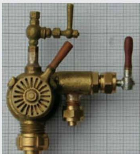
Above left, the brake valve made by Dave Noble and, above right, the real thing on 6106 (Prairie). Although generally the same shape, they do look rather different, plus the fact that the full size one doesn't have the dummy ejector control on the top.
