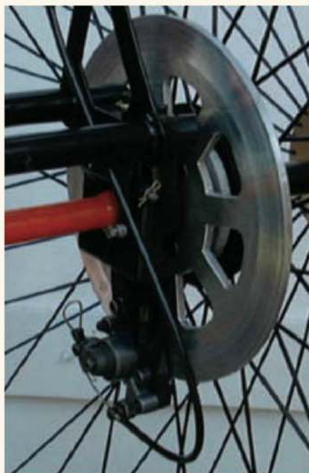
A view of the disc brake mechanism in place on the Author's finished Di-Cycle.
