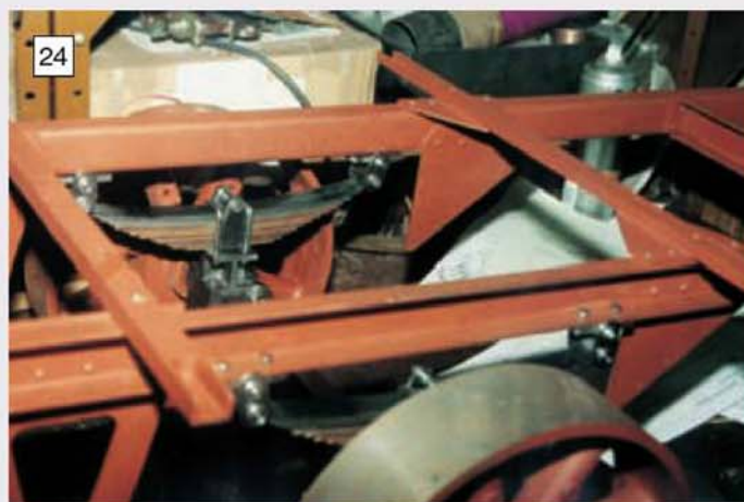
24 On Stan Nipper's wagon the Savage back spring design has been adapted to include two swing links.
