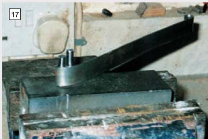
This simple jig is mounted in the vice and used to form the end loops in the top spring leaves. (Photos 17-20: John Thompson)
