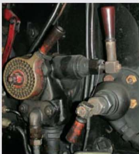
Above left, the brake valve made by Dave Noble and, above right, the real thing on 6106 (Prairie). Although generally the same shape, they do look rather different, plus the fact that the full size one doesn't have the dummy ejector control on the top.
