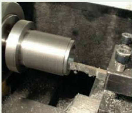
The internal taper in the chuck body is bored using the set-over top-slide.
