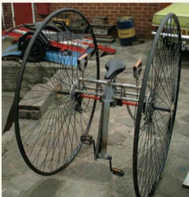
An initial assembly of the Di-Cycle was made for trial purposes.
