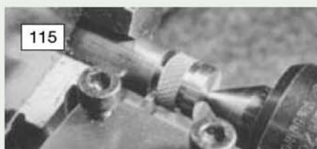
Parting off the final seat bolt nut.
