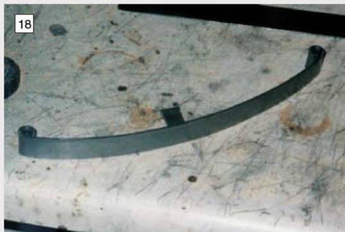
Formed to the appropriate curve, this front spring top leaf now has loops formed at its ends.
