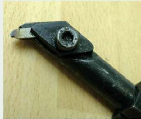
The tool used for internal screw cutting up to a shoulder. The boring bar is a commercial item.
