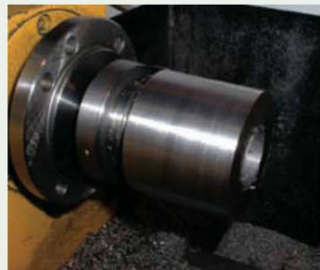
Fitted to the arbor, the chuck body is ready for threading the O/D and taper turning in the bore.
