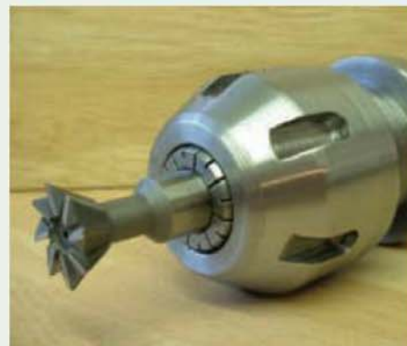
Shown here, a 60deg. dovetail cutter is firmly gripped by an ER collet in the Author's chuck.
