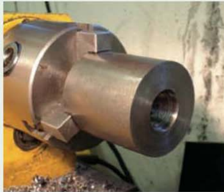
Here, the internal screw thread and arbor register have been machined into the chuck body.
