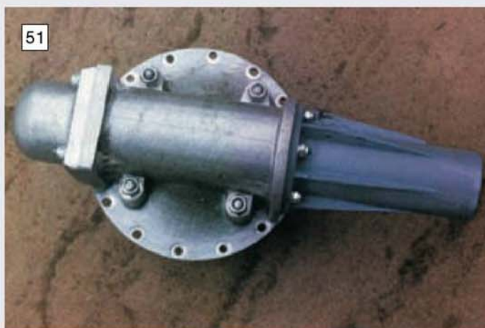
A top view of the assembled top cover. The four nuts hold the differential cage bearing caps. Note the holes for attachment to the axle casing.
