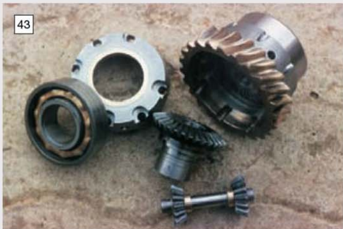
The partially dismantled differential assembly showing one of the 30 tooth bevel gears and the two 15 tooth bevel gears mounted on their shaft.
