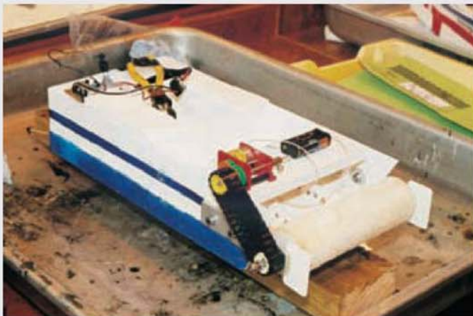
This design, from the Lochaber School in Fort William, used a paint roller to pick up the oil but lack of speed control spoilt their test run.
