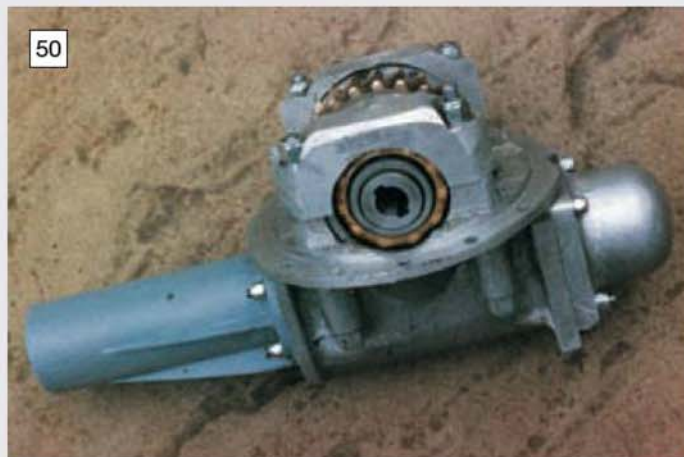
The top cover assembled with the differential cage and front and rear covers. The front cover is a steel fabrication.
