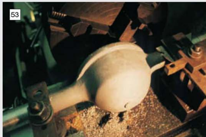
53 Further details of the machining of the rear axle casing. Note the method of attachment to the lathe cross-slide.
