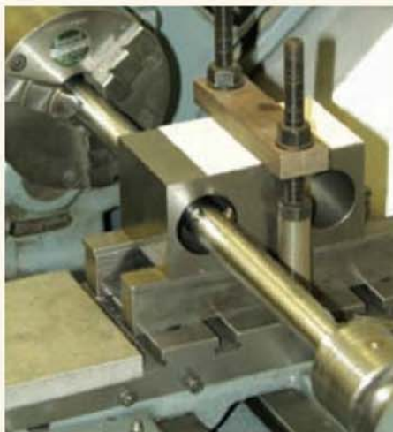
Boring a 5in. gauge Lion cylinder block using a between-centres boring bar. The cutting tool edge is ground to a large radius to produce a good finish in the bore, and the tool is gripped by means of a tapered cotter pin. Note the substantial work holding arrangement and the cover plate to prevent swarf ingress to the vacant top-slide mounting position.
