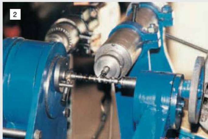
A close view of the working area of the machine set up in milling mode. A model internal combustion engine camshaft is being milled to the required profile using the end cutting face of a standard slot drill.
