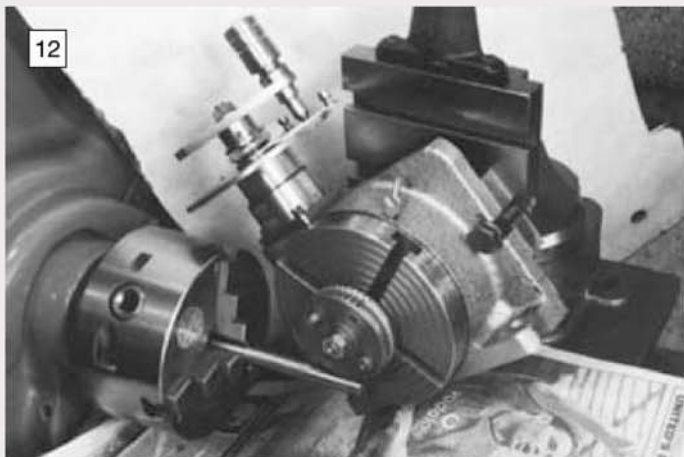
12 Gashing the gear teeth in one of the wormwheels. The teeth were taken to two-thirds of finished depth.
