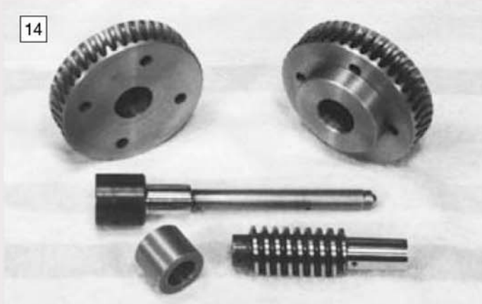
14 The finished wormwheels and worm. The latter item is hardened and polished to reduce wear in service.
