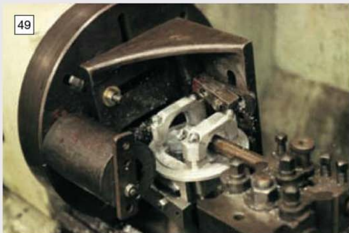
Boring the bearing seats for the differential cage. Note the complex lathe set up involving an angle plate, faceplate and balance weight.
