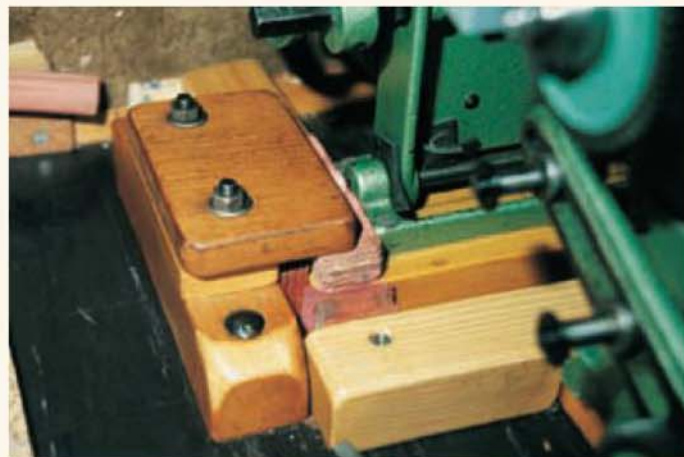
Close-up view of the countershaft mounts showing, in addition, the rubber washers fitted to the countershaft and the rubber wedge used to take up any residual clearance.
