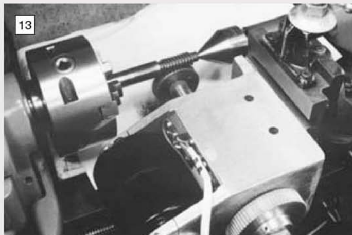
13 Hobbing one of the wormwheels with the previously finished hob. The work is mounted in the Author's mill/drill attachment with the drive belt removed.
