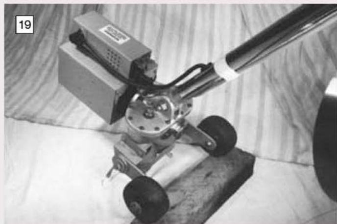
19 This photograph shows the top cover and pivoted handle mount. The main handle shaft is a chrome plated tube.
