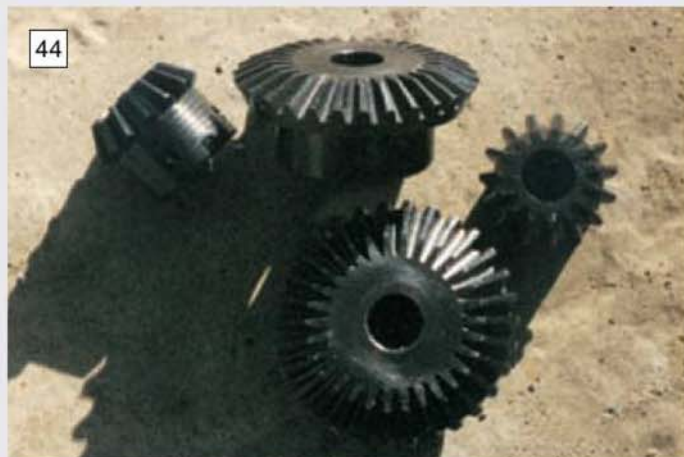
The set of bevel gears required for the differential assembly. These were bought in from an industrial gear supplier.
