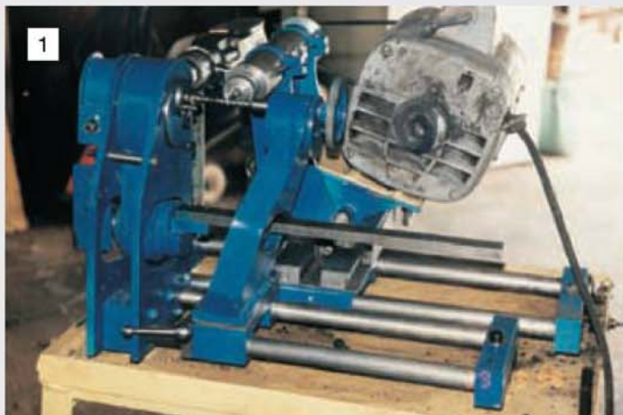
The prototype machine seen here in use in the Author's workshop. At this stage the machine is still under development and a pistol drill is in use to drive the work head until an improved drive can be developed.
