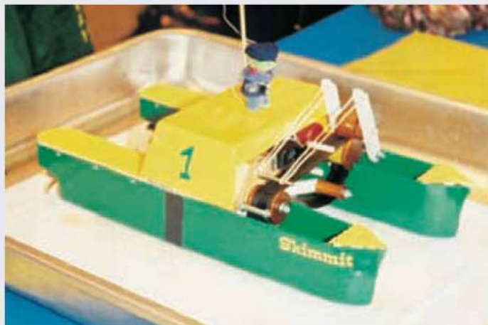
Skimmit was a catamaran fitted with a transverse collection belt with rollers to squeeze out the oil into the hull.
