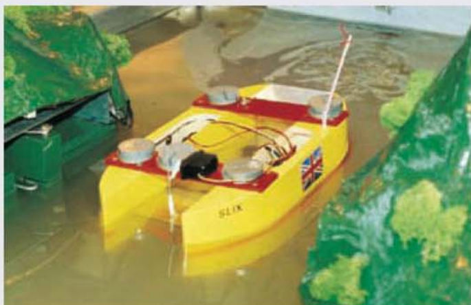
The winning entry negotiates the narrow inlet in the test tank with its plate lowered to pick up the oil.
