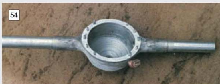
54 The finish machined rear axle casing. Some internal machining has been carried out to provide clearance for the differential cage and bearings.
