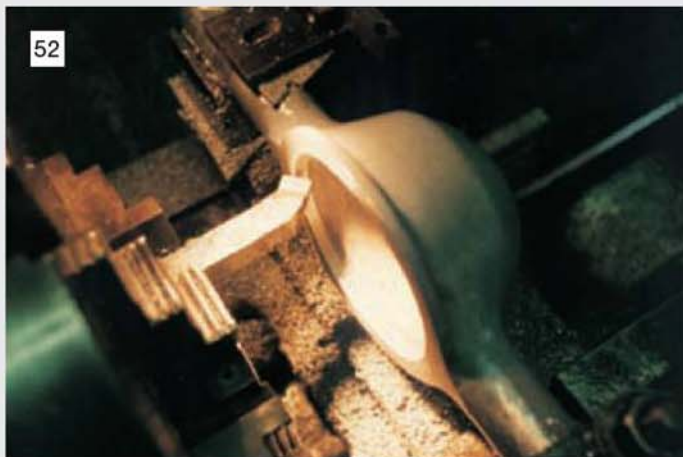
52 Machining the rear axle casing with the workpiece attached to the lathe cross-slide and boring and facing taking place from the lathe chuck.
