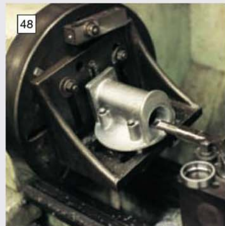
Boring the drive worm bearing seats in the rear axle top cover.
