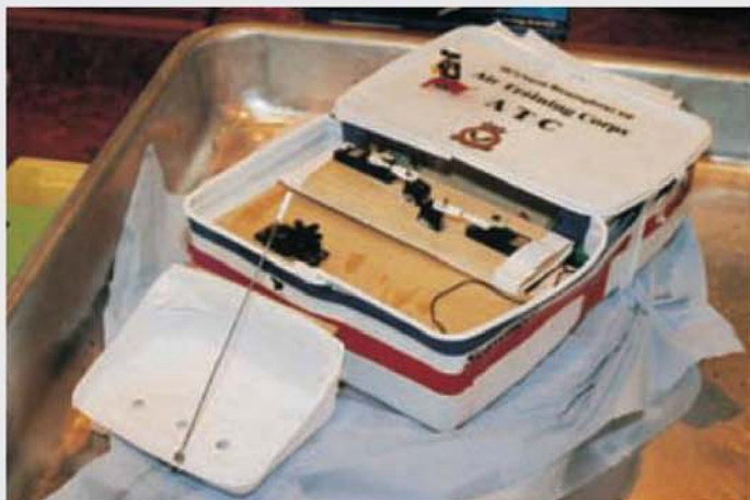
The team representing 487 (North Birmingham) DF ATC from West Midlands used a simple hull with a front mounted scoop.
