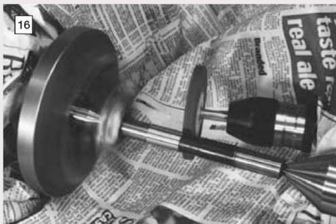
16 The grinding operation under way. Newspaper was used to prevent the grinding debris getting into the slides or bearings of the machine.
