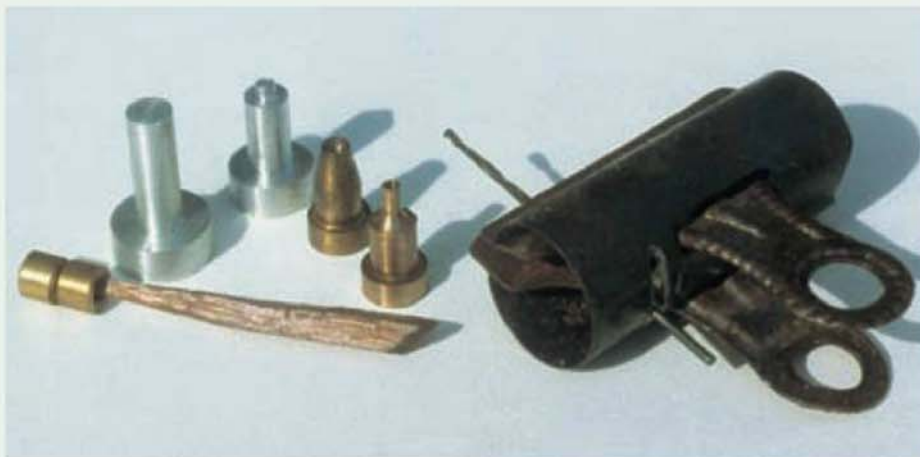
This photograph shows the various items referred to by the Author during his description of the construction of his flap valve injector. A set of brass cones are also shown.
