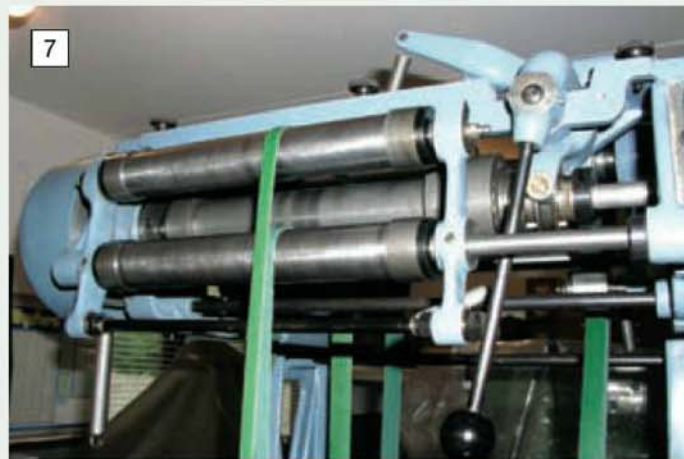
Another view of the countershaft showing the work head driving drum and tensioning pulleys. The clutch can be seen to the right of the photo.
