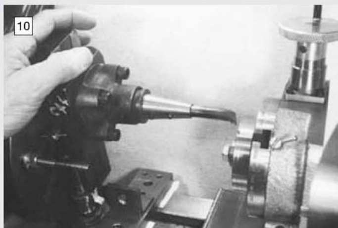
10 The method used to machine the cam. Each of the six segments was machined by laboriously pulling the cutting tool down by hand.
