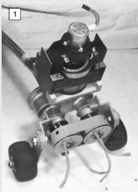
The complete micro-cultivator with the electrical cover removed to show some of its construction.
