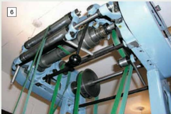
The countershaft assembly as viewed from below. Each shaft is mounted in self aligning ball races.
