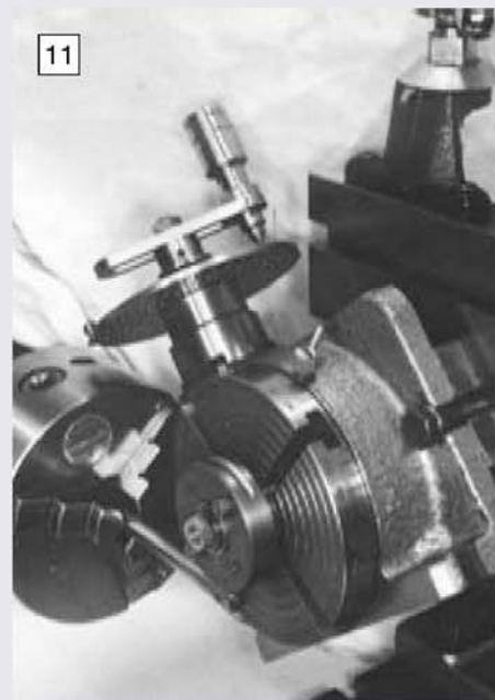
11 Cutting a depression in the periphery of the gear blank prior to gashing the teeth.
