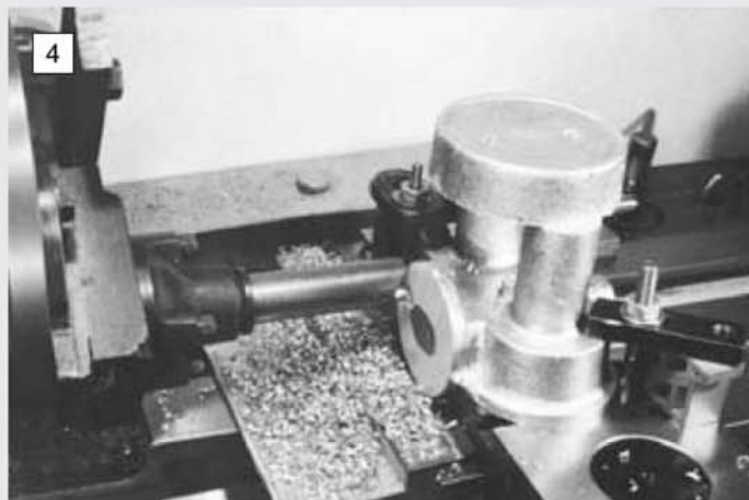
The motor flange being machined square with respect to the previously finished face. The time bearing housings are set square to the lathe bed.
