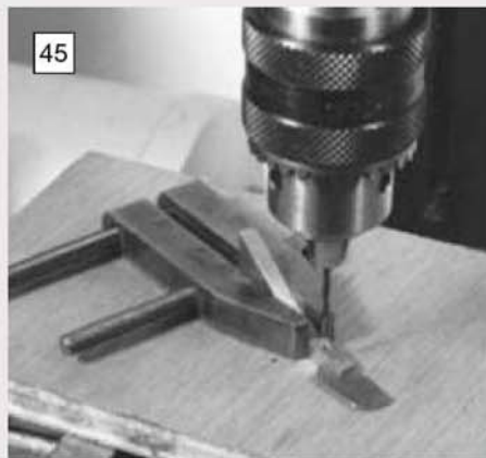
Drilling the No. 55 hole for the lower blade.
