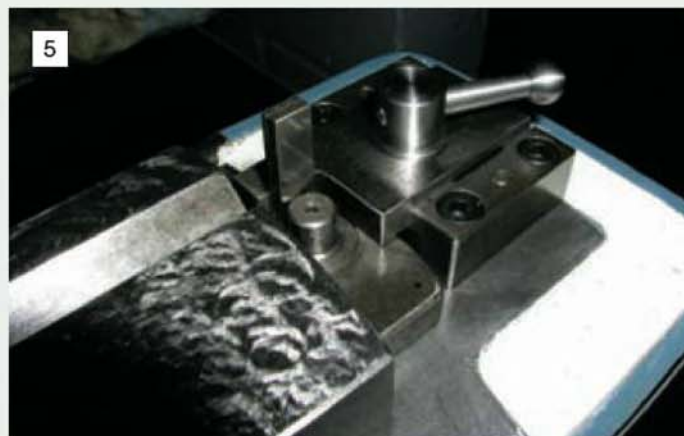
Work table angles can be set directly using a slip stack nipped between a fixed plate (reversible) and a pin attached to the top swivel table.
