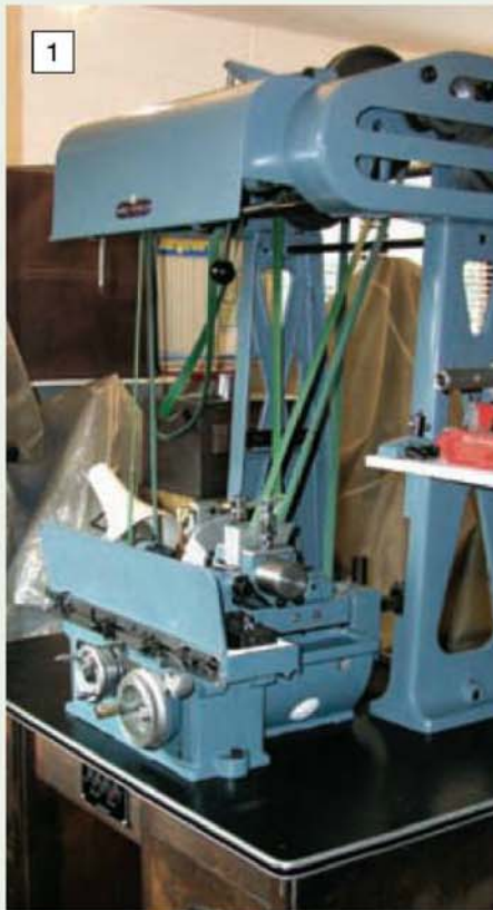
The Author's Jones and Shipman Fig. 520A Bench Precision Grinding Machine viewed through the workshop door.
