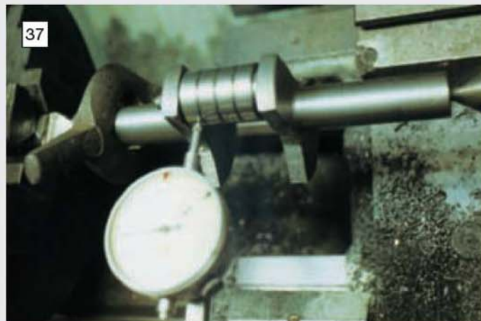
Checking both ends of the mainshafts and both ends of the crank pin with a dti to ensure everything is in alignment.
