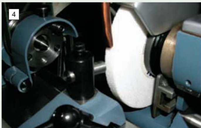
The external grinding wheel undergoing dressing using a diamond mounted in a rigid bracket clamped to the machine's table.
