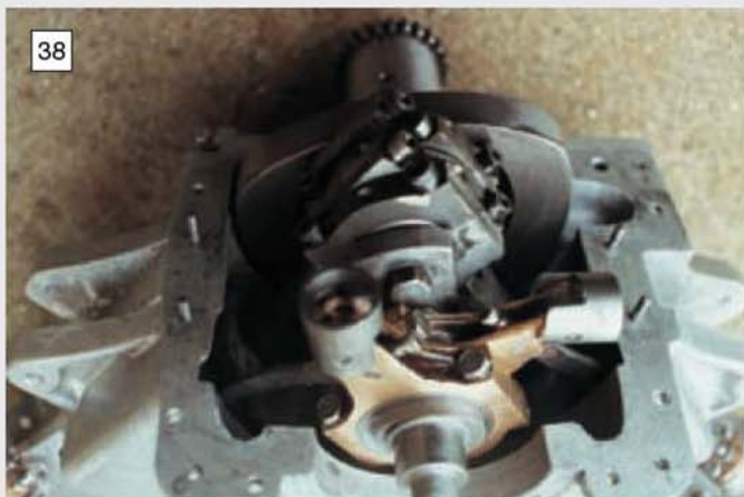
38 The underside of the assembled crankshaft showing the eccentric straps/rods and their pistons, big ends, joint studs, gear adaptor and first gear.
