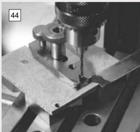
Set-up for drilling the lower blade.
