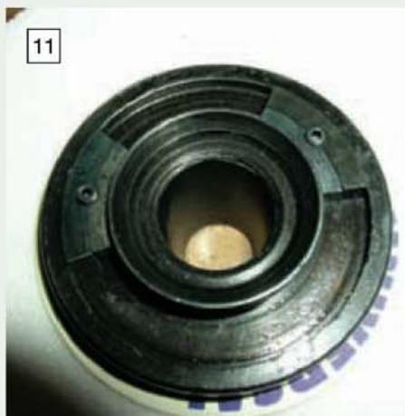
The balancing weights fitted to the external grinding wheel mounting hub.
