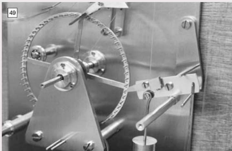
The maintaining work unit fitted on the clock.
