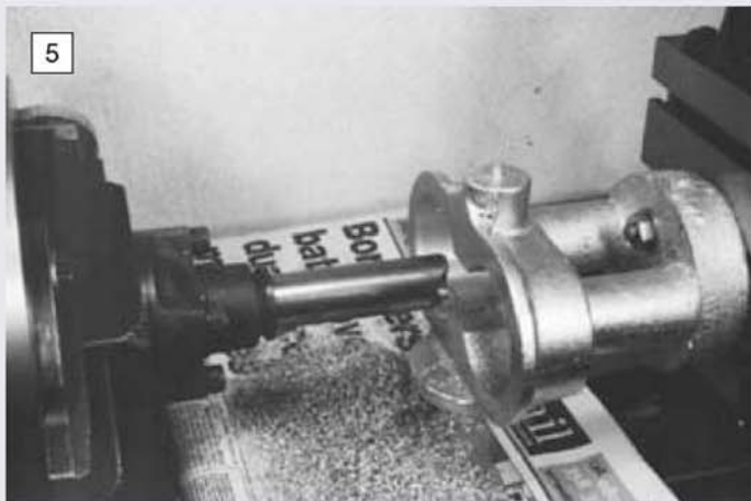
Boring the gear cavities to the correct gear centre-distance; note how the casting design has been arranged to facilitate work holding.
