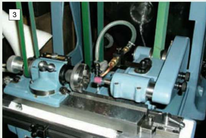
Here the machine has been converted into an internal grinder using a live spindle work head and bore grinding spindle.
