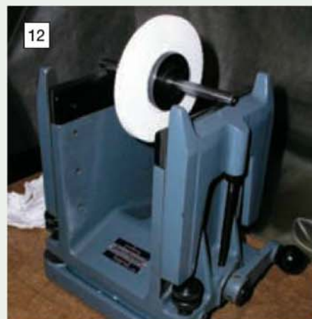
The J & S knife edge balancing unit seen with a grinding wheel mounted on the test mandrel.
