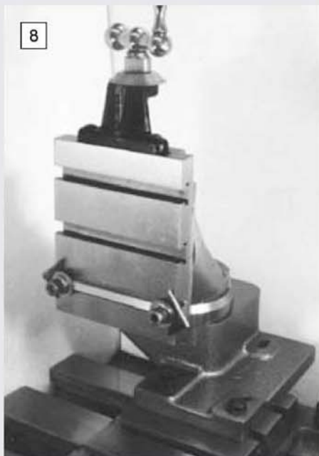
8 The method used to mount the piece of tool steel used as a cam follower.
