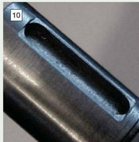
The keyways in each of the shafts had been carefully filed up to remove burrs.
