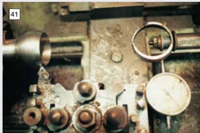
41 Finishing the sphere using auto-traverse to the left leaving 0.01in. stock for a final finishing pass to zero on the dti.
