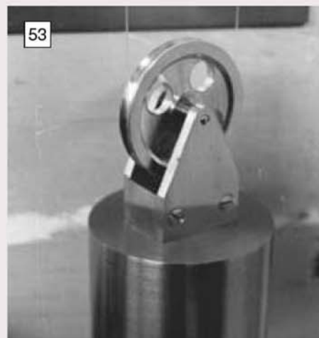
The pulley assembly secured to the driving weight.
