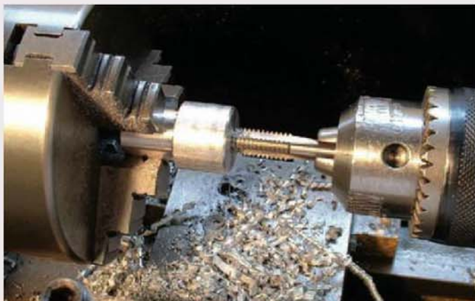
Tapping the draw bar nut using a tap mounted in the tailstock drill chuck to ensure correct axial alignment.
