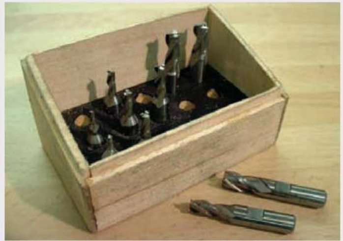
A set of three-flute cutters ideal for use with the adaptor described. These cutters can be used for both end milling and slot drilling operations.
