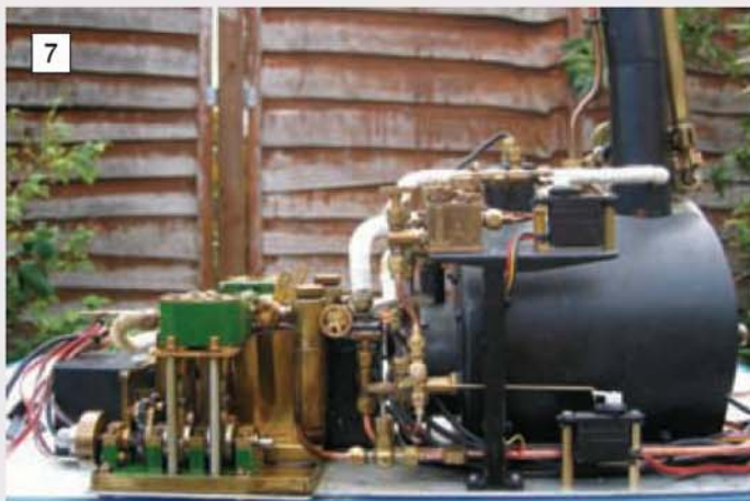
Between the vaporising coil and the gas control valve are two isolating valves, the upper being manual, the other servo controlled.
