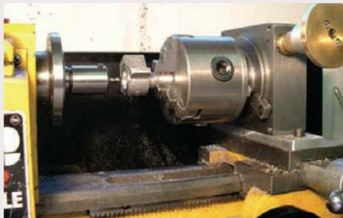
Using the milling cutter adaptor to machine a small component mounted on the rotary table located on the lathe's cross slide.
