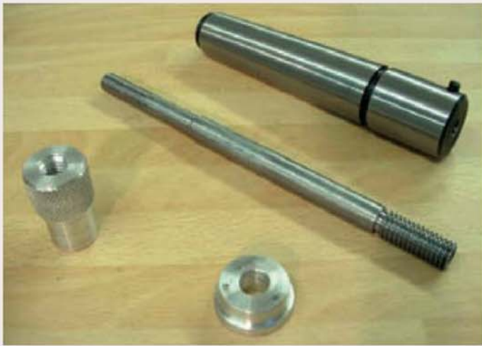
The project to be described. The milling cutter adaptor at the top of this group is shown with its draw bar, spindle plug and nut.
