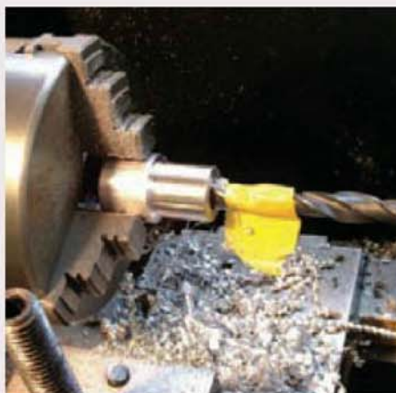
Controlling drilling depth by using a piece of insulating tape as a marker.
