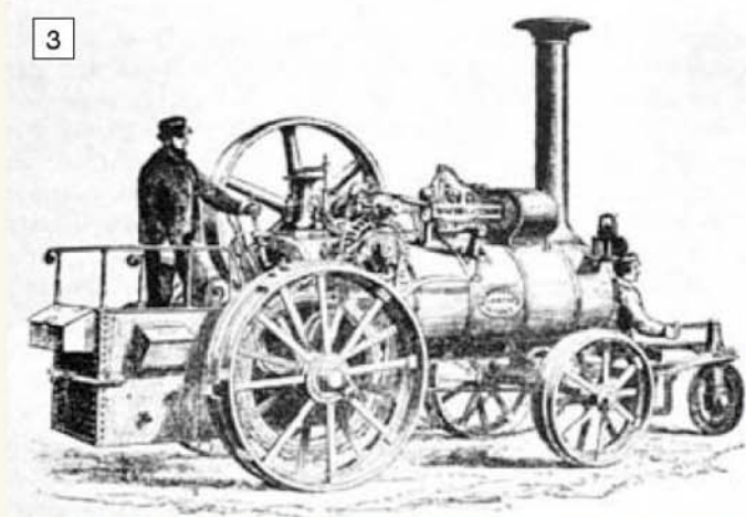
Left: an early Garrett chain engine using Aveling's patent fifth-wheel steering. Right: Garrett's first gear-driven traction engine built in 1876. The Stephenson valve gear is clearly on the other side of the engine, so what might be mistaken for the valve chest cover must be for another purpose.
