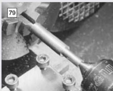
79 The other end is reduced to \frac{1}{4} in. diameter.
