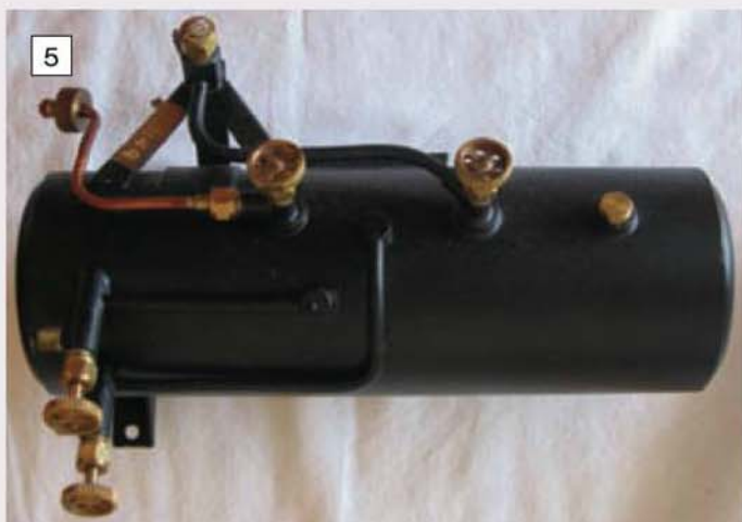
Left: after removal of the copper strips to combat the cooling effect of gas extraction, the fuel gas tank was tested certified and painted.
