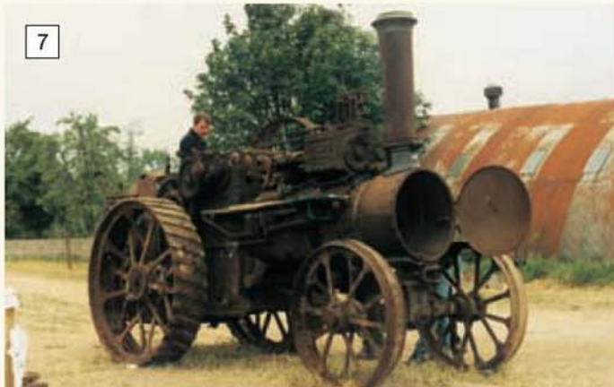
This 6nhp engine was in a sorry state when photographed. I believe the engine is No. 33068 completed in June 1918.
