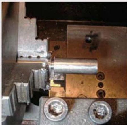
Using a parting tool to create a run-out groove prior to screw cutting.
