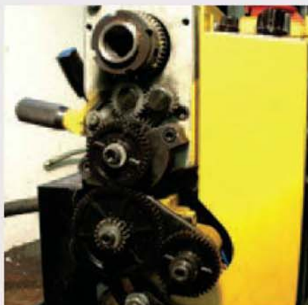
The gear train set up for screw cutting 16 threads per inch.
