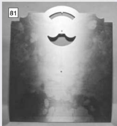
81 The \frac{1}{16} in. brass dial plate takes shape.
