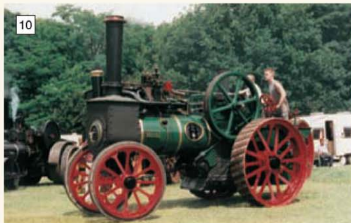
A 6nhp single cylinder superheated Garrett completed in August 1911. Note the prominent smokebox shape and plethora of pipework.
