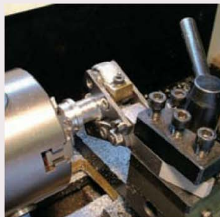
Knurling using a caliper type knurling tool. This tool relieves the lathe of excessive knurling loads.
