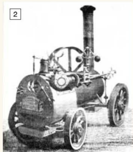
Left: an 1852 portable engine, the firebox is 'wet' having water all the way around it. The bottom row of fire tubes would be below the level of the grate. Right: by the end of the 1850s Garretts were using the more usual locomotive boiler.
