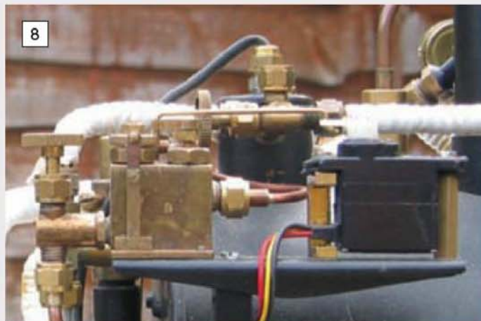
The gas control valve (left) operates under the control of the boiler control unit by means of the servo (right)
