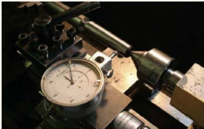
Setting the top slide angle using a centre and a dial test indicator. The DTI reading should not vary throughout the top slide's travel.
