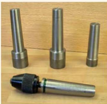
A selection of Morse taper shanks with one adapted to fit a small chuck.
