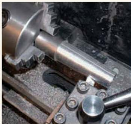
Turning a taper using the top-slide set round to the required half angle.
