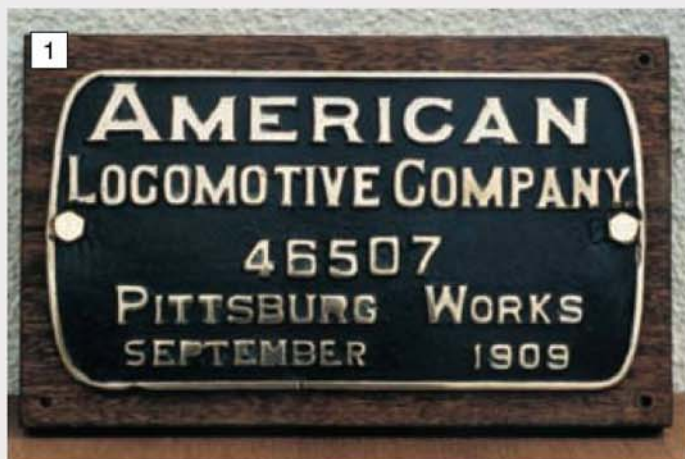
An early brass Alco plate of the new standard layout; the contemporary spelling of Pittsburgh is correct. The plate was from a Western Pacific 0-6-0.
