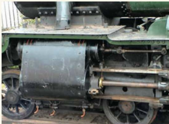
Rear view of Manor cylinder; note the round valve rod and glands.
