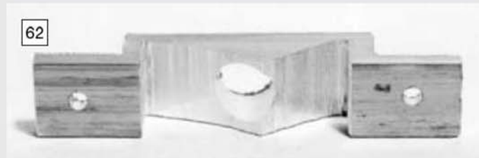
62 Diagonal cuts are made to remove some of the waste material.
