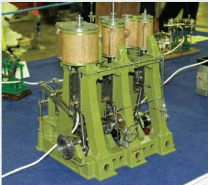
Two views of Peter Southworth's superb model of a Hawthorn Leslie 4,500hp triple expansion marine engine fitted with Marshall valve gear, patented in 1879 and derived from Hackworth valve gear. F. C. Marshall was a managing director of Hawthorn Leslie which built the ship Hanoverian launched in 1902 with a displacement of 24,140 tons and equipped with two full-size engines which the above model represents. Two 18ft. 6in. propellers drove the ship at 15 knots; it was sold to White Star Line in 1903, renamed Cretic and eventually scrapped in 1929.
