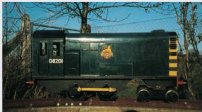
Mr. Geoff King's has modified his '08 shunter by fitting a leading 4-wheel bogie to negotiate the tight curves on his garden railway in Co. Sligo.
