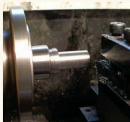
Preparing to cut the thread. The taper is mounted in an appropriate sleeve in the lathe headstock.
