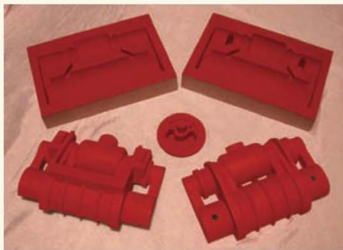
Penrhos Grange cylinder patterns with core boxes and rear cover.
