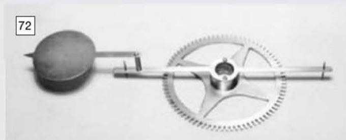
The hour pointer assembly can be made and dismantled as required.
