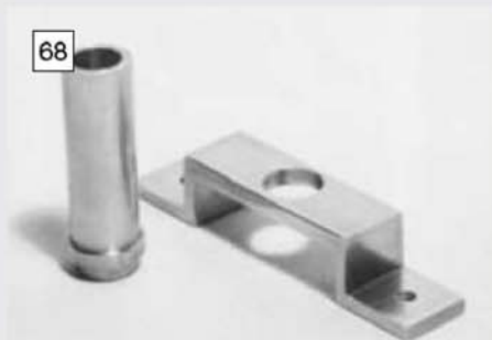
Bridge and pipe ready for assembly.
