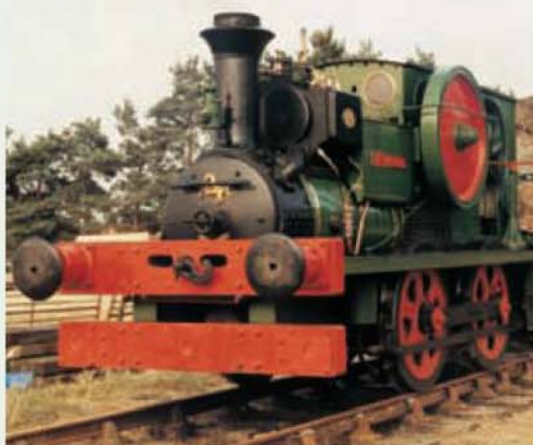
Left: Aveling & Porter Compound Tramway Locomotive called Sir Lancelot. Right: the Aveling & Porter type FGR wagon works number 8949 completed in November 1918. Note the 'Y' cast wheels at the back, the rubber tyres and the Ackerman steering.
