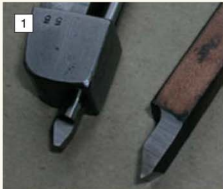
Two examples of screw cutting tools. That on the right is ground from a parting off tool.
