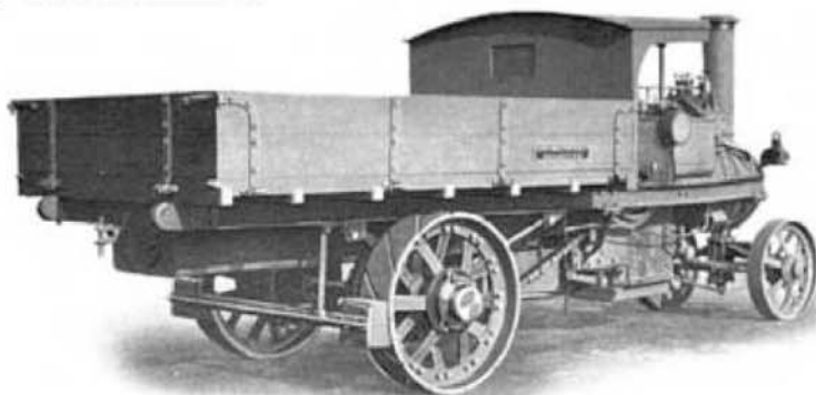
An early Aveling Wagon with steel shod wheels.
