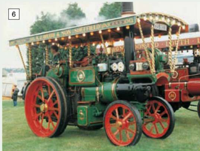
Left: a piston valve engine No. 11137 completed in March 1925; weight 8 tons. Right: sadly 31 (to date) Aveling & Porter rollers have been converted for duties they never performed in their working lives. In this case steam roller No. 7778, completed in October 1912 has become a showman's engine.
