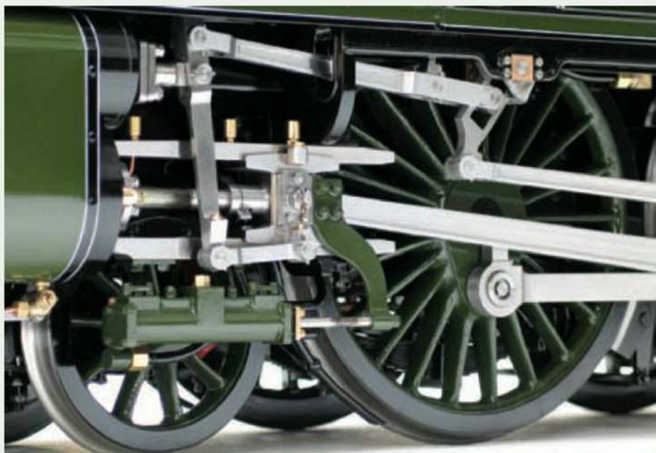
Valve gear on the King Arthur is of ample proportions, giving plenty of room to fit bronze bushes and to retain the motion pins with taper pins as full size practice.
