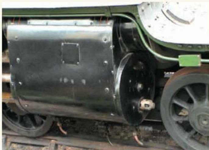
Manor cylinder; note the cleading.
