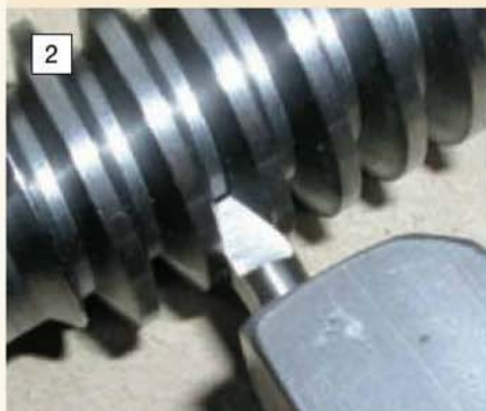
An example of a left hand, 20DP worm turned using the inserted bit type of tool shown.
