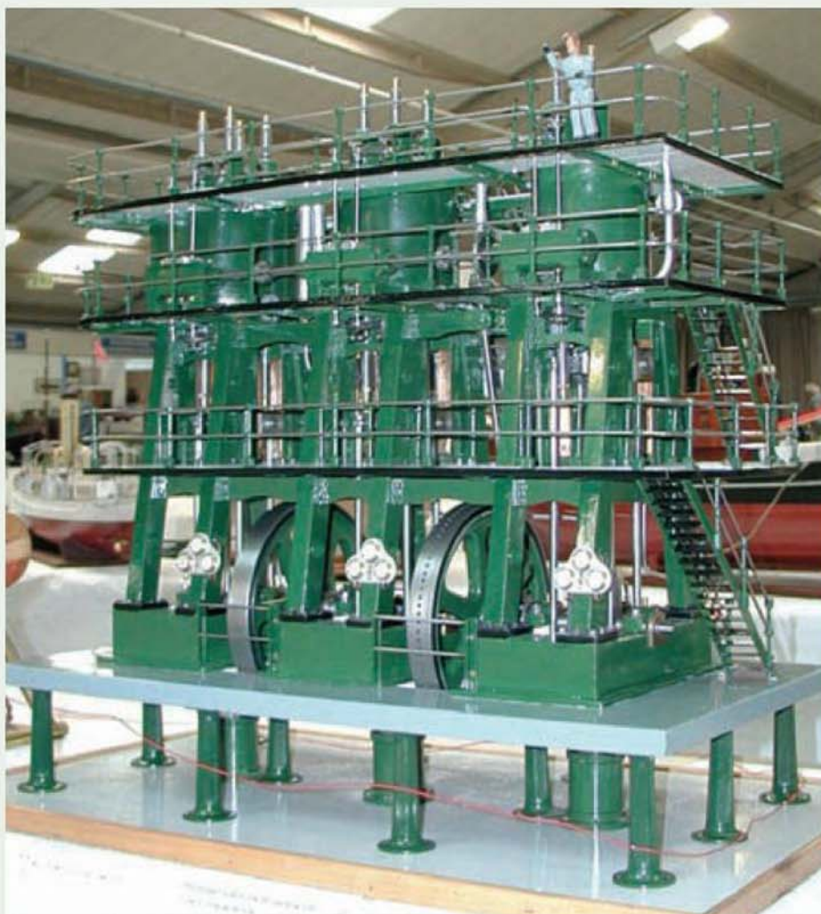
Dave Whalley's fine model of the magnificent No. 6 engine, one of two triple expansion engines installed at Kempton Park Waterworks. Standing 34ft. from bedplate to valves, the full-size engine developed 1008hp at 25rpm to operate three 30in. diameter x 66in. stroke ram pumps and pumped 24,000,000 gallons of water per day. The high, intermediate and low pressure cylinders diameters are 29, 54 and 86in. respectively.
