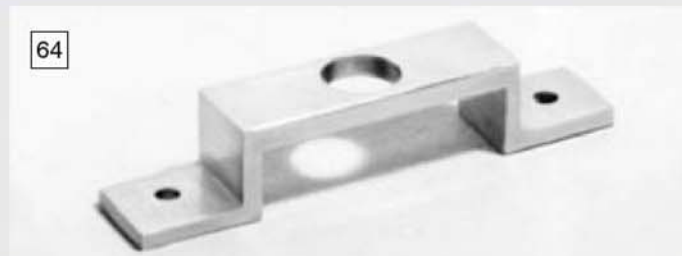
64 The bridge is finished by careful filing to size and shape.
