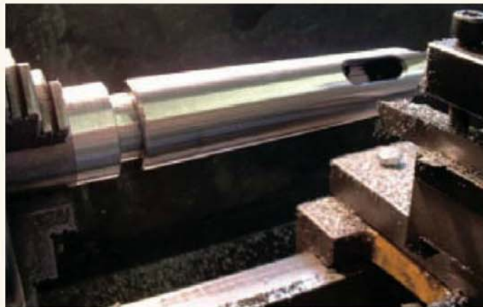
Checking a turned taper for fit in a commercial Morse taper sleeve. The quality of fit can be determined using engineers blue or a marker pen.
