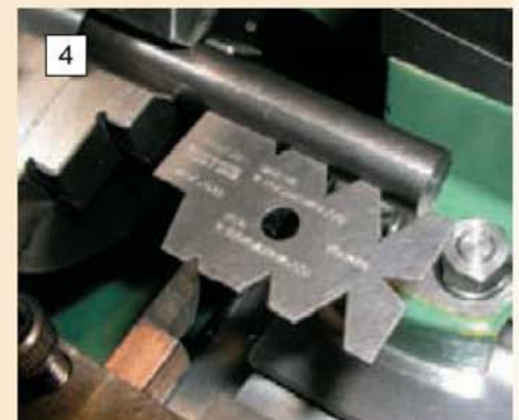
Using the screw cutting gauge to set the screw cutting tool square to the work.
