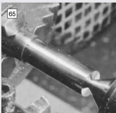
65 The pipe is faced, centred and turned to size.
