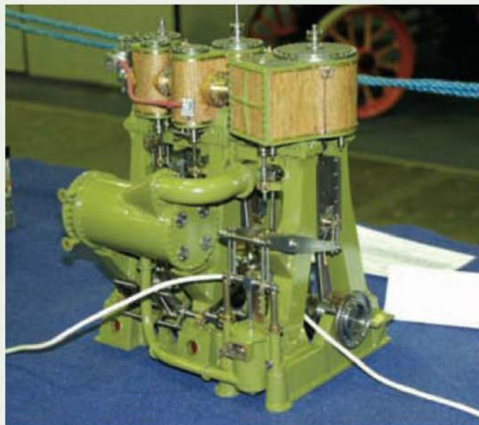
Two views of Peter Southworth's superb model of a Hawthorn Leslie 4,500hp triple expansion marine engine fitted with Marshall valve gear, patented in 1879 and derived from Hackworth valve gear. F. C. Marshall was a managing director of Hawthorn Leslie which built the ship Hanoverian launched in 1902 with a displacement of 24,140 tons and equipped with two full-size engines which the above model represents. Two 18ft. 6in. propellers drove the ship at 15 knots; it was sold to White Star Line in 1903, renamed Cretic and eventually scrapped in 1929.
