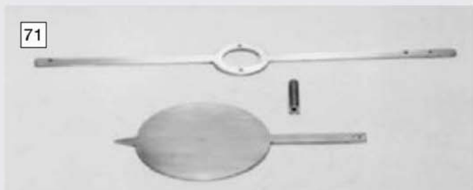
Hour pointer, arm and tapped fixing post before assembly.
