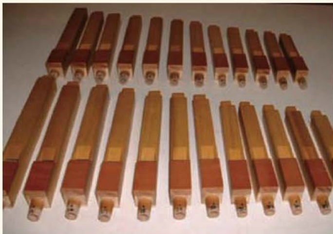
The violin pipes laid out prior to installation. Note the code numbers on the mounting spigots.
