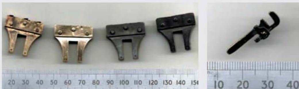
Mr. David Halfpenny's lost wax cast axlebox pedestals are straight from the packet, pickled, wire brushed, treated with browning fluid, buffed and oiled. The tiny wrench (right) has been buffed to show highlights and shadows.
