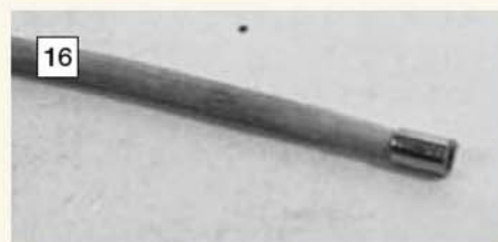
A steel bearing impaled on a length of pegwood and ready to offer up to the burnishing steel wire brush shown above (photo 15).
