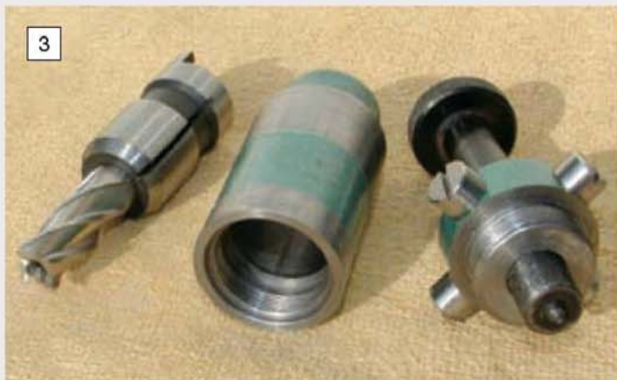
The barrel dismantled to show the main components. On the left is the cutter in its collet and on the right is the 'breech-block'.
