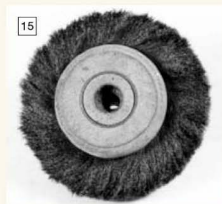
A soft steel burnishing brush; the wire in this particular brush is only 0.002 in. diameter.
