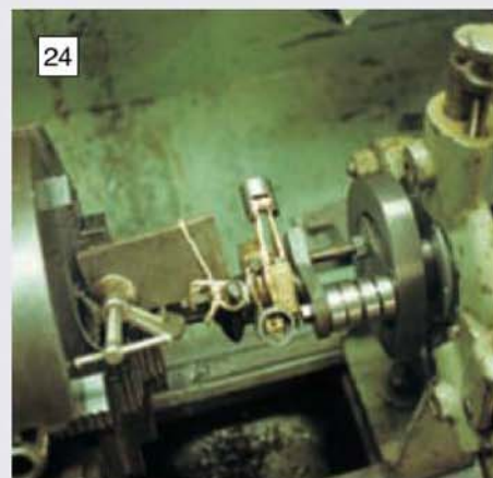
A test assembly of the crankshaft in the lathe. Note the use of a bolt as a jack to prevent the crankshaft distorting.
