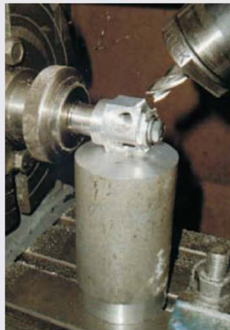
Machining a chamfer on the gearbox. The length of the support bar is machined to facilitate work setting.
