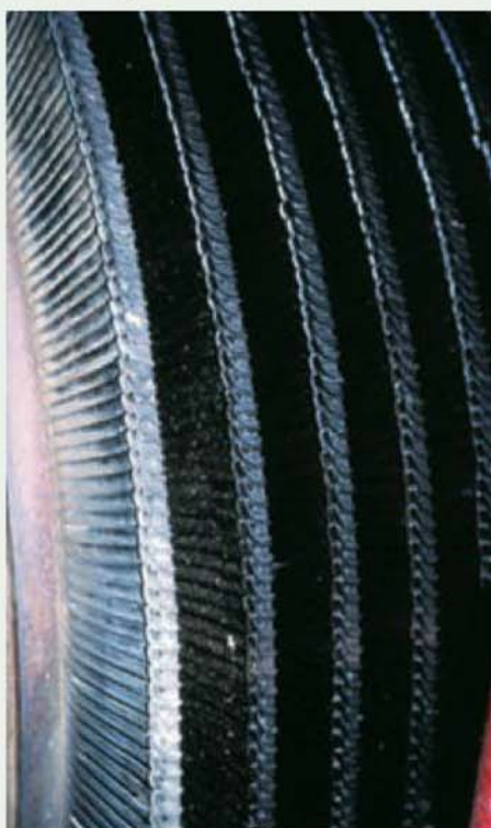
Turbine blades from TS King Edward, the first turbine engined commercial ship.
