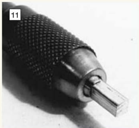
A method of holding \frac{1}{8} in. square brass.
