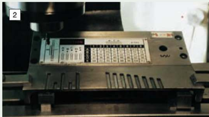
Milling the grooves leading to the 5mm dia. pin holes in the gearbox cover plate on the milling machine.
