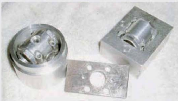
Left: turning fixture for boring cam boxes. Centre: drill jig for fins. Right: drill jig for top body.
