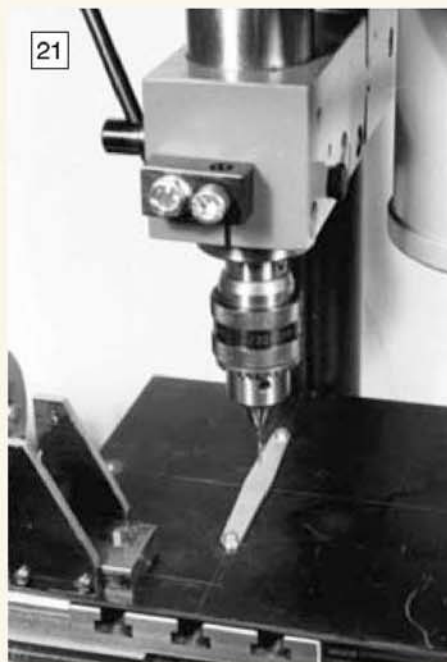
Drilling the pivot holes in the bridge piece and back plate.
