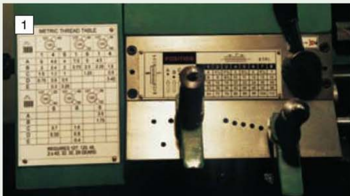
The original design of quick-change gearbox cover plate and metric screw cutting table fitted to the Warco BH600G lathe.
