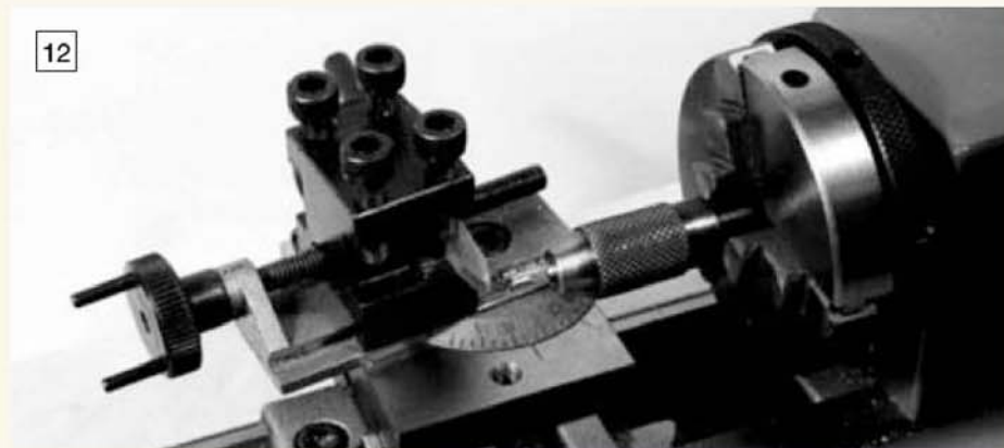
Machining the chamfer in the Unimat 4 lathe.
