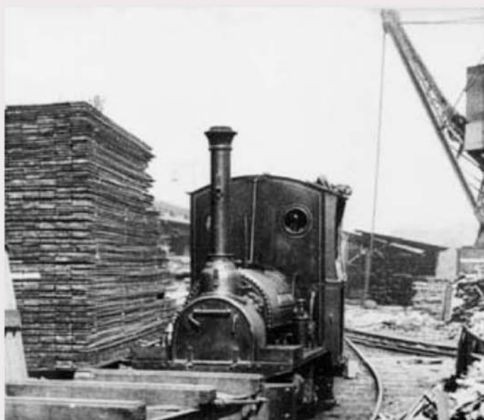
Manning Wardle 482 of 1873 Albert Edward seen at work in the Arsenal in 1918. The engine had been fitted with a new boiler by its owners in 1914, hence the peculiar horizontally hinged smokebox door and Neath pattern spark arrester. Albert Edward was sold to J. F. Wake of Darlington in 1919.
