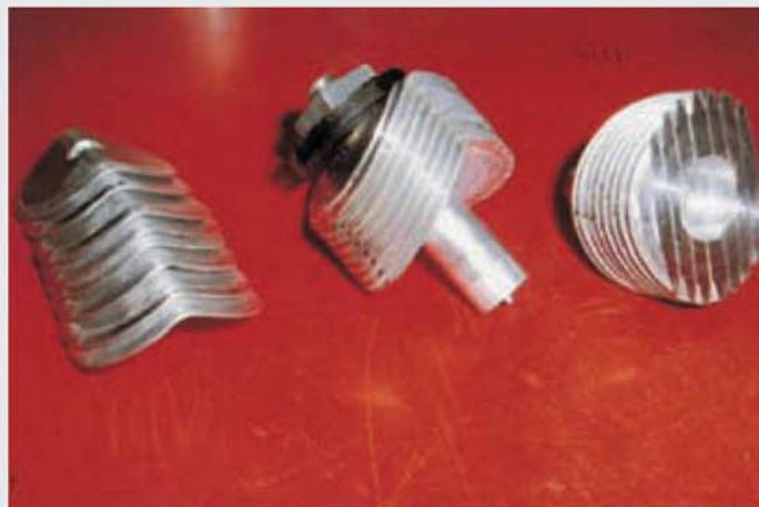
Left: Stack of cam box blanks after machining and bending. Centre: stack bonded together on a temporary pin. Right: faced to length and bored.
