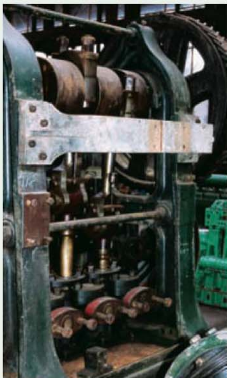
The three-throw hydraulic pump used to power the swing bridge at Aberdeen harbour.
