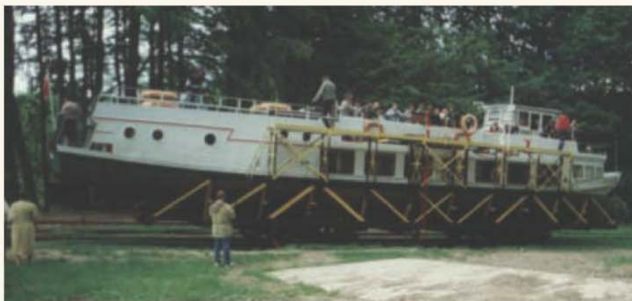
A canal boat makes its journey along the railway. The system accommodates boats up to a maximum of 24.5 metres in length.
