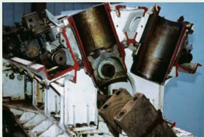
Cut away for training submarine engineers, this 'Polar' diesel engine is from HMS Oracle.
