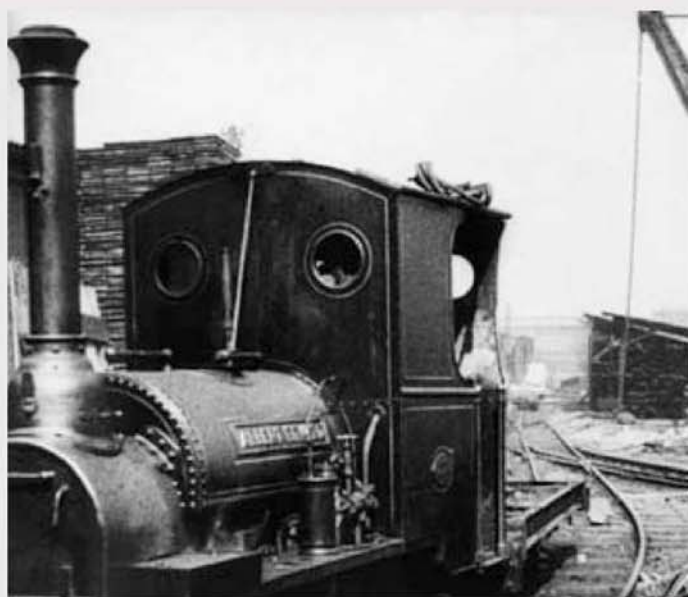
This view of Albert Edward shows in close-up the modifications made to the cab at the Arsenal. Also in evidence is a replacement injector, apparently used in conjunction with an original pattern water inlet cock on the saddle tank.
