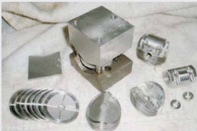
A photograph showing the various stages in producing the cam boxes. The sequence is explained in the text.
