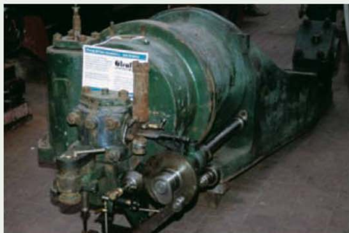
This gas engine from Aberdeen harbour swing bridge was originally used to create the necessary hydraulic power.
