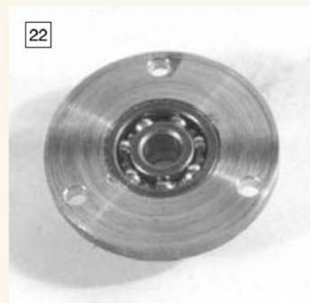
A ball race secured in its housing by two light pin punch indentations.
