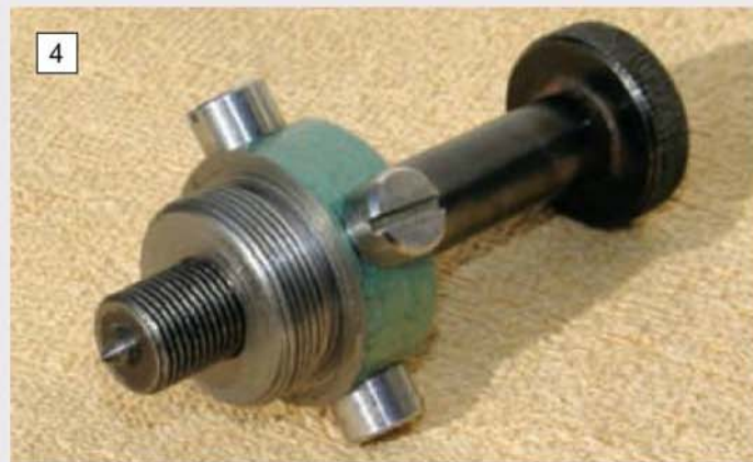
A view of the breech-block assembly showing the indexing studs and the centre or 'blocking pin' which supports the cutter during sharpening.
