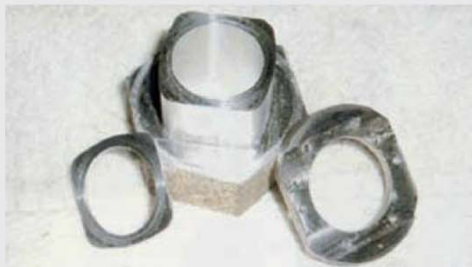
Left: Parted off bottom flange. Centre: Bar machined to profile. Right: Drill jig for gearbox and adaptor.
