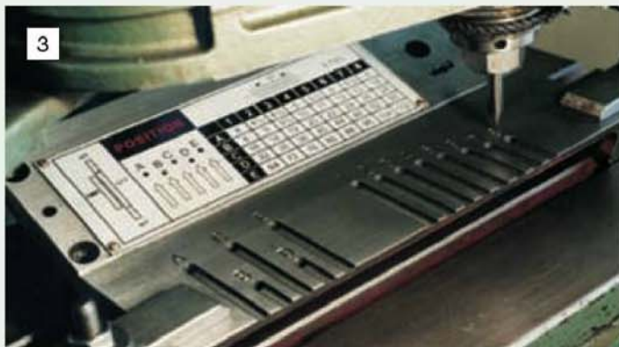
Engraving the identification letters and numbers on the cover plate. Other methods are described in the text for those without engraving facilities.
