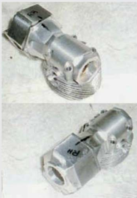
Rear cam boxes shown with their gearbox and adaptor. Note the aid to identification on the lower sample.
