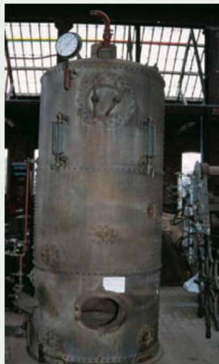
This vertical boiler was originally from a small steam ship and later used for soil sterilisation.
