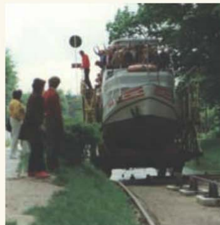
A canal boat being carried out of the water on one of the specially built platforms.
