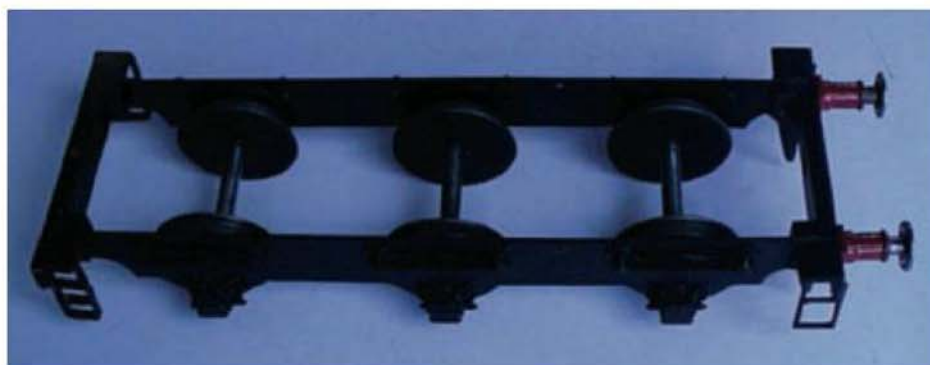
The tender chassis of our gauge 1 locomotive is of conventional construction, unsprung but with vertical and lateral play of the axles in the axleboxes.
