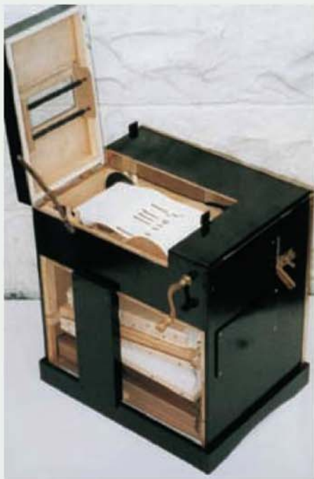
Rear view showing crank handle, pressure box lid open and shallow duct at back for tubes to bass notes in base.
