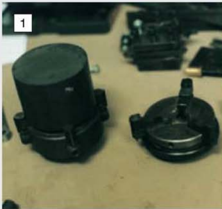
The Unimat 4-jaw chuck can just accommodate the cast iron bar for the toolpost to face its ends.
