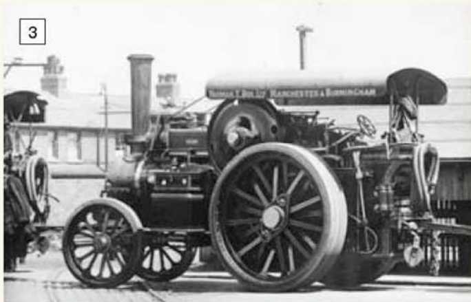
A good 'working' picture of a famous Norman Box engine, in this case Atlas, Works No. 17105 built in 1928. The engine is class B6, weighs 16½ tons and is rated 8nhp. The picture was taken at the same occasion as photo 2. Another equally clear photo of Vulcan survives.
