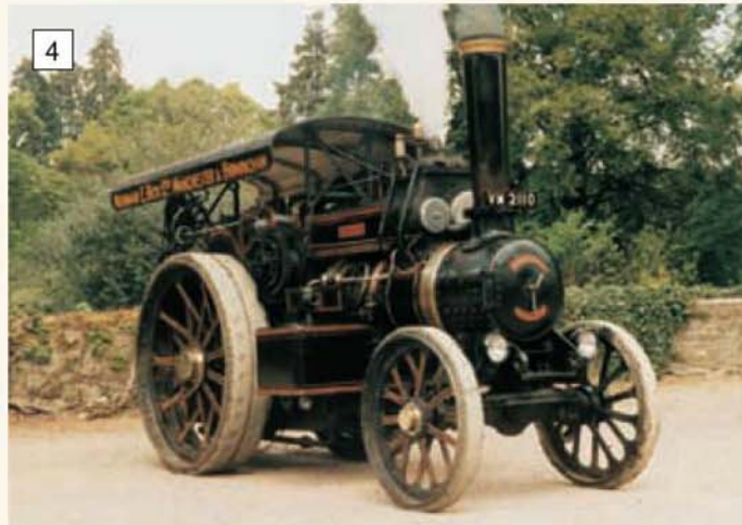
Happily, Atlas has survived into preservation. Note the crane fixings on the fore carriage, and winch drum under the crankshaft.
