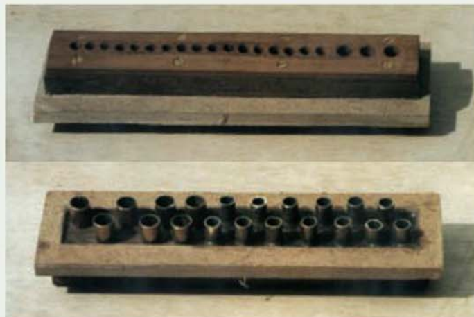
Top and bottom views of the tracker bar.
