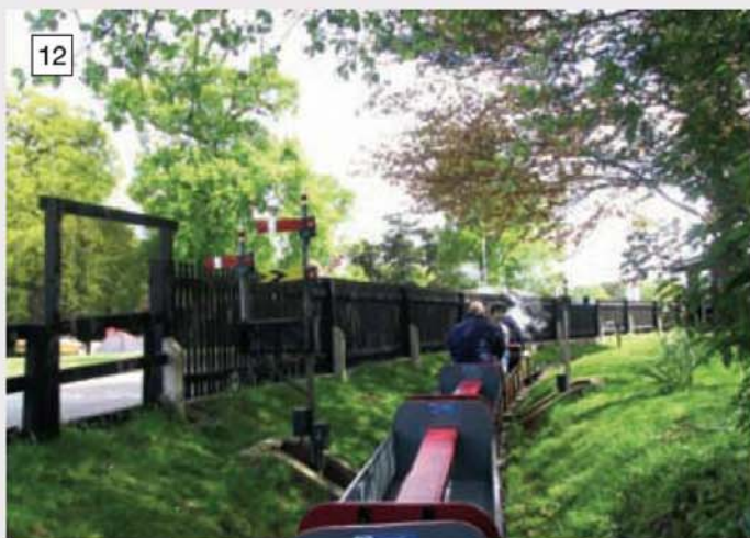
This double signal indicates our route into/through the station.
