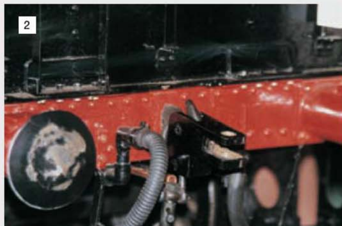
In order to use the device it is then dropped down into the horizontal position ready to be coupled to the flat draw bar.
