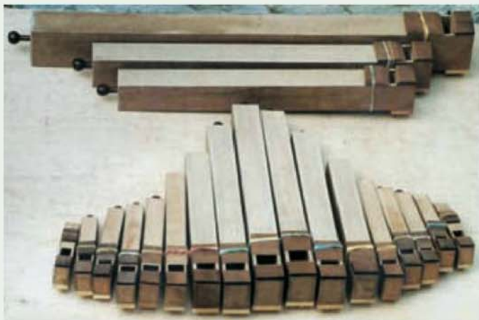
The set of 20 pipes with rubber bands securing top caps prior to voicing.
