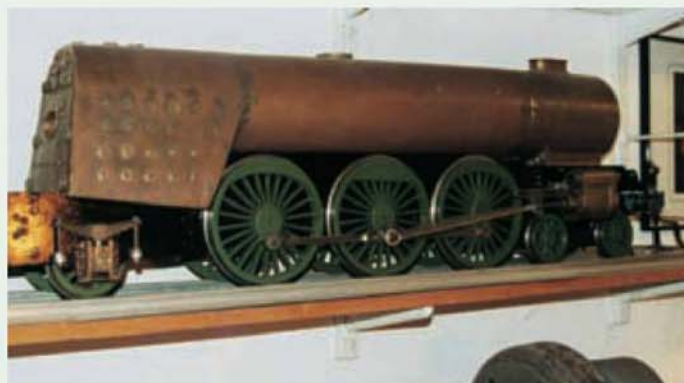
A 3 1/2in. gauge LNER Peppercorn A1 based on a modified Hielan' Lassie chassis with 3-cylinders and correct rear framing. (Photos: Paul Wiese)
