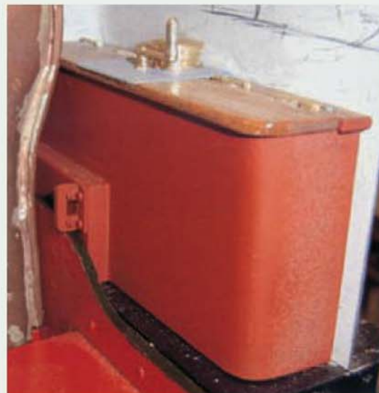
RH cab seat. Note bracket for supporting drain cock operating rod. (Unsatisfactory wood tops to be remade.)
