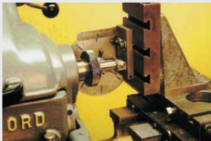
The fixture in use. The cutter is driven by the lathe mandrel and the work fed towards the operator.
