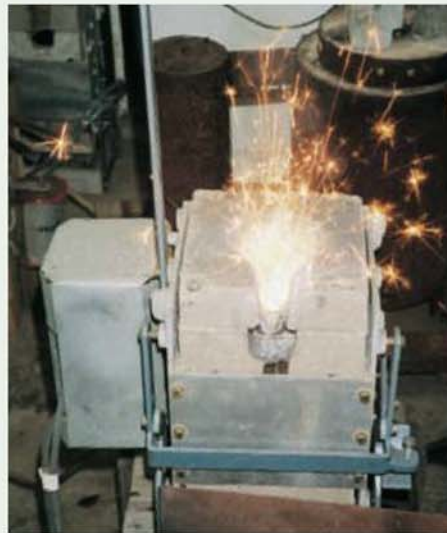
Reaction with the carbon in the pulverised coke reduces the melting temperature of the steel.
