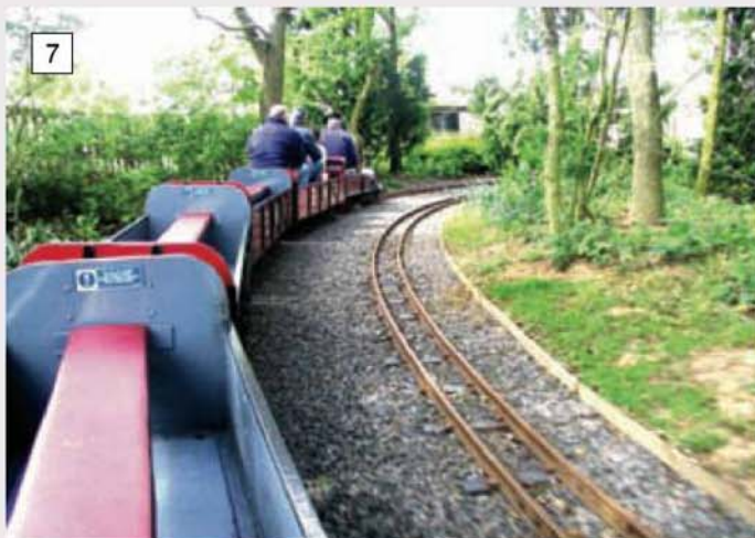
This view shows how the passenger stock keeps feet safely inboard.
