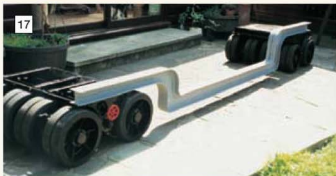
One of the six fabricated beams on Mervyn Greeves' fully detailed 3in. scale model of the Fowler double swan neck trailer.
