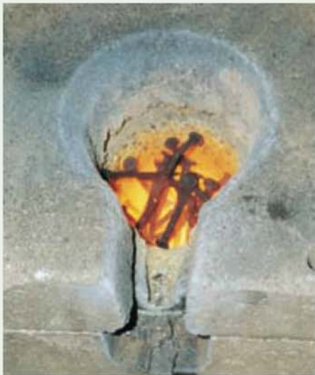
The furnace is charged with layers of rusty nails, pulverised coke and ferrosilicon.
