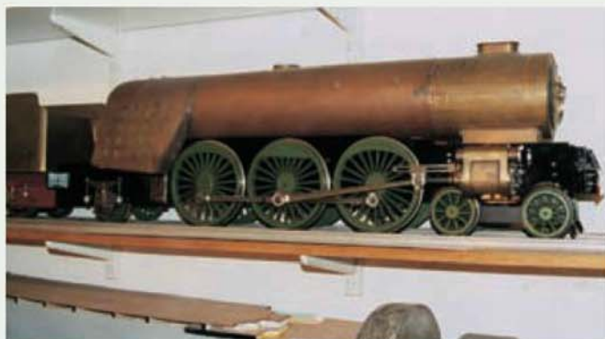
A 3 1/2in. gauge LNER Peppercorn A1 based on a modified Hielan' Lassie chassis with 3-cylinders and correct rear framing. (Photos: Paul Wiese)
