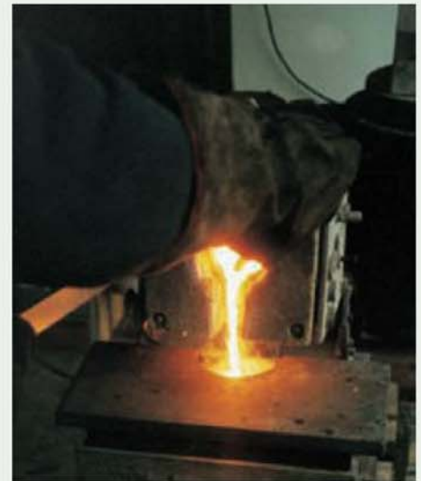
Ferrosilicon controls the form of the carbon in the resultant iron, ensuring the casting is not hard.
