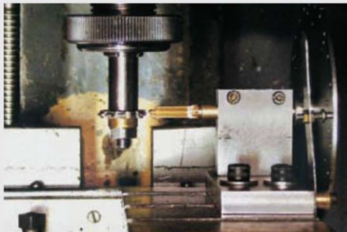
A bird's-eye view of the set up shown at left. Indexing is by use of the division plate and spring detent shown to the right of the photograph.
