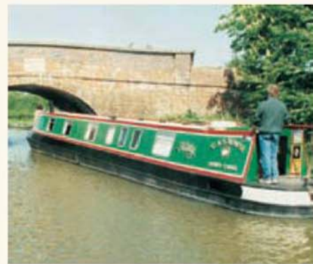
A typical 6ft. 6in x 72ft. UK narrow boat. A cabin has been fitted over the original open cargo space to provide all the comforts of home.
