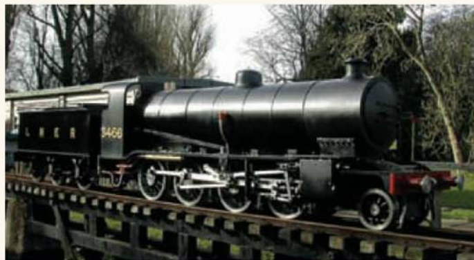
This fine photograph of Chingford DMEC's new loco., Martin Evans' 5in. gauge Nigel Gresley on its first appearance on the club track, 1 February 2004, when it had yet to be steamed, was sent to us by Robin Barfoot. He explains that, with the exception of the boiler which was professionally made, all parts were made by club members. Nearly everyone became involved, with almost all volunteering or being volunteered to make something depending upon their individual skills. In all it has been finished in about three years which is quite amazing when compared with the club electric loco. Dragonfly, which took closer to 23 years. Robin concludes his message thus: "We look forward to driving it and getting it run in before entering our passenger hauling service which begins at Easter. There were those that said the project would never get off the ground, let alone be finished. I'm glad they were wrong."
