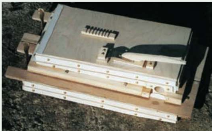
Twin bellows, air reservoir and release valve.
