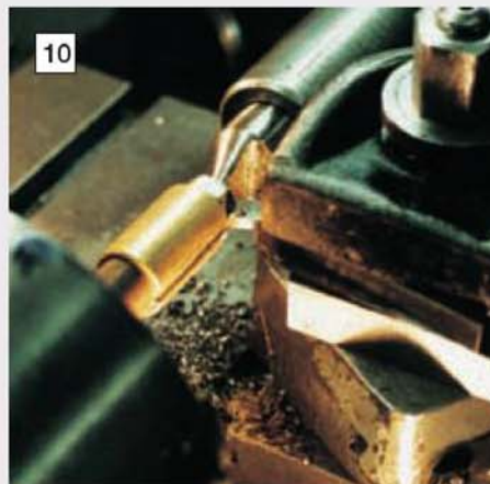
A keyway is cut into an Oilite bush by racking the lathe saddle to and fro.
