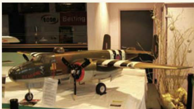
Colin Hammond's 1:6 scale WW2 B25 Mitchell bomber represents the prototype as Big Bad Bonnie and is powered by two 38cc petrol engines.
