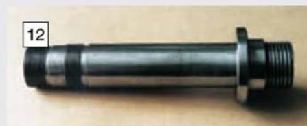
The finish turned spindle for the dividing head; a Myford spindle nose was used.
