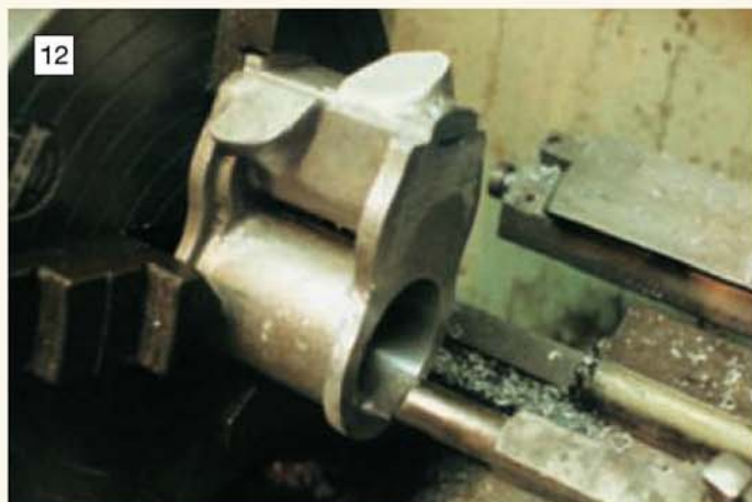
Operations on the cylinder barrels start with mounting the part in the 4-jaw chuck, facing off and then machining the cylinder bore to size for its liner.
