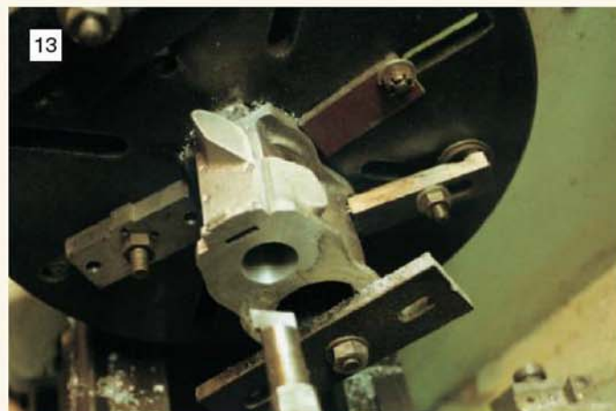
The casting is then reversed and held on the faceplate for boring the piston valve bore and facing the other end.
