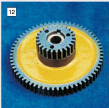
12 The 64/25 cluster on the 1in. long bush; the 25T gear detaches for exchange with the 64T gear.
