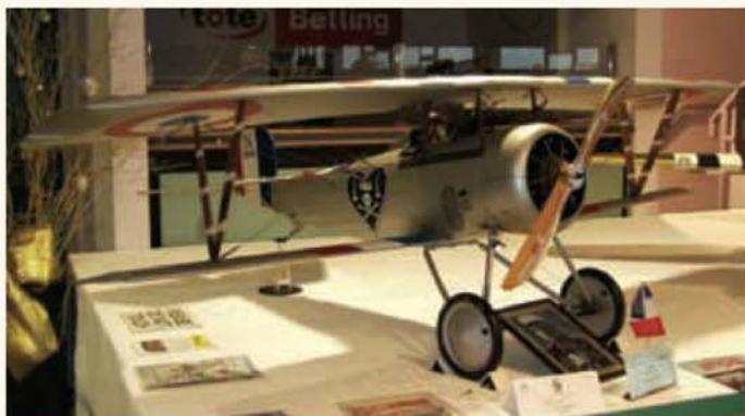
Unbelievably, Dave Horton's Nieuport 21/22b is 20 years old with over 3000 flights logged. Its 9ft. wingspan is powered by a 35cc OS BGX engine.
