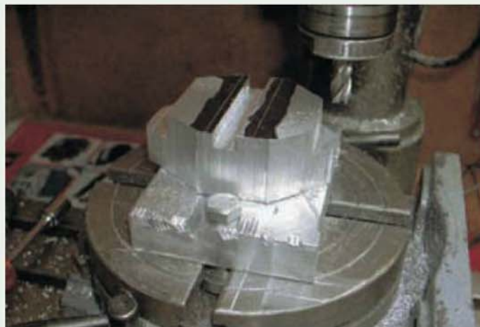
Initial profiling operations on the cylinder heads in the milling machine required the use of the rotary table again.
