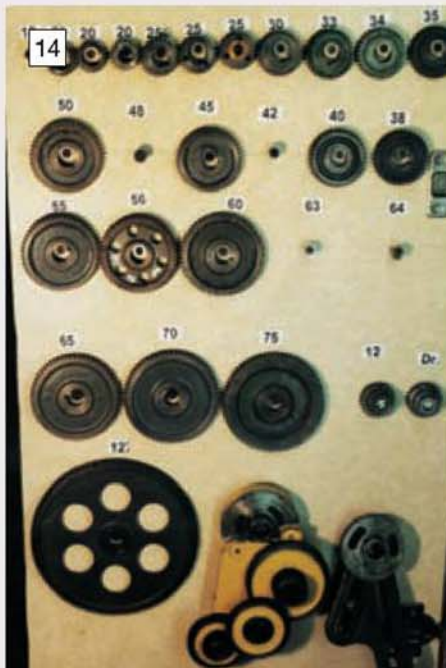
14 The change wheels are conveniently identified and stored on the left-hand hinged cabinet door.
