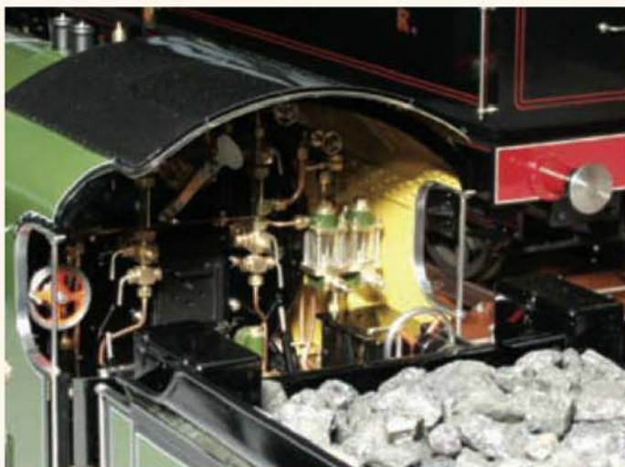
Peter Fagg designed the backhead fittings for Sir Bors de Ganis to a common scale determined by the availability of suitable gauge glass tubing.
