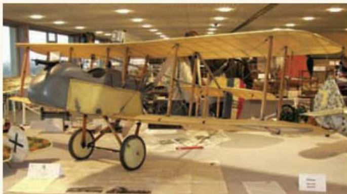
Ian Redshaw's Airco (de Havilland) DH2 has a 9ft. 6in. wingspan and is powered with a 62cc petrol engine driving a 30in. propeller.
