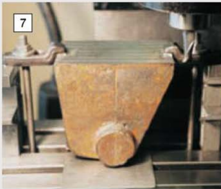
7 Machining the bottom surface of the dividing head casting.
