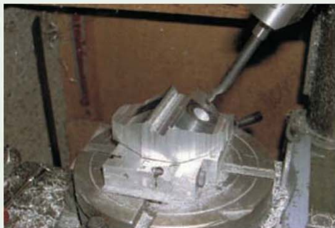
The valve seats were bored using an offset boring head. The rotary table enabled the work to be rotated to present the other valve seat.
