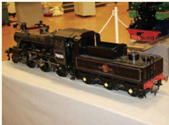
David Hudson's 5in. gauge BR Class 2 2-6-0 has been used as a vehicle for experimental purposes relating to draughting, superheating, etc.
