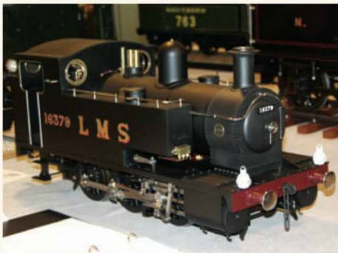
This 5in. gauge 0-6-0 dock shunter by Richard Castle is based on the Kennion Butch design worked up to represent a 1917 NB locomotive.
