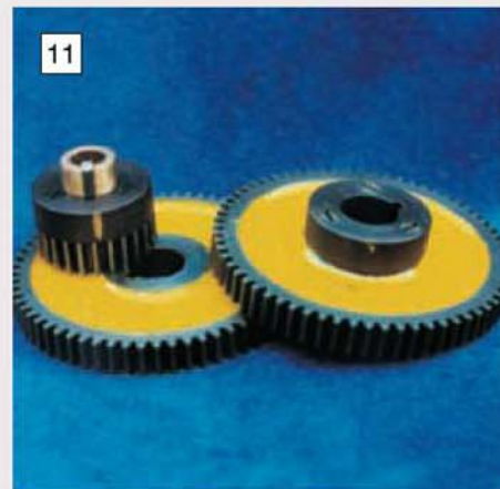
Blued steel \frac{3}{8} in. bosses are attached to the 25 and 64 tooth gears.
