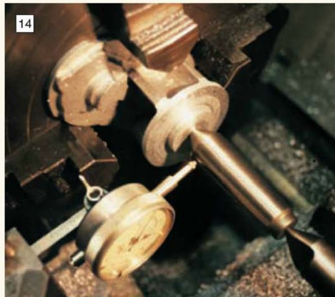
Setting one of the lower cylinder covers to run true in the 4-jaw chuck using a dial test indicator on a centre serving as a 'wobble bar'.
