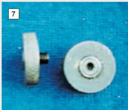
Large head thumb screws are made using 2BA countersunk screws.
