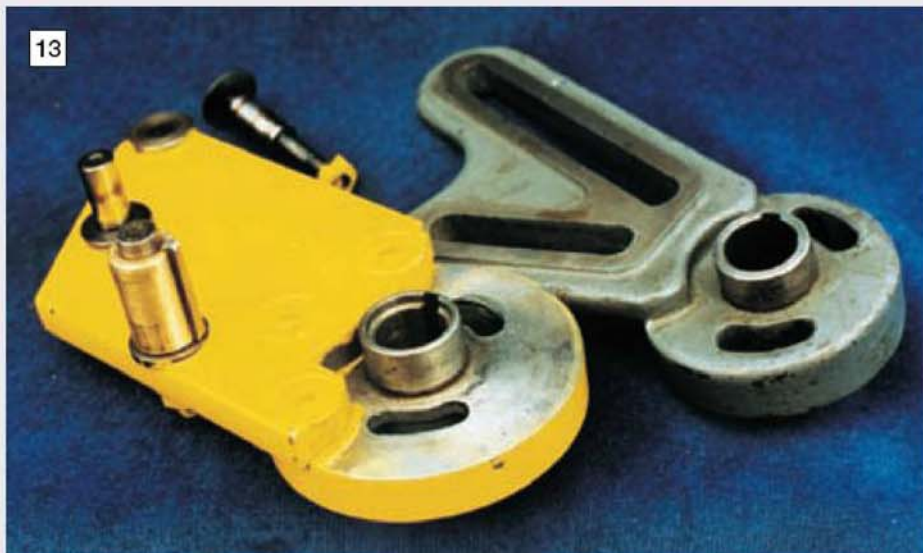
13 The Welland quadrant with its studs and bush shown with the standard Myford gear quadrant.
