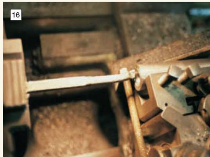
Boring one of the valve liners from the headstock of the lathe. The part is held in a Dickson tool holder which provides convenient height adjustment.
