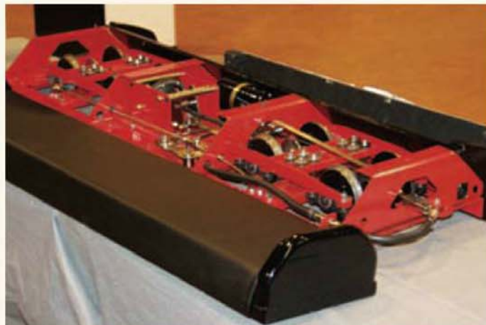
David Hudson's pivotless bogies with wheels to the Heumann profile and swing-link rubber suspension provide an exceptionally comfortable ride.
