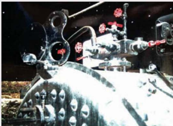
Backhead of prototype with the throttle just in sight at bottom right.
