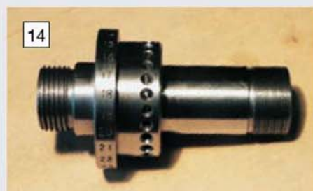
The simple indexer spindle after drilling and numbering the indexing holes.
