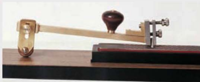
Mr. Derek Winks' device for honing indexable inserts with below, much enlarged views of a tip before (left) and after (right) attention.
