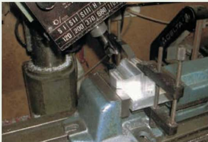
With the milling machine head set over to the required angle, the 30deg. facets for the valve inserts could be machined.
