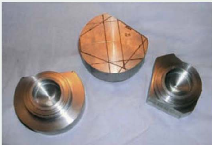
Preliminary operations on the new set of cylinder head blanks involved the use of simple turning operations and some attention with the bandsaw.
