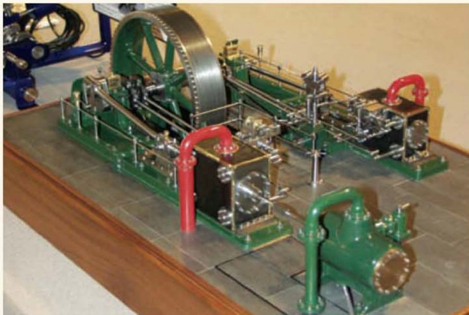
John Smith entered this fine cross-compound Corliss valve mill engine based on a design by the late Arnold Throp. It was awarded a well deserved Silver Medal and the Tom Nevins Memorial Trophy.
