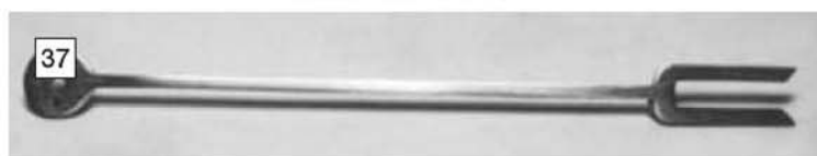
© Pendulum crutch to profile, all that remains is for the foot to be bent up at 90deg.
