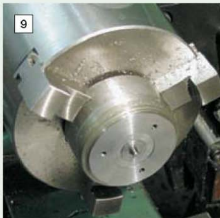
9 The special fixture used to finish the index discs to a good standard.
