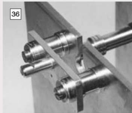
The back cock plate with suspension post fitted is mounted on the back plate.
