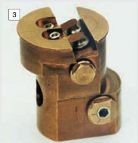
The complete poppet valve regulator block fully assembled and ready to be fitted into position through the boiler dome.
