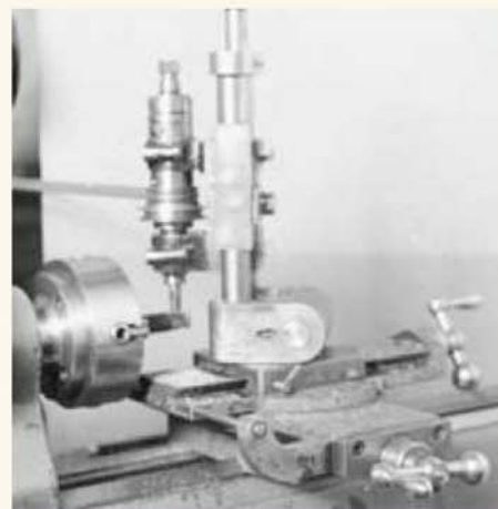
A milling spindle in use on the lathe to prepare a special drift.
