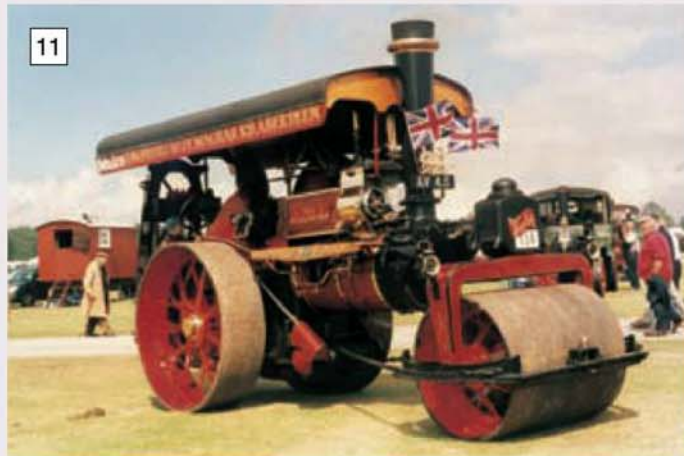
A Fowler DN1 roller works number 16235 built in 1924. She is a 7nhp engine weighing some 10 tons. The brass cylinder lagging, towing pin on the front roll scraper, and wooden canopy end boards are not Fowler features.
