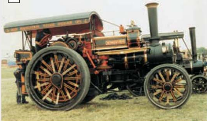
A TE2 haulage and winding engine built for Russia but never exported. Note the slanting shaft below the crankshaft which takes the drive to the winding drum beneath the boiler barrel.
