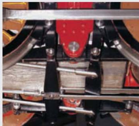
A tight squeeze: ashpan, brakes and equalisers.
