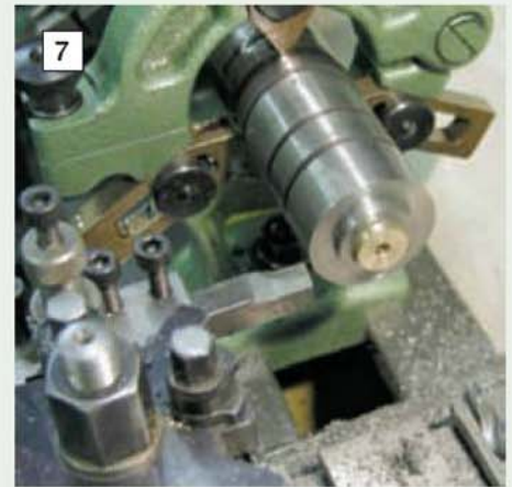
7 The brass sleeve has now been fitted to the index hub and the index disc locating boss turned.
