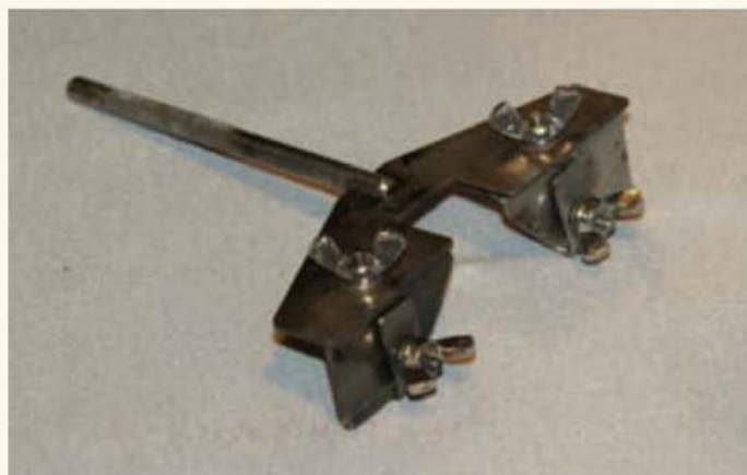
A simple tool, simply made, which works well, Gary Wooding's bandsaw blade soldering jig created considerable interest and was Commended.
