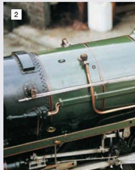
The regulator operating rod extends down the outside of the 'Brit' boiler.
