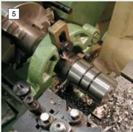
5 Turning multiple components. Here the sections have been defined with the parting tool.
