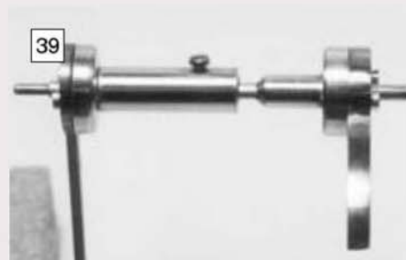
The crutch is fitted to the arbor and held in position with the adjustment screw.
