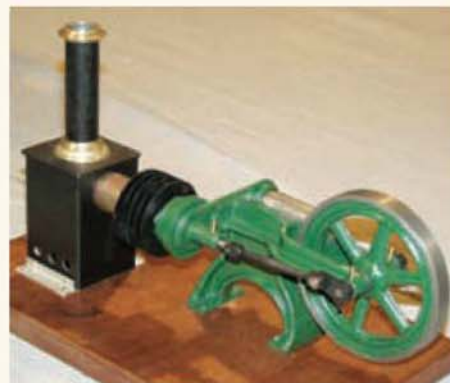
This 'gamma' type hot air engine entered by Ian Cornish was built from a German kit.
