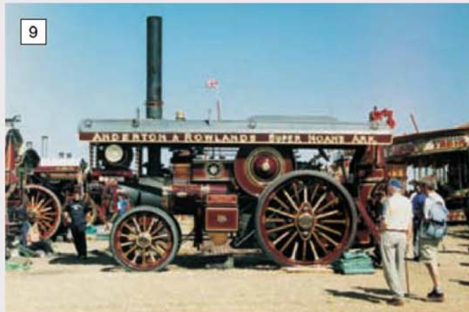
Fowler B6 10nhp showman's engine Lion Works No. 19782 photographed at the GDSF in 2003. Note the non-standard chimney top, as fitted from new.
