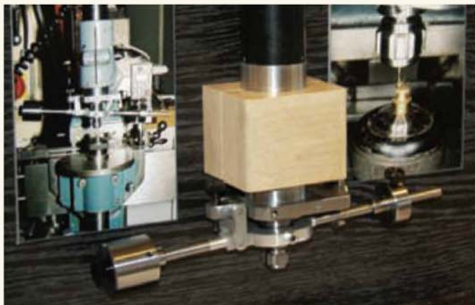
This attachment for his Aciera F1 milling machine by Dr. Peter Clark permits the use of drills down to 0.1mm diameter and was Very Highly Commended.
