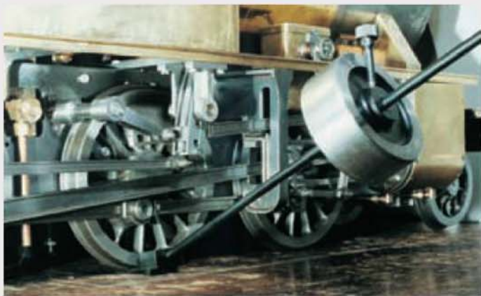
The loading gauge in use with the author's 5in. gauge 2-8-0 locomotive. The device is designed to be used with the locomotive standing on a hard surface.
