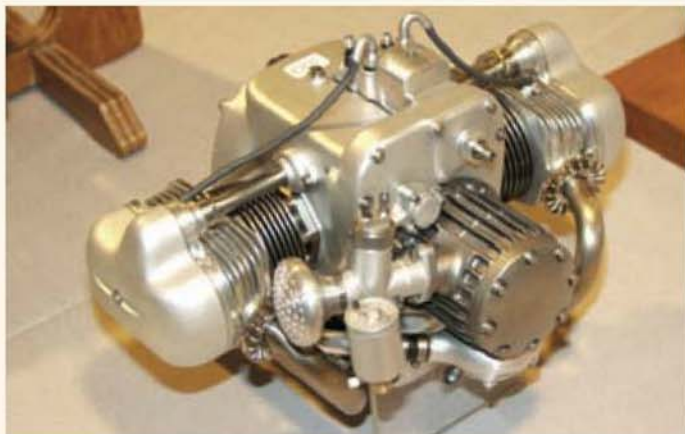
Rolf Depping's superb BMW RS500 horizontally-opposed twin-cylinder racing motor cycle engine of 1939 was awarded a Gold Medal and the Edgar Westbury Trophy.
