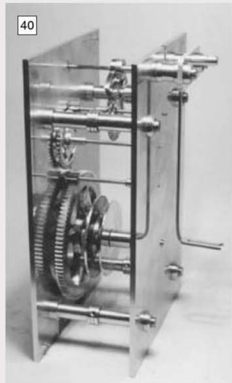
The movement can be assembled and set running while work continues on other parts.
