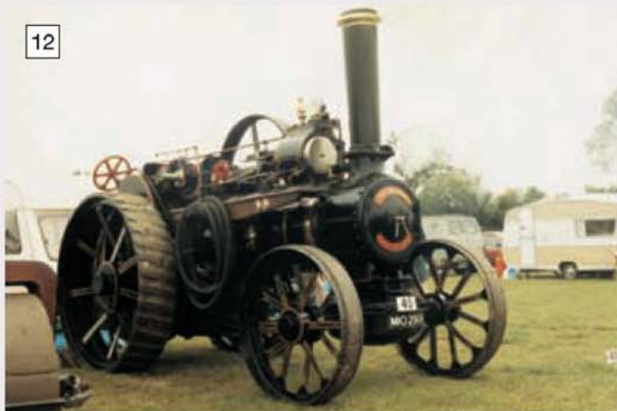
An example of a Fowler 6hp agricultural engine Works No. 11814 manufactured in 1919.
