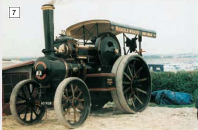
Class A9 7nhp road locomotive, Works No. 15462, built in 1919 demonstrates the classic Fowler light road locomotive outline.
