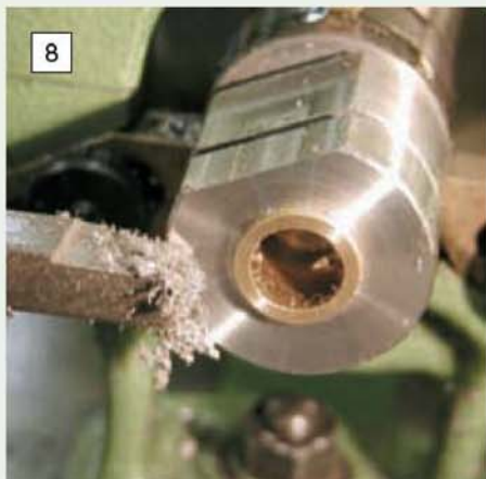
8 The index hub has now been parted off and the bearing fitted to the centre bearing housing.
