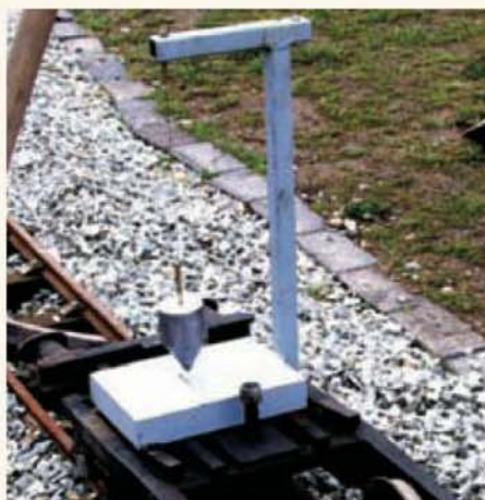
Checking and setting superelevation.
