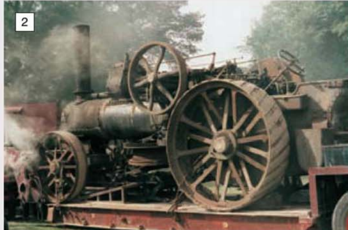
Fowler K7 10nhp ploughing engine built in May 1916 photographed in 'working order' raising steam on its low loader.
