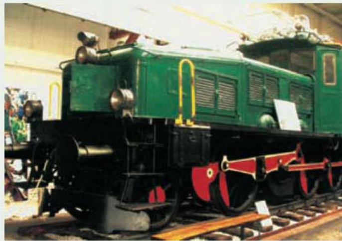
A 'Crocodile' locomotive from Switzerland whose articulated bogies allow tight curves on the railway.
