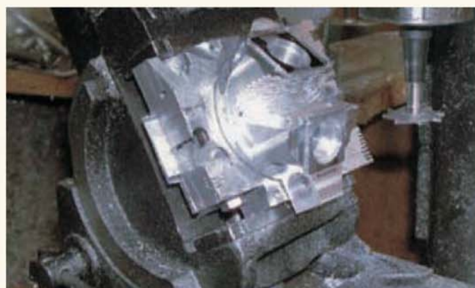
Here the final outline of the cylinder head is being generated in \frac{1}{16} inch steps using a home-made cutter.
