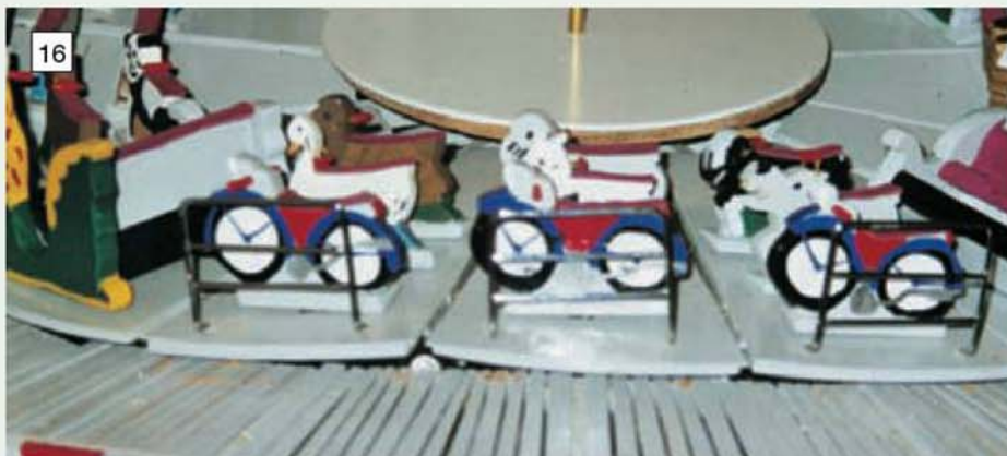
The safety rails were fitted alongside each of the rides.
