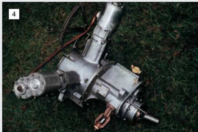
Another view of the engine and gearbox. Note the method of attaching the gearbox to the crankcase and the final drive arrangements.
