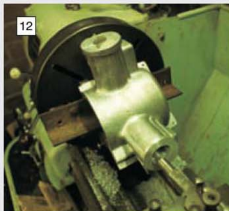
12 Boring the trunk guides with the work piece again mounted on the faceplate.
