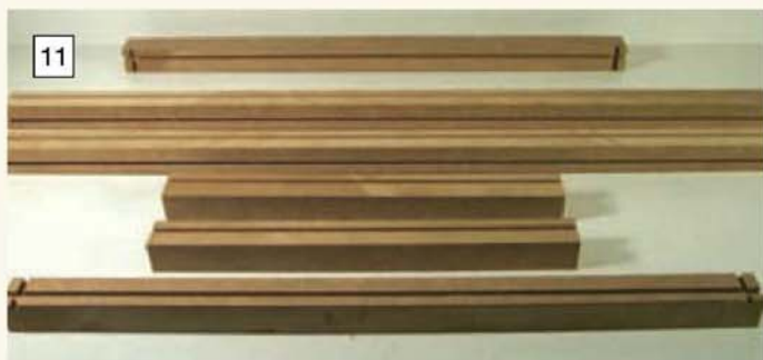
The \frac{3}{4} in square MDF case rails after the glazing groove had been cut.
