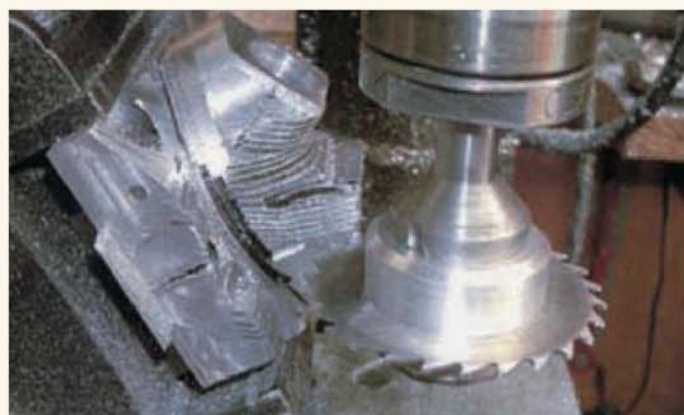
The more straightforward fins on the inlet turret were cut with a standard 0.035 in. slitting saw, one at a time because of varying depths.
