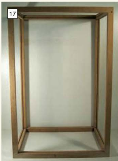
A temporary assembly to check alignments.
