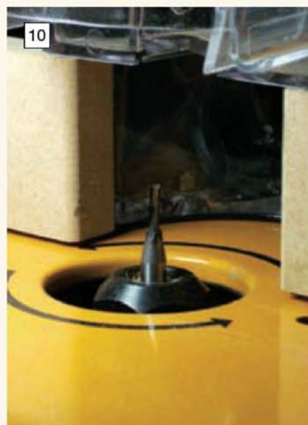
A \frac{1}{8} in. diameter routing cutter was used to machine the \frac{1}{8} \times \frac{1}{8} in. glazing grooves.
