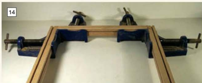
Mitre clamps are very useful for clamping the rail joints while the adhesive cures.
