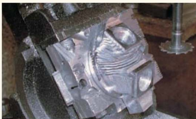
Cutting the cooling fins with a 1 in. dia. x 0.035 in. wide cutter. Many of these cutters were made before achieving a successful design.
