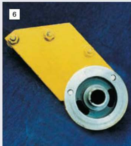
The fabricated quadrant showing the relief groove for the arcuate slots.
