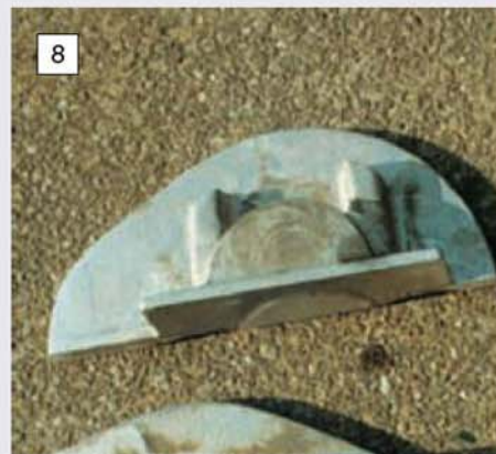
Rear flange and bearing housing castings as received from the foundry.
