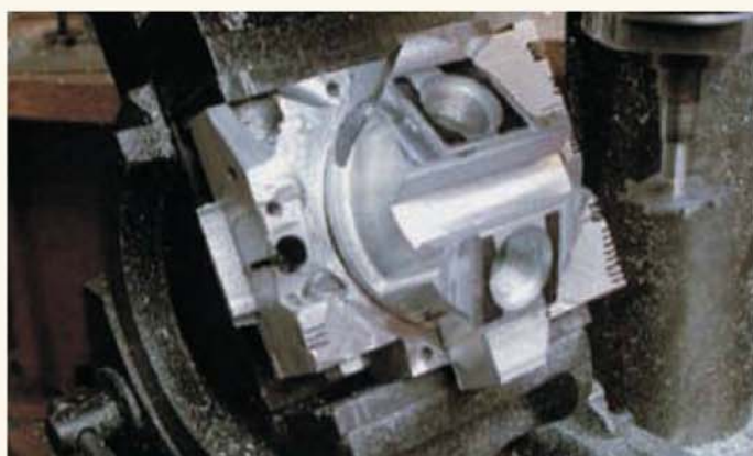
A tilting vice was used to hold the fixture and workpiece for some of the detailed shaping operations on the cylinder heads.
