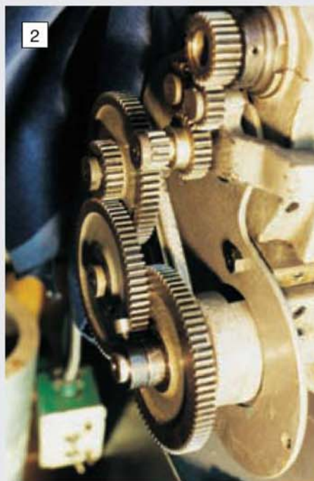
The standard Myford feed train set up using the optional 12 tooth input gear.
