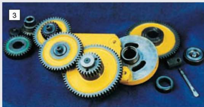
The new quadrant with its fixed train of gears. Those on the left are the input gear and tumbler sleeve gear.
