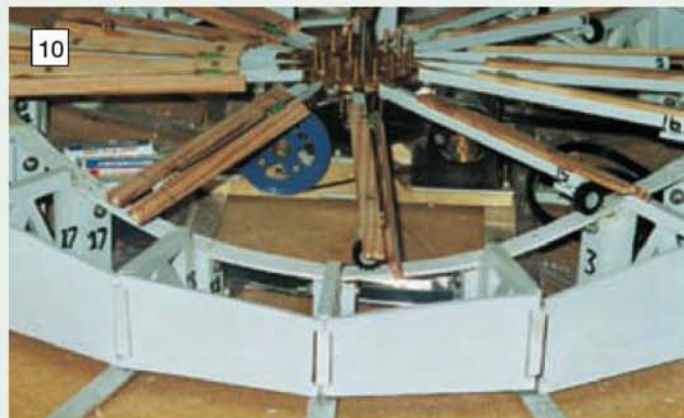
Bar hinges were made, fitted and adjusted for free movement.
