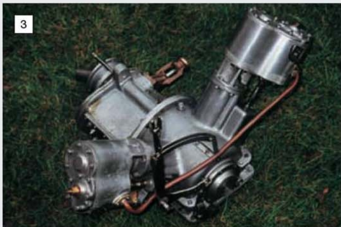
A view of the completed V-twin engine and gearbox assembly showing the reversing lever and steam receiver pipe.
