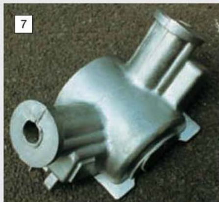
The crankcase top half casting as received from the foundry and prior to machining.
