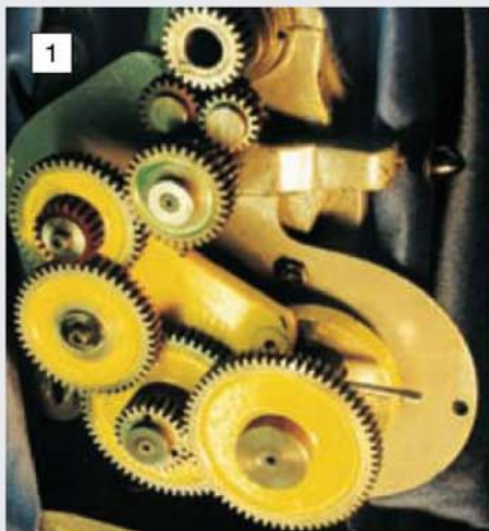
The Welland gear quadrant fitted to the author's Myford ML7 lathe.
