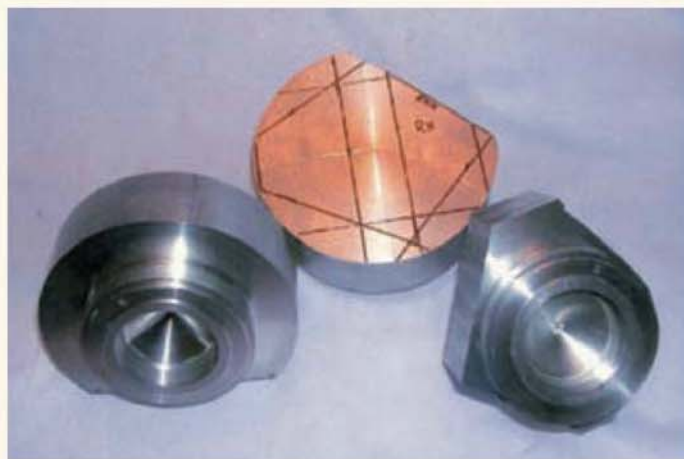
The first stages in cylinder head manufacture. Left: the blank has been screw cut. Centre: marked out for band sawing. Right: band sawn to shape.
