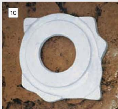
10 The aluminium alloy casting used as a fixture plate for machining the crankshaft.
