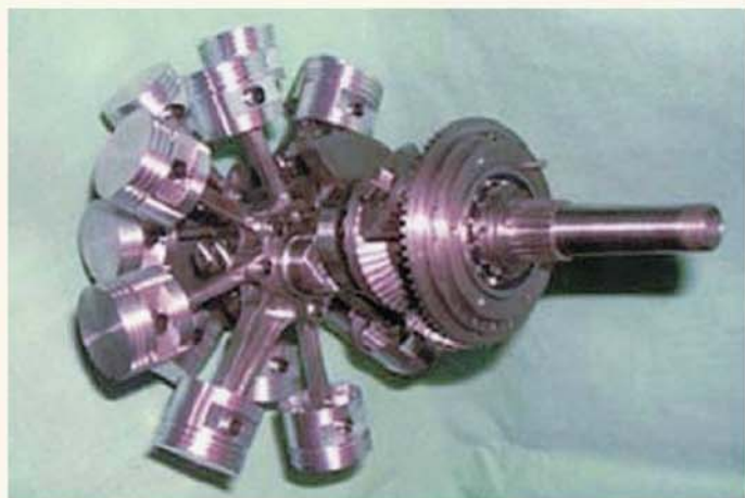
The complex crank assembly complete with the speed reducer assembly, the master con-rods, con-rods and pistons.
