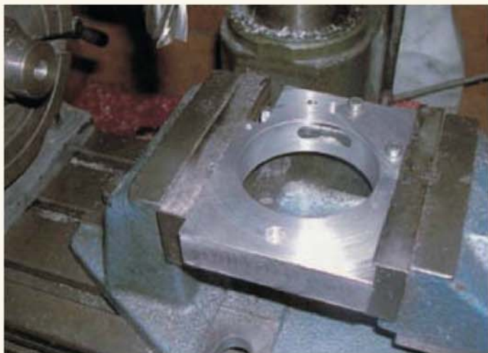
The fixture devised for holding the cylinder head blanks for milling. The blanks are clamped by the tapered plugs.
