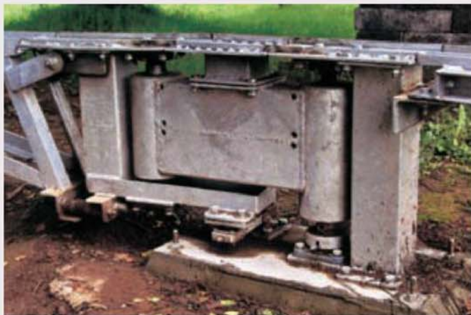
Construction is substantial; springs are used to counterbalance the weight of the swing beam and the assembly has been galvanised for longevity.
