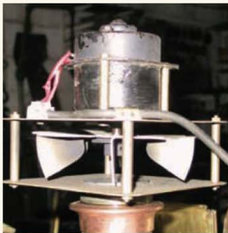
Essentially simple, this blower is constructed around a suitable ex-automotive 12V dc motor.
