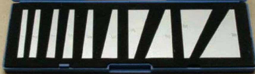
A set of inexpensive but serviceable imported angle gauges ideal for home workshop use.
