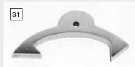
The impulse faces are brought to a high level of finish, checked and adjusted as necessary.
