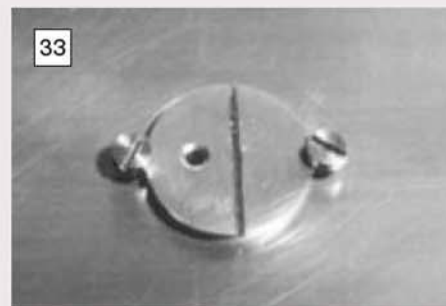
The eccentric bush is adjusted using a screwdriver and secured with two 10BA screws.
