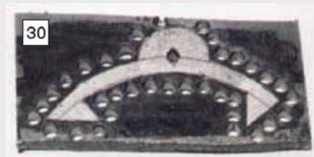
The pallet outline can be prepared by chain drilling, sawing and careful filing to the pattern.
