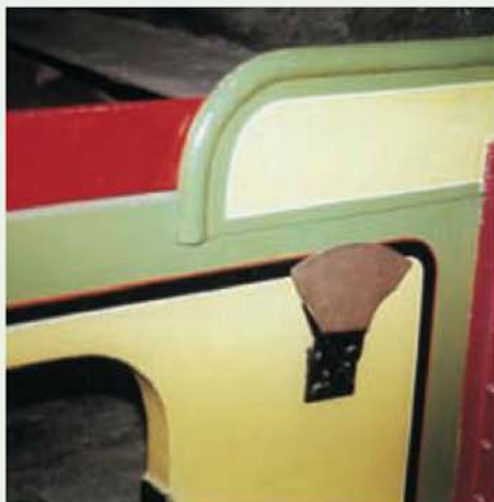
Front of tank; note shovelling plate hole and side plate.
