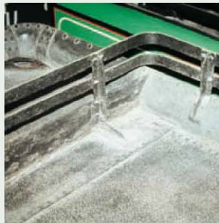
Detail of coal rails at rear of tank.
