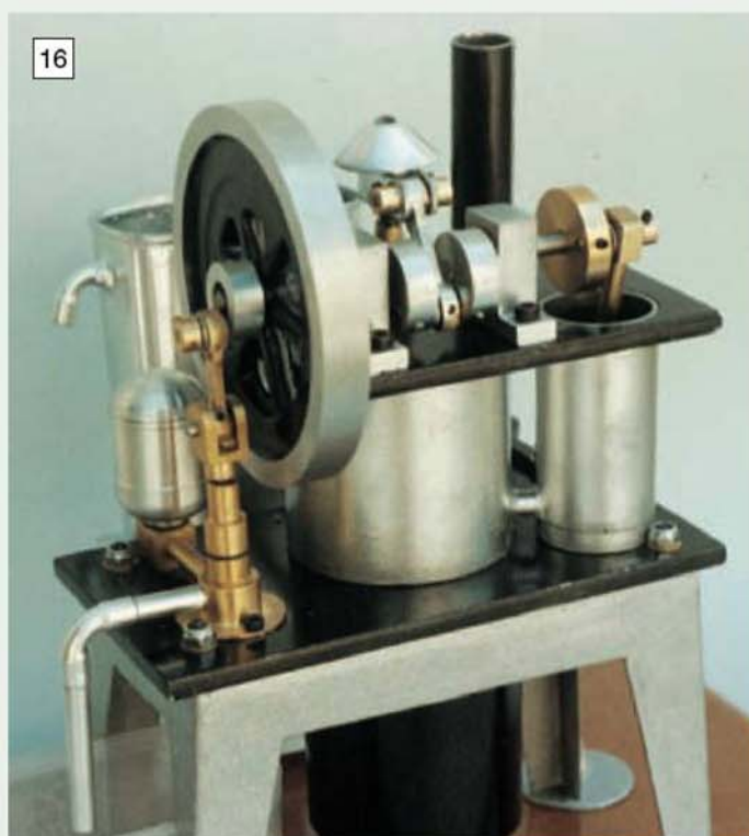
The Author's Hopkins Mk. II engine starts easily and by adjustment of the phase angle can be fine tuned to maximise efficiency.
