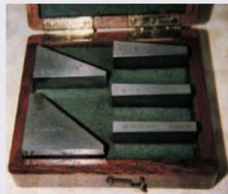
The set of angle blocks made by the Author and housed in a smart beize lined wooden case.
