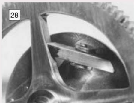
The face angle of the click should be such that its full width bears against the crossing.
