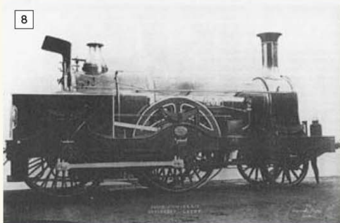
Above left: Archibald Sturrock's 2-4-0 GNR express locomotive built at the Steam Plough works. Above Right: a John Fowler 0-4-0 traction tram engine built in 1866. Note the single large wood brake block behind the back wheel.
