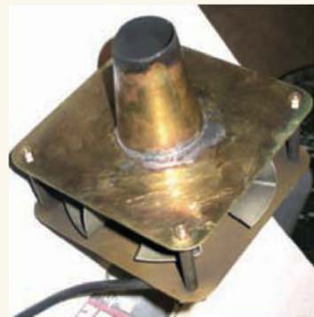
The body is furnished with a tapered inlet to suit a range of chimney diameters.
