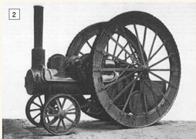
The 1877 'Steeplechaser' fitted with 12ft. diameter back wheels. Note the large drive gear visible on the inside of the far back wheel rim.
