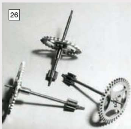
The wheels and pinions assembled and fixed to their arbors with Loctite.
