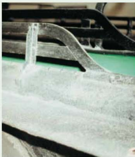
Front of coal rails; note recessed coal plate.
