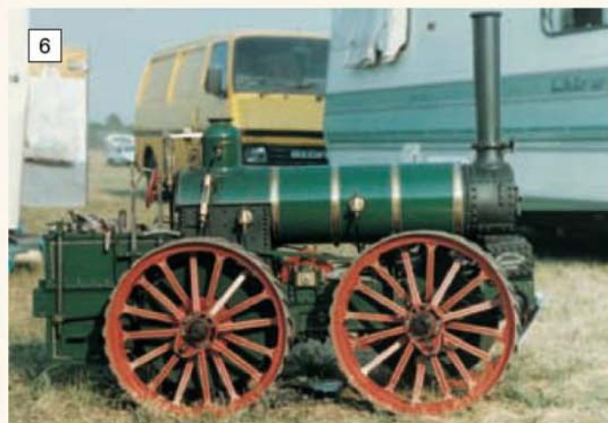
Above left: works photograph of Fowler's undertype four-wheel drive traction engine of 1886. Above right: A very fine 3in. scale model of the undertype engine in photo 5 built by Les Vince. Note for safety reasons the gauge frame on the model has a protector but other than that it is very close scale indeed.
